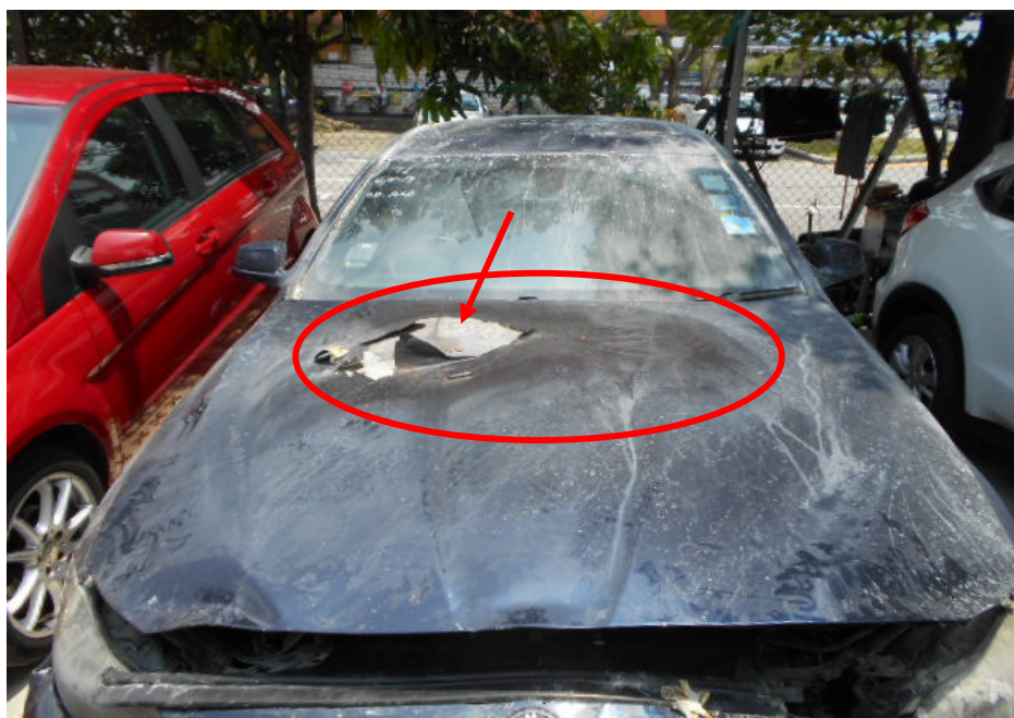
Photo 8 shows the whitish burn marks (arrowed) that were found on the rear right area of the Insured Vehicle's front bonnet, within an area (circled) of the front bonnet that was found with paint blackened. Such whitish burn marks are a result of exposure to prolong heat intensity. Following the characteristic of heat rising upwards, the fire to the Insured Vehicle can then be determined to have originated around the rear right area of the engine compartment.
