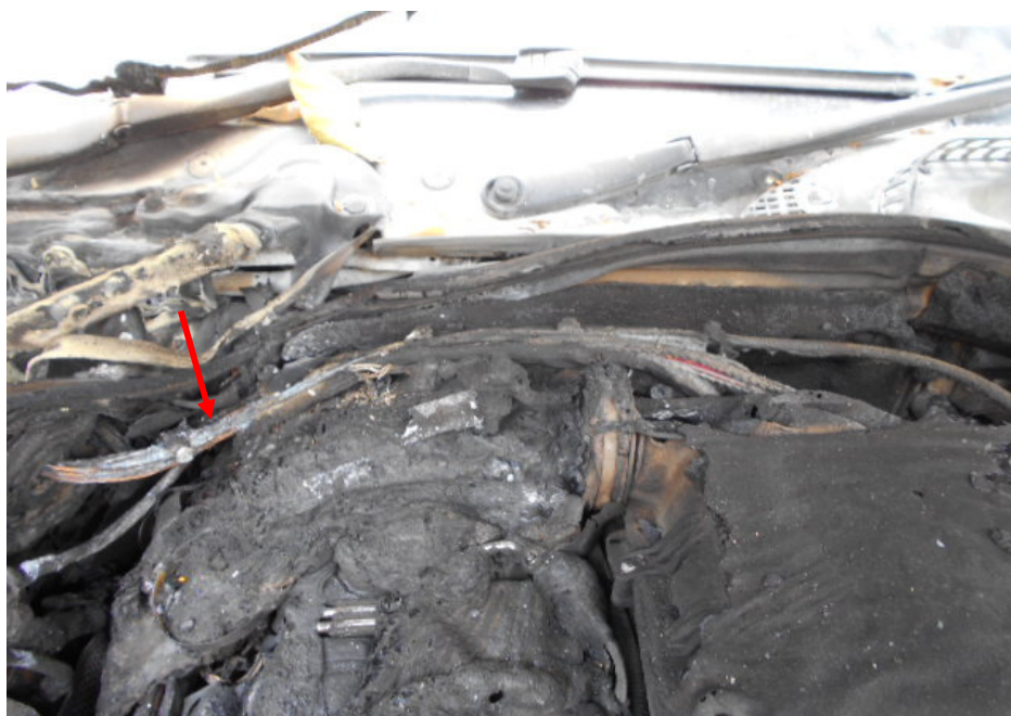
Photo 11 shows the stretch of wirings at the rear right area of the Insured Vehicle's engine compartment, which was where the fire had originated. Greenish residue was found along a stretch of original factory fitted wirings. The presence of such greenish residue suggests occurrence of an electrical short circuit.
