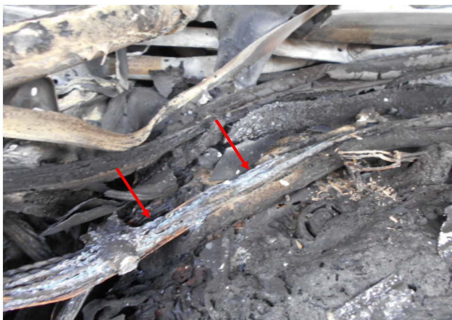
Photo 12 shows a closer view of the greenish residue (arrowed) that were found on the original factory fitted wirings at the rear right area of the Insured Vehicle's engine compartment. The presence of greenish residue suggests occurrence of an electrical short circuit. This physical evidence would then appear to suggest that the cause of fire to the Insured Vehicle was due to electrical in nature.
