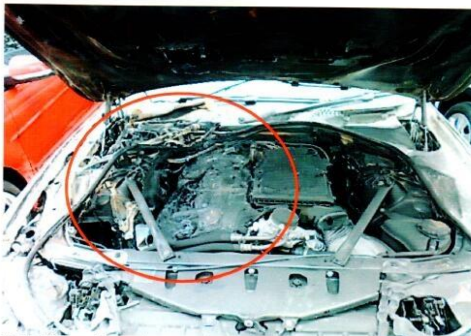
Photo 3 shows the engine compartment of the Insured Vehicle at the time of my inspection. The fire damage was observed to have been more severe at the right side of the engine compartment (circled). The parts that were found to have been burnt and/or melted include the air intake manifold, engine top cover, air filter housing, various hoses and pipes amongst others.
