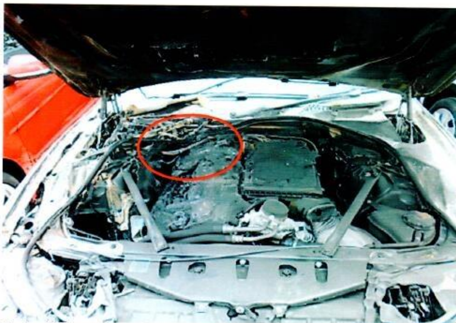
Photo 10 shows the engine compartment of the Insured Vehicle. Following the burn pattern, in particular the location where the high heat intensity burned marks were found on the front bonnet, and the characteristic of heat rising upwards, the fire to the Insured Vehicle had originated around the rear right side (circled) of the engine compartment. Correspondingly, the extent of fire damage was more severe at the right side of the engine compartment.
