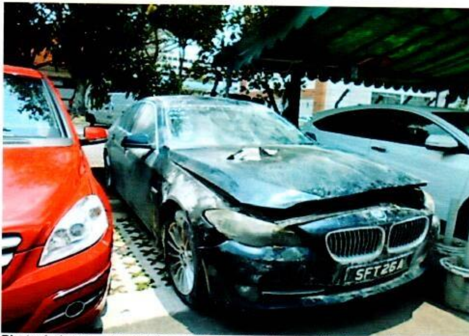
Photo 1 shows a general view of the front right body of the Insured Vehicle at the time of my inspection. The fire damage to the Insured Vehicle was confined to its frontal right body. Its front bumper, front bonnet, front right headlamp and front right fender were amongst the exterior body parts that were found to have been affected as a result of the fire.
