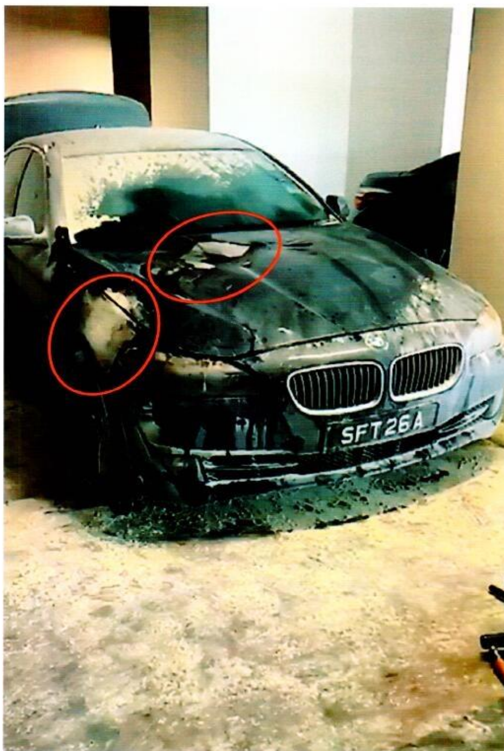
Photo 5 shows a screenshot taken from the video recording that was provided by Mr Ang. The damage of burnt nature to the Insured Vehicle immediately after the fire was put out had corresponded to the damage as seen by me during my inspection of the Insured Vehicle ie the frontal right body (circled) of the Insured Vehicle was exteriorly affected. Also, apart for the powder residue left behind by fire extinguishers, there appears to be no unusual foreign material(s) and/or object(s) found on the ground in the immediate area of where the Insured Vehicle was parked.
