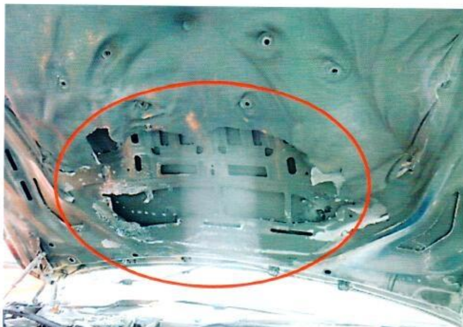
Photo 9 shows the underside of the Insured Vehicle's front bonnet. The front bonnet insulator at the rear centre area was melted whereas other areas was observed to be intact. The melted area of the front bonnet insulator was directly below the area where the paint at the top side of the front bonnet was blackened.
