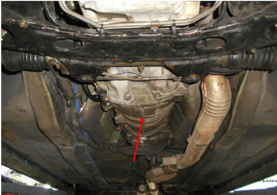
Photo 2 shows a general view of the transmission assembly (arrowed) that was fitted on the Motor Car. The front (input) side of the transmission is bolted to the crankshaft side of the engine block while the rear (output) side of the transmission was connected to the propeller shaft, which links to the rear axle of the Motor Car.
