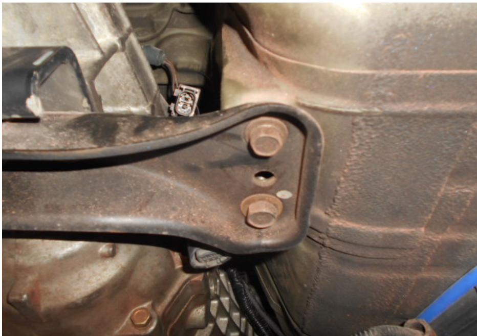
Photo 7 shows the bracket mounted on the underside of the Motor Car's floor board, via bolts and nuts.
