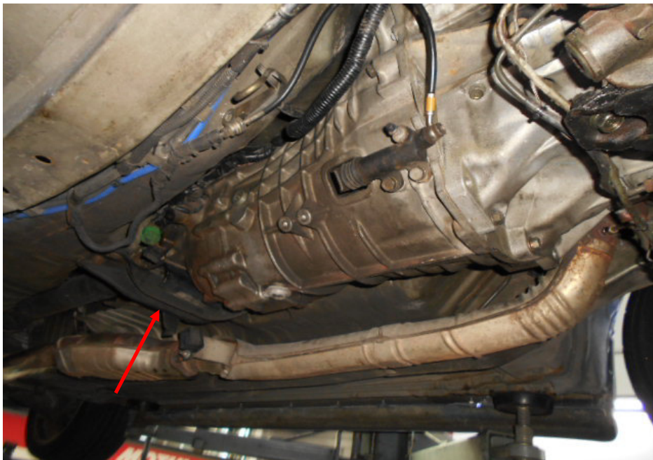
Photo 3 shows a general view of the bracket (arrowed) mounted to the underside of the floor board of the Motor Car, via bolts and nuts. The bracket supports the rear (output) side of the transmission.
