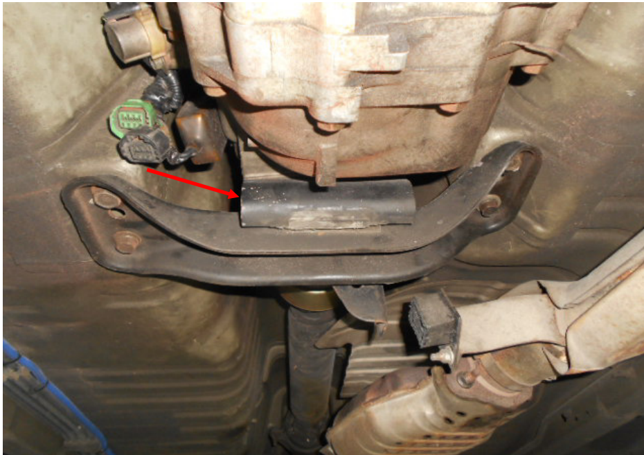
Photo 4 shows a closer view of the bracket mounted to the underside of the Motor Car's floor board, via bolts and nuts. The bracket supports the rear (output) side of the transmission. Rubber bushings (arrowed) absorbs any vibrations arising from the rotation of the transmission gears, minimising any stress to the bracket.
