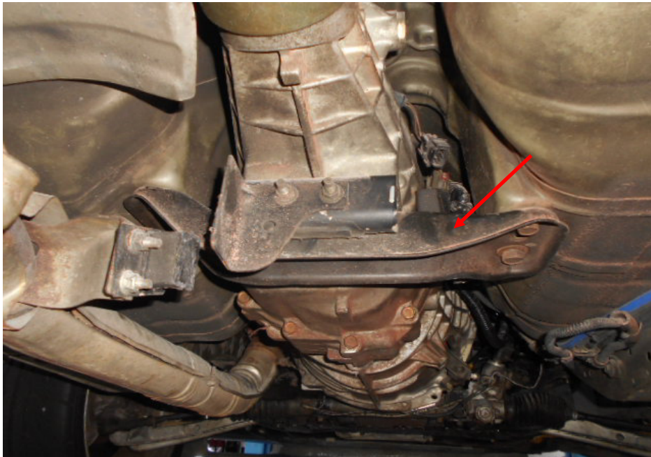
Photo 6 shows a general view of the transmission assembly that was fitted on the Motor Car, as viewed from the rear to front. The transmission assembly is supported by a bracket (arrowed) that is mounted on the underside of the floor board of the Motor Car, via bolts and nuts.
