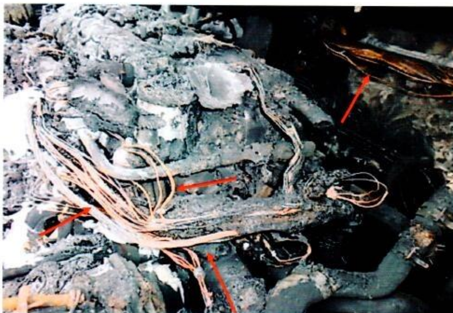
Photo 11 shows the wirings at the rear centre area of the Insured Vehicle's engine compartment. Several stretches of wirings (arrowed) at/or around the immediate vicinity of the rear centre area were found to be burnt to its bare copper state. Such condition normally indicates internal heating of copper wires which is a sign of an electrical short circuit occurring. These wirings were all original wiring harnesses of the Insured Vehicle.
