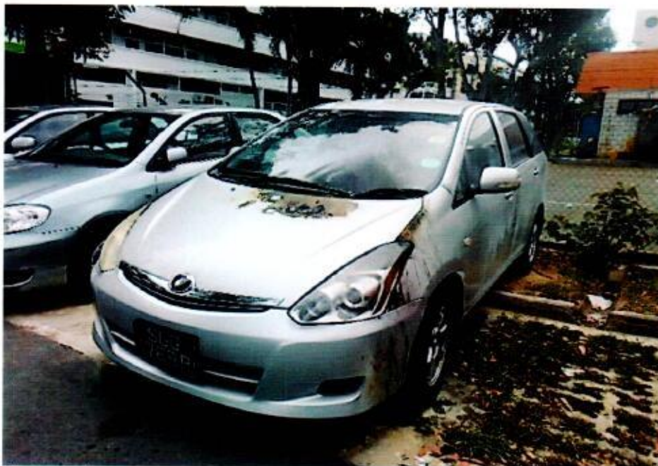
Photo 2 shows a general view of the front left body of the Insured Vehicle at the time of my inspection. The fire damage was confined to the engine compartment of the Insured Vehicle. Exterioirly, only the front bonnet, front left fender and front windscreen were affected by the incident.
