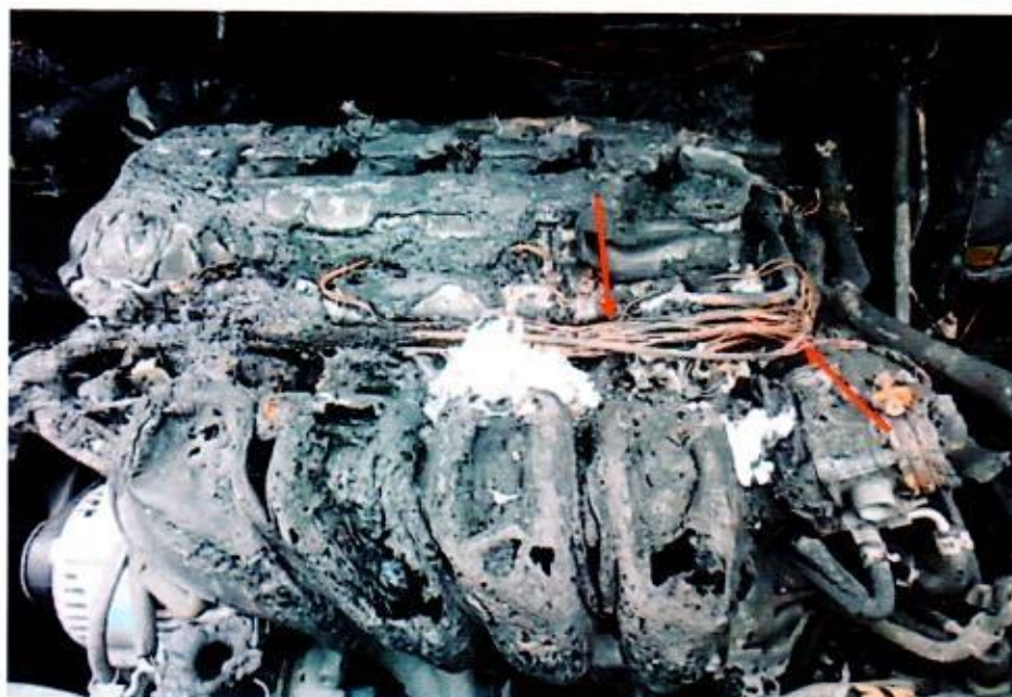
Photo 10 shows the centre area of the Insured Vehicle's engine compartment. Several stretches of wirings (arrowed) at/or around the immediate vicinity of the rear centre area were found to be burnt to its bare copper state. The bright reddish colour of the copper wires suggest that the wirings were exposed to high heat. Such condition normally indicates internal heating of copper wires which is a sign of an electrical short circuit occurring.
