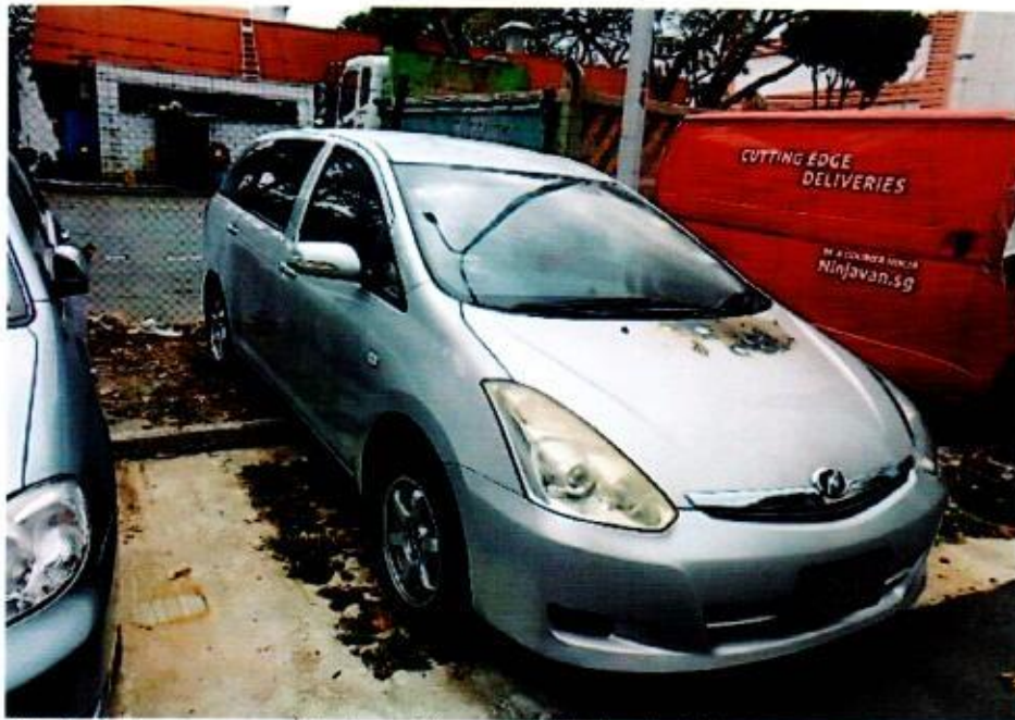
Photo 1 shows a general view of the front right body of the Insured Vehicle at the time of my inspection. The fire damage was confined to the engine compartment of the Insured Vehicle. The interior compartment and the rear portion of the Insured Vehicle were unaffected.
