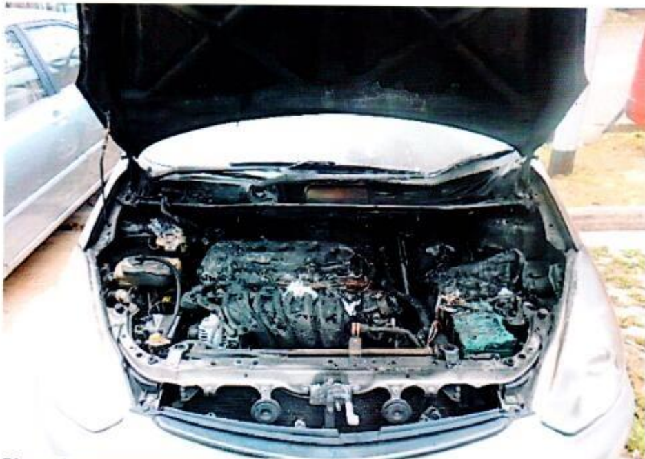
Photo 3 shows a general view of the Insured Vehicle's engine compartment at the time of my inspection. Most of the parts and components within the engine compartment were burnt and/or melted. This had included various rubber hoses, wiper panel, battery, air intake duct, fuse box, brake fluid reservoir, cooling fan, radiator, intake manifold and alternator amongst others.
