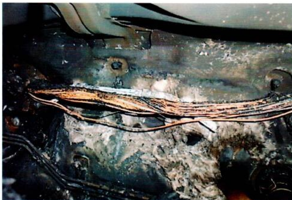
Photo 12 shows the wirings at the rear centre area of the Insured Vehicle's engine compartment, which was where the fire to the Insured Vehicle had originated. Several stretches of wirings at/or around the immediate vicinity of the rear centre area were found to be burnt to its bare copper state, an indication of an electrical short circuit occurring. These wirings were all original wiring harnesses of the Insured Vehicle.
