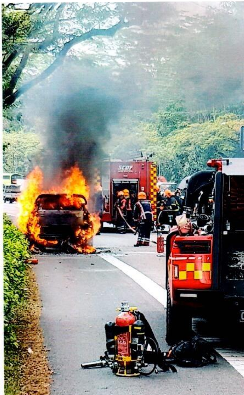
Photo 8 shows the Insured Vehicle completely covered by fire at the incident scene (photograph taken by Mr Wang). Upon examination of the photographs provided, it was noted that flames had first engulfed the frontal portion of the Insured Vehicle, outside of its interior compartment before spreading to its rear portion. Base on the sequence of events seen from the photographs provided by Mr Wang and shown in photograph 6 to 8 above, it can be established that the fire to the Insured Vehicle had originated at its frontal portion, outside of its interior compartment.
