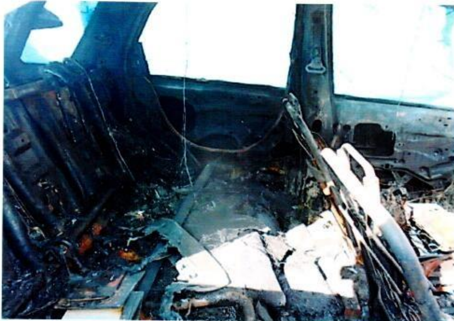
Photo 3 shows the interior compartment of the Insured Vehicle. All the parts inside the interior compartment were found to be extensively burnt. Its front seats, rear seats, roof upholstery, carpet and various trims were all burnt and/or melted as a result of the fire.
