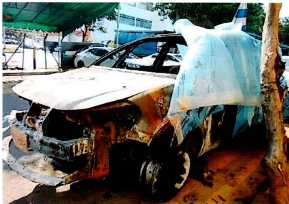
Photo 2 shows a general view of the front left body of the Insured Vehicle at the time of inspection. The Insured Vehicle was observed to have sustained extensive fire damage all around. The body panels at the frontal portion and the undercarriage components at the front underside were all burnt to char.
