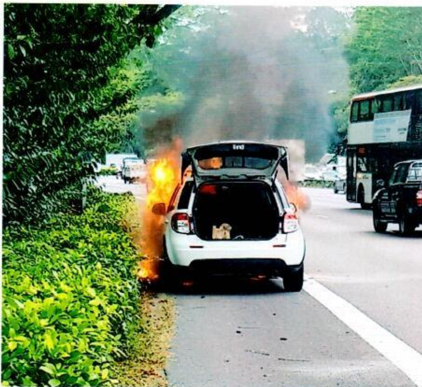
Photo 6 shows the Insured Vehicle at the incident scene. From the photographs provided by Mr Wang, the Insured Vehicle could be seen parked along the road shoulder with the fire at its frontal portion, outside of its interior compartment. The flames thereafter spread to its interior compartment before spreading to its rear portion and eventually covering the entire Insured Vehicle. Base on the sequence of events seen from the photographs provided by Mr Wang, it can be established that the fire to the Insured Vehicle had originated at its frontal portion.
