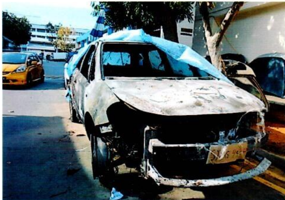
Photo 1 shows a general view of the front right body of the Insured Vehicle at the time of inspection. The Insured Vehicle was observed to have sustained extensive fire damage all around. The body panels at the frontal portion and the undercarriage components at the front underside were all found to have been burnt to char.
