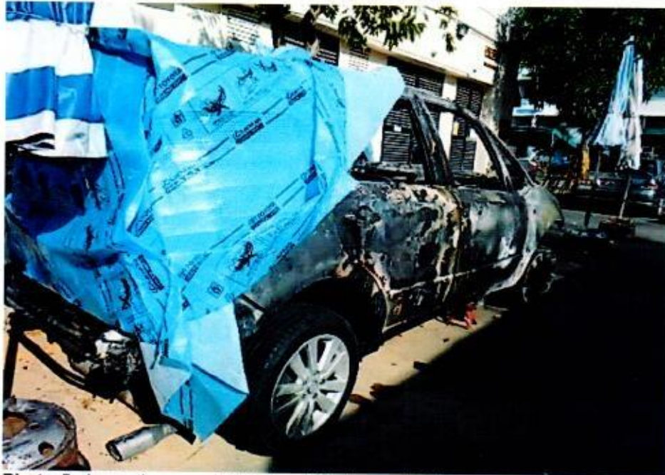
Photo 5 shows the rear right body of the Insured Vehicle. Comparing the overall extent of fire damage like the rear tyres vs the front tyres, rear exhaust pipe unaffected etc, it would appear that the frontal portion of the Insured Vehicle was more affected as compared to its rear portion.
