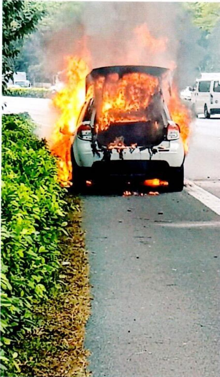
Photo 7 shows the Insured Vehicle with the fire having spread to its interior compartment (photograph taken by Mr Wang). Base on the sequence of events seen from the photographs provided by Mr Wang, it can be established that the fire to the Insured Vehicle had originated at its frontal portion, outside of its interior compartment.
