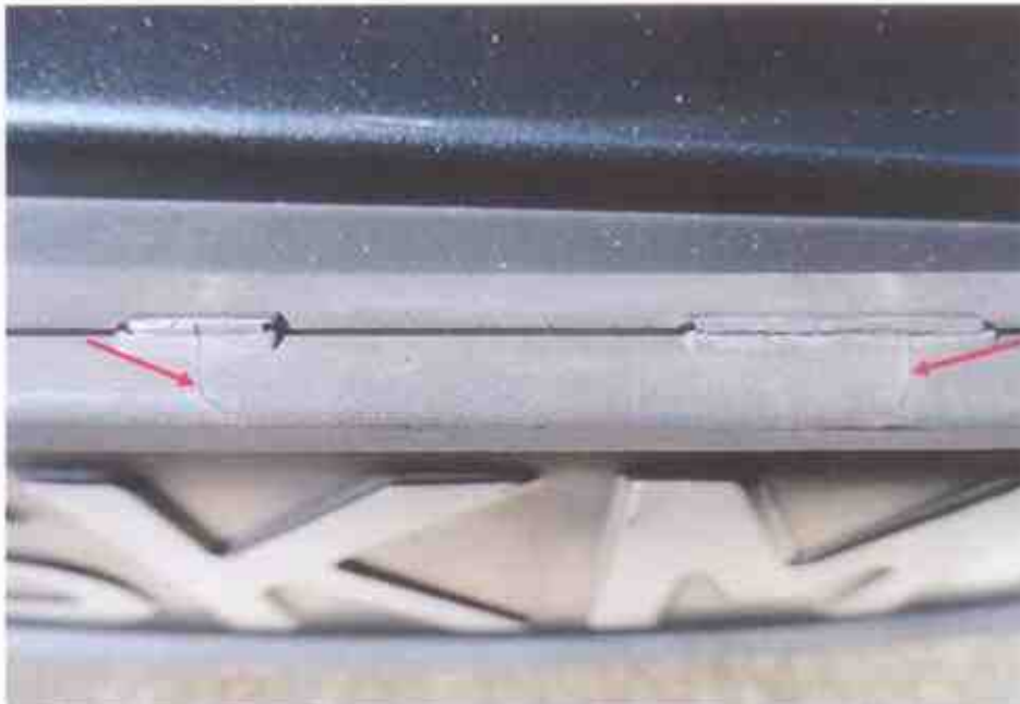
Photo 10 shows a close up view of the cracks on the top centre portion of the Mercedes's front number plate frame (red arrows).
