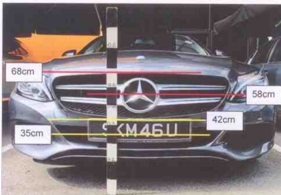
Photo 17 shows the height measurement being conducted on the front portion of the Mercedes. The height range of the damages found on the front number plate and the front number plate frame was measured to be between 35cm and 42cm. The height above ground level of the front emblem where the dent was found was measured to be approximately 58cm. The height above ground level of the white mark on the front centre portion of the Mercedes's front bonnet was measured to be approximately 68cm.
