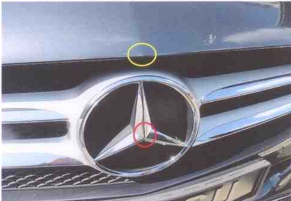
Photo 6 shows the white mark on the centre portion of the front bonnet (yellow circle). The front emblem was observed to be slightly dented at the centre portion (red circle).
