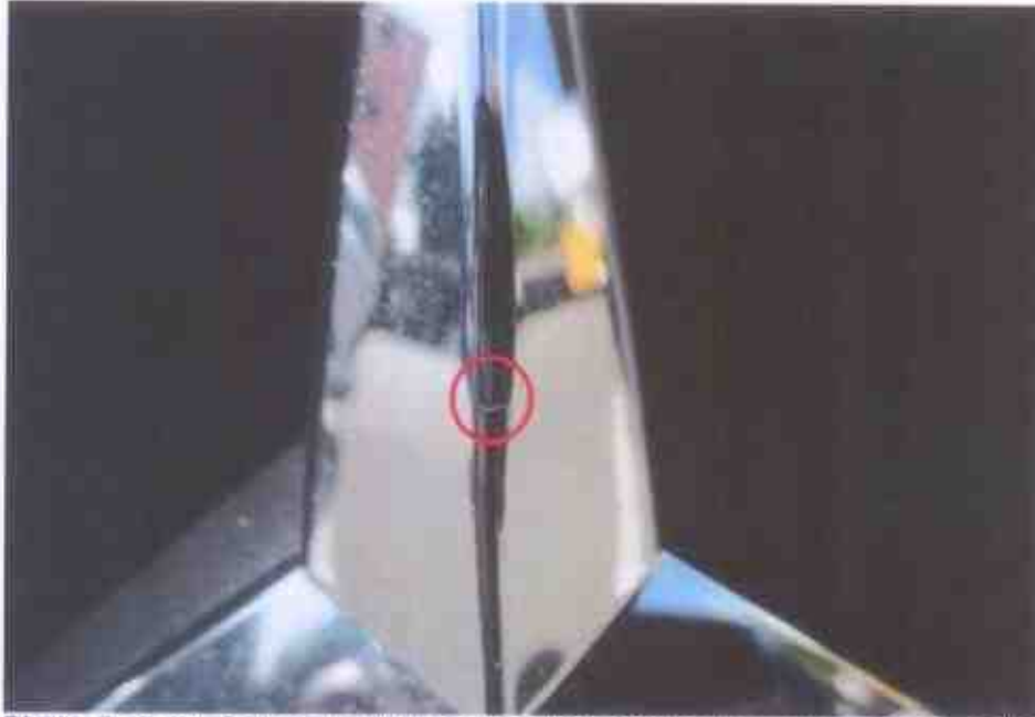
Photo 8 shows a close up view of the slight dent at the centre portion of the Mercedes's front emblem (circled).
