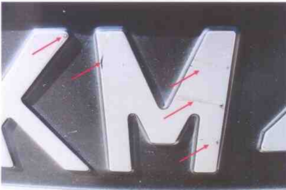
Photo 11 shows a close up view of the several black marks on the alpha-numeric letterings of the front number plate of the Mercedes (red arrows).
