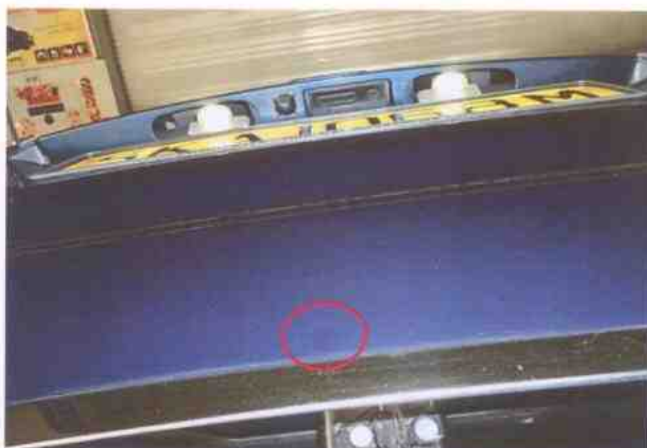
Photo 4 shows a close up view of the slight dent on the lower centre portion of the boot lid (circled).
