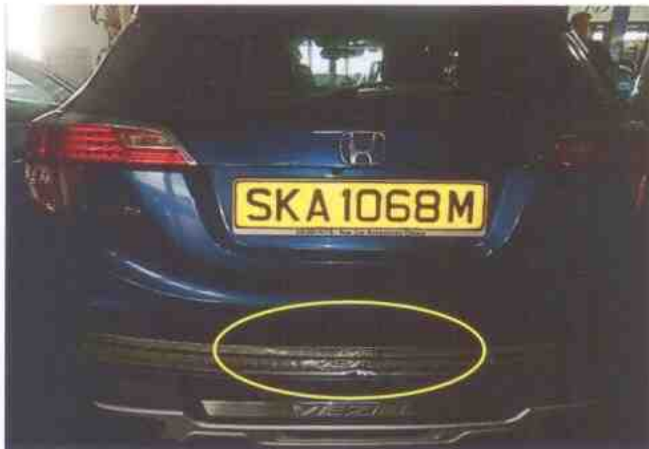
Photo 1 shows the general view of the rear of the Honda at the time of the Pre-Repair Survey conducted by LKK Auto Consultants Pte. Ltd. taken 5 months after the accident. The damage to the Honda was observed to be confined to its rear centre portion (circled).
