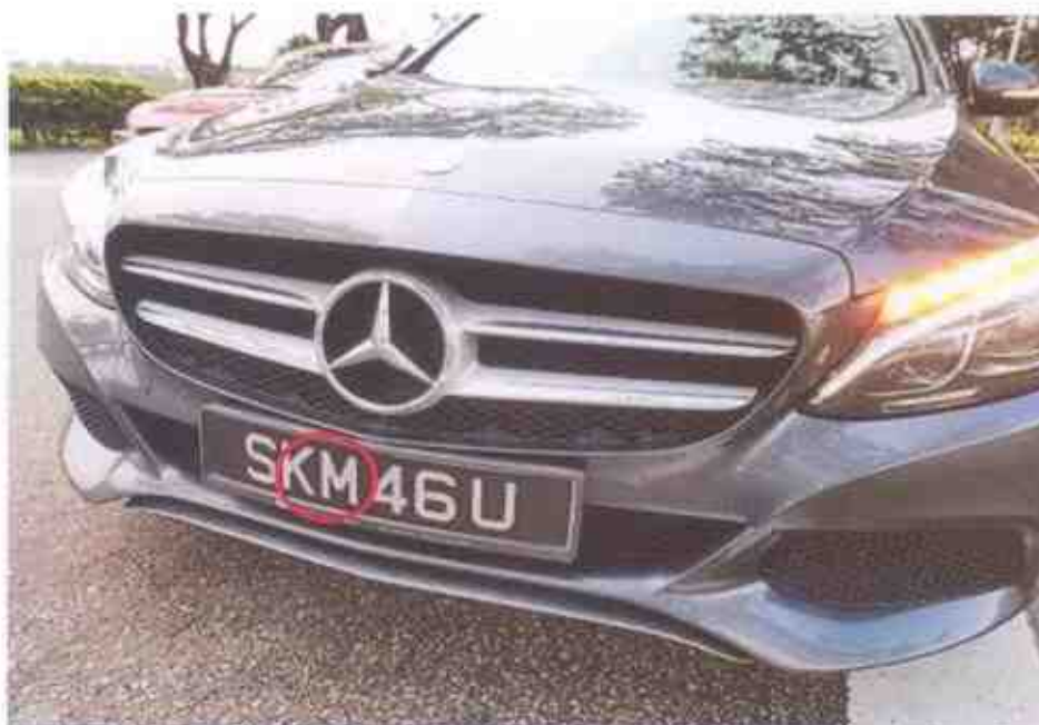
Photo 15 shows the position of the Mercedes after the accident. Upon closer examination of the accident photograph, we observed the same black marks on several alpha- numeric letterings of the front number plate of the Mercedes as per our physical inspection (circled).
