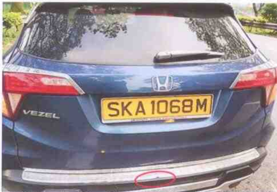
Photo 14 shows the position of the Honda after the accident. Closer examination of the accident photograph shows the damaged rear bumper scuff plate as well as the rear bumper of the Honda (circled).
