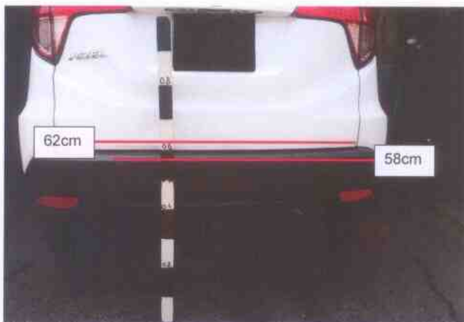
Photo 16 shows the height measurement being conducted on the rear portion of the Honda (using a similar make and model). The height above ground level of the top portion of the rear bumper where the damages were found was measured to be approximately 58cm. The height above ground level of the lower part of the boot lid where the dent was found was measured to be approximately 62cm.
