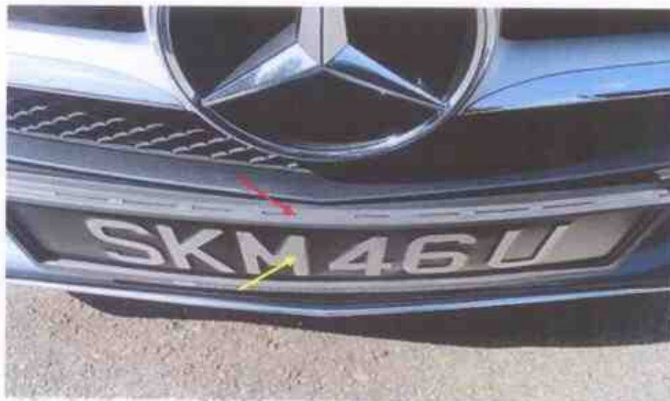
Photo 9 shows upon closer examination of the front number plate of the Mercedes, we observed cracks on the top centre portion of the front number plate frame (red arrow). There were also several black marks on the alpha- numeric letterings of the front number plate of the Mercedes (yellow arrow).
