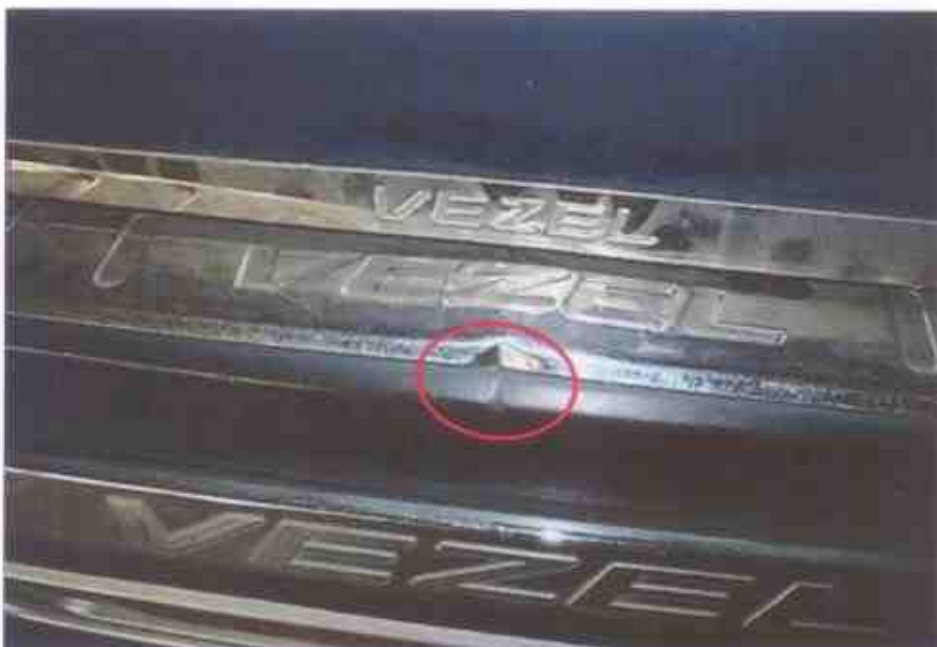
Photo 2 shows a close up view of the rear bumper of the Honda at the time of the Pre-Repair Survey conducted by LKK Auto Consultants Pte. Ltd. taken 5 months after the accident. We observed that the rear bumper scuff plate as well as the rear bumper were buckled at the centre portion (circled).
