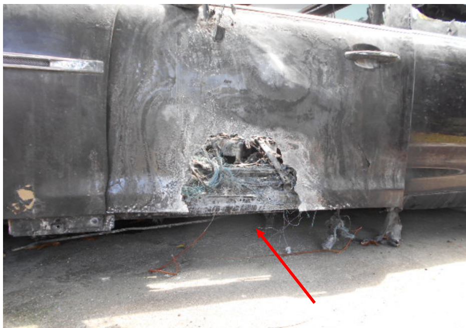
Photo 9 shows the left centre of the Insured Vehicle, at its left front door area. The DPF is located at the underside centre of the Insured Vehicle (arrowed).
