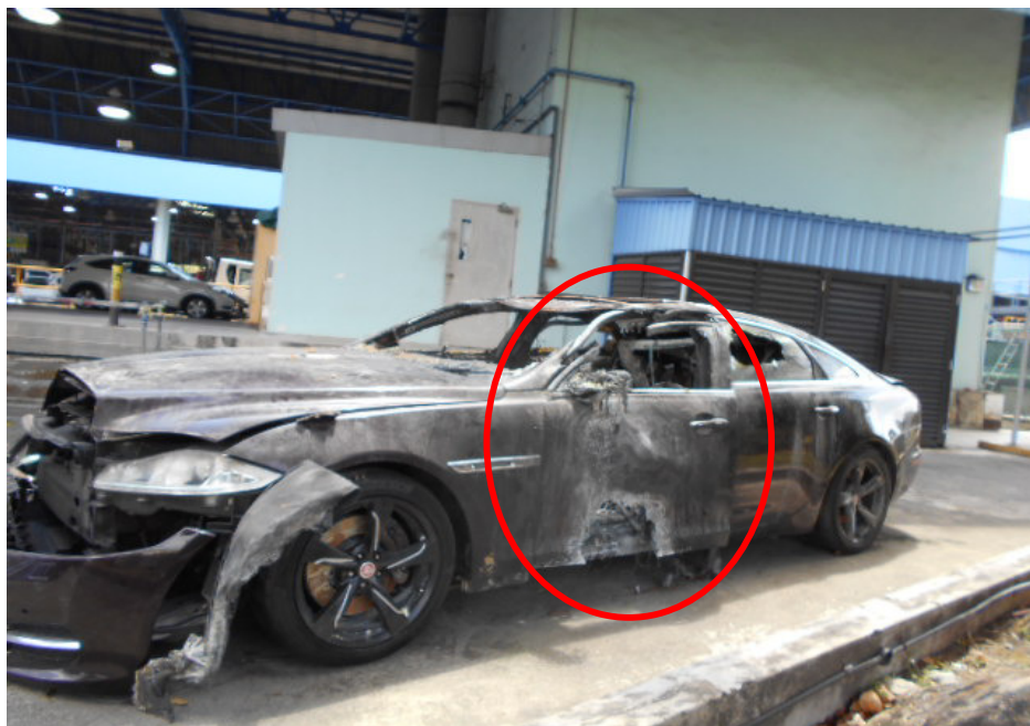
Photo 3 shows a general view of the left side of the Insured Vehicle at the time of my inspection. From the burn pattern, the fire appears to have been most intense at the centre portion (circled) of the Insured Vehicle. This follows the severe fire damage that was observed within the interior compartment of the Insured Vehicle.
