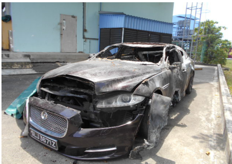
Photo 2 shows a general view of the front portion of the Insured Vehicle at the time of my inspection. The Insured Vehicle was observed to have sustained severe fire damage at its centre portion. Its front portion had sustained minor fire damage that was mainly due to heat from the fire.
