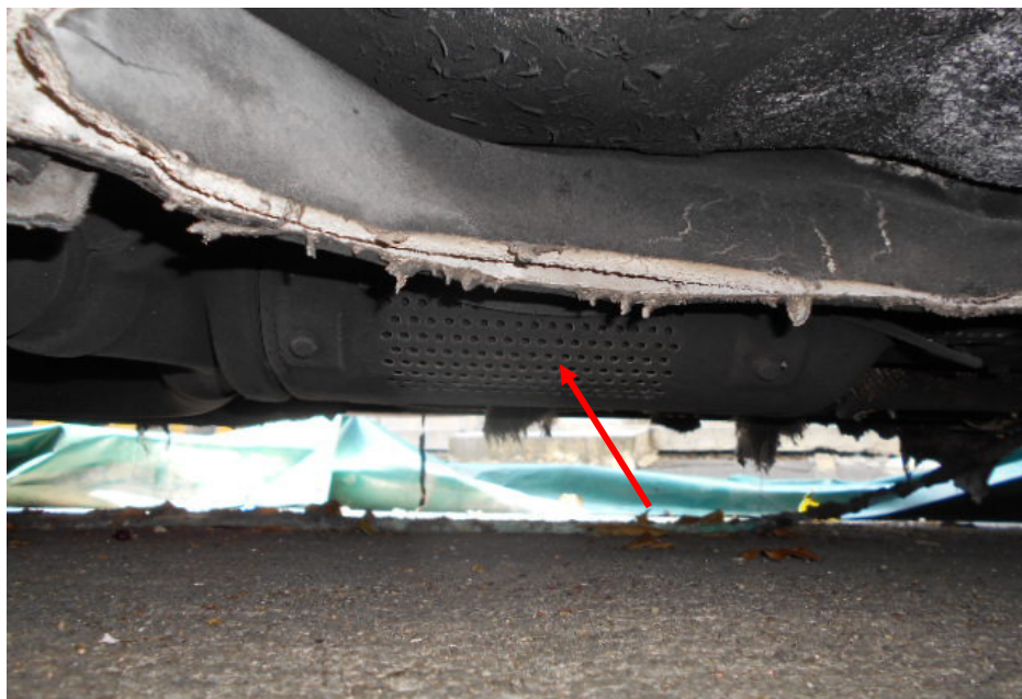
Photo 10 shows the DPF (arrowed) of the Insured Vehicle. The DPF is located at the underside centre of the Insured Vehicle. From my observations, the DPF of the Insured Vehicle was blackened, indicating exposure to the fire/extreme heat.
