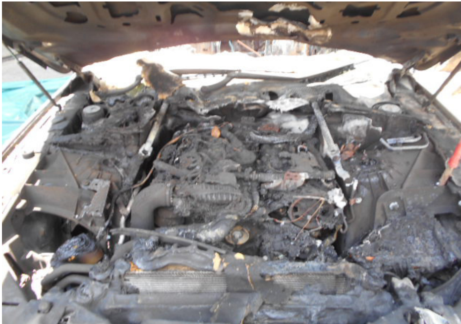
Photo 5 shows a general view of the engine compartment of the Insured Vehicle. Although the parts within the engine compartment were also affected by the fire, the extent of burn damage was less severe as compared to the parts within the interior compartment.
