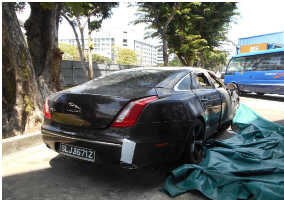
Photo 1 shows a general view of the rear portion of the Insured Vehicle at the time of my inspection. The Insured Vehicle was observed to have sustained severe fire damage at its centre portion. Its rear portion had sustained minor fire damage that was mainly due to heat from the fire.
