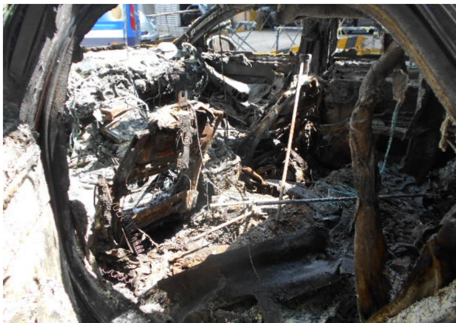
Photo 4 shows a general view of the interior compartment of the Insured Vehicle, which was affected the most by the fire. Almost all the parts within the interior compartment were severely burnt and/or melted.
