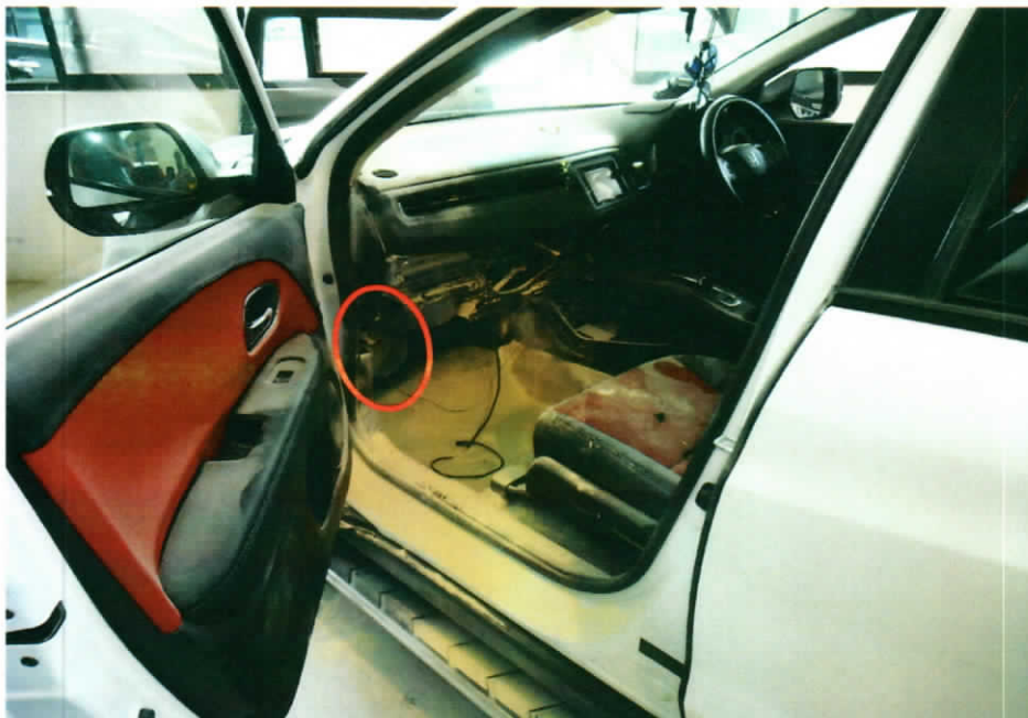
Photo 2 shows a general view of the interior compartment of the Insured Vehicle at the time of inspection. I had observed slight fire/smoke damage that was confined to a single area of the Insured Vehicle. This was at the front left side of its interior compartment, near the glove compartment at the left side of the front dashboard (circled).
