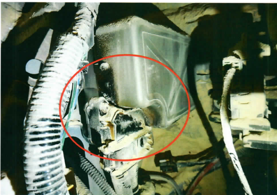
Photo 11 shows a closer view of the partially burnt component (circled), which the slightly burnt/melted wire connector connects into. This physical evidence at the area where the smoke had originated would appear to indicate that the cause of the smoke incident to the Insured Vehicle was due to electrical in nature that involved the partially burnt component.
