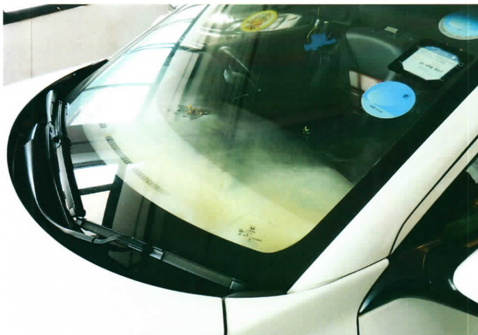
Photo 5 shows the blackened front windscreen of the Insured Vehicle as a result of the incident. Apart from this blackened front windscreen, the exterior of the Insured Vehicle was unaffected by the fire.
