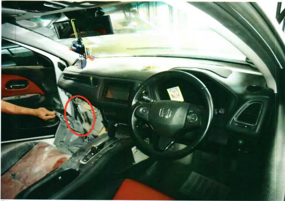
Photo 3 shows a general view of the interior compartment of the Insured Vehicle at the time of inspection. I had observed slight fire/smoke damage that was confined to a single area of the Insured Vehicle. This was at the front left side of its interior compartment, near the glove compartment at the left side of the front dashboard (circled).
