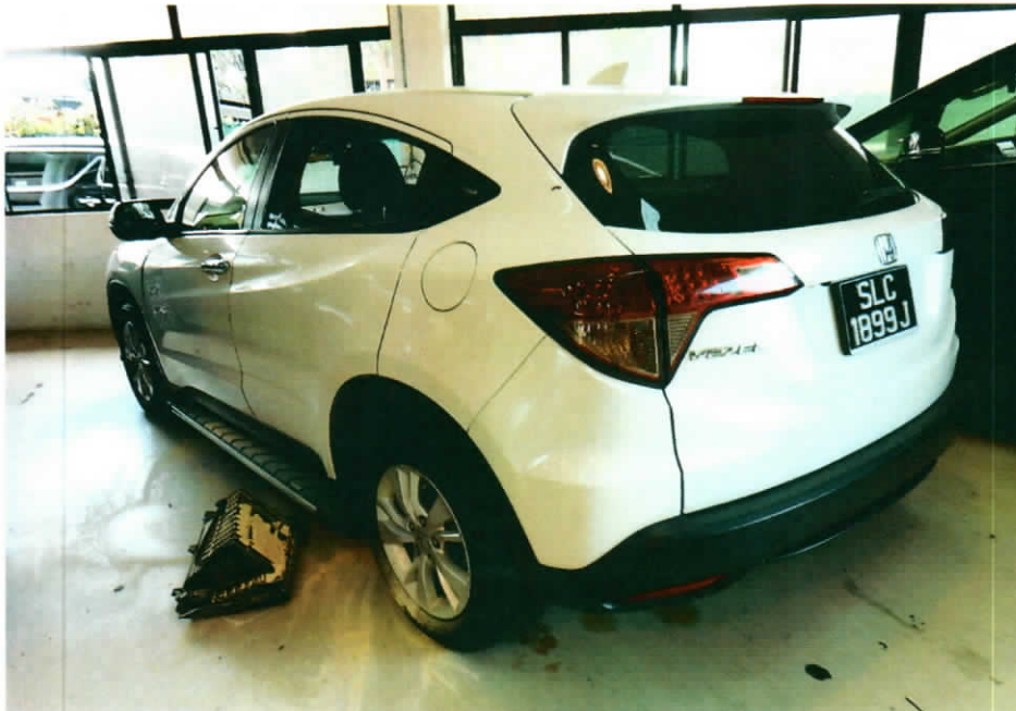
Photo 1 shows a general view of the rear left body of the Insured Vehicle at the time of my inspection. The exterior body of the Insured Vehicle was observed to be in good general condition with no damage of fire/smoke nature found apart from a blackened front windscreen.
