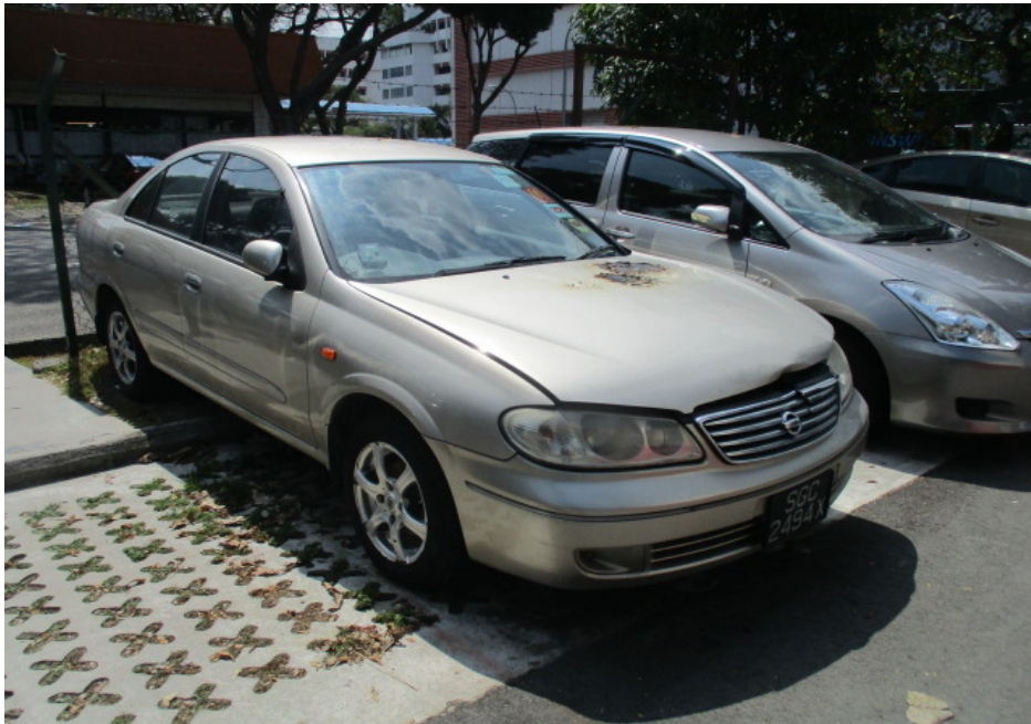
Photo 3 shows the general view of the front right portion of the Insured Vehicle at the time of our inspection. The fire damage to the Insured Vehicle was confined to its front portion. Its front bonnet and front right headlamp were amongst the body parts that were found to have been affected as a result of the fire.
