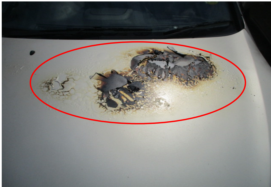
Photo 6 shows the burn pattern and paint bubbles on the left portion of the front bonnet of the Insured Vehicle (circled). Such burn marks are a result of exposure to prolonged heat intensity, which may indicate where the fire had started. Rust would also begin to develop on these areas soon after the fire.
