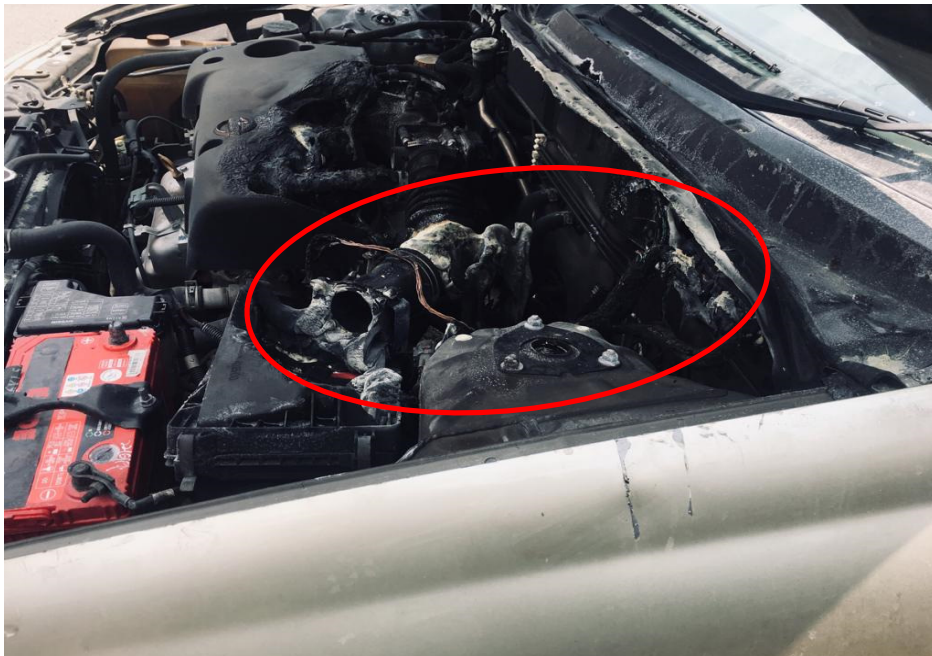
Photo 16 shows a close up view of the engine compartment of the Insured Vehicle at the incident scene after the fire was extinguished. In general, the information that could be gathered from this photograph had corresponded to the events that were related to us by Mr Tan. The extent of fire damage observed indicates that the fire had started from the left rear portion of the engine compartment (circled).
