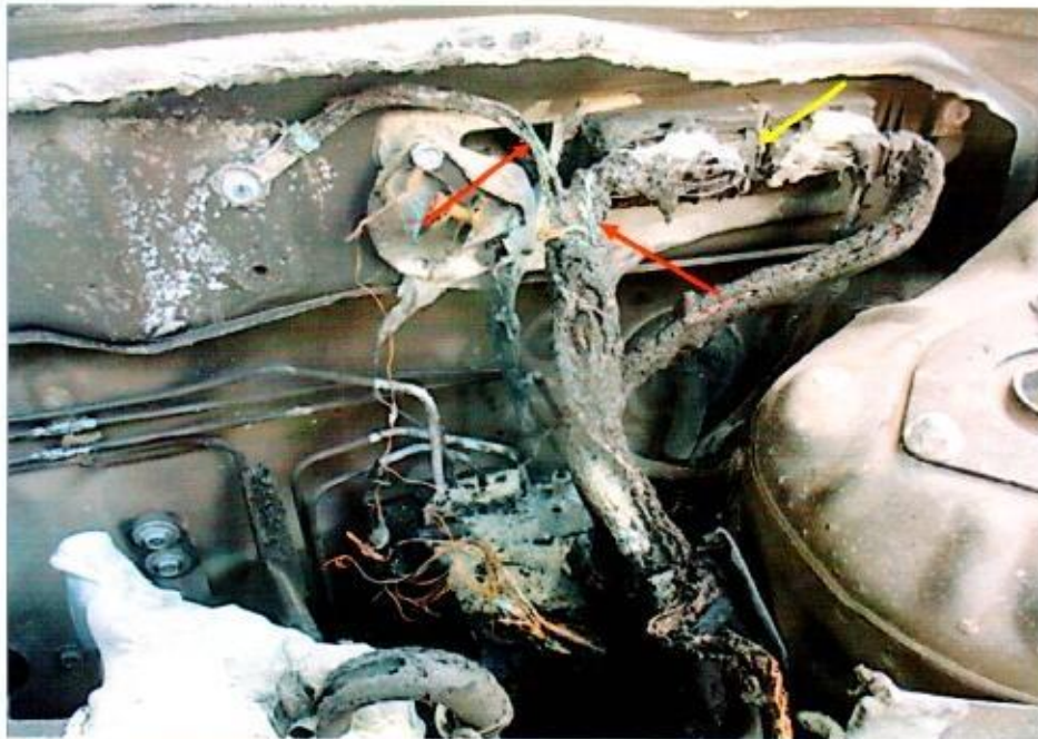
Photo 10 shows a closer view of the wirings with greenish residue (red arrows) leading to the Engine Control Module (ECM) (yellow arrow). The presence of such greenish residue suggest occurrence of an electrical short circuit.
