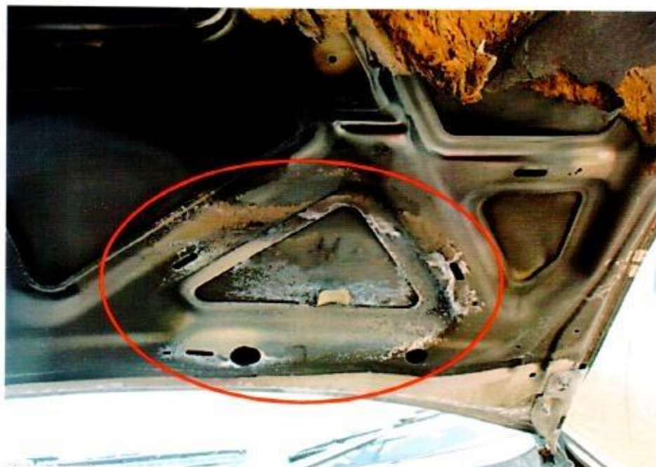
Photo 8 shows the rust that had developed on the underside of the front bonnet, around the left rear area (circled). The development of rust is an indication that the area was exposed to prolonged exposure to high heat intensity, which had caused the steel/metal material of the front bonnet to be exposed to natural environmental condition. Hence the fire to the Insured Vehicle can be determined to have originated towards the left rear portion of the engine compartment.
