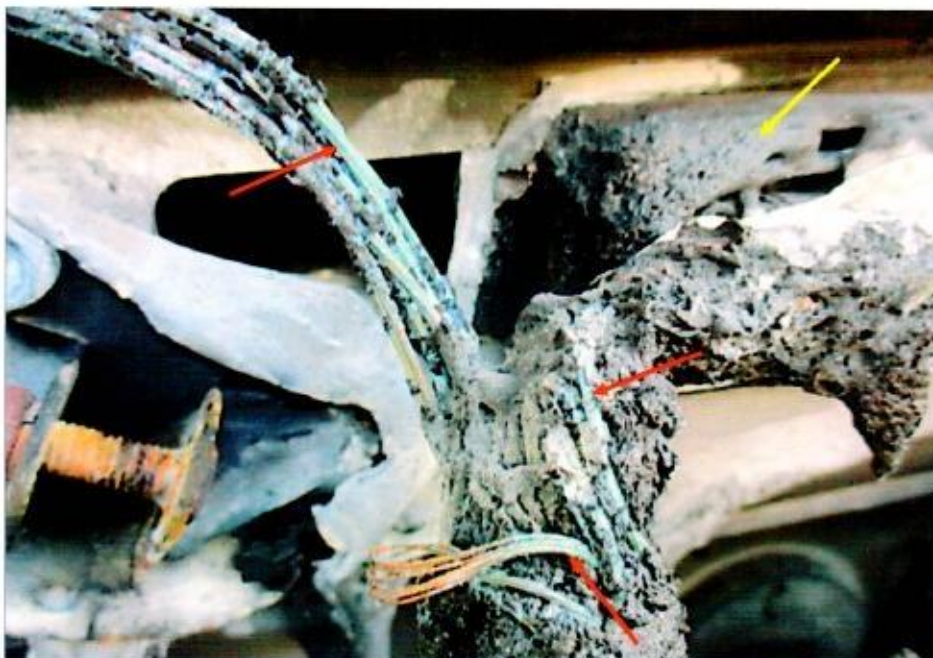
Photo 11 shows a close up view of the wirings with greenish residue (red arrows) leading to the Engine Control Module (ECM) (yellow arrow). The presence of such greenish residue suggest occurrence of an electrical short circuit.
