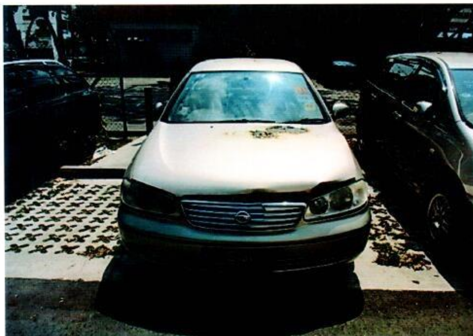
Photo 1 shows the general view of the front portion of the Insured Vehicle at the time of our inspection. The fire damage to the Insured Vehicle was confined to its front portion. Its front bonnet, front grille and front headlamps were amongst the body parts that were found to have been affected as a result of the fire.
