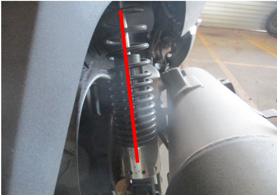
Photo 18 shows the right shock absorber of the motorcycle was found to be intact without any misalignment.
