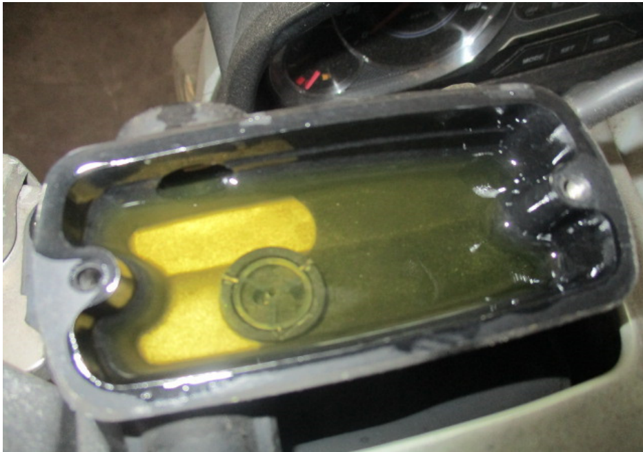
Photo 26 shows a close up view of the brake fluid reservoir for the rear brake of the Motorcycle. The brake fluid was observed to be of sufficient level and without contamination for operational purposes.
