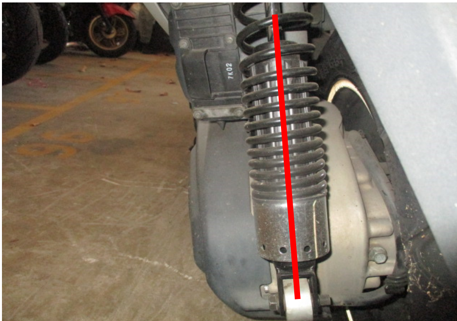
Photo 17 shows the left shock absorber of the motorcycle was found to be intact without any misalignment.
