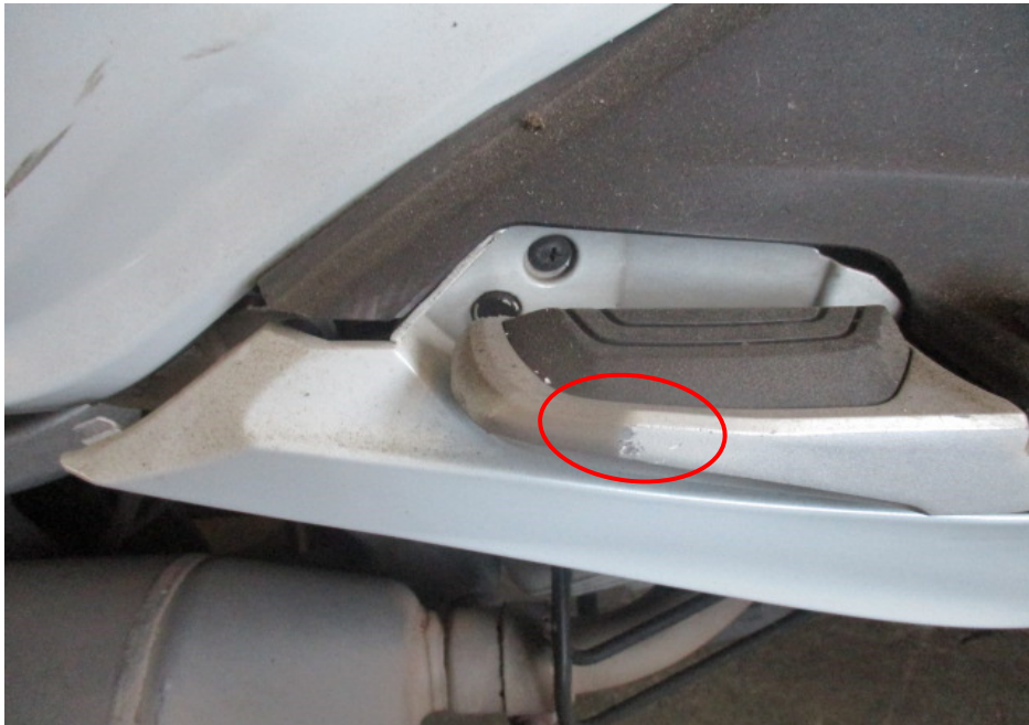
Photo 11 shows a closer view of the damaged right pillion footrest (circled) of the Motorcycle at the time of our inspection.
