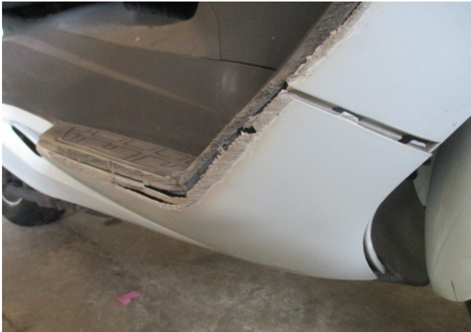
Photo 5 shows a closer view of the right bottom cowling of the Motorcycle which was observed to be damaged due to the accident.
