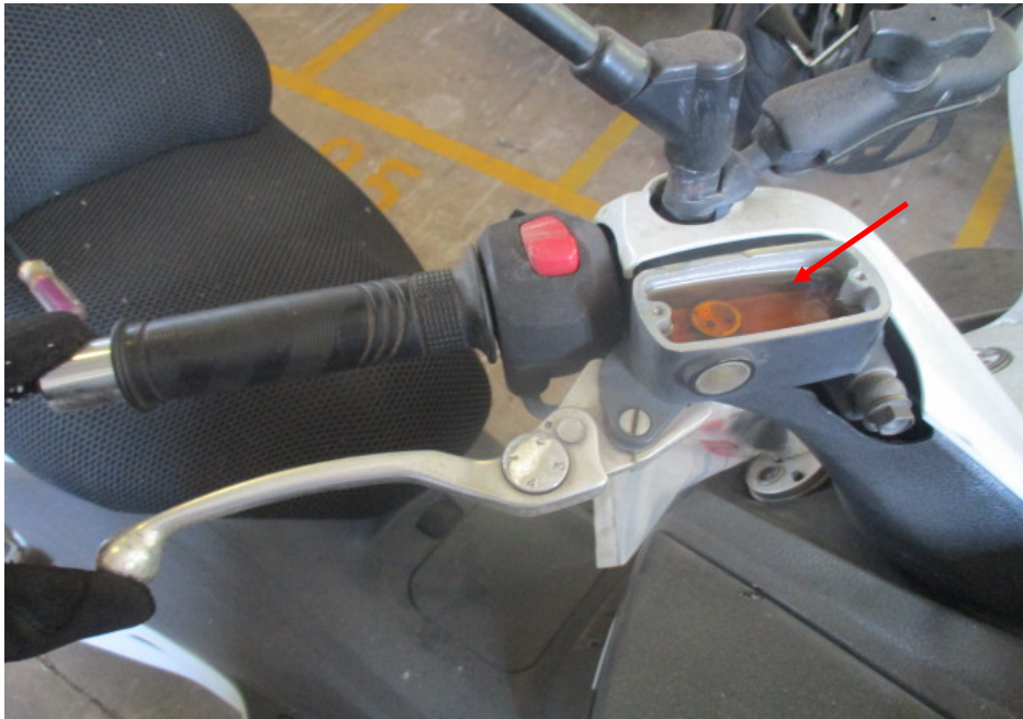
Photo 24 shows the brake fluid reservoir for the front brake of the Motorcycle. The brake fluid was observed to be of sufficient level and without contamination for operational purposes (arrowed).
