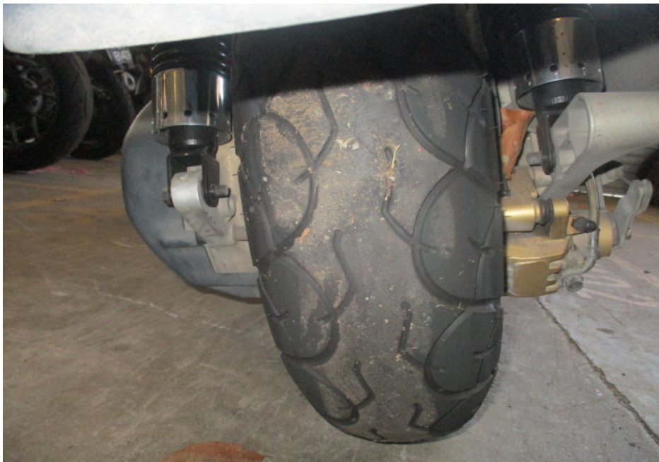
Photo 14 shows the condition of the Motorcycle's rear tyre. The rear tyre was observed to be in serviceable condition with remaining tread depth of approximately 3mm. The tyre was also observed to be sufficiently inflated for vehicular operation. We did not observe any tear, burst mark(s) and/or punctured hole(s) on the sidewalls as well as across the tread of the rear tyre.
