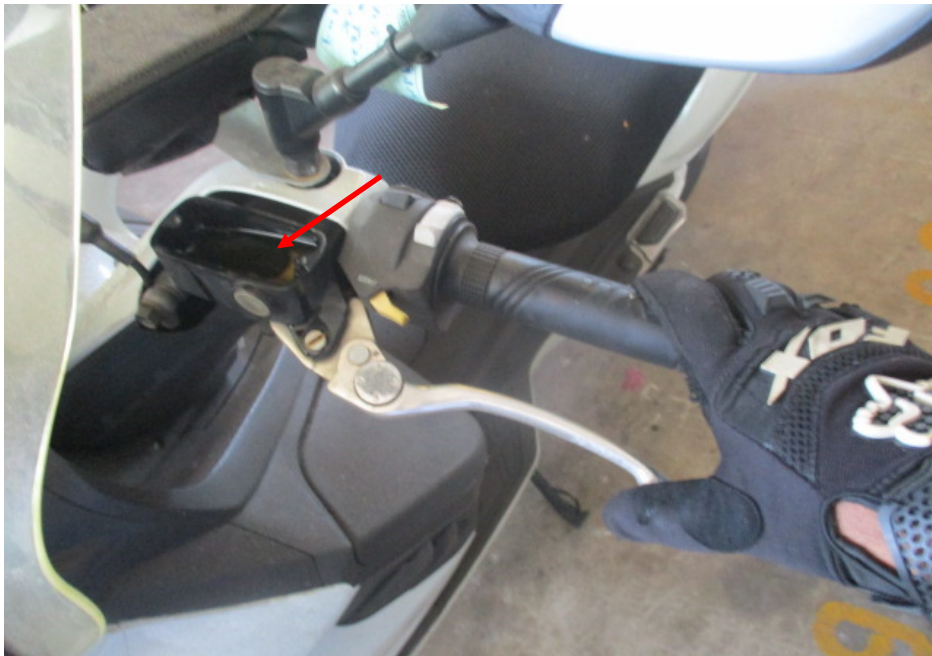
Photo 25 shows the brake fluid reservoir for the rear brake of the Motorcycle. The brake fluid was observed to be of sufficient level and without contamination for operational purposes (arrowed).
