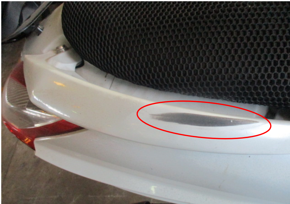
Photo 8 shows the damaged right pillion grab rail of the Motorcycle. The damage sustained was mainly of grazing nature (circled).
