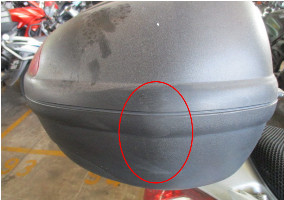
Photo 10 shows a closer view of the top box of the Motorcycle which was observed to have sustained scratches due to the accident (circled).
