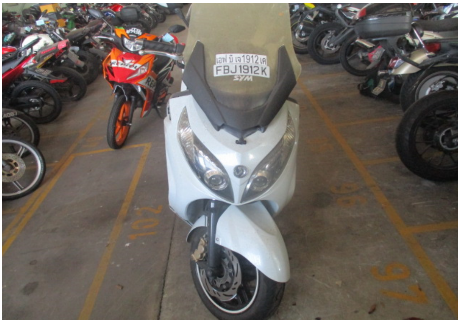
Photo 21 shows the front wheel of the Motorcycle turned towards its full left. Turning the Motorcycle's handle bar towards the left and right did not produce any abnormal free play and/or resistance. This would indicate that the steering system of the Motorcycle was in serviceable condition at the time of our inspection.
