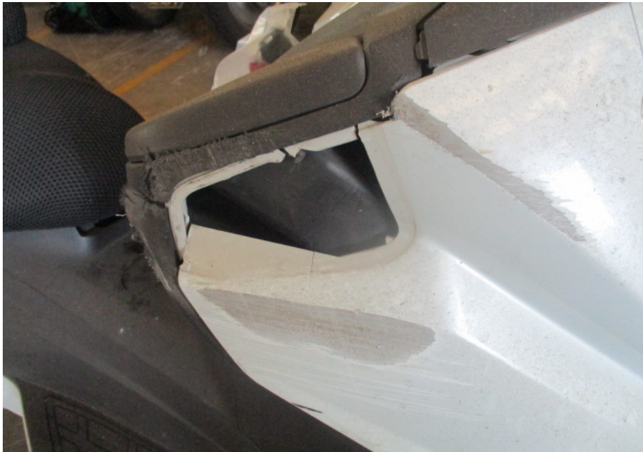
Photo 3 shows a closer view of the right cowling which was amongst the body parts at the front body of the Motorcycle that had sustained damage as a result of the accident.
