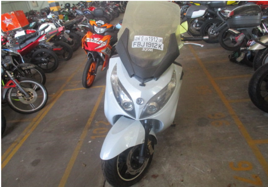
Photo 20 shows the front wheel of the Motorcycle turned towards its full right. Turning the Motorcycle's handle bar towards the left and right did not produce any abnormal free play and/or resistance. This would indicate that the steering system of the Motorcycle was in serviceable condition at the time of our inspection.
