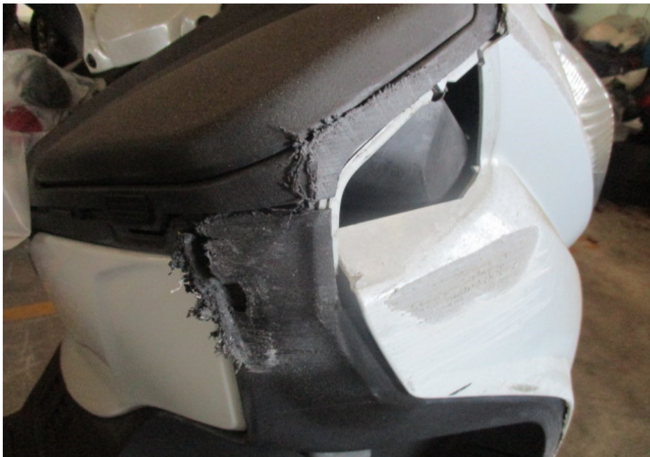
Photo 4 shows a closer view of the right inner cowling which was amongst the body parts at the front body of the Motorcycle that had sustained damage as a result of the accident.
