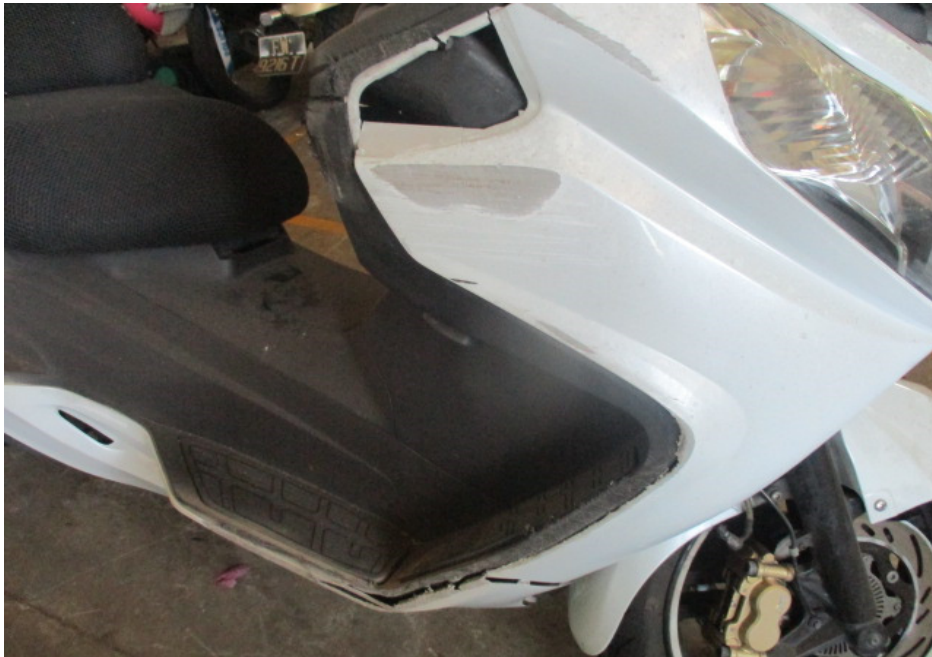
Photo 7 shows a close-up view of the right front portion of the Motorcycle at the time of our inspection. The right cowling sustained damages of grazing nature due to the accident.
