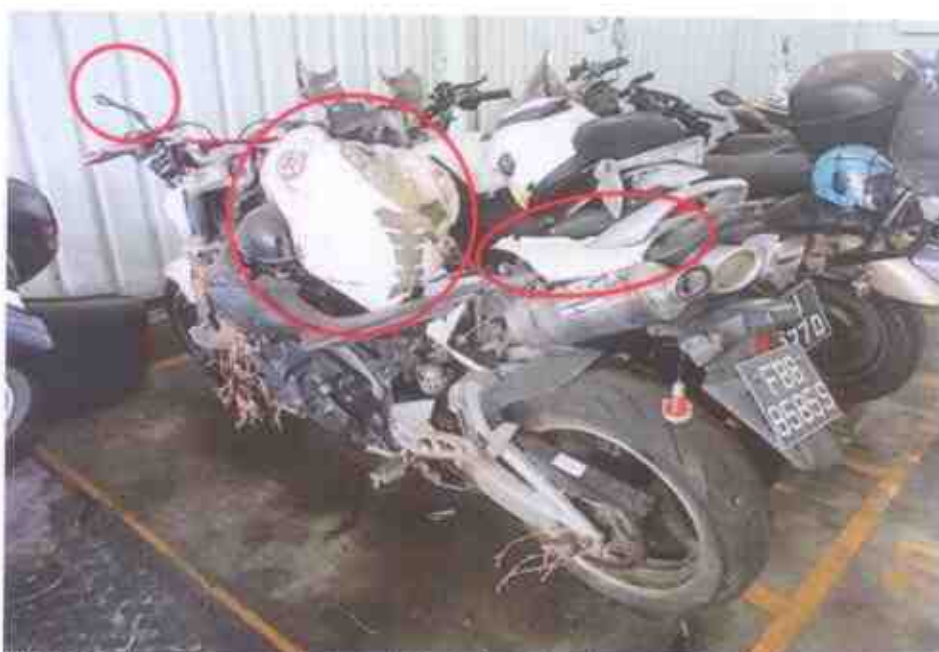
Photo 2 shows a general view of the left body of the Motorcycle at the time of our inspection. Body parts that were found to have been damaged include its left side mirror, fuel tank and left rear side cover (circled).
