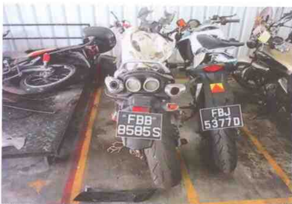
Photo 1 shows a general view of the rear body of the Motorcycle at the time of our inspection. The Motorcycle had sustained damages all around, significantly at its front portion and left body. The mileage of the Motorcycle was not recorded at the time of our inspection due to the damage sustained to the odometer display screen as a result of the accident.
