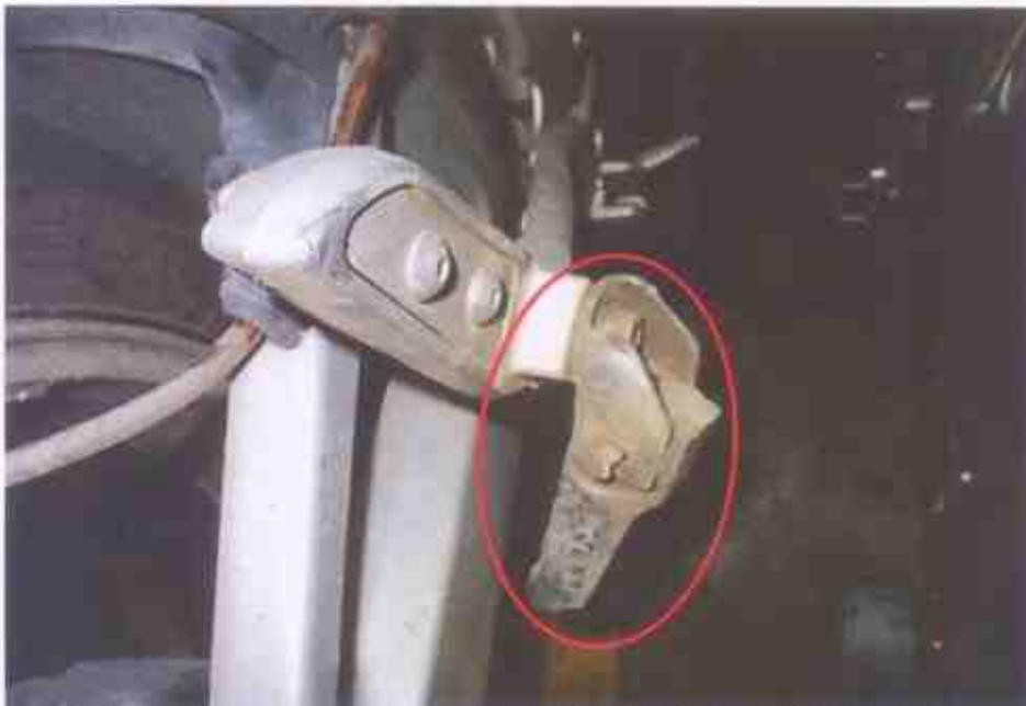
Photo 10 shows the damaged right rear footrest (circled) of the Motorcycle.
