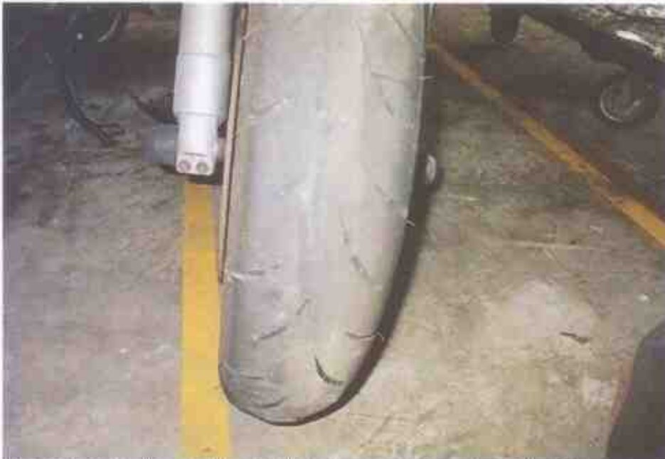
Photo 9 shows the condition of the Motorcycle's front tyre. The front tyre was observed to be in serviceable condition with remaining tread depth of approximately 3mm. The tyre was also observed to be sufficiently inflated for vehicular operation. We did not observe any tear, burst mark(s) and/or punctured hole(s) on the sidewalls as well as across the tread of the front tyre.
