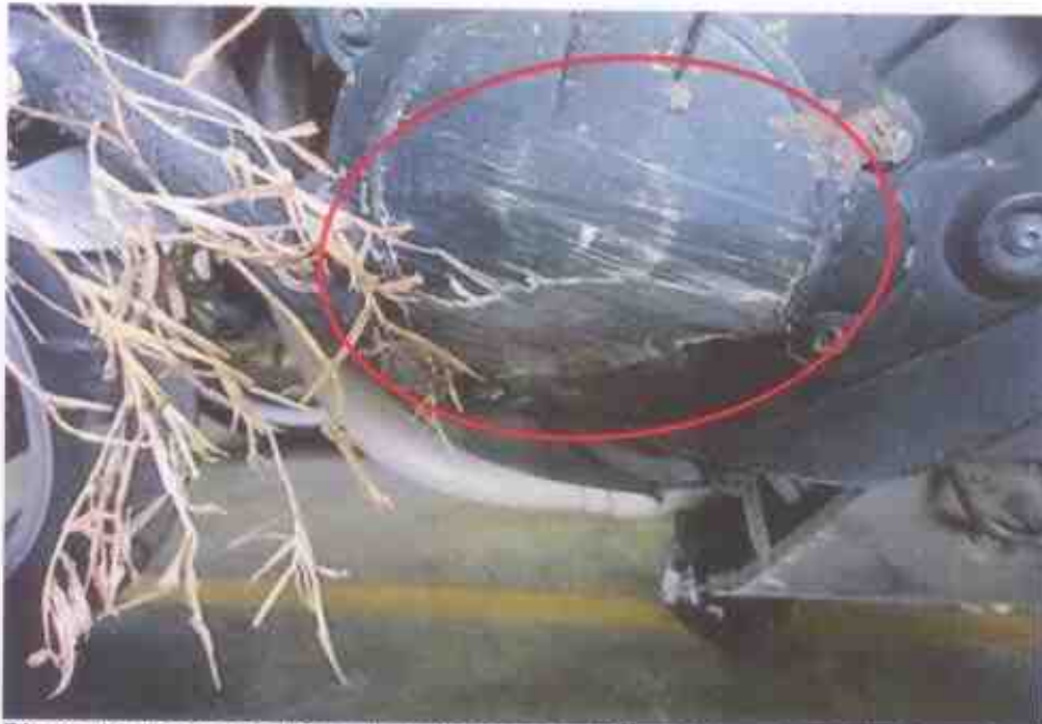
Photo 14 shows the left side of the engine of the Motorcycle at the time of our inspection. The various left engine components had sustained damage of grazing nature as a result of the accident (circled) however the engine components were still intact. There was also no fluid leak and/or fluid stain found around the left engine area of the Motorcycle.
