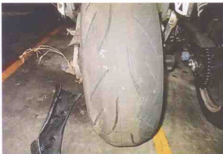
Photo 12 shows the condition of the Motorcycle's rear tyre. The rear tyre was observed to be in serviceable condition with remaining tread depth of approximately 4mm. The tyre was also observed to be sufficiently inflated for vehicular operation. We did not observe any tear, burst mark(s) and/or punctured hole(s) on the sidewalls as well as across the tread of the rear tyre.
