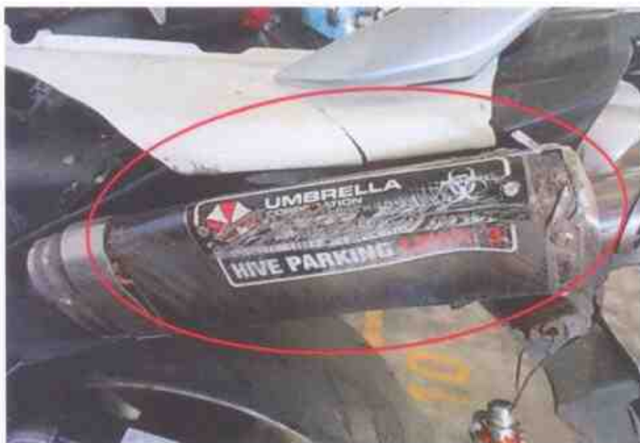
Photo 11 shows the damaged left rear side cover and left exhaust muffler (circled) of the Motorcycle as a result of the accident.
