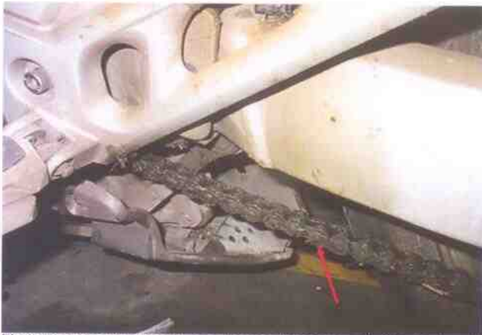
Photo 16 shows the closer view of the gear chain (arrowed) of the Motorcycle, which was observed to be intact with no misalignment. It was also adequately lubricated for operating purposes.
