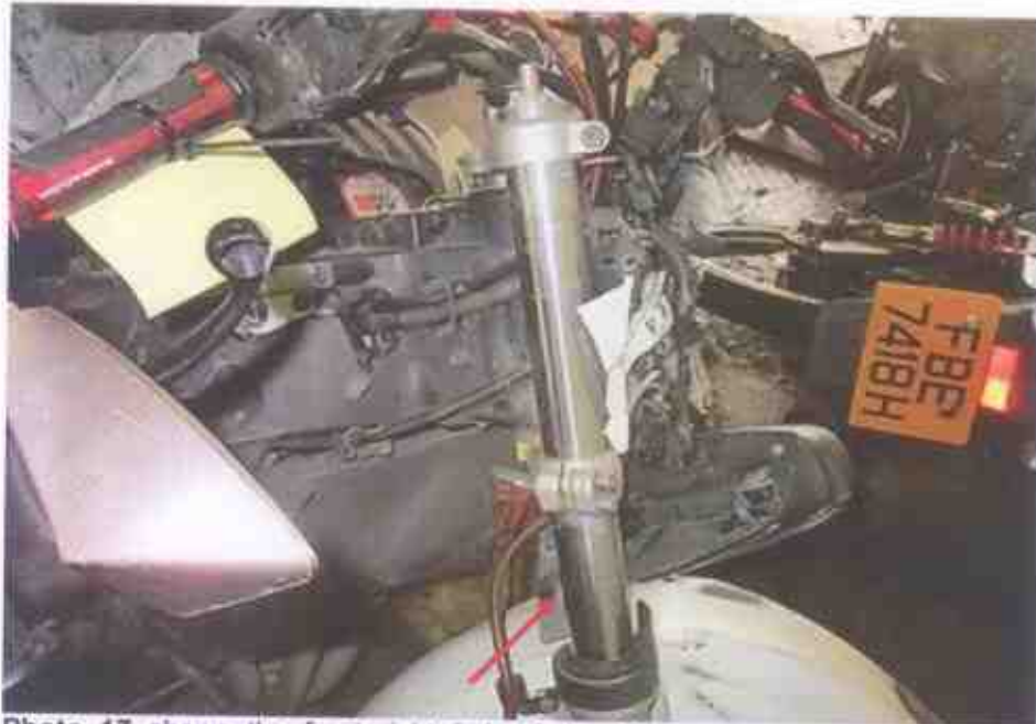
Photo 17 shows the front right fork of the Motorcycle. The front right fork (arrowed) was observed to be bent inwards as a result of the accident. We were hence not able to conduct any tests on the steering system of the Motorcycle.
