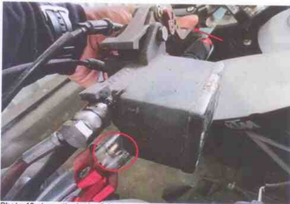
Photo 19 shows the brake fluid reservoir for the front brake of the Motorcycle. A leakage of brake fluid from the front brake fluid reservoir was observed (circled) when the front brake lever was depressed (arrowed).
