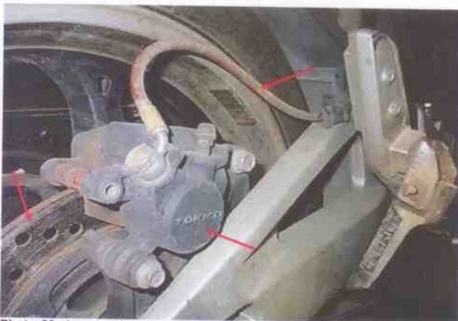
Photo 20 shows a close up view of the rear brake caliper, rear brake disc and rear brake hose (arrowed) of the Motorcycle, which are all part of the components in the hydraulic rear brake system of the Motorcycle. Our visual checks of these various components revealed all to be intact with no visible damage. No leakage of brake fluid was also observed.
