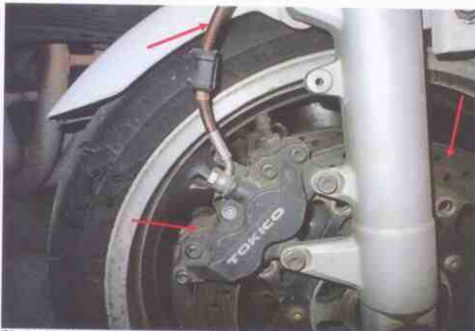
Photo 18 shows a close up view of the front brake caliper, front brake disc and front brake hose (arrowed) of the Motorcycle, which are all part of the components in the hydraulic front brake system of the Motorcycle. Our visual checks of these various components had revealed all to be intact with no visible damage. No leakage of brake fluid was also observed.
