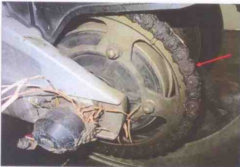
Photo 15 shows the gear chain (arrowed) of the Motorcycle, which was observed to be intact with no misalignment. It was also adequately lubricated for operating purposes. The gear chain rotates the rear wheel of the Motorcycle.
