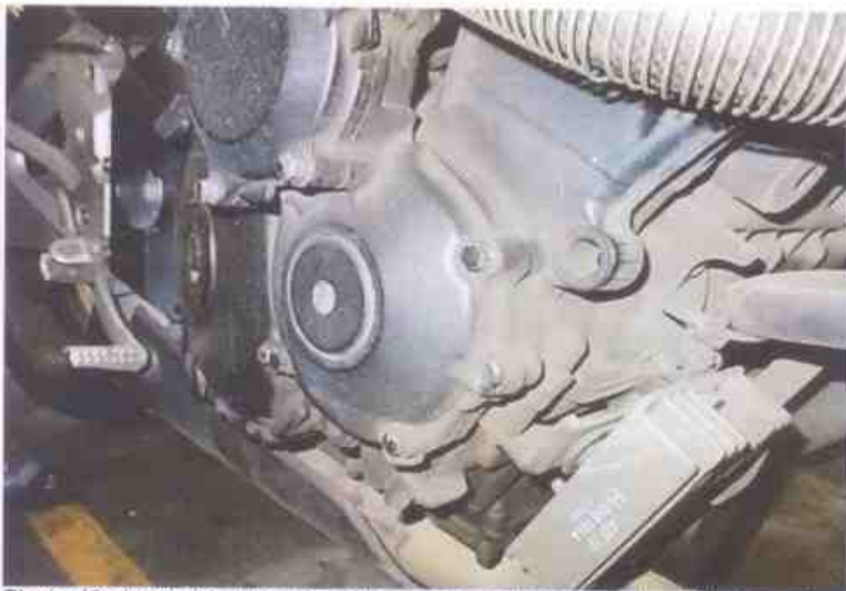
Photo 13 shows the right side of the engine of the Motorcycle at the time of our inspection. The various engine related parts and components were found to be intact with no visible damage. There was also no sign(s) or indication(s) of fluid leak observed around the right engine area of the Motorcycle.
