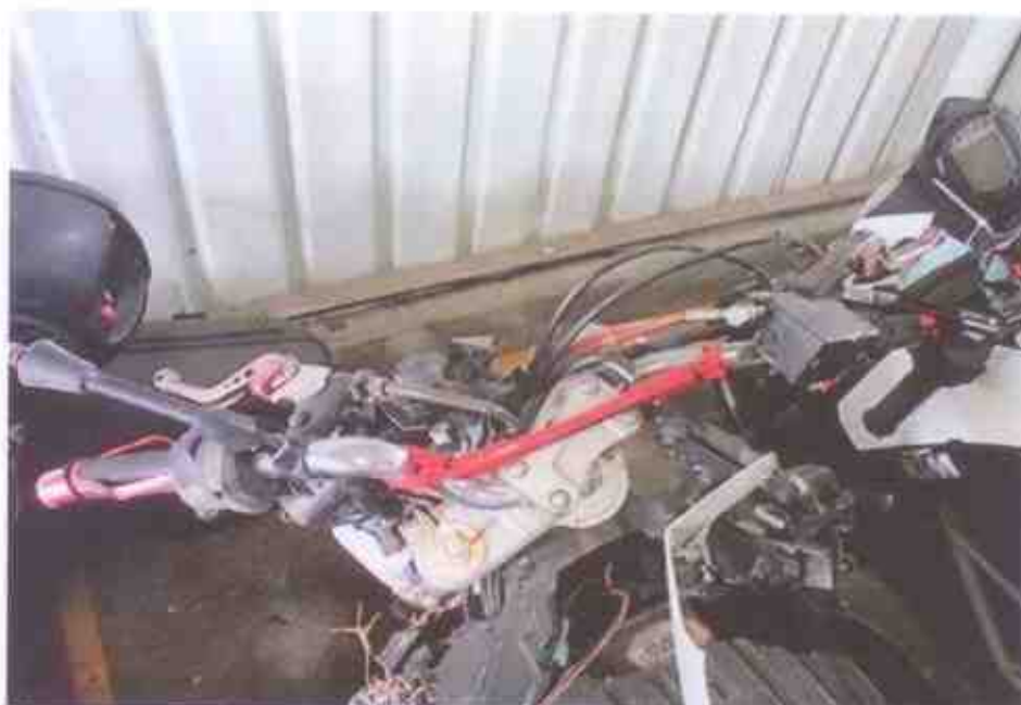
Photo 6 shows a close up view of the front brake lever, front brake fluid reservoir, left side mirror, clutch lever, left handlebar grip and left handlebar end of the Motorcycle. These parts were amongst the body parts of the Motorcycle which were damaged as a result of the accident.
