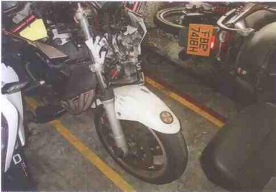
Photo 3 shows a general view of the right front body of the Motorcycle at the time of our inspection. Body parts that were found to have been damaged include its headlamp assembly, speedometer, front mudguard, left side mirror, clutch lever, right side mirror, front brake lever, front brake fluid reservoir, petrol tank, rear right footrest, left exhaust muffler and left rear side cover amongst others.
