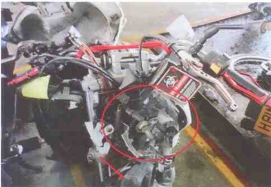
Photo 4 shows a closer view of the headlamp assembly (circled) and speedometer (arrowed) which were amongst the body parts at the front body of the Motorcycle that had sustained damage as a result of the accident.
