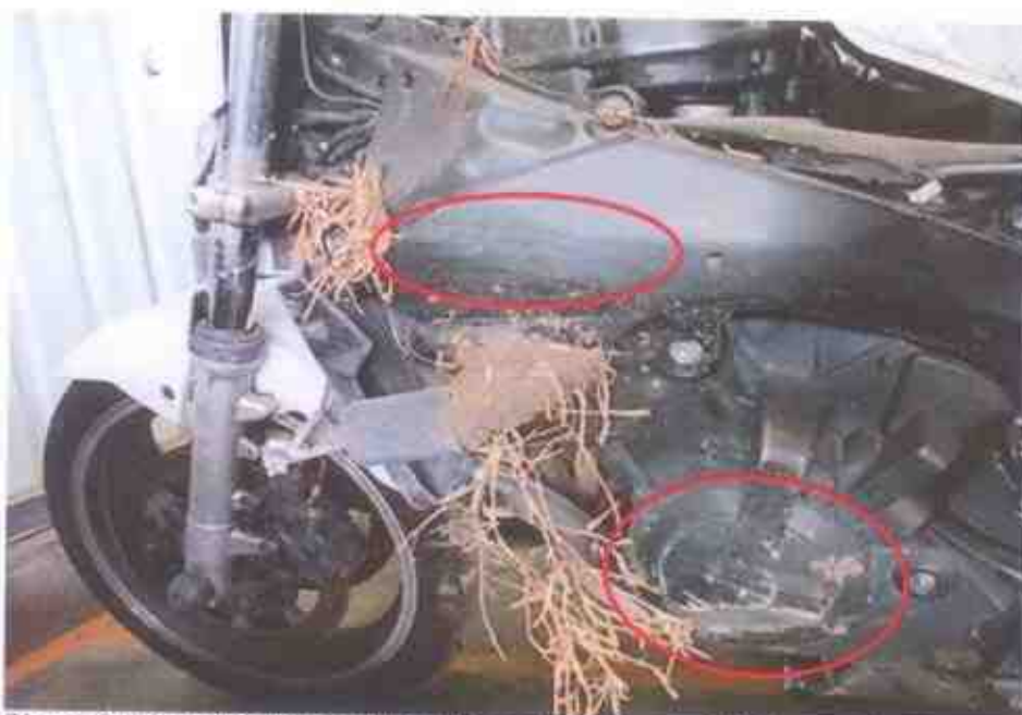
Photo 8 shows the damaged left side engine cover and left frame (circled) of the Motorcycle. The damage sustained at the left frame of the Motorcycle was mainly of grazing nature.
