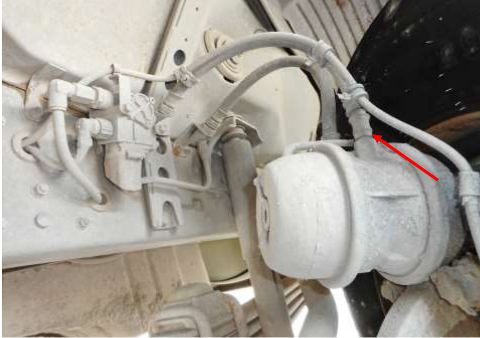
Photo 18 shows the brake pipe (arrowed) at the front right wheel of the Motor Lorry. I did not observe any leakage of brake fluid at the time of my inspection of the Motor Lorry. My static tests of the Motor Lorry's braking system, along with my visual examination of the various mechanical components in the braking system, had indicated that there was no internal leakage of pressure/vacuum. Hence the braking system of the Motor Lorry was likely to be in serviceable condition at the material time of accident.
