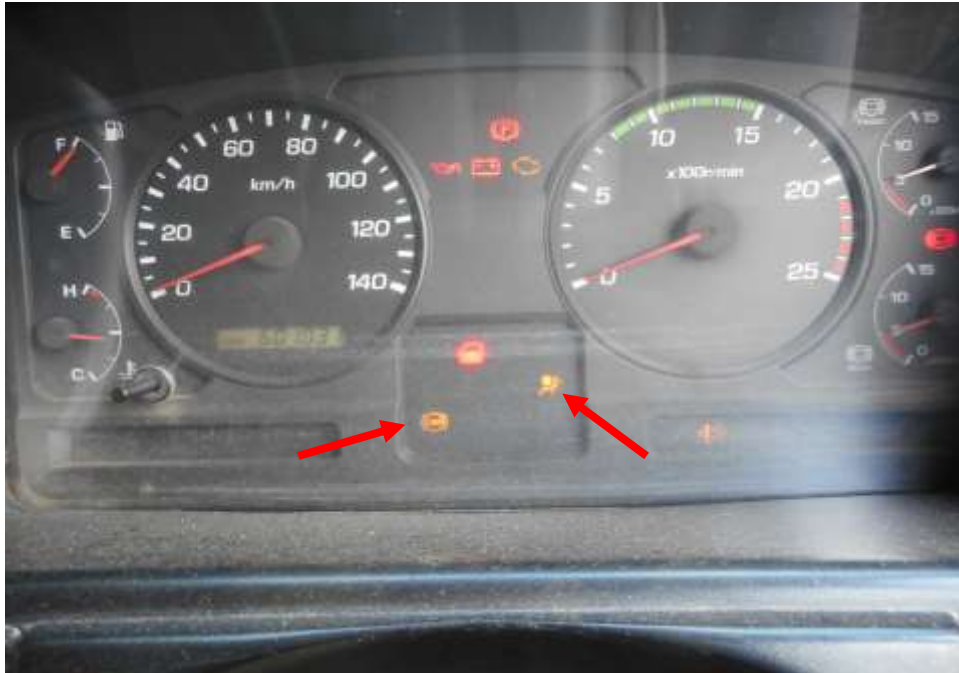
Photo 25 shows the warning light for Anti-Lock Brake System (ABS) and Safety Restraint System (SRS) (arrowed) appearing on the instrument panel of the Motor Lorry during the self-test of its various electronic operating systems when its engine was cranked.
