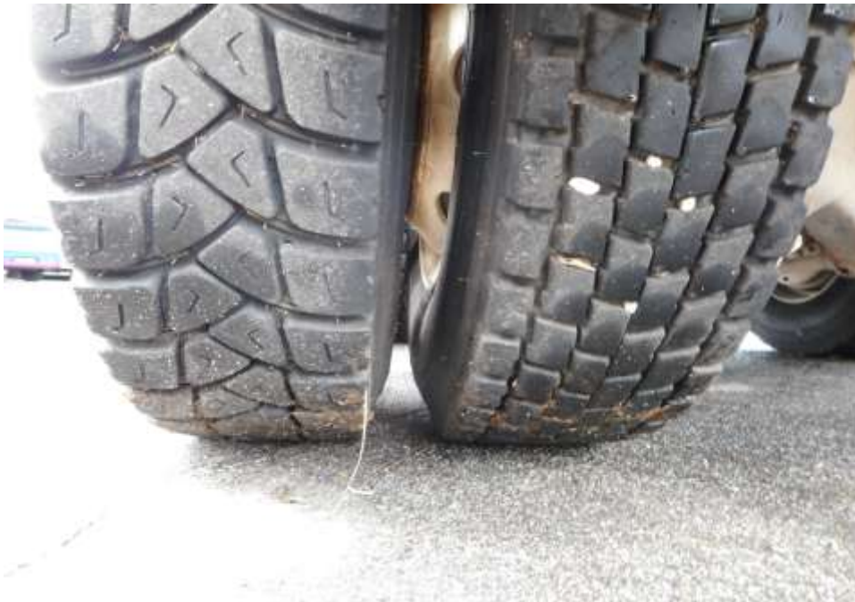
Photo 9 shows the condition of the rear left tyres of the Motor Lorry, which was observed to be in serviceable condition with remaining tread depth of approximately 9.1mm. The tyres, which were wrapped around standard steel wheel rim, were also observed to be sufficiently inflated for vehicular operation. There was also no damage found on all 6 steel wheel rims of the Motor Lorry.
