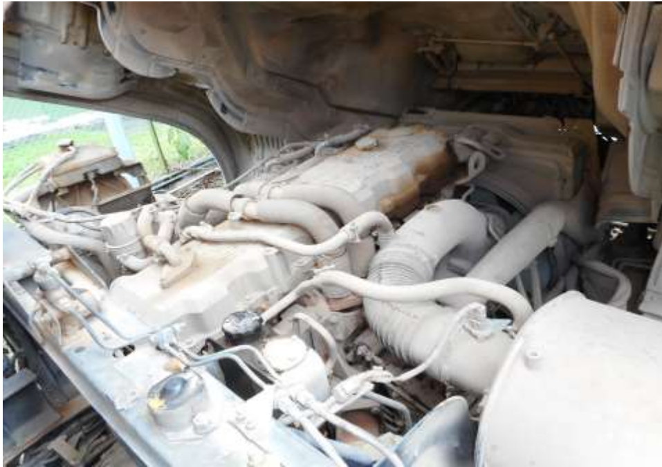
Photo 11 shows a general view of the Motor Lorry's engine compartment, which was accessed by lifting the front cabin of the Motor Lorry. The various parts and components inside the engine compartment were unaffected by the accident. There was also no sign(s) or indication(s) of fresh fluid leakage and/or fluid stain within the engine compartment (photograph shows the engine compartment as viewed from the right front side of the Motor Lorry).
