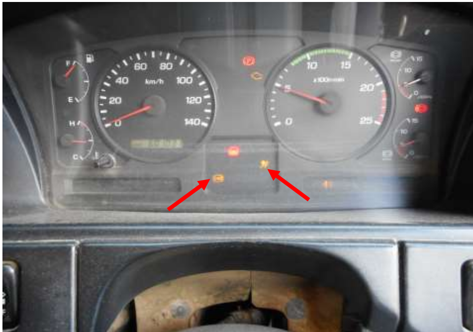
Photo 26 shows the warning lights for Anti-Lock Brake System (ABS) and Safety Restraint System (SRS) (arrowed) stayed illuminated on the instrument panel of the Motor Lorry after the engine was cranked.
