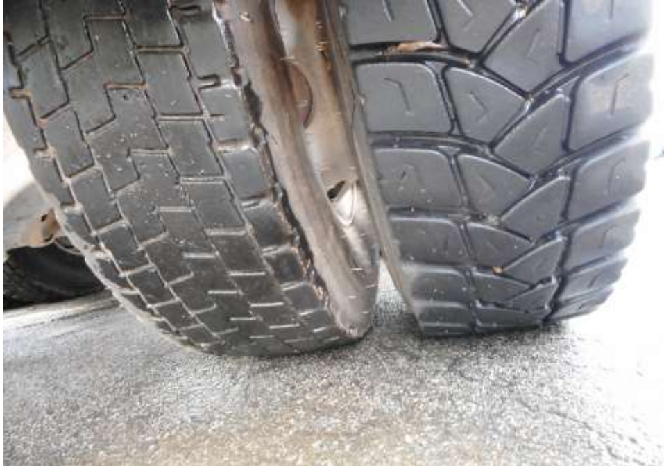
Photo 8 shows the condition of the rear right tyre of the Motor Lorry, which was observed to be in serviceable condition with remaining tread depth of approximately 8.7mm. The tyre, which was wrapped around standard steel wheel rim, was also observed to be sufficiently inflated for vehicular operation.
