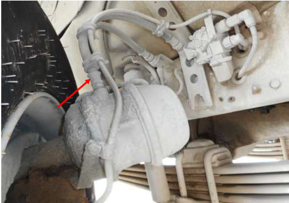
Photo 19 shows the brake pipe (arrowed) at the front left wheel of the Motor Lorry. I did not observe any leakage of brake fluid at the time of my inspection of the Motor Lorry. My static tests of the Motor Lorry's braking system, along with my visual examination of the various mechanical components in the braking system had indicated that there was no internal leakage of pressure/vacuum. Hence the braking system of the Motor Lorry was likely to be in serviceable condition at the material time of accident.
