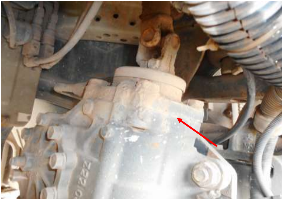
Photo 23 shows the steering box component (arrowed) at the undercarriage of the Motor Lorry was found to be intact without any visible damage. There was also no sign of fluid stain(s) observed on the various undercarriage components.
