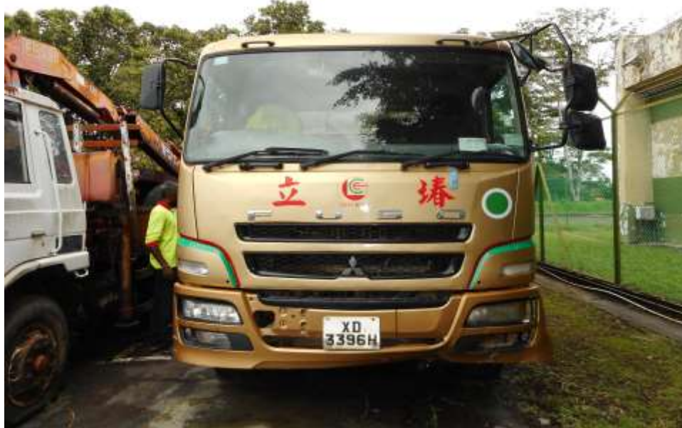
Photo 2 shows a general view of the front body of the Motor Lorry at the time of my inspection. The Motor Lorry was observed to have sustained minor damage to its frontal portion; its front bumper was damaged as a result of the accident.
