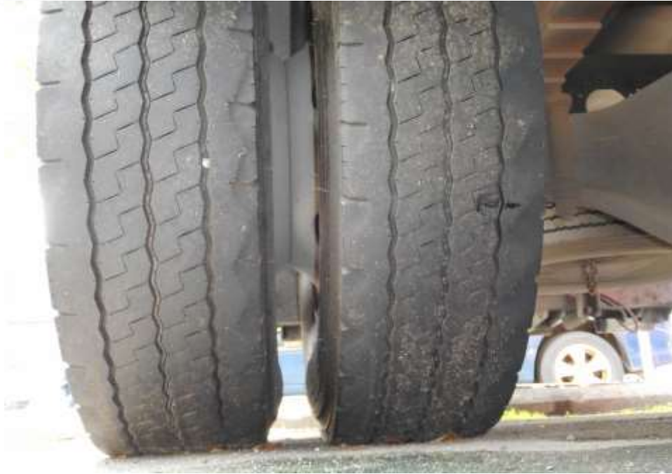
Photo 10 shows the condition of the front left tyres of the Motor Lorry, which were observed to be in serviceable condition with remaining tread depth of approximately 10.3mm. There was also no tear, cut or burst mark(s) on the outer and the inner sidewalls as well as across the tread of the 6 tyres that were fitted on the Motor Lorry.
