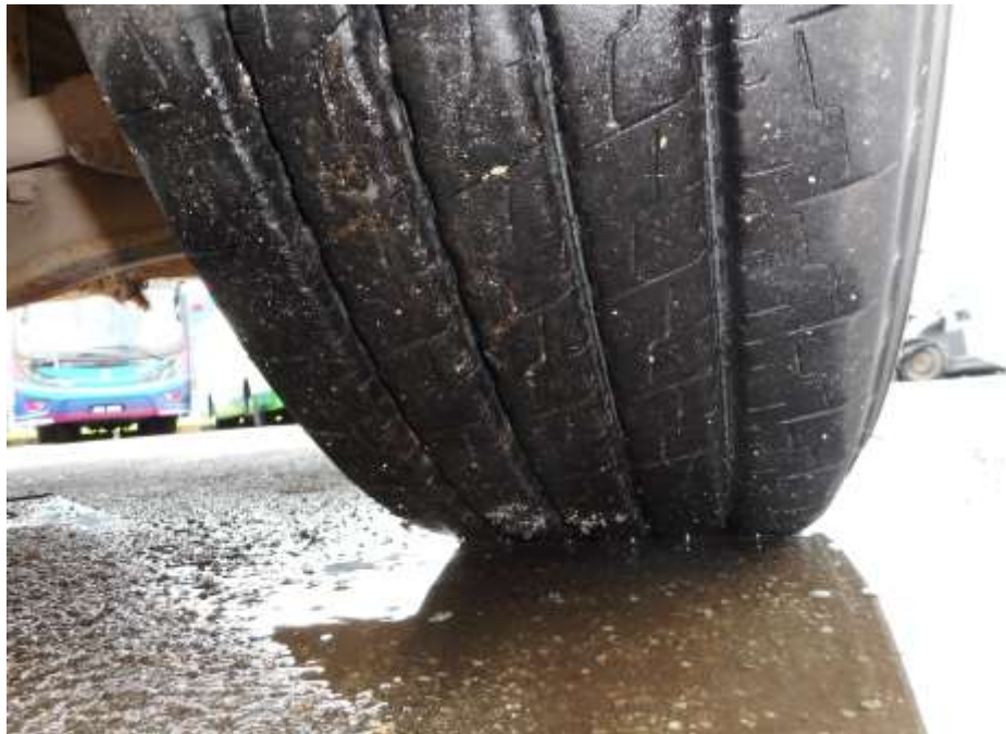
Photo 7 shows the condition of the front right tyre of the Motor Lorry, which was observed to be in serviceable condition with remaining tread depth of approximately 11 mm. The tyre, which was wrapped around standard steel wheel rim, was also observed to be sufficiently inflated for vehicular operation. There was no tear, cut or burst mark(s) on the outer and the inner sidewalls as well as across the tread of the 6 tyres that were fitted on the Motor Lorry.
