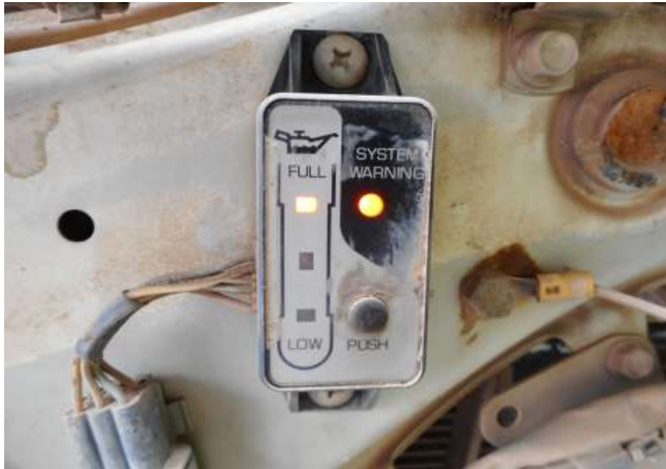
Photo 15 shows the engine oil dip stick system of the Motor Lorry at the time of my inspection. The engine oil was observed to be of sufficient level and without any visible contamination.
