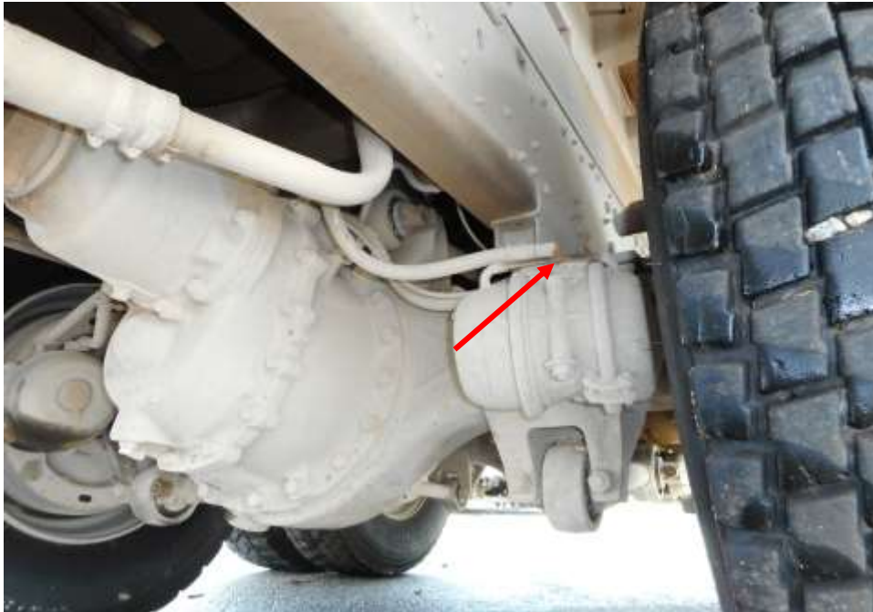
Photo 17 shows the brake pipe (arrowed) at the rear left wheel of the Motor Lorry. I did not observe any leakage of brake fluid at the time of my inspection of the Motor Lorry. My static tests of the Motor Lorry's braking system, along with my visual examination of the various mechanical components in the braking system, had indicated that there was no internal leakage of pressure/vacuum. Hence the braking system of the Motor Lorry was likely to be in serviceable condition at the material time of accident.
