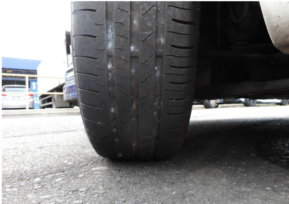
Photo 9 shows the condition of the front left tyre of the Police Car, which was observed to be in serviceable condition with remaining tread depth of approximately 4.5mm. The tyre was sufficiently inflated for vehicular operation with no tear, cut or burst mark(s) on the outer and the inner sidewalls as well as across the tread. The 4 tyres of the Police Car were wrapped around standard alloy wheel rims that were without any significant damage apart for some relatively minor kerb grazing type of damage on the outer side of the wheel rims.
