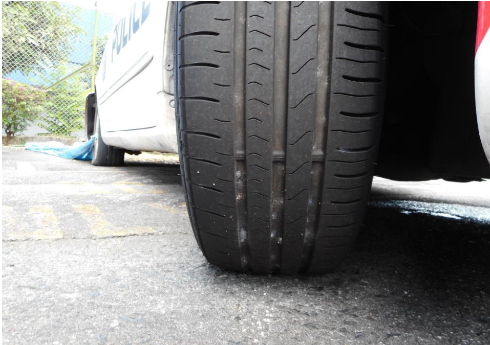
Photo 10 shows the condition of the front right tyre of the Police Car, which was observed to be in serviceable condition with remaining tread depth of approximately 5.4mm. The tyre was also observed to be sufficiently inflated for vehicular operation with no tear, cut or burst mark(s).
