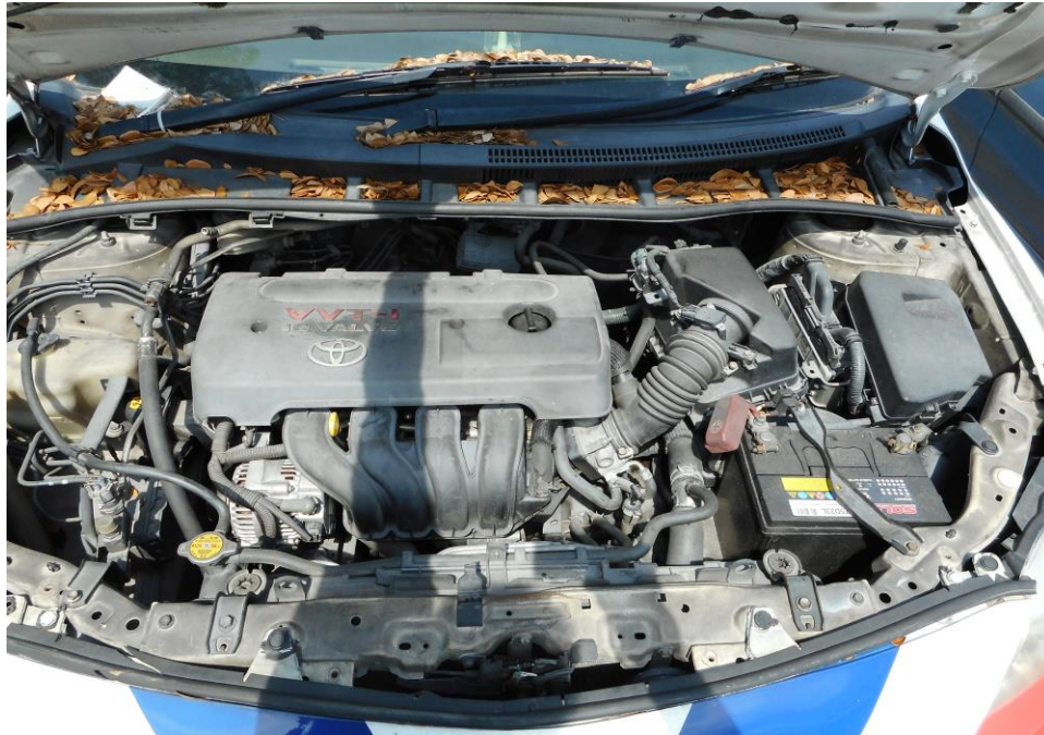
Photo 13 shows a general view of the Police Car's engine compartment. The various parts and components inside the engine compartment were unaffected by the accident. There was also no sign(s) or indication(s) of fluid leakage and/or fluid stain within the engine compartment.
