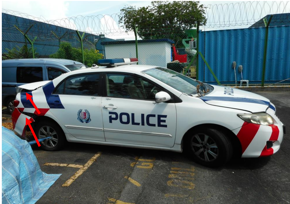
Photo 8 shows a general view of the Police Car's right body at the time of my inspection. The right portion of the Police Car was observed to have been unaffected by the accident, other than the damage at the rear bonnet and bumper (arrowed)
