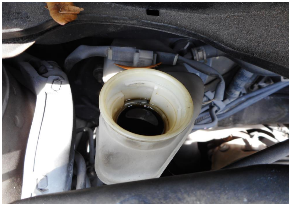
Photo 14 shows the brake fluid reservoir of the Police Car at the time of my inspection. The brake fluid was observed to be of sufficient level and without any visible contamination.
