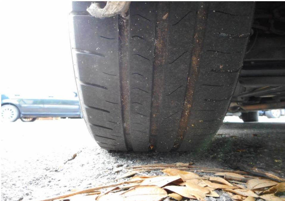
Photo 11 shows the condition of the rear left tyre of the Police Car, which was observed to be in serviceable condition with remaining tread depth of approximately 5mm. The tyre, which was wrapped around alloy wheel rim, was also observed to be sufficiently inflated for vehicular operation.
