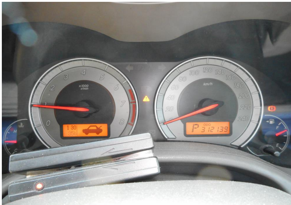
Photo 24 shows no warning lights illuminated on the instrument panel of the Police Car after the engine was cranked. This would suggest that there was no abnormality to the various electronic operating systems of the Police Car, like the ABS, EPS, TC and SRS etc.
