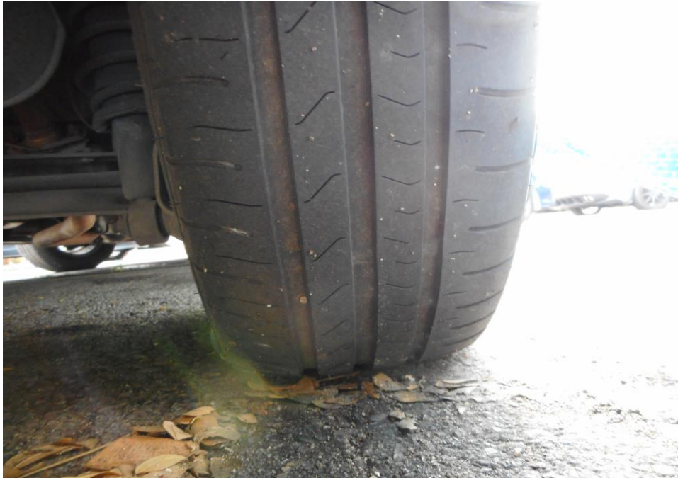
Photo 12 shows the condition of the rear right tyre of the Police Car, which was observed to be in serviceable condition with remaining tread depth of approximately 5.2mm. There was also no tear, cut or burst mark(s) on the outer and the inner sidewalls as well as across the tread of the Police Car's 4 tyres.
