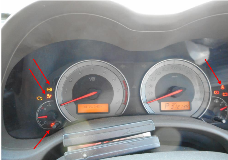
Photo 23 shows the warning light for Anti-Lock Brake System (ABS), Electric Power Steering System (EPS), Traction Control (TC) and Supplemental Restraint System (SRS) appearing on the instrument panel of the Police Car during the self-test of its various electronic operating systems when its engine was cranked.
