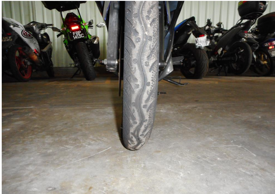
Photo 7 shows the front tyre of the Motorcycle. The front tyre was observed to be in serviceable condition with remaining tread depth of 3.5mm. The tyre was also observed to be sufficiently inflated for vehicular operation. See photo above.
