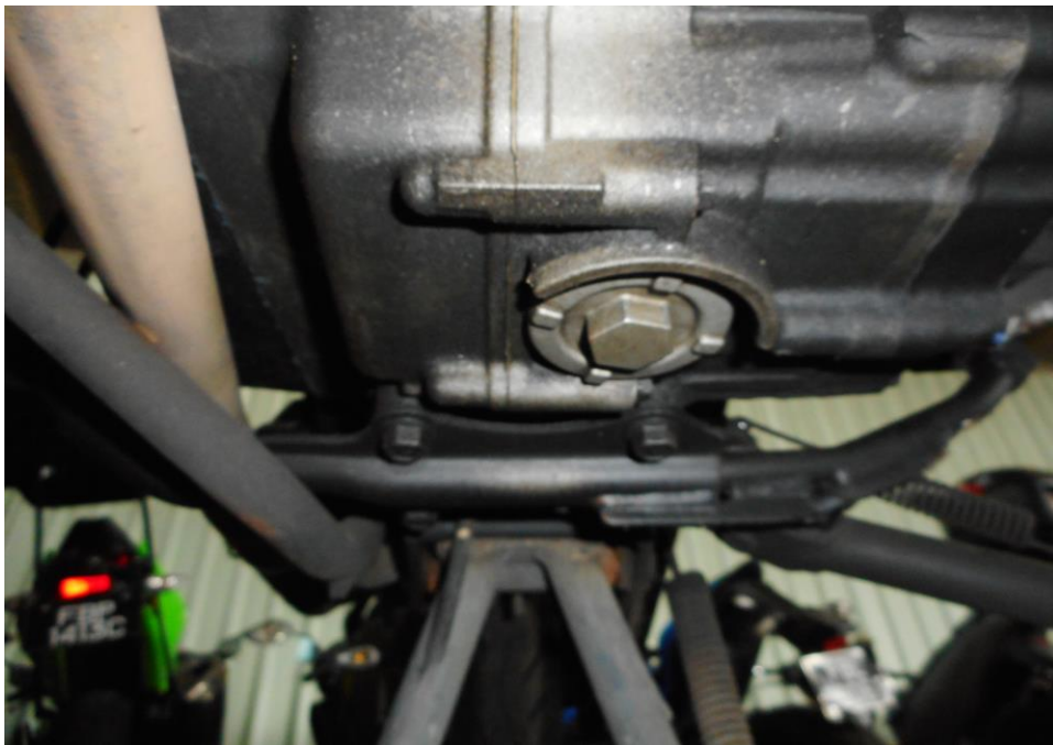
Photo 9 shows no sign(s) or indication(s) of fluid leak observed around the undercarriage of the engine area of the Motorcycle.
