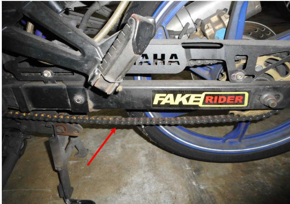
Photo 12 shows the general view of the gear train (arrowed) of the Motorcycle, which was observed to be intact with no misalignment. It was also adequately lubricated for operating purposes. Free play tension was observed & found adequately acceptable.
