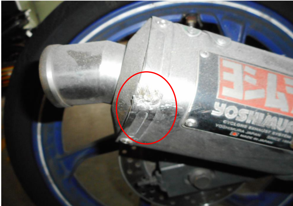
Photo 6 shows a close up view of the exhaust muffler of the Motorcycle at the time of our inspection. The Motorcycle was observed to have sustained relatively minor damages at time of inspection.
