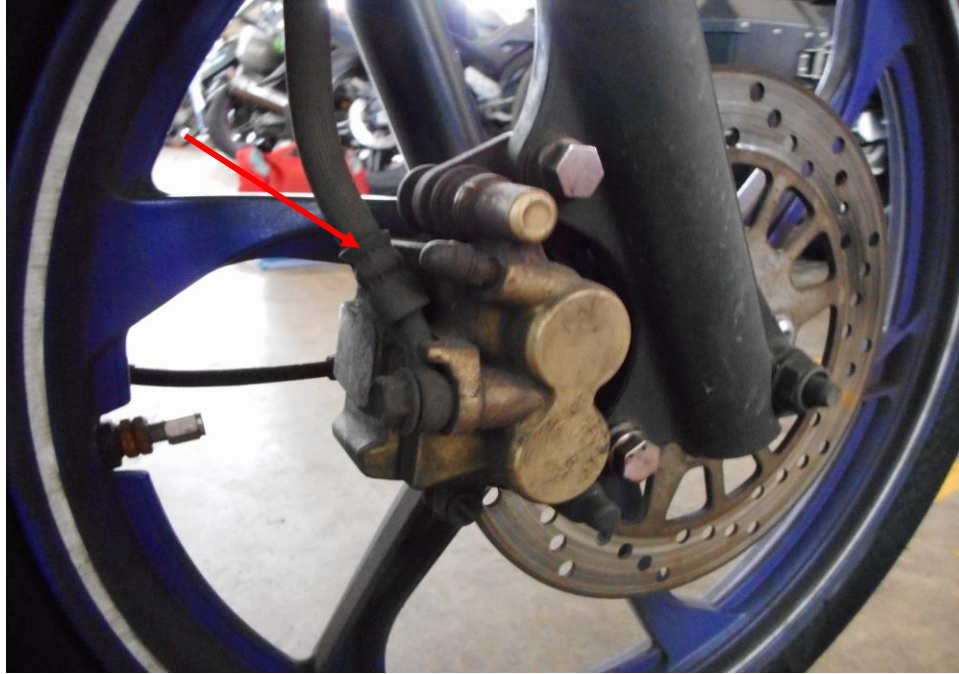
Photo 14 shows our checks on the brake callipers housing (front). There was also no sign(s) or indication(s) of fluid leak observed around the Motorcycle.
