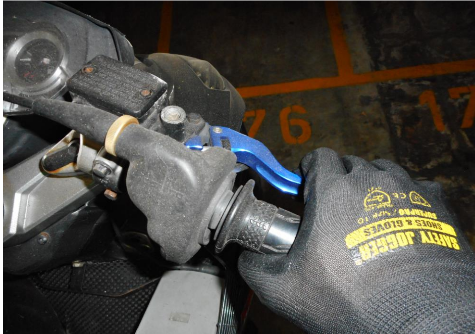
Photo 18 shows testing of the braking of the front brake in progress. The braking force was felt upon pressing the brake lever. The brakes are in serviceable condition.
