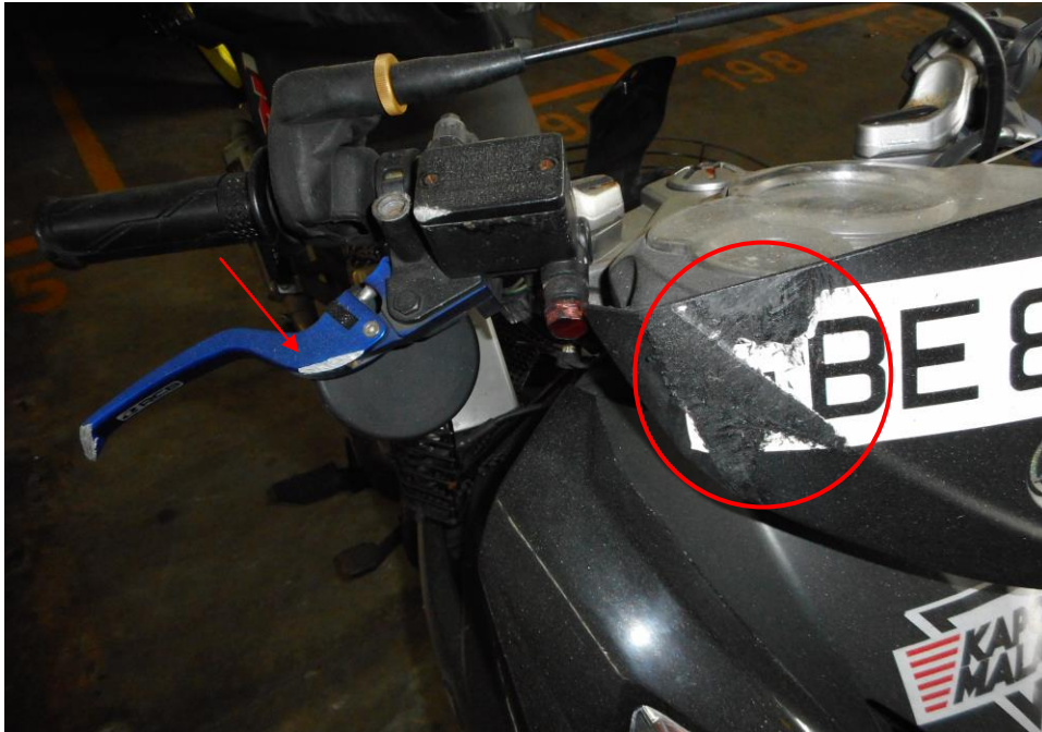
Photo 4 shows a close up view of the front body of the Motorcycle at the time of our inspection. The Motorcycle was observed to have sustained relatively minor damages at time of inspection. The damages were observed to be confined to its number plate and brake lever of the Motorcycle.
