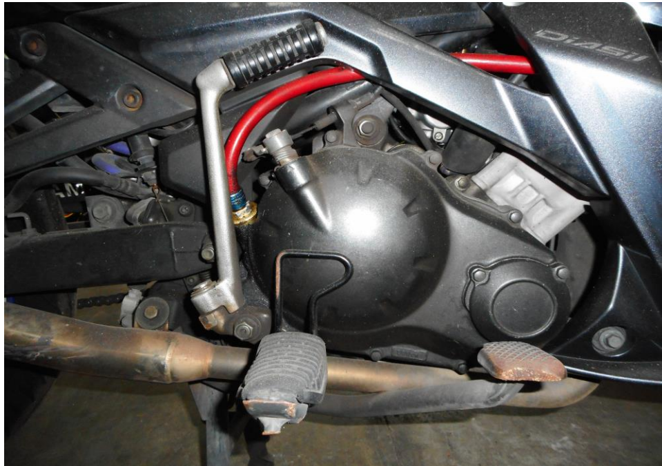
Photo 10 shows no sign(s) or indication(s) of fluid leakage stain observed around the engine area of the Motorcycle.
