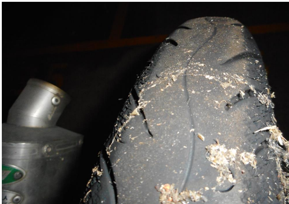
Photo 8 shows the rear tyre of the Motorcycle. The rear tyre was observed to be in serviceable condition with remaining tread depth of 1.6mm. The tyre was also observed to be sufficiently inflated for vehicular operation. See above.
