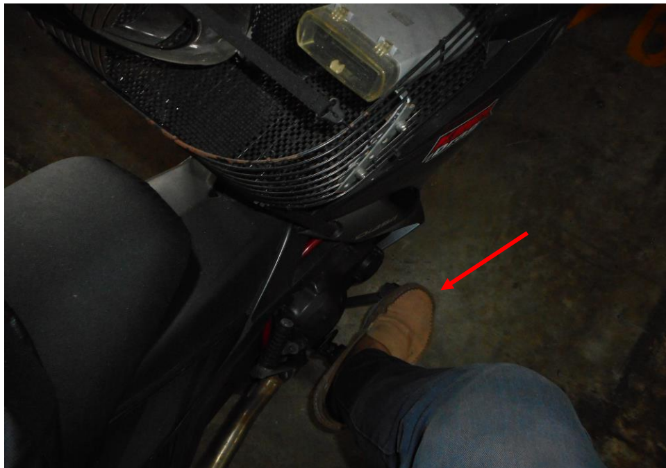
Photo 19 shows testing of the braking of the rear brake in progress. The braking force was felt upon stepping on the brake lever. The brakes are in serviceable condition
