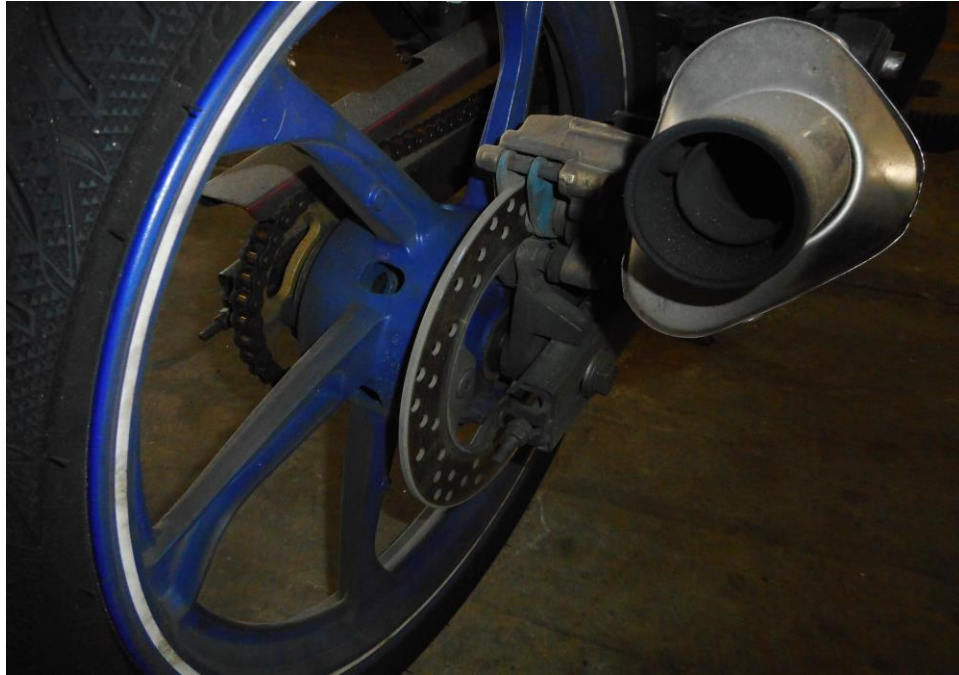
Photo 16 shows a general of the brake calliper (rear) no leakage or fluids is present around it, and without contamination.
