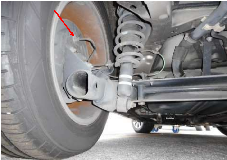
Photo 15 shows the brake hose/pipe (arrowed) at the rear left wheel of the Motor Car. I did not observe any leakage of brake fluid at the time of my inspection of the Motor Car. Static tests of the Motor Car's braking system had indicated that there was no internal leakage of pressure/vacuum. The undercarriage components of the Motor Car were also all found to be intact and without any visible damage.
