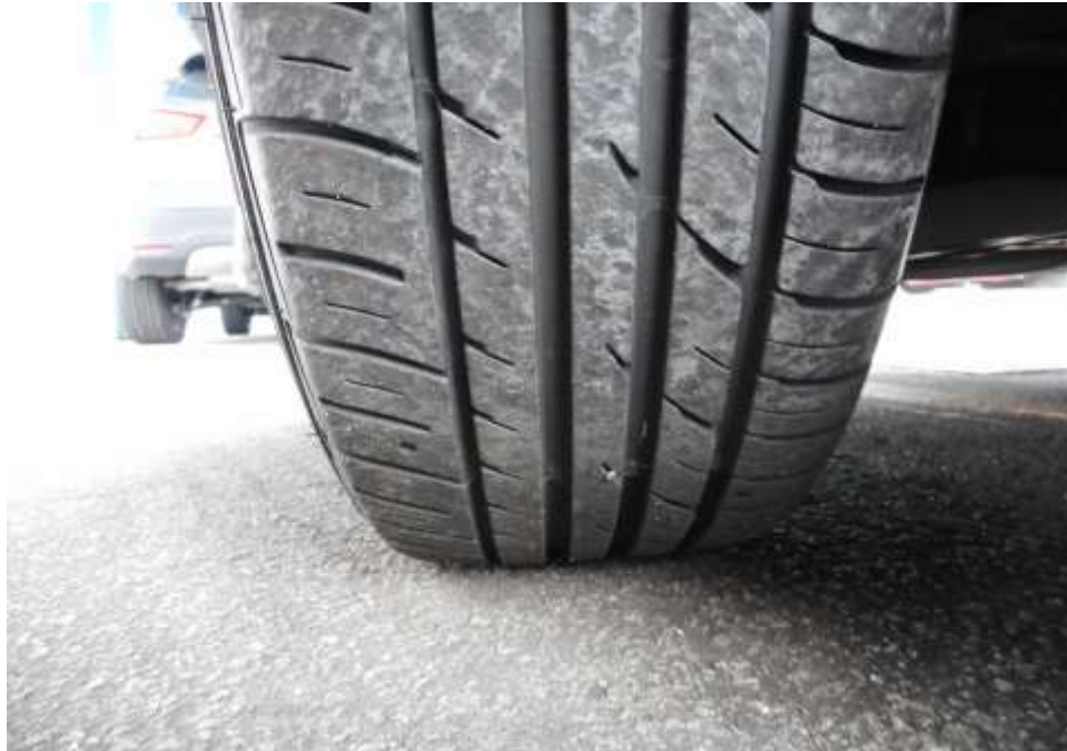
Photo 6 shows the condition of the front left tyre of the Motor Car, which was observed to be in serviceable condition with remaining tread depth of approximately 6.1mm. The tyre was sufficiently inflated for vehicular operation with no tear, cut or burst mark(s) on the outer and the inner sidewalls as well as across the tread. The 4 tyres of the Motor Car were wrapped around standard alloy wheel rims without any damage.
