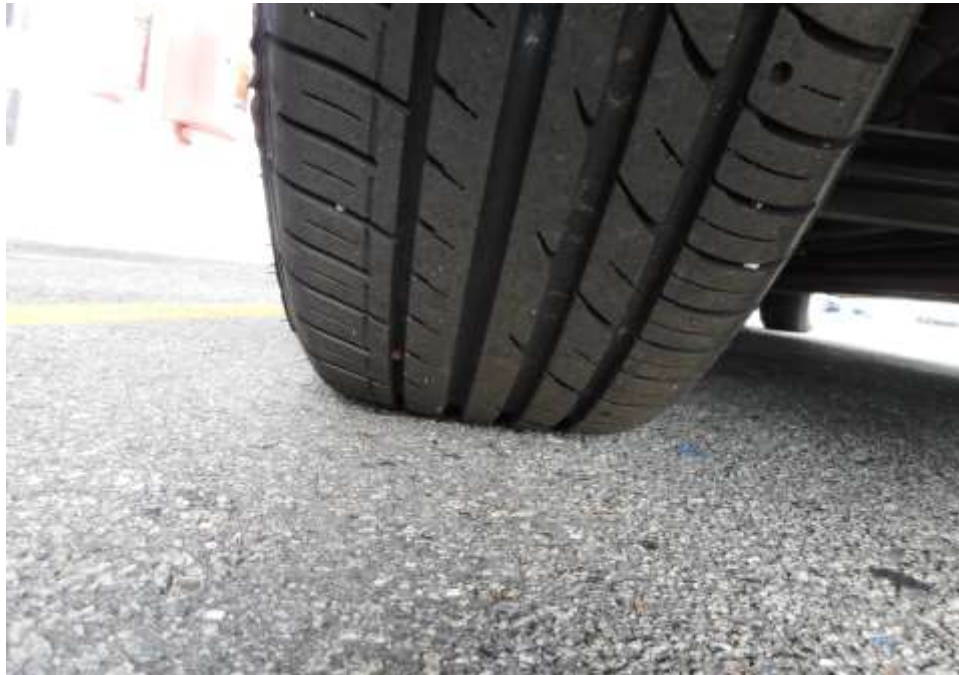
Photo 8 shows the condition of the rear left tyre of the Motor Car, which was observed to be in serviceable condition with remaining tread depth of approximately 7mm. The tyre, which was wrapped around alloy wheel rim, was also observed to be sufficiently inflated for vehicular operation. The 4 tyres of the Motor Car were wrapped around standard alloy wheel rims that were without any significant damage apart for some relatively minor kerb grazing type of damage on the outer side of the wheel rims
