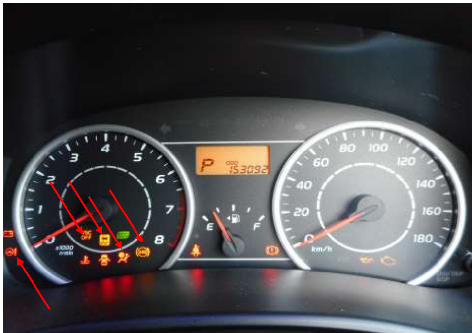
Photo 20 shows the warning light for Anti-Lock Brake System (ABS), Electric Power Steering System (EPS), Traction Control (TC) and Supplemental Restraint System (SRS) appearing on the instrument panel of the Motor Car during the self-test of its various electronic operating systems when its engine was cranked.
