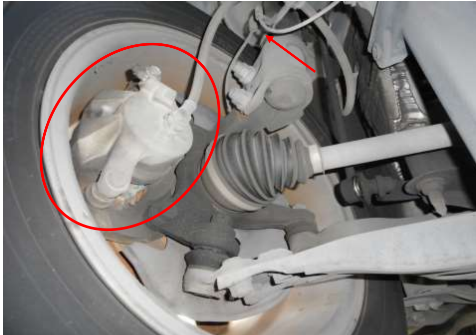
Photo 16 shows the brake hose/pipe (arrowed) at the front right wheel of the Motor Car. No leakage of brake fluid was observed. Visual examination of the various components of the braking system like the brake caliper (circled), brake booster, brake pedal etc had revealed all to be intact and without visible damage.
