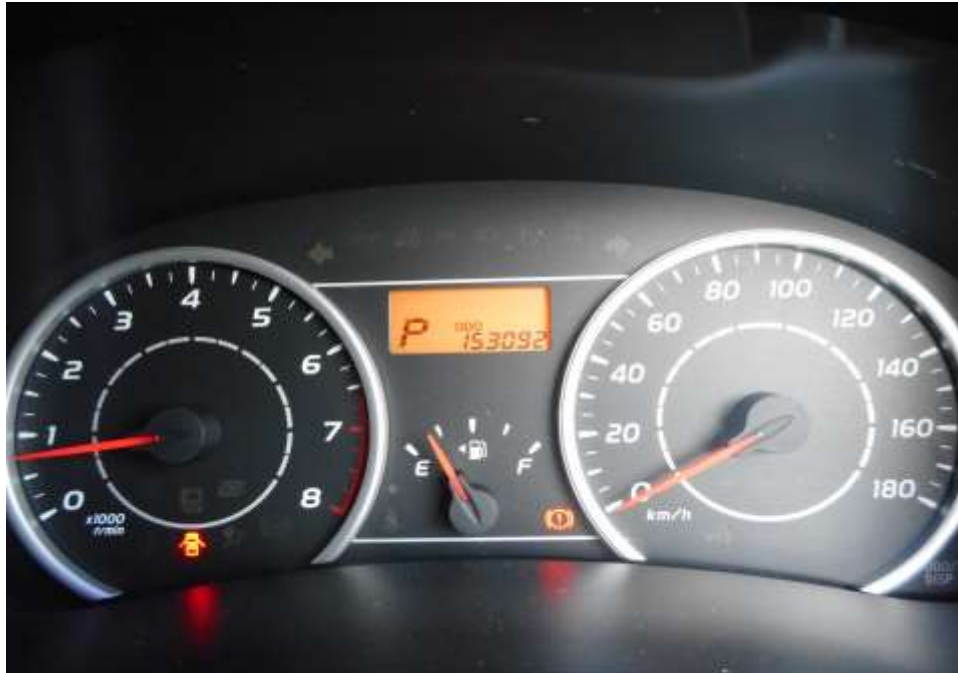
Photo 21 shows no warning lights illuminated on the instrument panel of the Motor Car after the engine was cranked. This would suggest that there was no abnormality to the various electronic operating systems of the Motor Car, like the ABS, EPS, TC and SRS etc.
