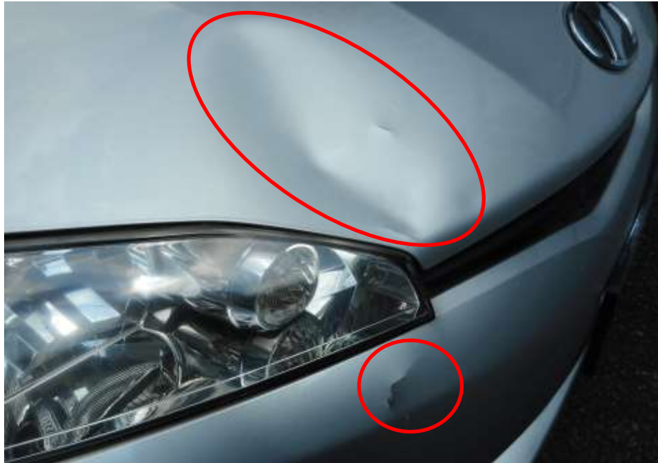
Photo 4 shows a close up view of the front body of the Motor Car at the time of my inspection. The Motor Car was observed to have sustained relatively minor damage at its frontal portion. Its front bonnet and bumper (circled) were damaged as a result of the accident.
