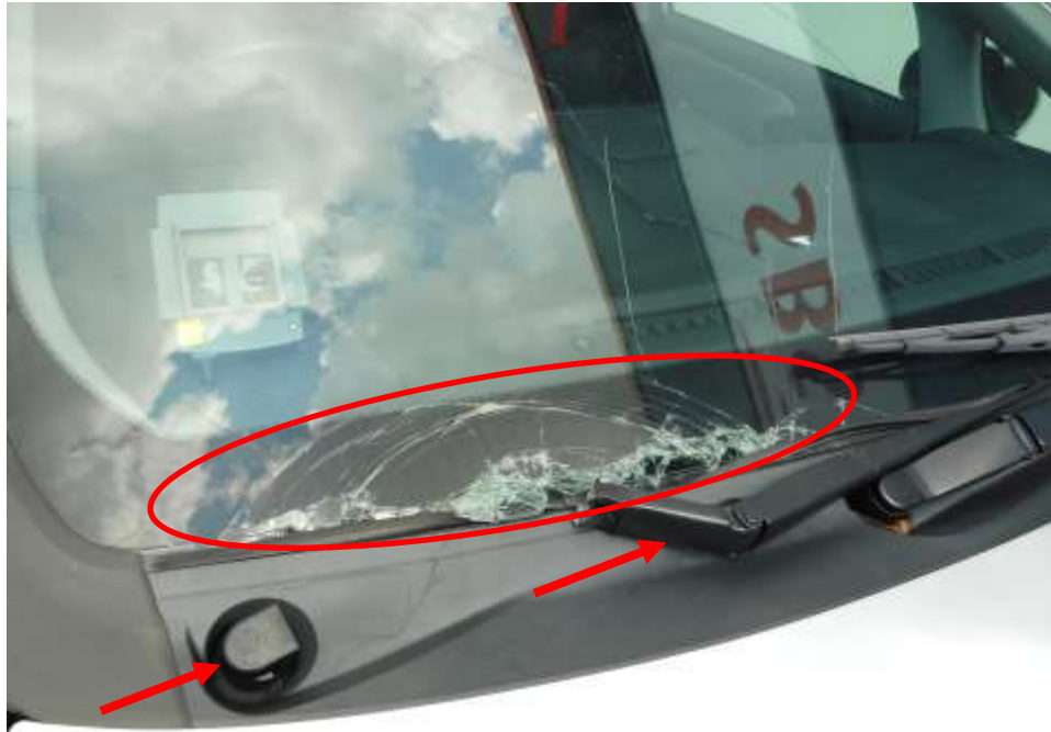
Photo 2 shows a close up view of the damaged front windscreen (circled) and right windscreen wiper (arrowed) of the Motor Car. The mileage of the Motor Car at the time of my inspection was recorded to be 111,492km.
