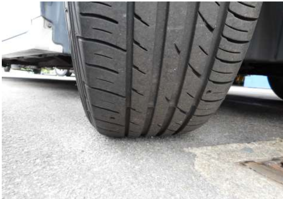
Photo 7 shows the condition of the front right tyre of the Motor Car, which was observed to be in serviceable condition with remaining tread depth of approximately 6.1mm. The tyre was also observed to be sufficiently inflated for vehicular operation with no tear, cut or burst mark(s).
