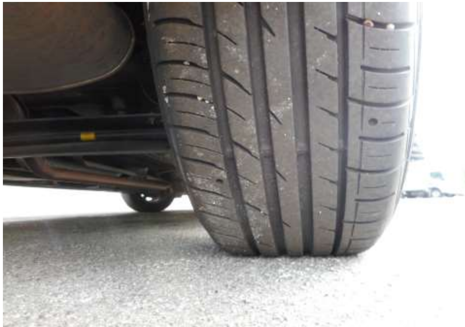
Photo 9 shows the condition of the rear right tyre of the Motor Car, which was observed to be in serviceable condition with remaining tread depth of approximately 7mm. There was also no tear, cut or burst mark(s) on the outer and the inner sidewalls as well as across the tread of the Motor Car's 4 tyres.
