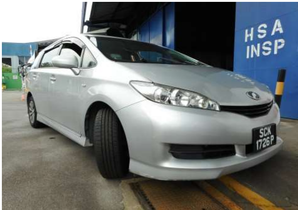
Photo 17 shows the front right wheel of the Motor Car turned to its full right. During my steering system test, I did not experience any abnormal free play and/or resistance when I had turned the steering wheel towards the left and right. This would suggest that the steering system of the Motor Car was likely to be in serviceable condition at the material time of accident.
