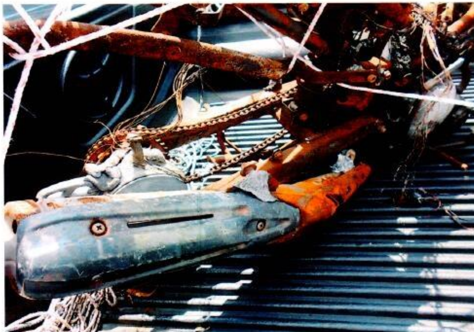
Photo 4 shows the general view of the right rear body of the Insured Motorcycle at the time of our inspection. The Insured Motorcycle was observed to have sustained extensive fire damage all around. Rust had accumulated all over the Insured Motorcycle as a result of exposure to environmental condition for a period of time.
