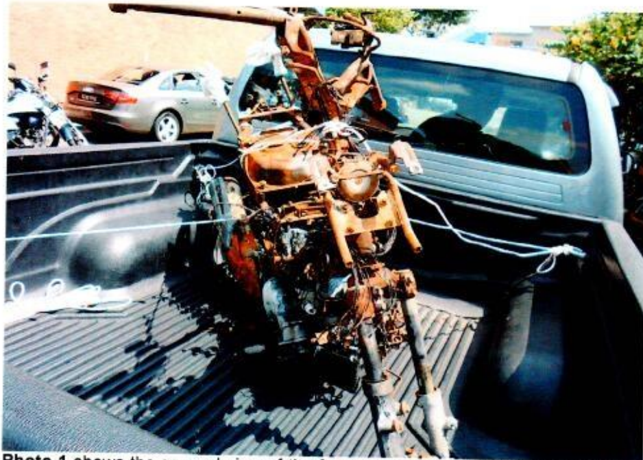
Photo 1 shows the general view of the front portion of the Insured Motorcycle at the time of our inspection. The Insured Motorcycle was observed to have sustained extensive fire damage all around. Rust had accumulated all over the Insured Motorcycle as a result of exposure to environmental condition for a period of time.
