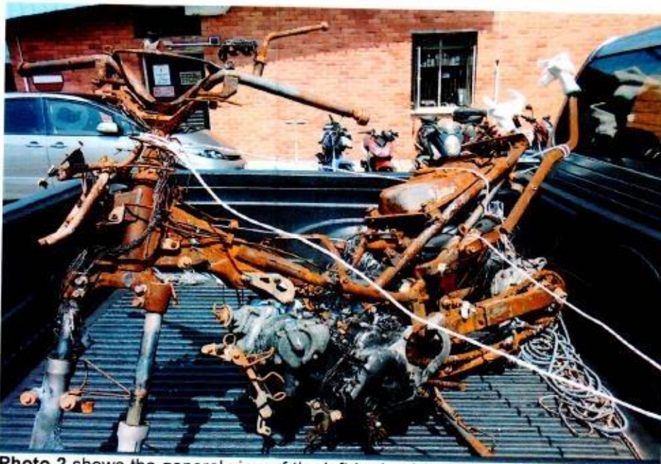
Photo 2 shows the general view of the left body of the Insured Motorcycle at the time of our inspection. The Insured Motorcycle was observed to have sustained extensive fire damage all around. Rust had accumulated all over the Insured Motorcycle as a result of exposure to environmental condition for a period of time.
