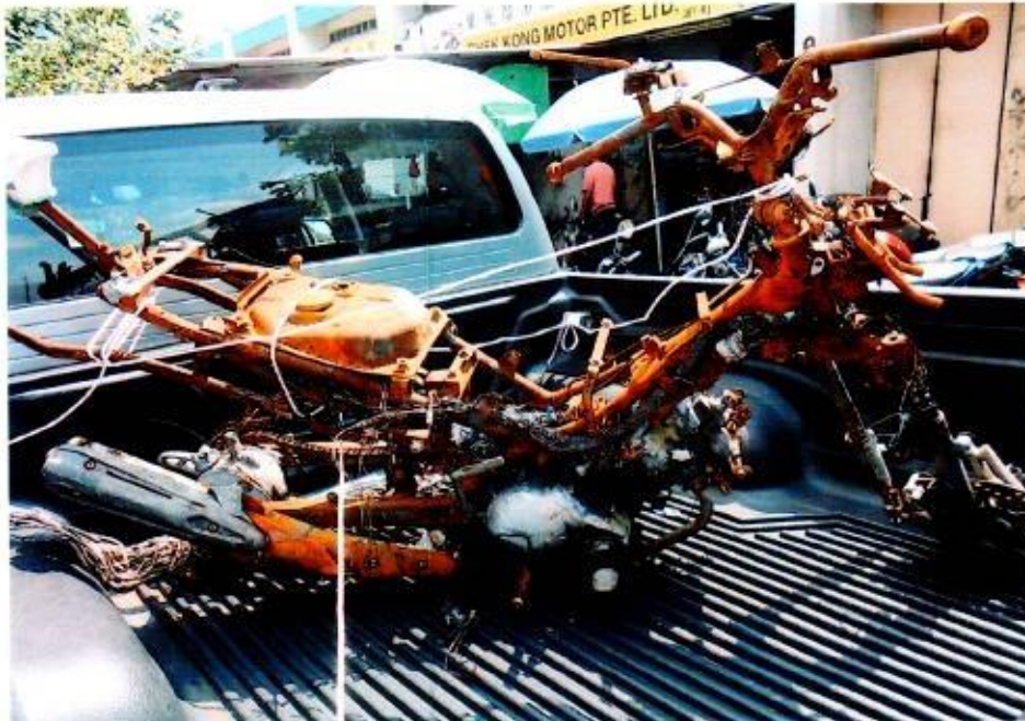
Photo 3 shows the general view of the right body of the Insured Motorcycle at the time of our inspection. The Insured Motorcycle was observed to have sustained extensive fire damage all around. Rust had accumulated all over the Insured Motorcycle as a result of exposure to environmental condition for a period of time.
