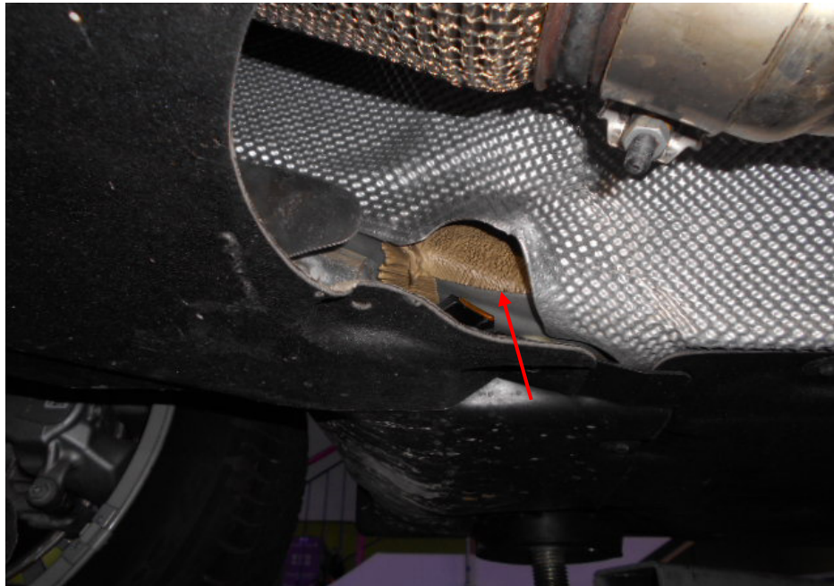
Photo 16 shows the structural body at the underside right front of the Motor Car. The original factory sealant (arrowed) at the joints along the chassis body was untouched, indicating no work was done on the chassis body of the Motor Car and that the chassis body was originally fitted.
