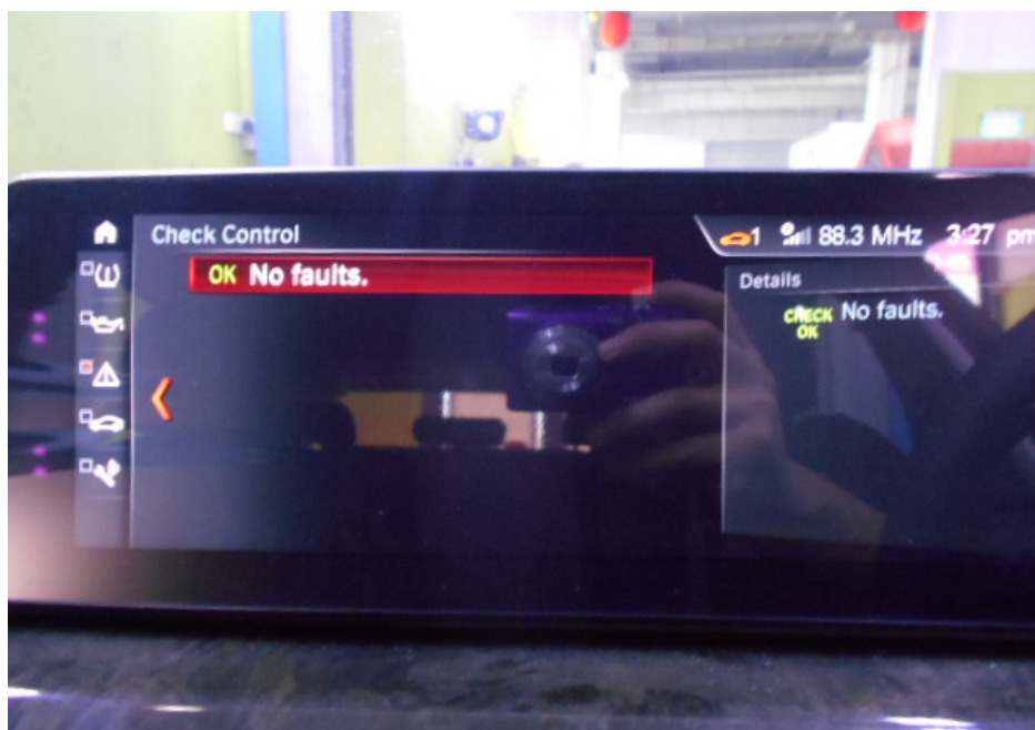
Photo 8 shows no fault(s) was detected to the various controls and systems of the Motor Car after my initiation of the Motor Car's on-board self-diagnostic check.
