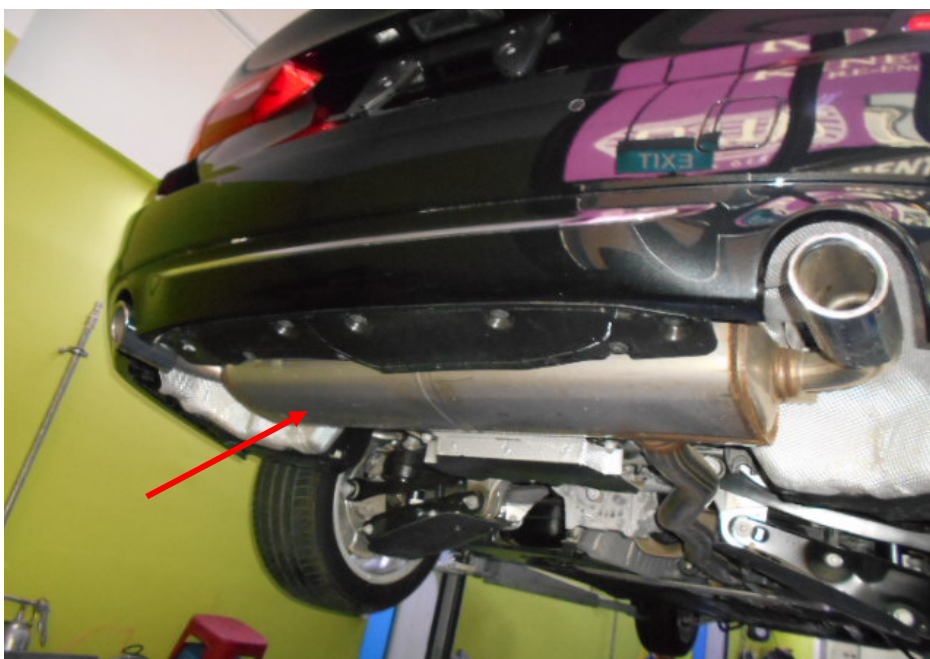
Photo 13 shows the Motor Car's rear exhaust muffler (arrowed). My examination of the Motor Car's exhaust system revealed no sign(s) or indication(s) of any cut or weld marks along its exhaust pipes and on its rear mufflers.
