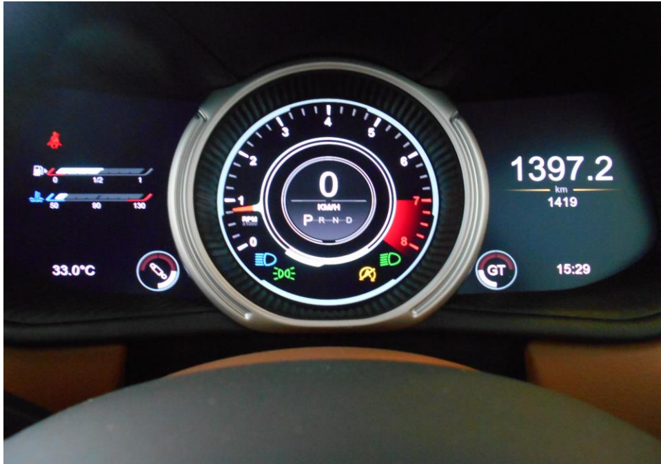
Photo 21 shows most warning lights disappearing from the instrument panel of the Motor Car after the engine was cranked.
