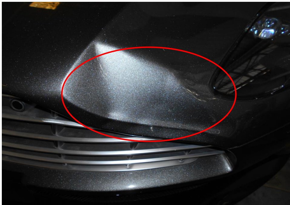
Photo 6 shows a close up view of the front left lower bonnet of the Motor Car at the time of our inspection. The Motor Car had sustained relatively minor damages at the front lower bonnet of the Motor Car.
