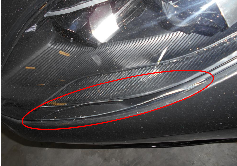
Photo 7 shows a close up view of the front left headlamp of the Motor Car at the time of our inspection. The Motor Car had sustained relatively minor scratches at the headlamp of the Motor Car.
