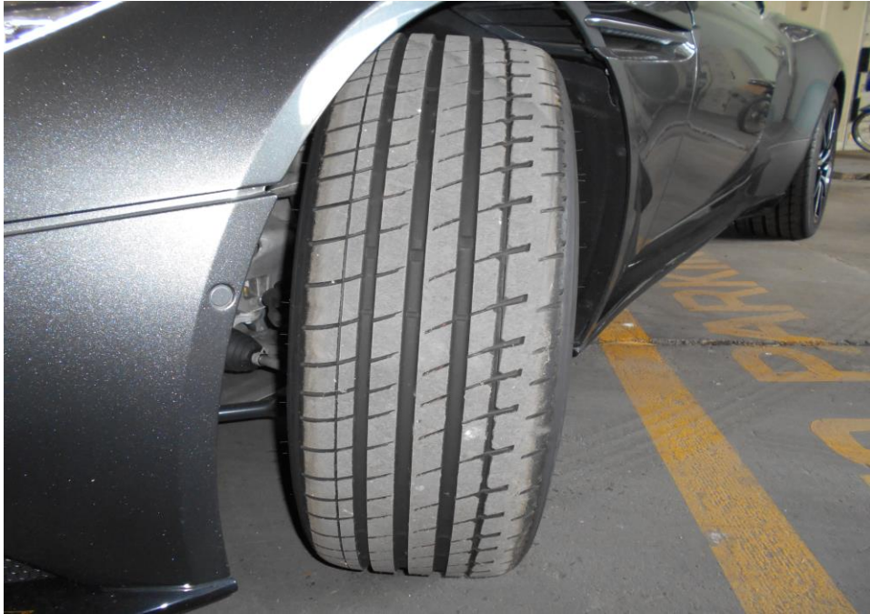
Photo 10 shows the condition of the front left tyre of the Motor Car, which was observed to be in serviceable condition with remaining tread depth of approximately 7mm. The tyre, which was wrapped around alloy wheel rim, was also observed to be sufficiently inflated for vehicular operation.
