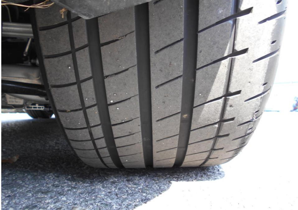
Photo 12 shows the condition of the rear right tyre of the Motor Car, which was observed to be in serviceable condition with remaining tread depth of approximately 7mm.
