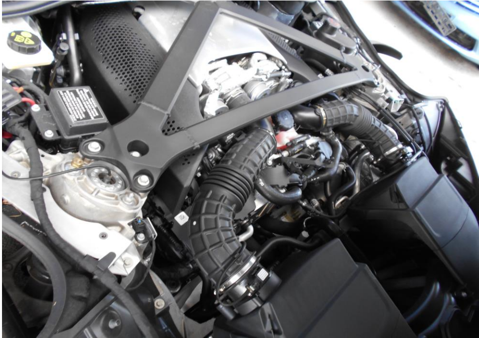
Photo 13 shows a general view of the Motor Car's engine compartment. The various parts and components inside the engine compartment were unaffected by the accident. There was also no sign(s) or indication(s) of fresh fluid leakage and/or fluid stain within the engine compartment.
