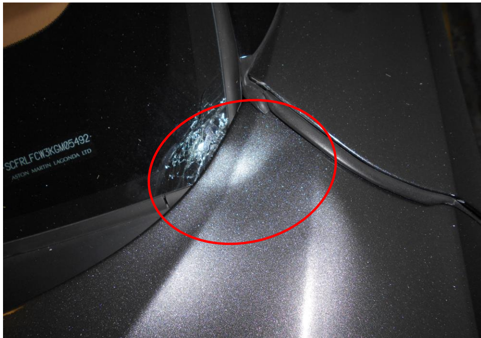
Photo 8 shows a close up view of the front left lower windshield and upper left portion of the front bonnet of the Motor Car at the time of our inspection. The Motor Car had sustained relatively minor damages as a result of the accident.
