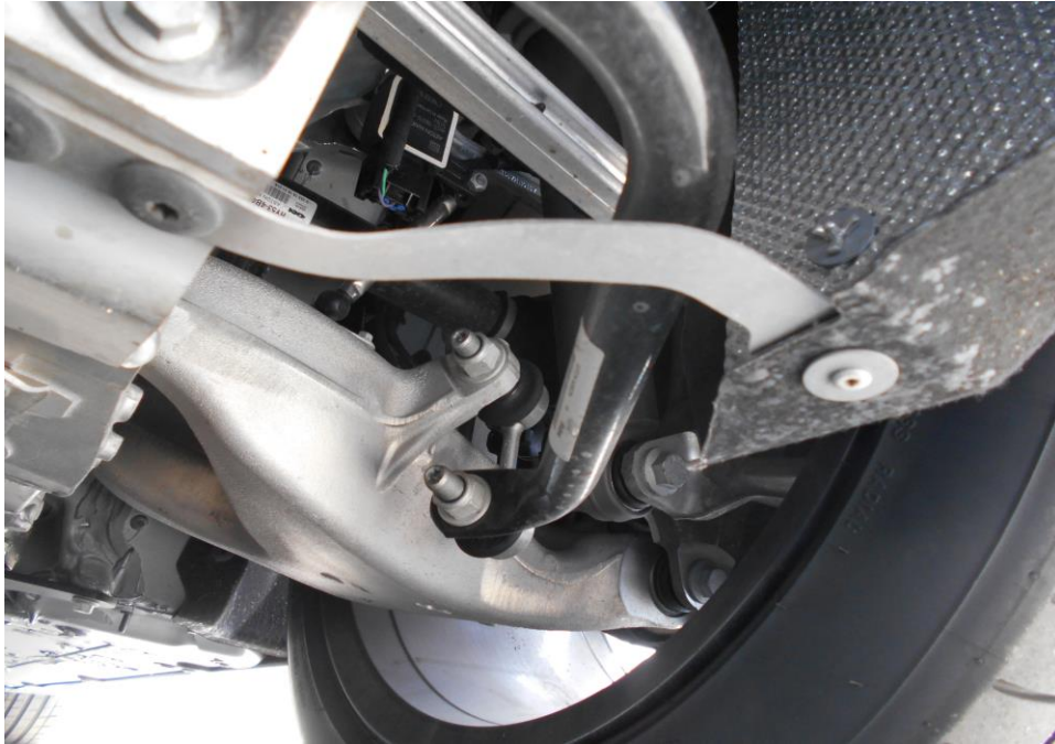
Photo 18 shows the brake hose at the rear right wheel of the Motor Car. We did not observe any leakage of brake fluid at the time of our inspection of the Motor Car. Our visual inspection of the various mechanical components of the Motor Car's braking system revealed all to be intact without visible damage.
