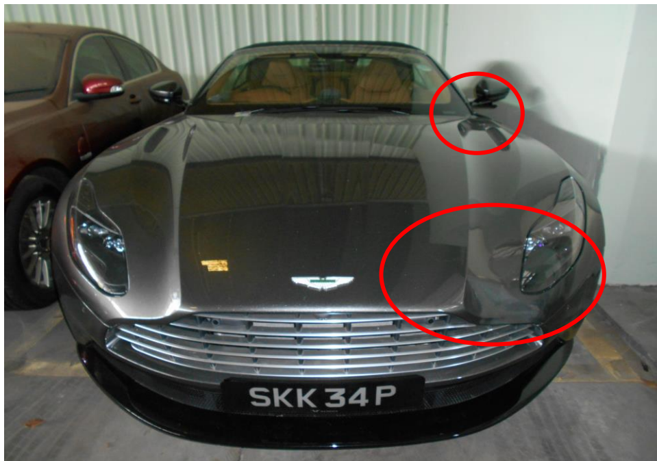
Photo 2 shows a general view of the front body of the Motor Car at the time of our inspection. The Motor Car was observed to have sustained a relatively minor impact damages that was confined to its front left portion. Its lower left bonnet, left side fender and lower left windshield was observed to be damaged likely due to the accident.
