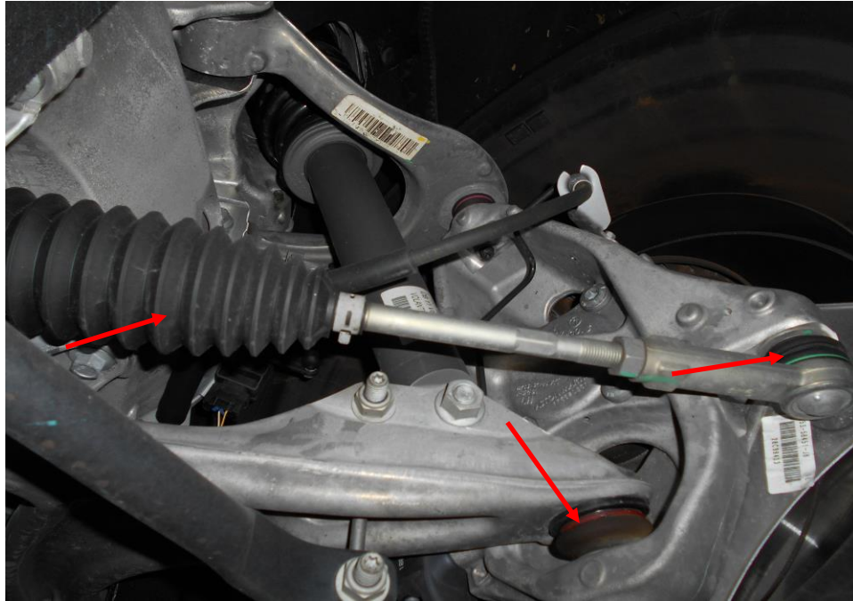
Photo 20 shows the various undercarriage components at the front left wheel of the Motor Car. We did not observe any leakage of brake fluid (arrowed) at the time of our inspection of the Motor Car. Our visual inspection of the various mechanical components of the Motor Car's braking system revealed all to be intact and without visible damage, indicating that the braking system was likely to be in serviceable condition at the material time of accident.
