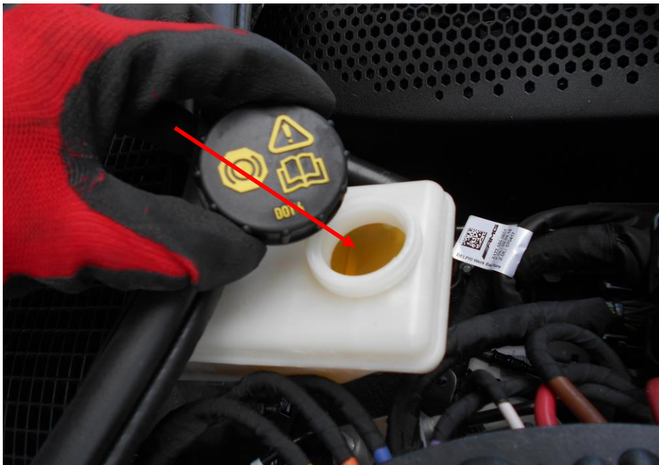
Photo 14 shows the brake fluid reservoir of the Motor Car at the time of our inspection. The brake fluid was observed to be of sufficient level (arrowed) and without any visible contamination.
