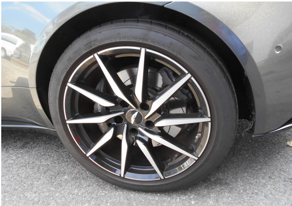
Photo 11 shows the condition of the rear left tyre of the Motor Car, which was observed to be in serviceable condition with remaining tread depth of approximately 7mm.
