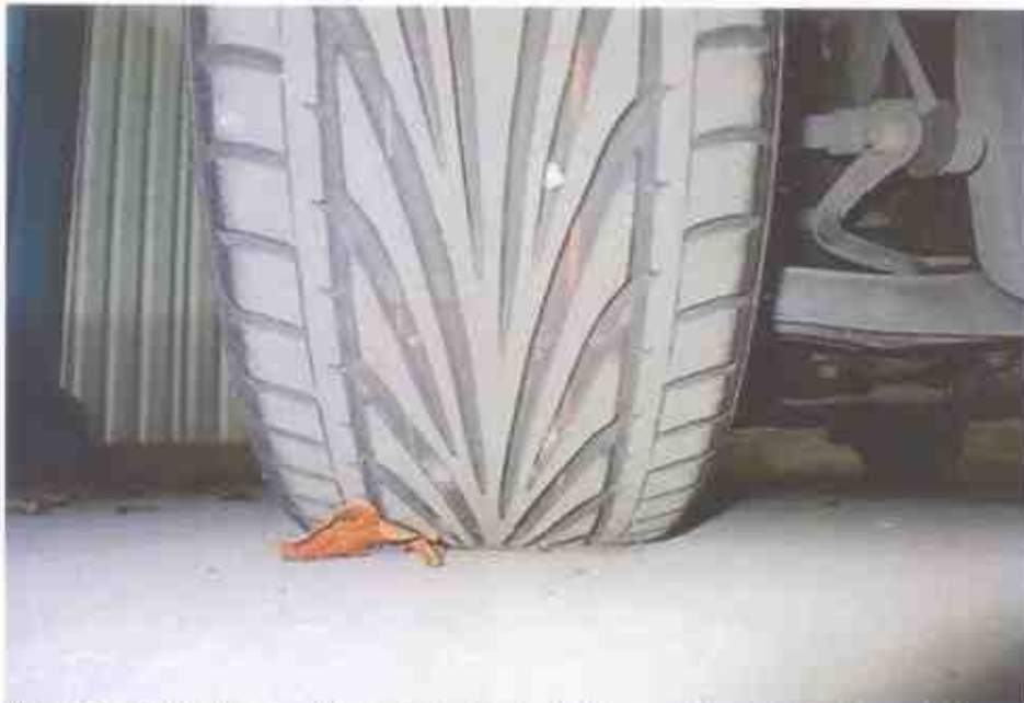
Photo 7 shows the condition of the front right tyre of the Motor Car, which was observed to be in serviceable condition with remaining tread depth of approximately 4mm. The tyre, which was wrapped around alloy wheel rim, was also observed to be sufficiently inflated for vehicular operation.
