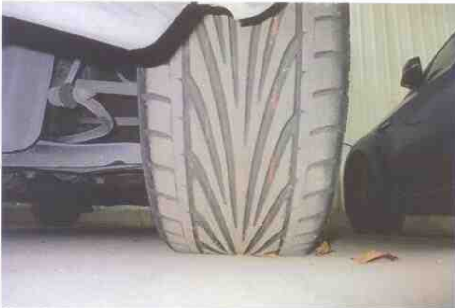
Photo 6 shows the condition of the front left tyre of the Motor Car, which was observed to be in serviceable condition with remaining tread depth of approximately 6mm. The tyre, which was wrapped around alloy wheel rim, was also observed to be sufficiently inflated for vehicular operation. There was no tear, cut or burst mark(s) on the outer and the inner sidewalls as well as across the tread of the 4 tyres.
