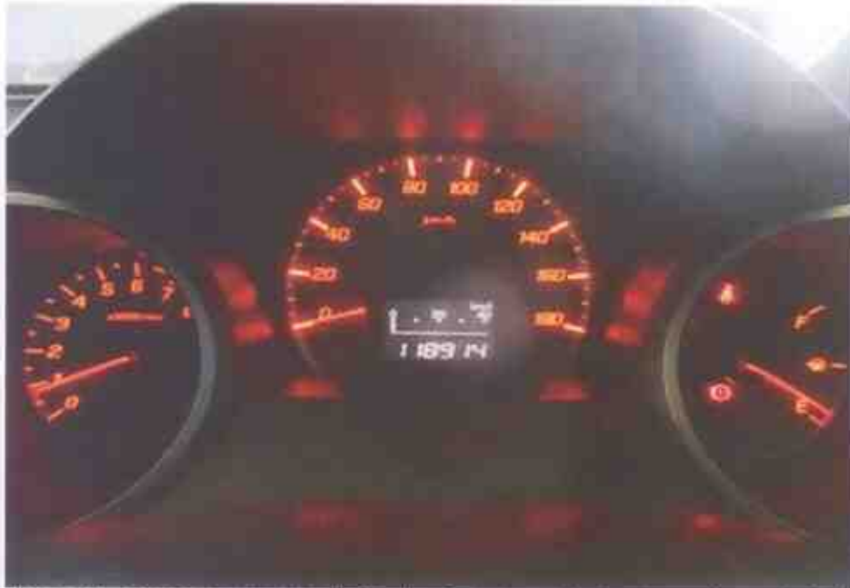
Photo 21 shows no warning lights illuminated on the instrument panel of the Motor Car after the engine was cranked. This would suggest that there was no abnormality to the various electronic operating systems of the Motor Car, like the EPS and SRS etc.
