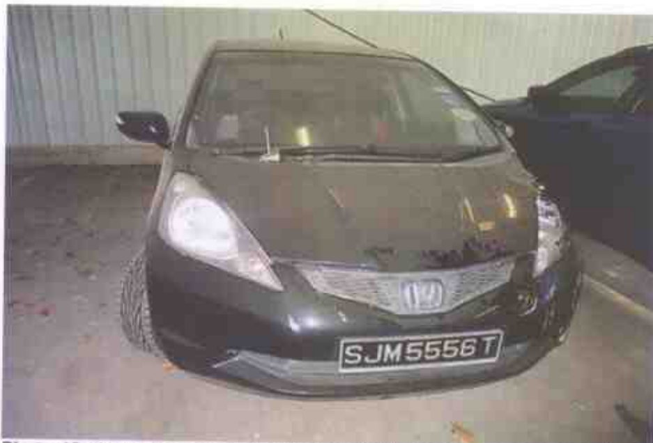
Photo 19 shows the front right wheel of the Motor Car turned to its full right. During our steering system test, we did not experience any abnormal free play and/or resistance when we had turned the steering wheel towards the left and right. This would suggest that the steering system of the Motor Car was likely to be in serviceable condition at the material time of accident.
