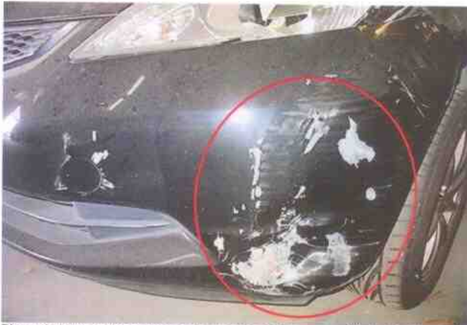
Photo 4 shows a closer view of the cracked front bumper of the Motor Car at the time of our inspection (circled).
