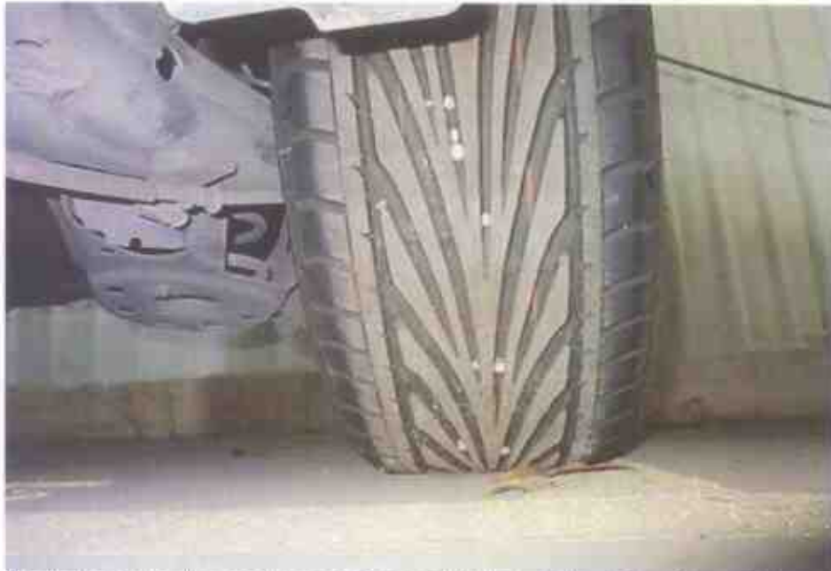
Photo 8 shows the condition of the rear left tyre of the Motor Car, which was observed to be in serviceable condition with remaining tread depth of approximately 8mm. The tyre, which was wrapped around alloy wheel rim, was also observed to be sufficiently inflated for vehicular operation. There was also no damage found on the 4 wheel rims of the Motor Car.
