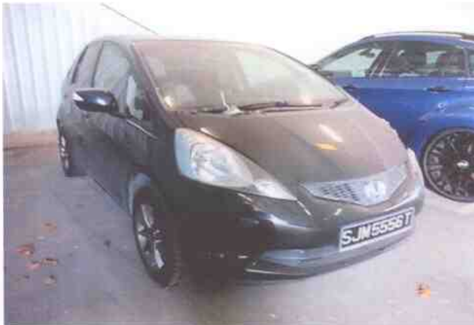
Photo 1 shows a general view of the front right body of the Motor Car at the time of our inspection. The Motor Car was observed to be in good general condition except for some relatively minor impact damage at its left frontal portion. The mileage of the Motor Car was recorded to be 118, 914km.
