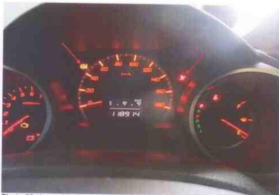
Photo 20 shows the warning lights for the various electronic operating systems of the Motor Car appearing on its instrument panel during the self-test when the engine is cranked, in particular the EPS light and SRS light (arrowed).
