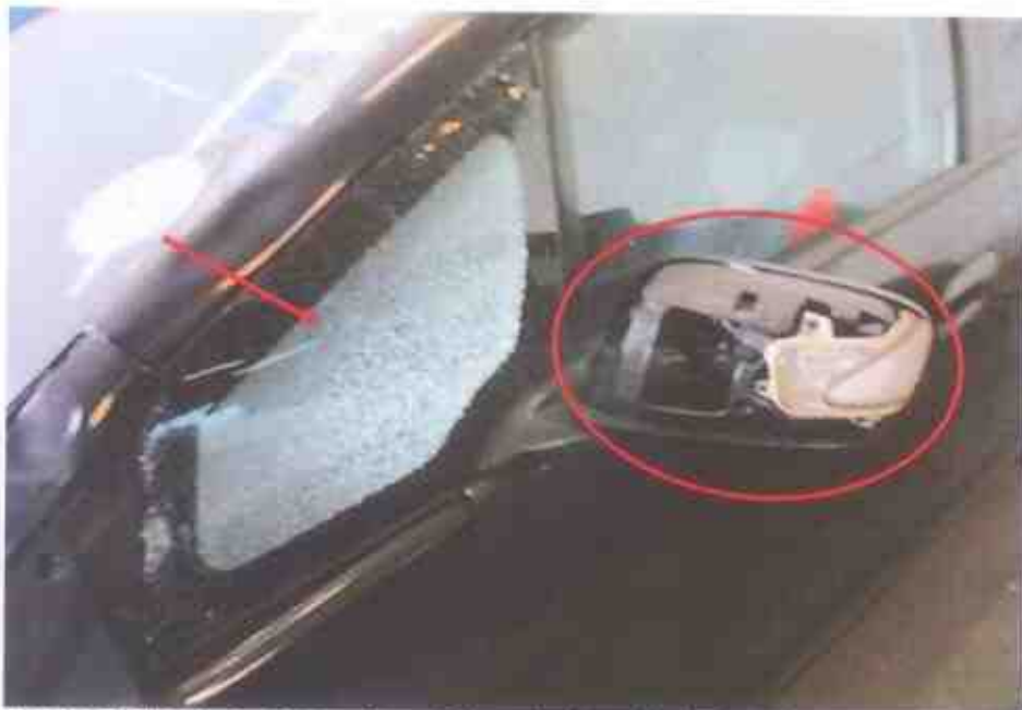
Photo 5 shows a closer view of the shattered left front door quarter glass (arrowed) as well as the missing left side mirror cover (circled) of the Motor Car at the time of our inspection.
