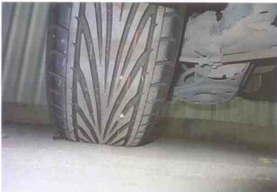
Photo 9 shows the condition of the rear right tyre of the Motor Car, which was observed to be in serviceable condition with remaining tread depth of approximately 6mm. There was also no tear, cut or burst mark(s) on the outer and the inner sidewalls as well as across the tread of the 4 tyres.
