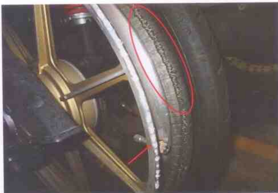
Photo 9 shows the rear tyre of the Motorcycle at the time of our inspection. We observed that the left sidewall of the rear tyre had burst (circled). The tread pattern of the rear tyre was clearly visible with remaining tread depth of approximately 5mm. The rear rim had sustained significant damage due to the burst left sidewall of the rear tyre (arrowed).
