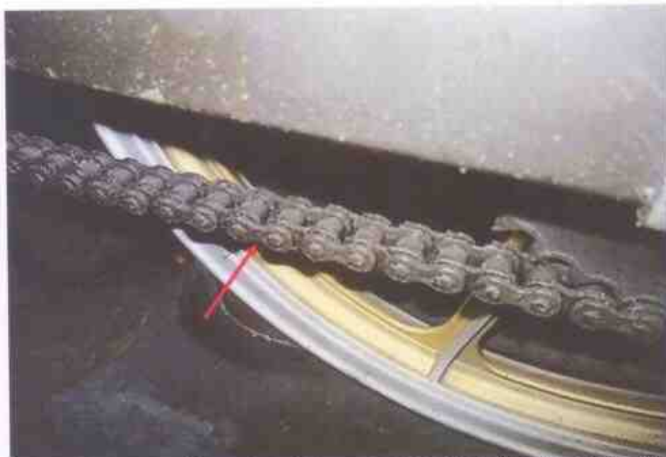
Photo 15 shows a closer view of the gear train (arrowed) of the Motorcycle, which was observed to be intact with no misalignment. It was also adequately lubricated for operating purposes.
