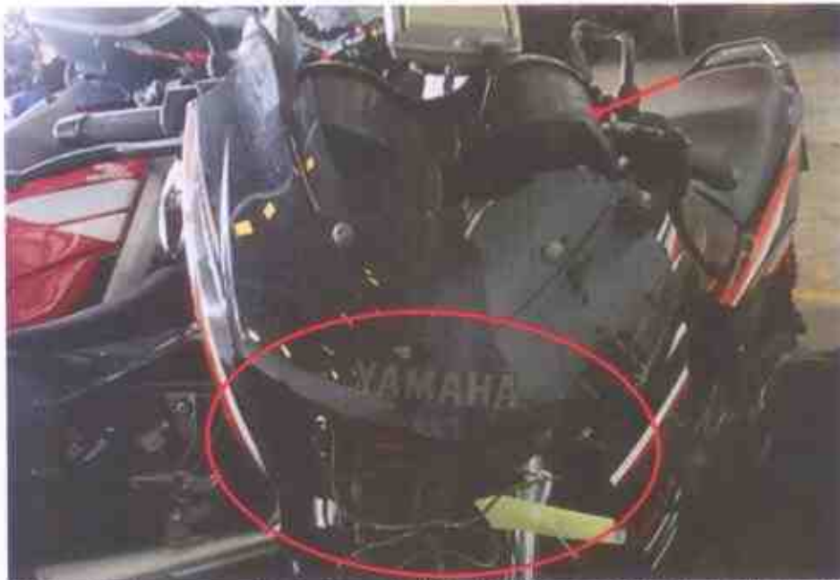
Photo 3 shows a closer view of the headlamp assembly (circled) and speedometer (arrowed) which were amongst the body parts at the front body of the Motorcycle that had sustained damage as a result of the accident.
