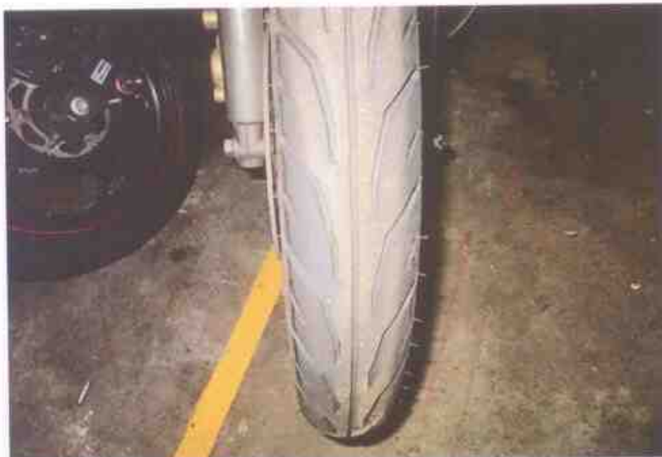
Photo 8 shows the front tyre of the Motorcycle at the time of our inspection. The front tyre was observed to be in serviceable condition. The pattern of the tread was also clearly visible. There was no tear, burst mark(s) and/or punctured hole(s) on the sidewalls as well as across the tread of the front tyre.
