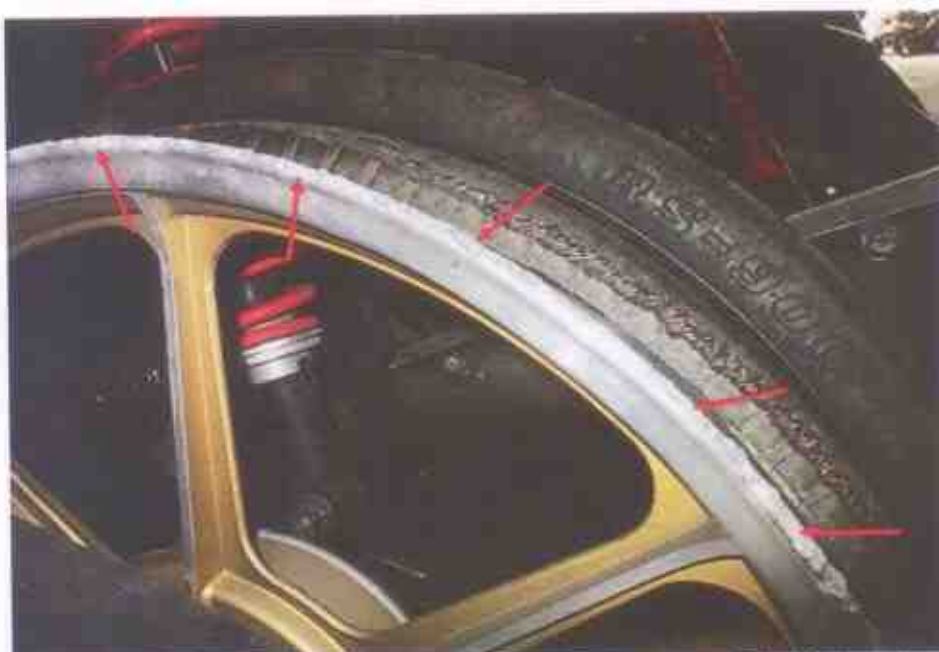
Photo 10 shows the left side of the rear wheel rim and tyre of the Motorcycle at the time of our inspection. Some relatively minor marks of grazing nature were observed on the edges of the rear wheel rim (arrowed).
