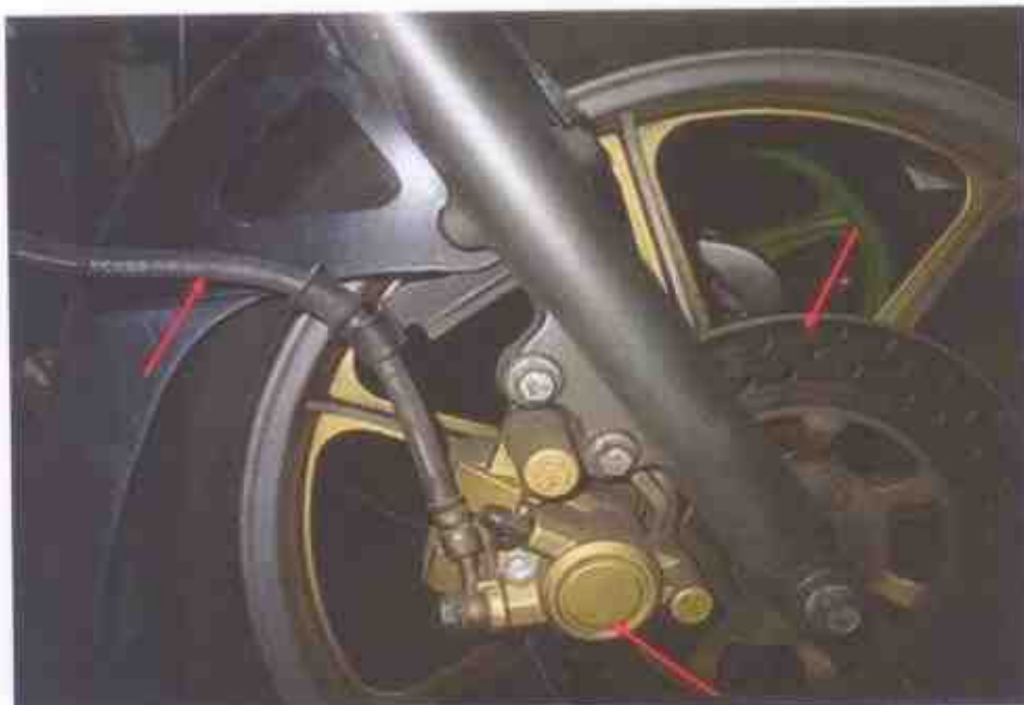
Photo 17 shows a close up view of the front brake caliper, front brake disc and front brake hose (arrowed) of the Motorcycle, which are all part of the components in the hydraulic front brake system of the Motorcycle. Our visual checks of these various components had revealed all to be intact with no visible damage. No leakage of brake fluid was also observed.
