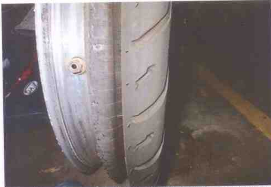
Photo 11 shows the condition of the Motorcycle's rear tyre. The tread pattern of the rear tyre was clearly visible with remaining tread depth of approximately 5mm.
