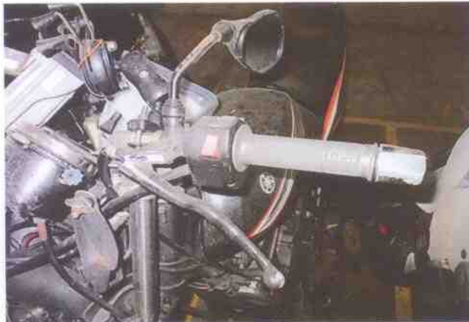
Photo 4 shows a close up view of the left side mirror, clutch lever and left handlebar end of the Motorcycle. These parts were amongst the body parts of the Motorcycle which were damaged as a result of the accident.
