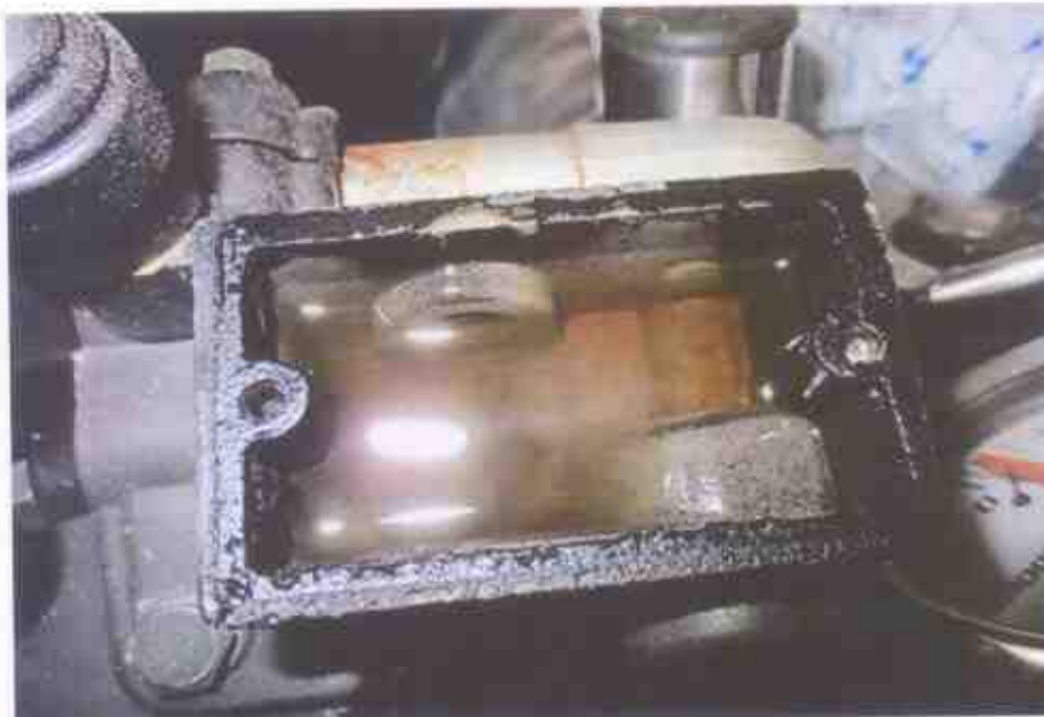
Photo 18 shows the brake fluid reservoir for the front brake of the Motorcycle. The brake fluid was observed to be of sufficient level and without contamination for operational purposes.
