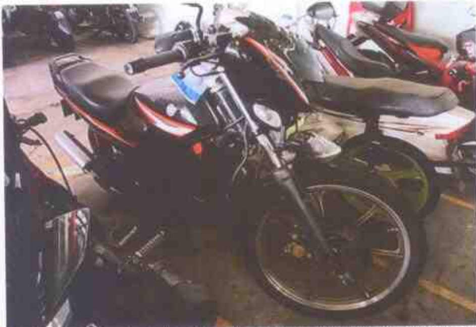
Photo 7 shows the front wheel rim and front tyre of the Motorcycle at the time of our inspection. The front tyre was observed to be in serviceable condition with remaining tread depth of approximately 5mm. The tyre was also observed to be sufficiently inflated for vehicular operation. There was no significant damage observed on the front wheel rim.
