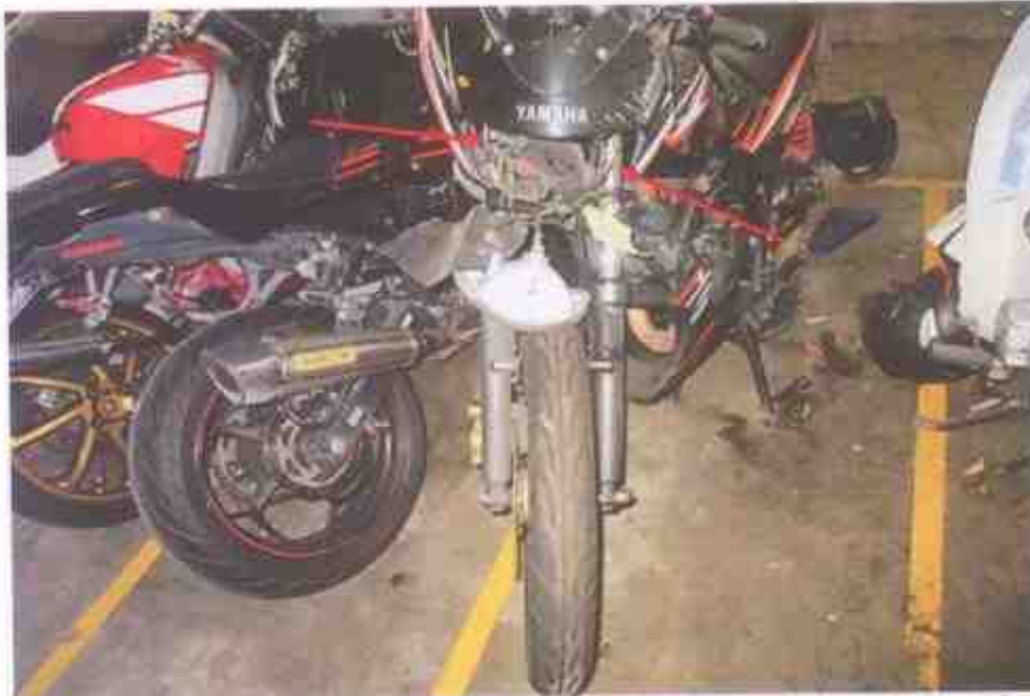
Photo 16 shows the front fork (arrowed) of the Motorcycle. The front fork and fork bracket of the Motorcycle were both found to be intact and undamaged. Turning the Motorcycle's handle bar towards the left and right did not produce any abnormal free play and/or resistance. The steering system of the Motorcycle was in serviceable condition at the time of our inspection.
