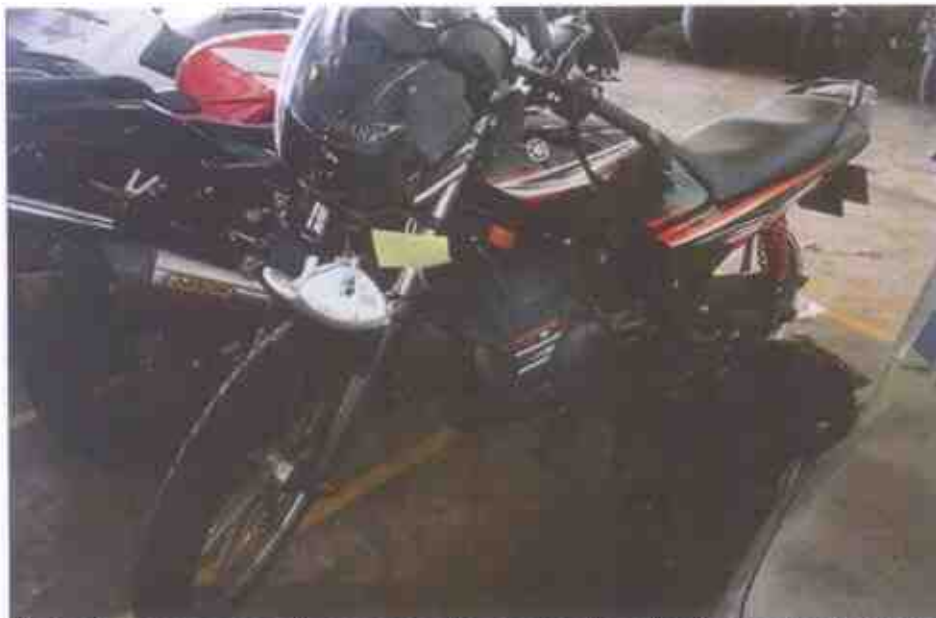
Photo 2 shows a general view of the left front body of the Motorcycle at the time of our inspection. The Motorcycle was observed to have sustained damages along its left side. Amongst the body parts that were found to have been damaged include its headlamp assembly, front left signal lamp, left side mirror, clutch lever, left handlebar end, front mudguard, gear shift rod, gear shift pedal, left front footrest, left front foot rest bracket, left rear side cover, rear wheel rim and rear tyre amongst others.
