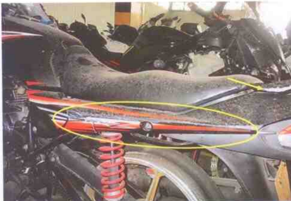
Photo 6 shows the damaged left rear side cover (circled) and pillion grab bar (arrowed) which were amongst the body parts of the Motorcycle that had sustained damage as a result of the accident.
