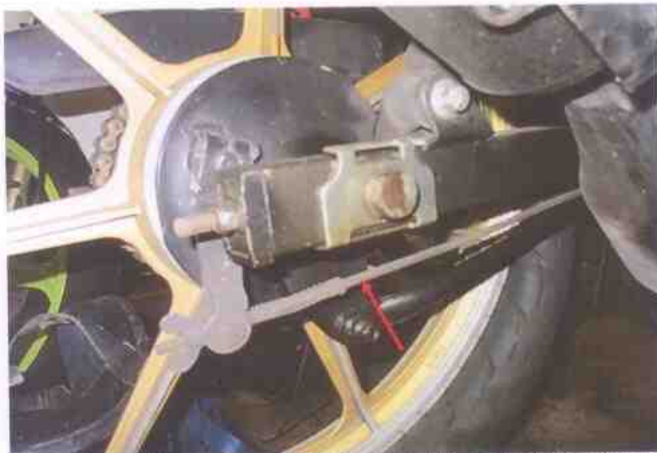
Photo 19 shows the rear wheel of the Motorcycle. The type of brake system for the rear wheel was of a mechanical type, controlled by the brake foot pedal of the Motorcycle. Our checks of the cable (arrowed), spring and drum which are all part of the components in the rear brake system of the Motorcycle reveal all to be intact and without damage.
