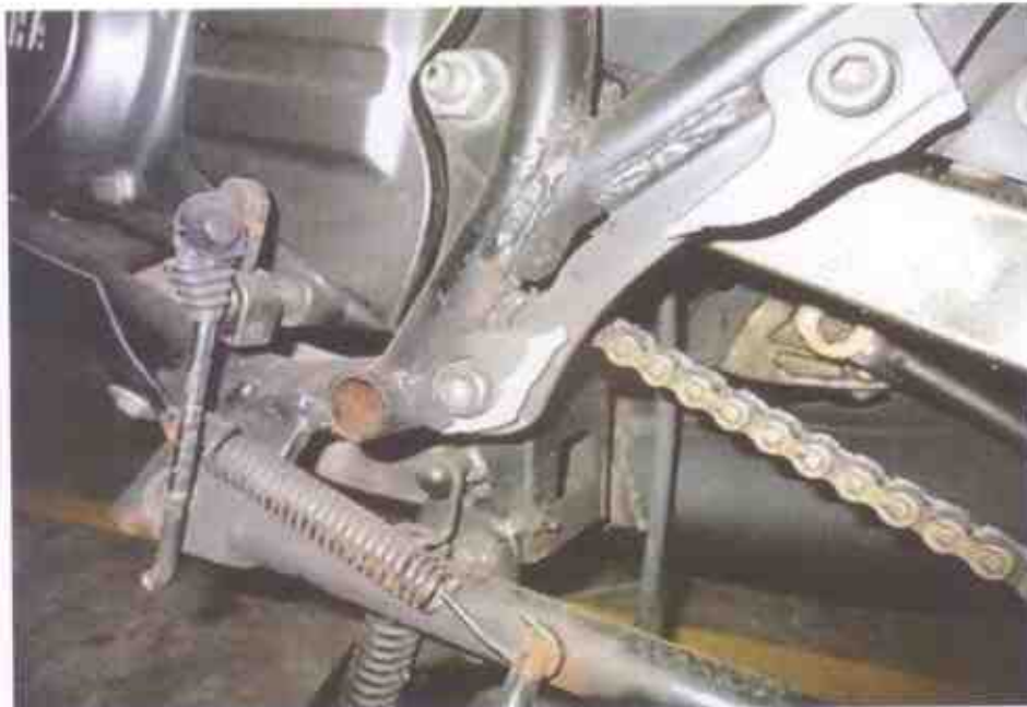
Photo 5 shows a closer view of the gear shift rod, gear shift pedal, left front footrest and left front footrest bracket, which were amongst the body parts of the Motorcycle that had sustained damage as a result of the accident.
