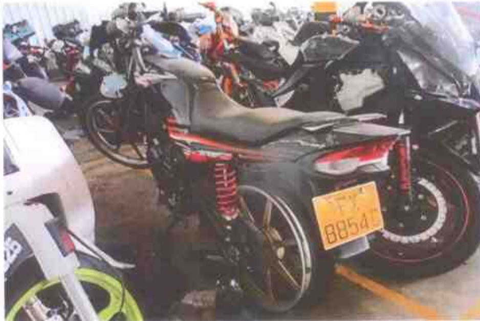
Photo 1 shows a general view of the left rear body of the Motorcycle at the time of our inspection. The Motorcycle was observed to have sustained damages along its left side. The mileage at the time of inspection was recorded to be 15,505km.
