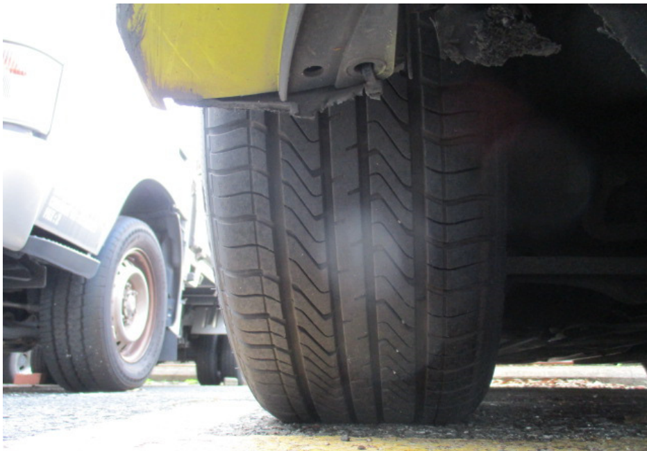
Photo 7 shows the condition of the front right tyre of the Motor Taxi, which was observed to be in serviceable condition with remaining tread depth of approximately 6mm. The tyre, which was wrapped around alloy wheel rim, was also observed to be sufficiently inflated for vehicular operation.
