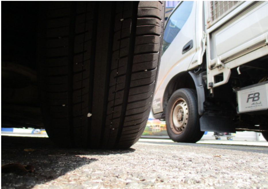
Photo 9 shows the condition of the rear right tyre of the Motor Taxi, which was observed to be in serviceable condition with remaining tread depth of approximately 7mm. There was also no tear, cut or burst mark(s) on the outer and the inner sidewalls as well as across the tread of the 4 tyres.
