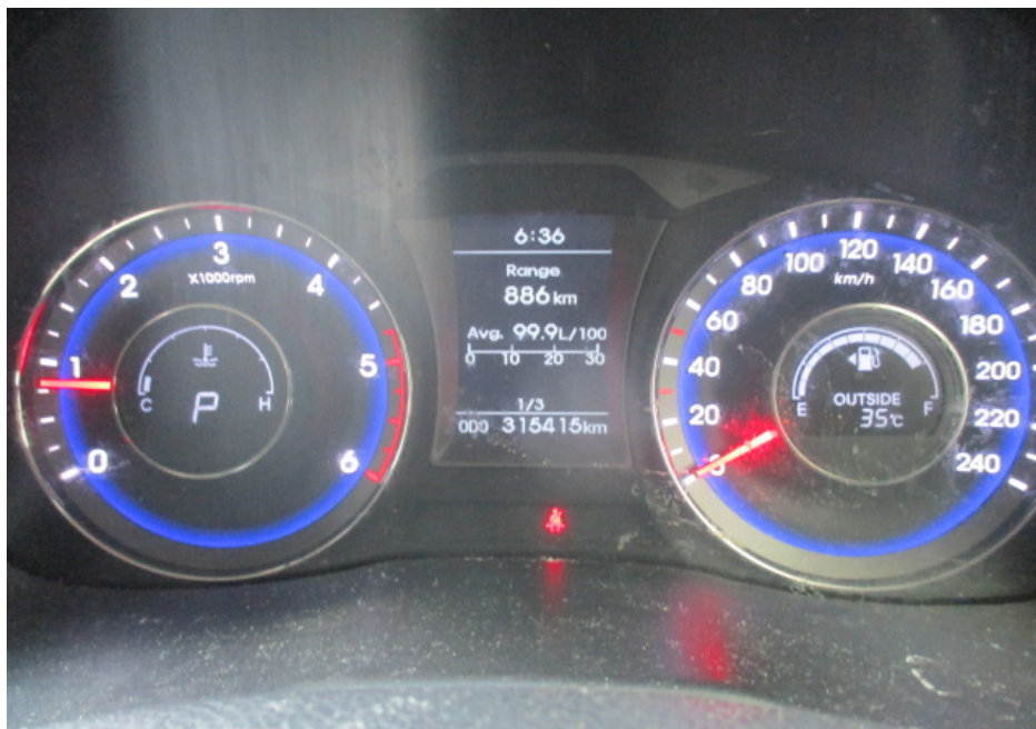
Photo 20 shows no warning lights illuminated on the instrument panel of the Motor Taxi after the engine was cranked. This would suggest that there was no abnormality to the various electronic operating systems of the Motor Taxi, like the EPS, ABS, ESC and SRS etc.
