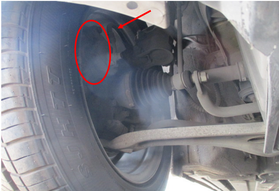
Photo 14 shows the brake hose/pipe (arrowed) at the front right wheel of the Motor Taxi. No leakage of brake fluid was observed. Visual examination of the various components of the braking system like the brake caliper (circled), brake pedal etc. had revealed all to be intact and without visible damage.
