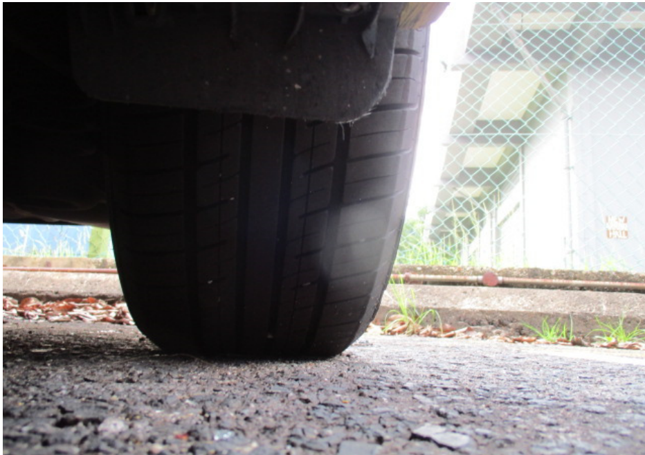
Photo 8 shows the condition of the rear left tyre of the Motor Taxi, which was observed to be in serviceable condition with remaining tread depth of approximately 7mm. The tyre, which was wrapped around alloy wheel rim, was also observed to be sufficiently inflated for vehicular operation. There was also no damage found on the 4 wheel rims of the Motor Taxi.
