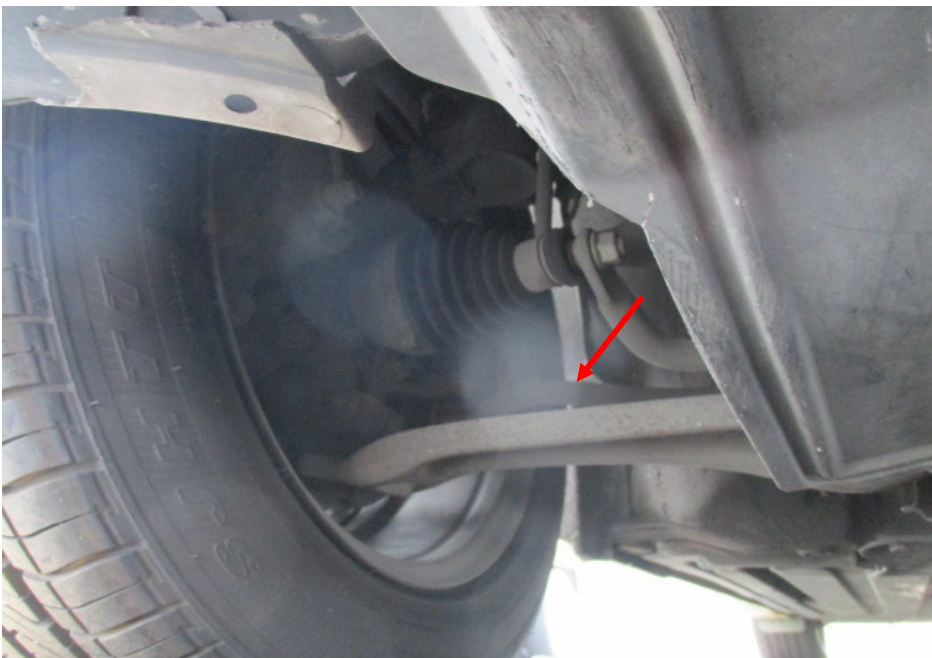
Photo 15 shows the various undercarriage components at the front right wheel of the Motor Taxi, in particular the steering tie rod (arrowed). The various steering components were all found to be intact, suggesting that the steering system of the Motor Taxi was likely to be in serviceable condition at the material time of accident. There was also no sign of fluid stain observed on the various undercarriage components at the front right wheel of the Motor Taxi.
