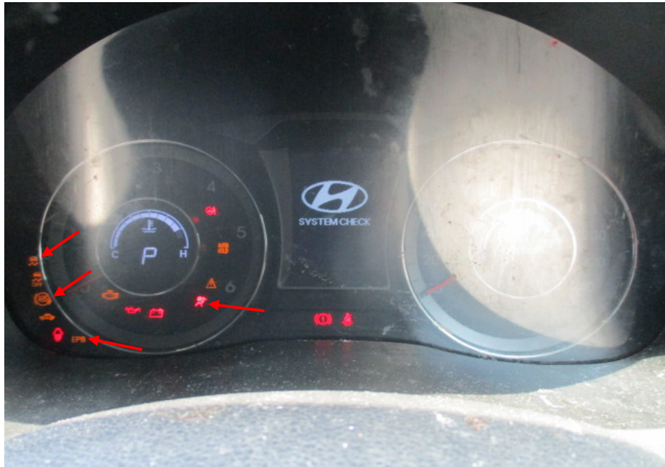
Photo 19 shows the warning lights for the various electronic operating systems of the Motor Taxi appearing on its instrument panel during the self-test when the engine is cranked, in particular the EPS light, ABS light, ESC light and SRS light (arrowed).
