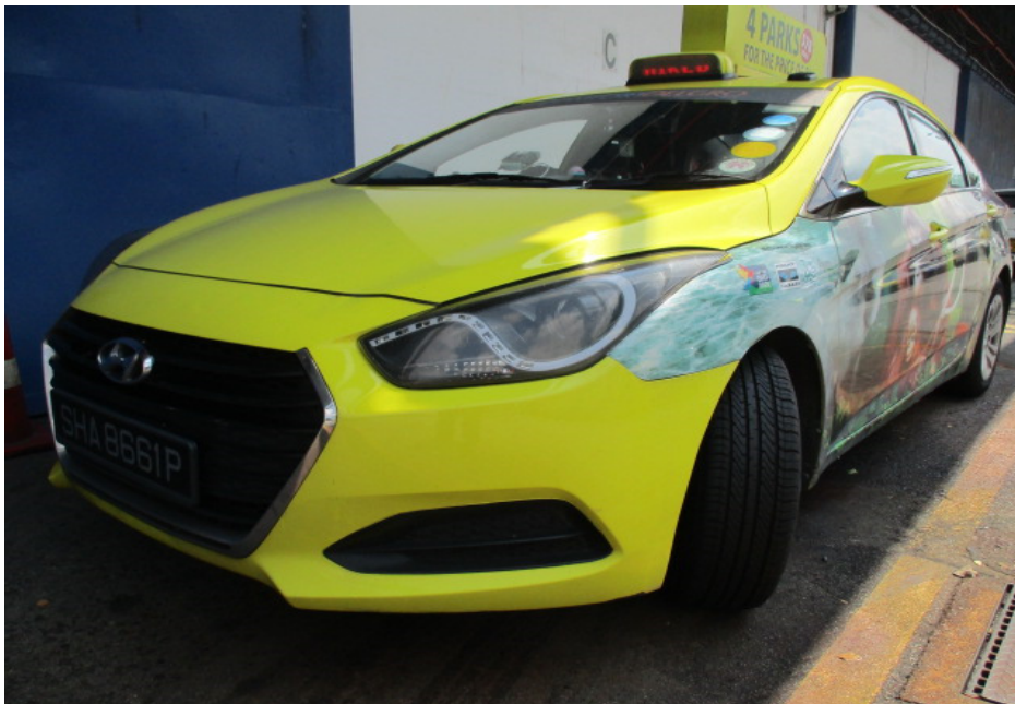
Photo 17 shows the front left wheel of the Motor Taxi turned to its full left. During our steering system test, we did not experience any abnormal free play and/or resistance when we had turned the steering wheel towards the left and right. This would suggest that the steering system of the Motor Taxi was likely to be in serviceable condition at the material time of accident.
