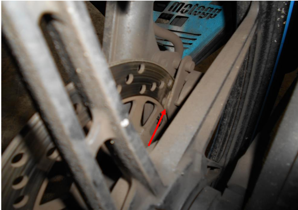
Photo 16 shows the front brake pad at time of our inspection. The frictional material was observed to be sufficient for operational purposes.
