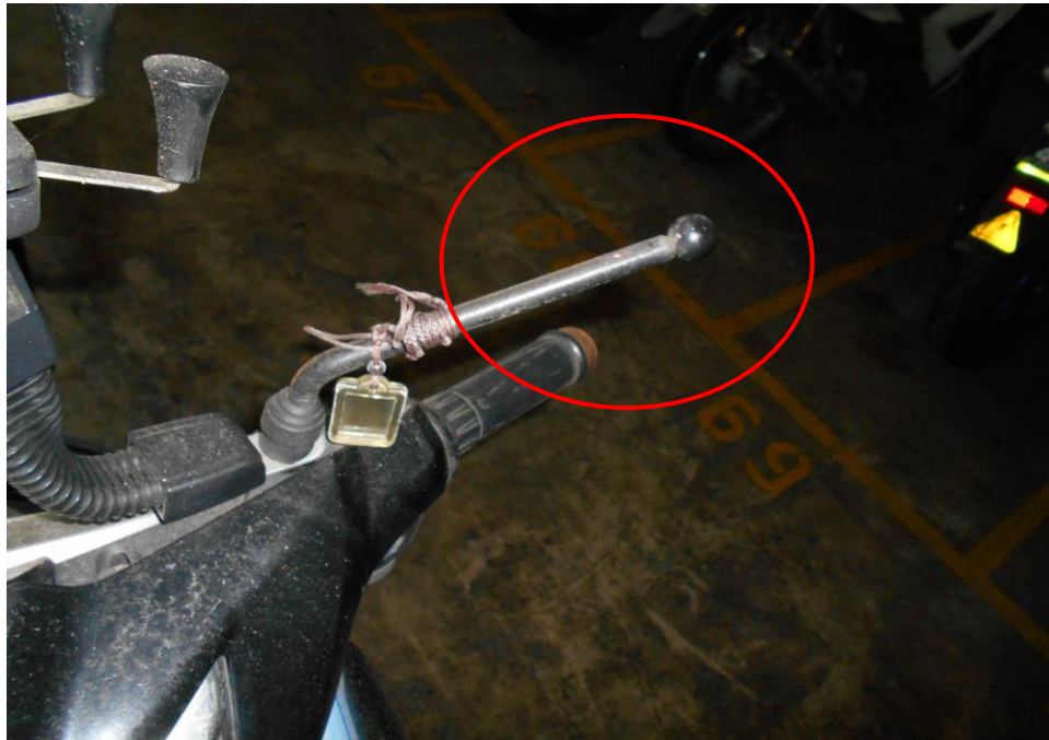
Photo 6 shows a closer view of the front left wing mirror of the Motorcycle at the time of our inspection. The Motorcycle wing mirror was observed to be dislodged due to the accident collision. (Circled)
