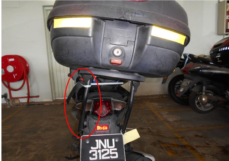
Photo 4 shows a general view of the rear body of the Motorcycle at the time of our inspection. The Motorcycle was observed to have sustained relatively minor damage on the compartment bracket at time of our inspection.
