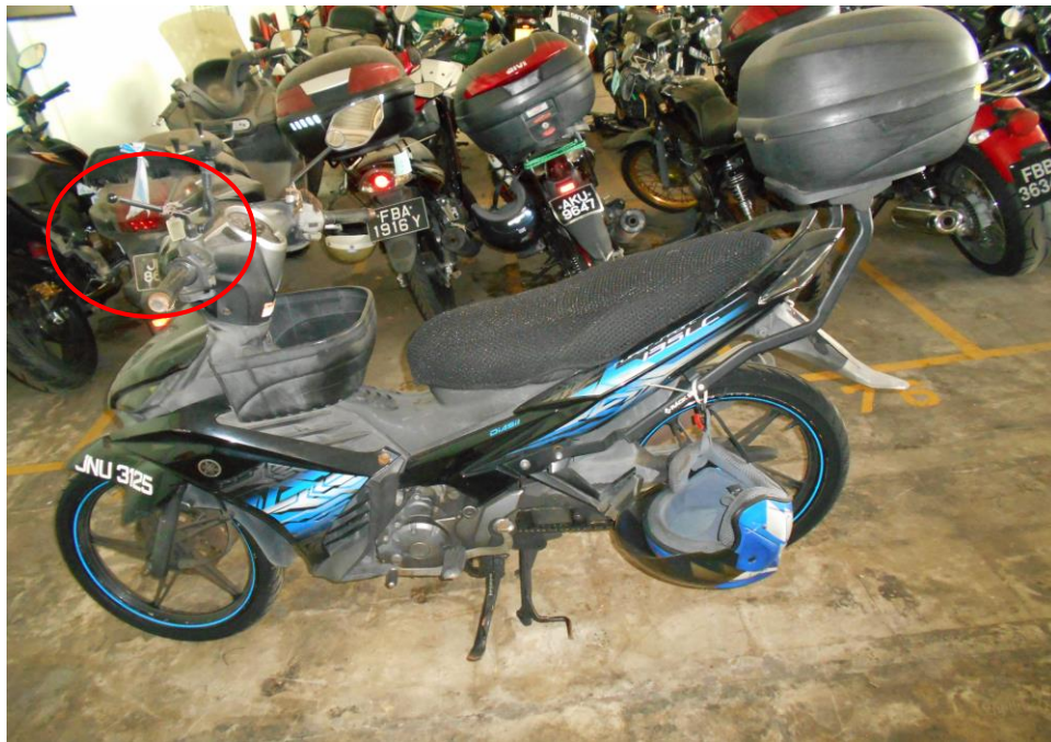
Photo 5 shows a general view of the left body of the Motorcycle at the time of our inspection. The damages were observed to be confined to its frontal & left side of the Motor Cycle at time of our inspection.
