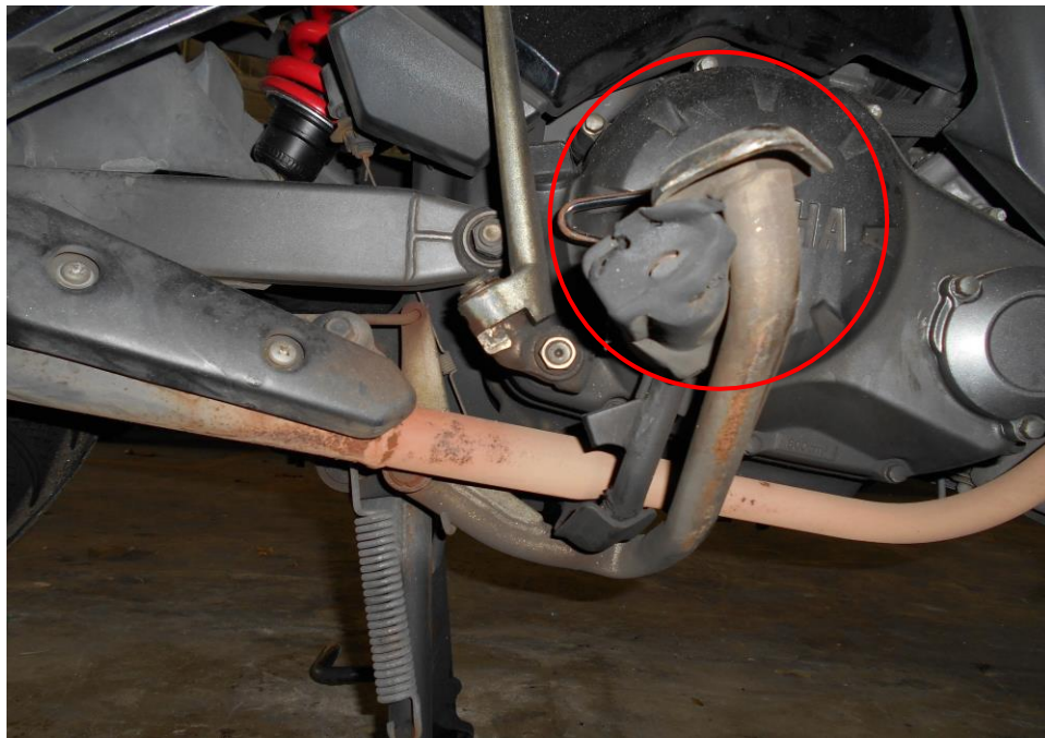
Photo 7 shows a closer view of the rear foot pedal of the Motorcycle at the time of our inspection. It was observed to be stuck to the foot pedal due to the accident collision. (Circled)
