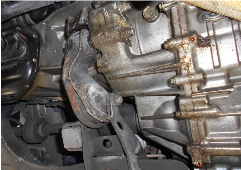
Photo 21 shows the close up view of the undercarriage fluid leakage affected by the accident's impact.
