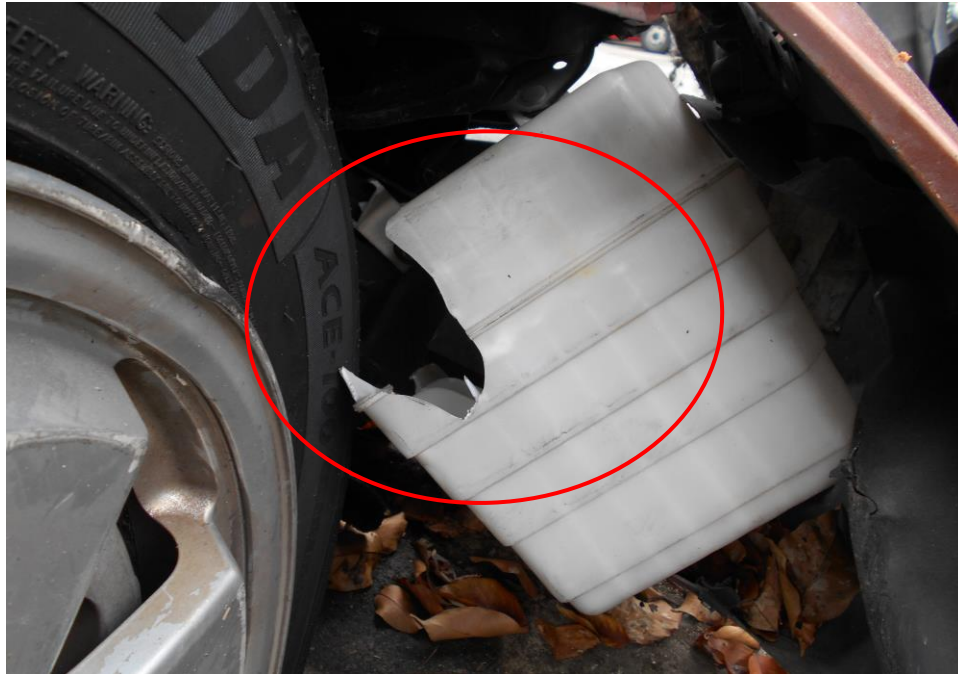
Photo 19 shows the close up view of the wiper washer container that was observed to be damaged (broken) by the accident's impact.
