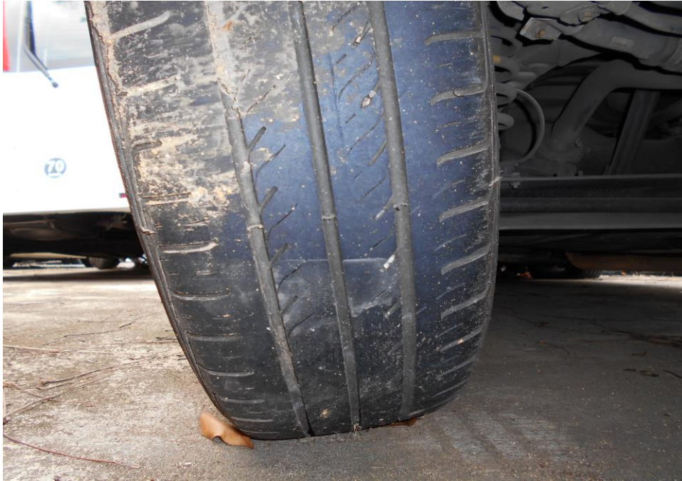
Photo 16 shows the condition of the rear left tyre of the Motor Taxi, which was observed to be in serviceable condition with remaining tread depth of approximately 5mm. There was also no tear, cut or burst mark(s) on the outer and the inner sidewalls as well as across the tread of this tyre.
