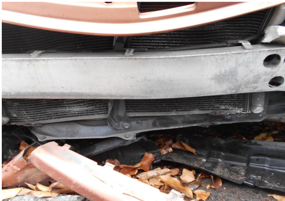
Photo 18 shows the close up view of the radiator tank that was affected by the accident's impact.
