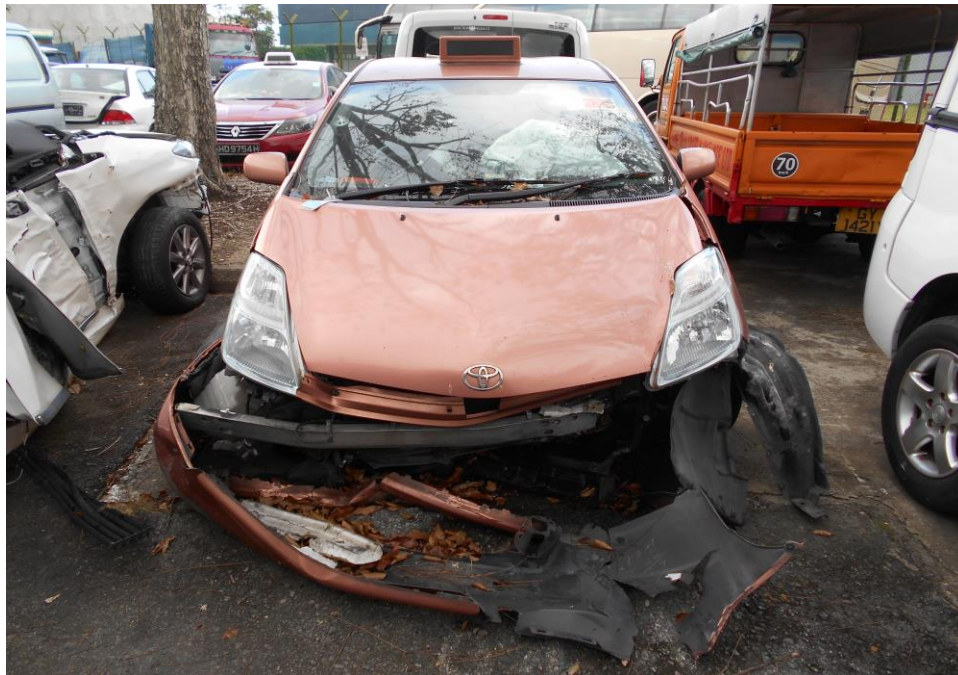
Photo 1 shows a general view of the frontal portion of the Motor Taxi at the time of our inspection. The Motor Taxi was observed to have sustained extensive impact damage at its frontal, left & right portion. The impact force was significant, causing the various parts and components to be damaged as a result of the accident.
