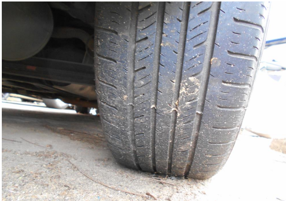
Photo 15 shows the condition of the rear right tyre of the Motor Taxi, which was observed to be in serviceable condition with remaining tread depth of approximately 6mm. There was also no tear, cut or burst mark(s) on the outer and the inner sidewalls as well as across the tread of this tyre.
