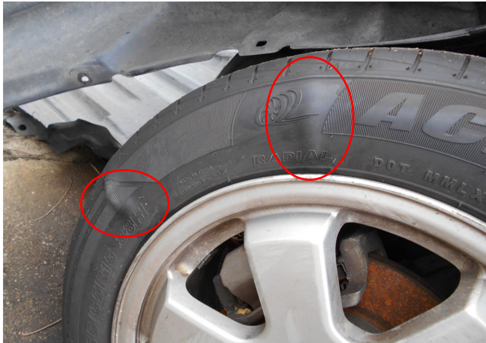
Photo 14 shows the condition of the front left tyre of the Motor Taxi, which was observed to be in serviceable condition with remaining tread depth of approximately 5mm. However, 2 small bloated marks were observed on the outer sidewall of the tyre likely due to the accident.
