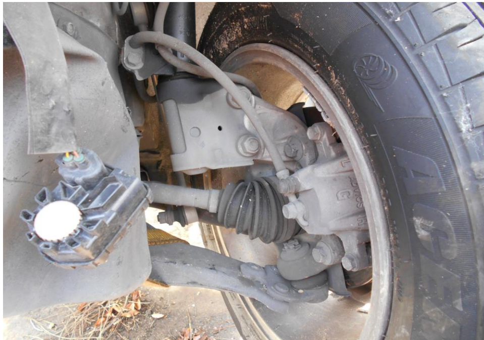
Photo 28 shows the Motor Taxi left wheel steering components which was found to be unaffected by the accident's impact.
