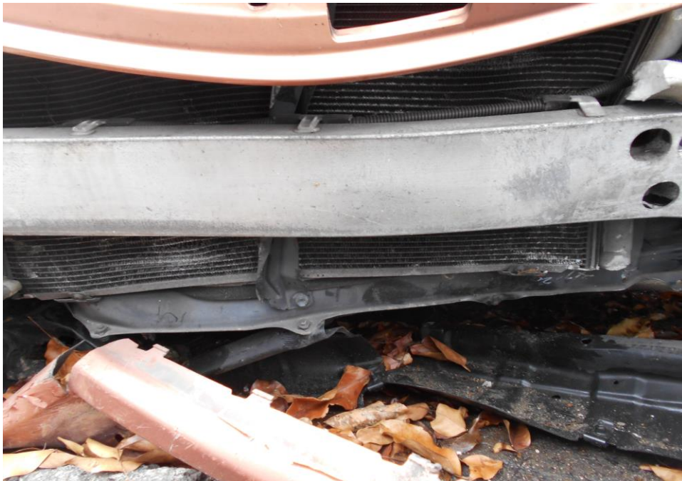
Photo 5 shows a closer view of the damaged radiator tank of the Motor Taxi. The impact force was significant, causing also other various parts and components inside the engine compartment to be damaged as a result of the accident.
