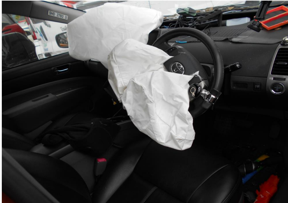
Photo 33 shows the Supplemental Restraint System (SRS) of the Motor Taxi was however likely to be in normal operating condition at the material time of the accident. The evidence of the deployed front driver & passenger's airbag indicates that the impact sensors and control module of the Motor Taxi's SRS were all in serviceable condition at the material time of accident.
