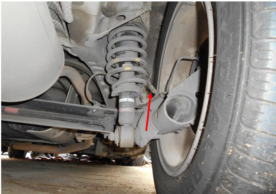
Photo 31 shows the braking components at the rear right wheel of the Motor Taxi. We did not observe any leakage of brake fluid at the time of our inspection of the Motor Taxi.
