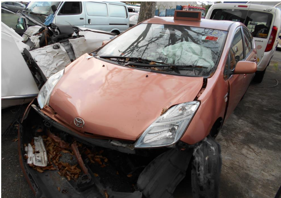
Photo 3 shows a general view of the front left portion of the Motor Taxi at the time of our inspection. The Motor Taxi was observed to have sustained minor impact damage at its front left portion.
