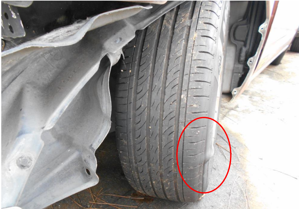
Photo 13 shows the condition of the front left tyre of the Motor Taxi, which was observed to be in serviceable condition with remaining tread depth of approximately 5mm. However, 2 small bloated marks were observed on the outer sidewall of the tyre likely due to the accident's impact.
