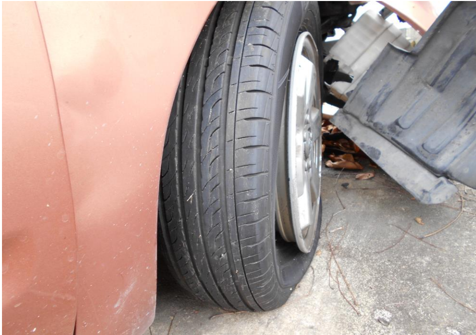
Photo 10 shows the condition of the front right tyre of the Motor Taxi, which was observed to be deflated (likely due to the accident) which might cause by dented alloy wheel rim.
