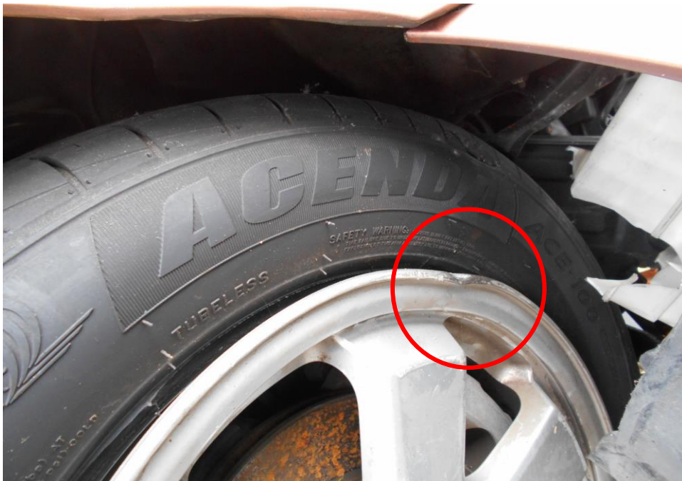
Photo 11 shows the condition of the dented front right wheel rim of the Motor Taxi as a result of the accident.
