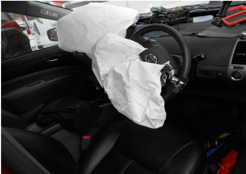
Photo 8 shows the interior portion of the Motor Taxi. The impact force triggered both driver & front passenger's airbag as a result of the accident.
