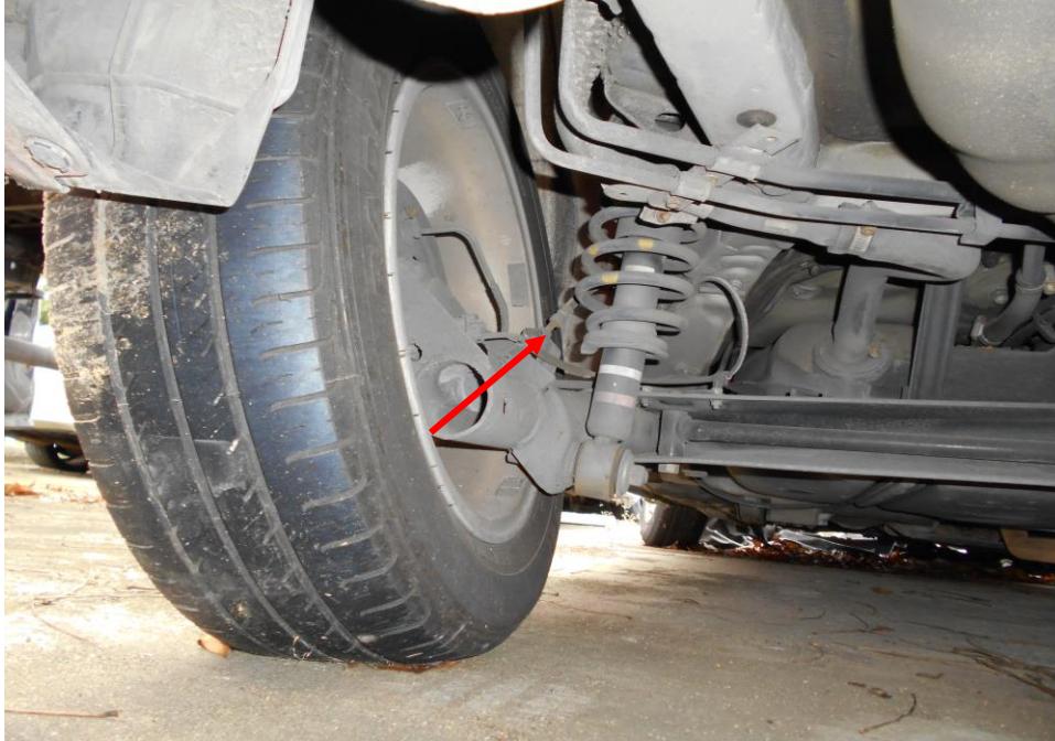
Photo 32 shows the braking components at the rear left wheel of the Motor Taxi. We did not observe any leakage of brake fluid at the time of our inspection of the Motor Taxi.
