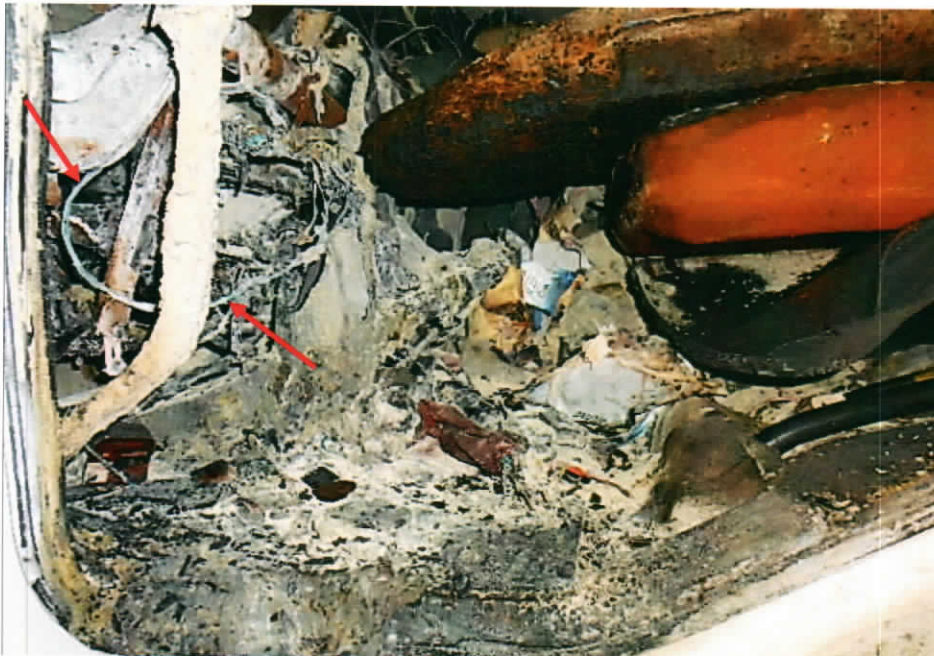
Photo 9 shows some original factory fitted wirings within the glove compartment with greenish residue (arrowed). The presence of greenish residue indicates internal heating of copper wires, a sign of an electrical short circuit occurring. The greenish residue is normally left behind from oxidation as a result of chemical reaction involving the copper wires.
