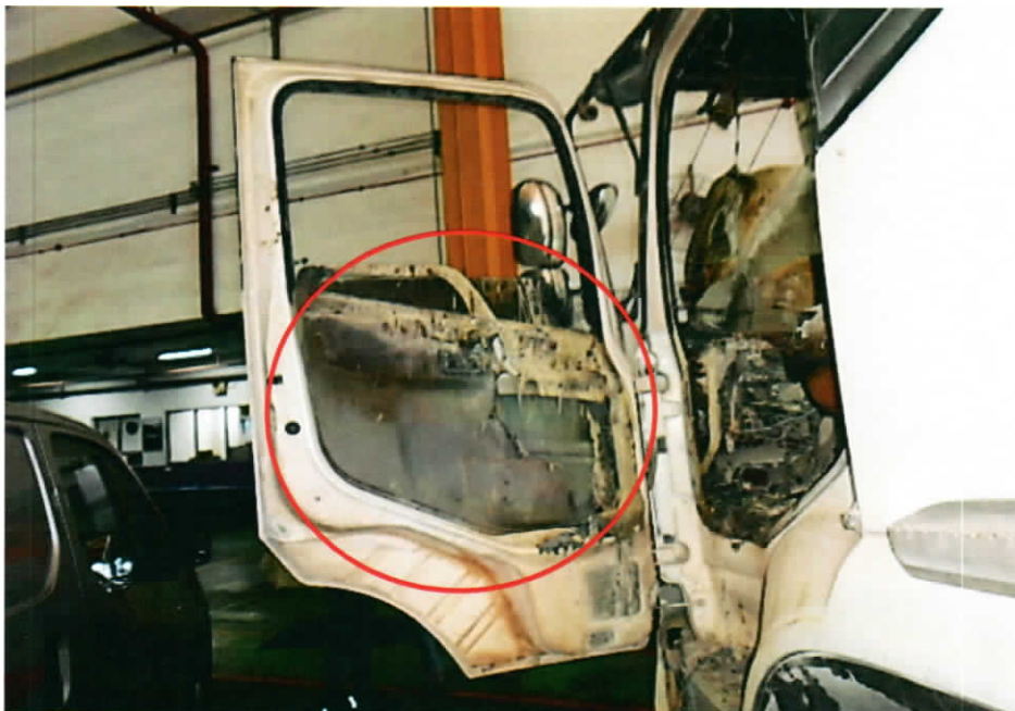
Photo 4 shows a closer view of the interior portion of the left passenger door of the Insured Vehicle at the time of our inspection. The left passenger door was observed to have sustained serious fire damage (circled).
