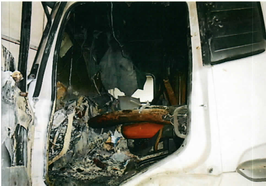
Photo 6 shows the interior compartment of the Insured Vehicle at the time of our inspection. Most of the components in the interior compartment were found to be burnt and/or melted as a result of the fire.
