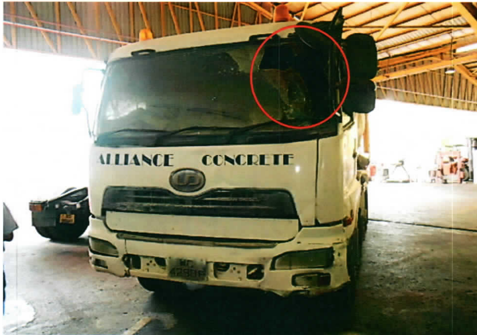
Photo 1 shows the front view of the Insured Vehicle at the time of our inspection. The fire damage to the Insured Vehicle was confined to its interior compartment. Most parts of the front portion were unaffected by the fire except for the front windscreen (circled).
