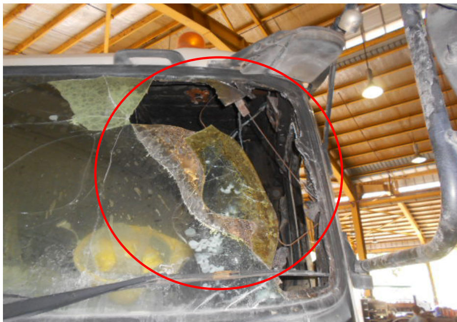
Photo 2 shows a close up view of the front windscreen of the Insured Vehicle. The left portion of the front windscreen seemed to have sustained serious fire damage (circled).
