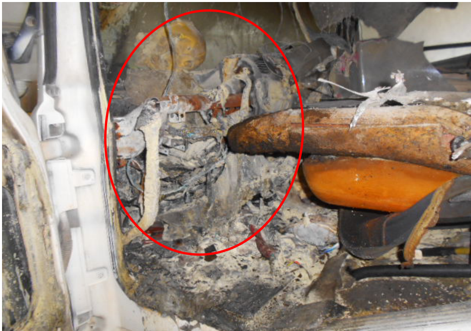
Photo 7 shows the dashboard instrument panel of the Insured Vehicle. The fire seemed to have originated from the left portion of the dashboard basing on the area where the extent of fire damage was most severe. Various components of the instrument panel were observed to have been burnt and/or partly melted from prolonged exposure to high heat intensity which included the glove compartment, upper and central parts of the instrument panel assembly (circled).
