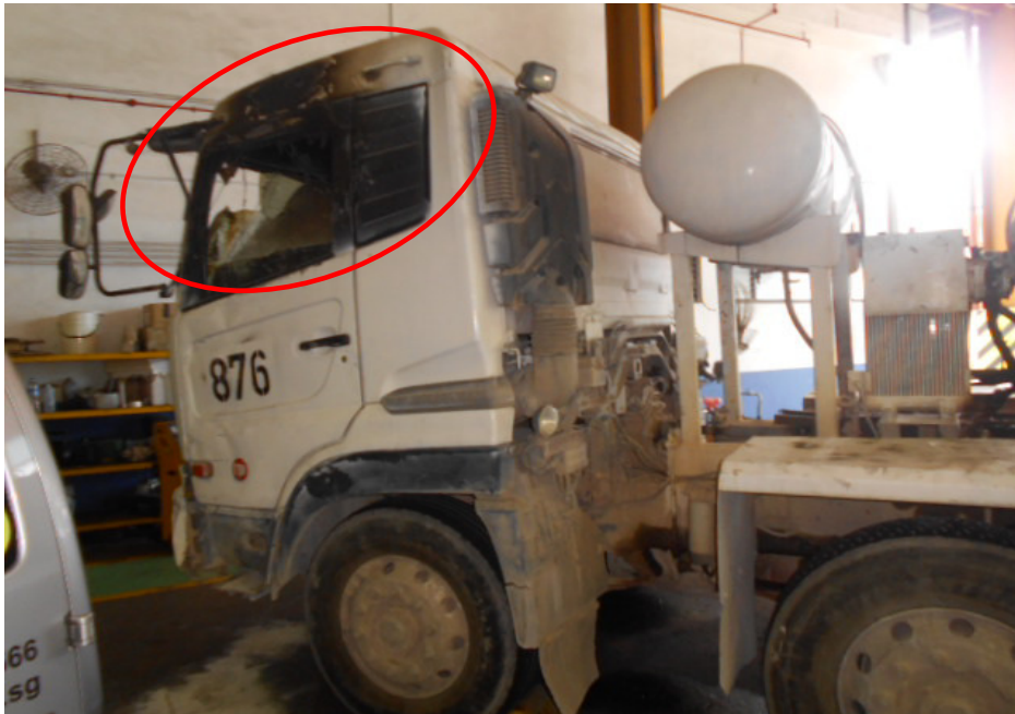
Photo 3 shows the left side view of the Insured Vehicle at the time of our inspection. The fire damage to the Insured Vehicle was confined to its interior compartment. The left side was observed to have been unaffected by the fire except for the left passenger door window (circled).
