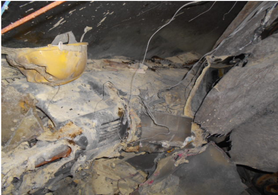
Photo 8 shows a closer view of the centre portion of the instrument panel. Various components of the instrument panel were observed to have been burnt and/or partly melted from prolonged exposure to high heat intensity which included the glove compartment, upper and central parts of the instrument panel assembly.
