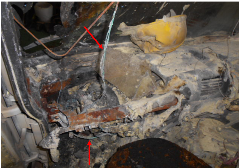
Photo 10 shows a closer view of the original factory fitted wirings within the glove compartment with greenish residue (arrowed). The presence of such greenish residue suggests occurrence of an electrical short circuit.
