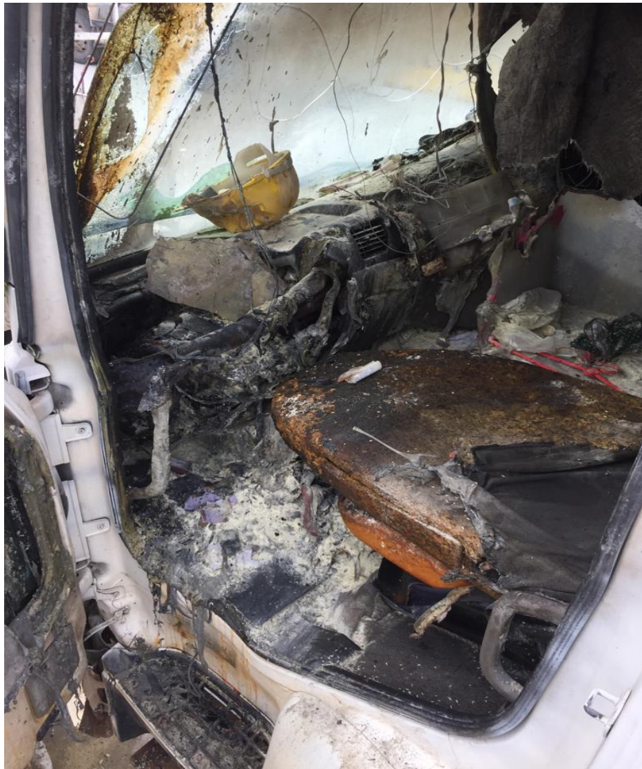
Photo 12 shows the interior compartment of the Insured Vehicle after the fire was extinguished. In general, the extensive damages sustained to the left portion of the dashboard had corresponded to the events that were related to us by Mr Siva, which is the fire started from the left portion of the interior compartment of the Insured Vehicle.
