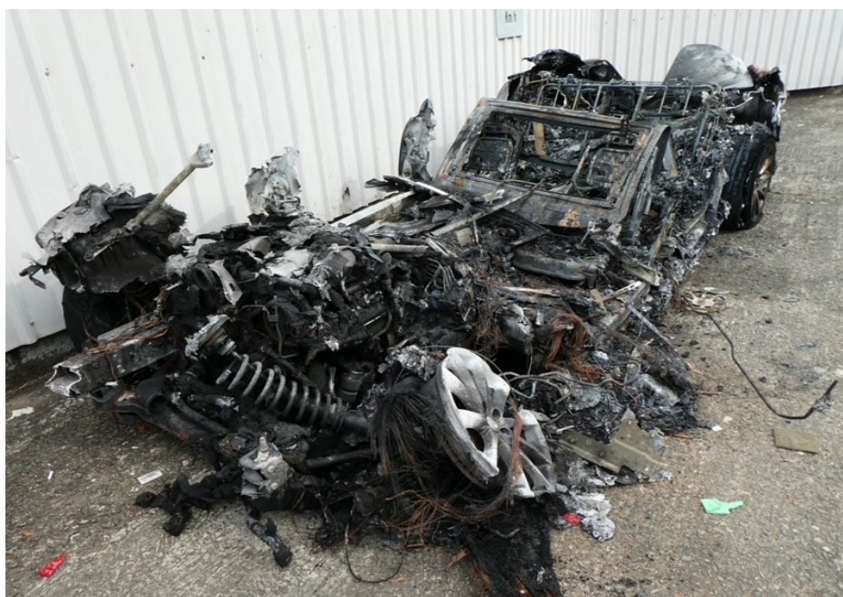
Photo 2 shows a general view of the front portion of the Insured Vehicle at the time of my inspection. Its front portion and centre portion were burned to char leaving skeletal remains.
