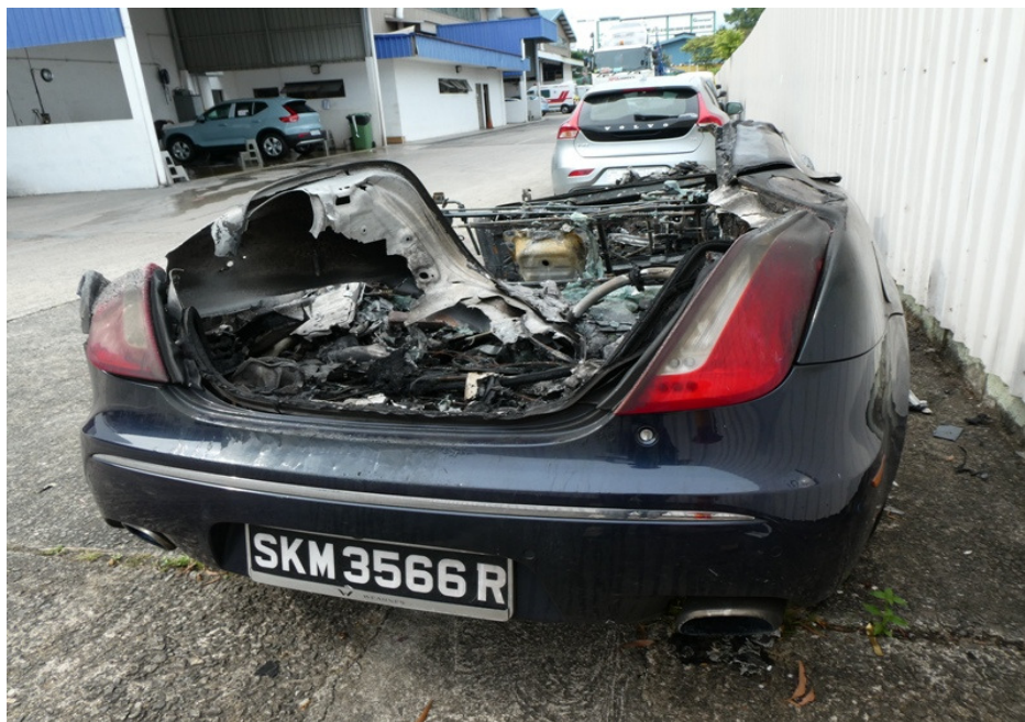
Photo 1 shows a general view of the rear portion of the Insured Vehicle at the time of my inspection. The Insured Vehicle was observed to have been extensively burnt. Its rear bumper was the only part that was relatively unaffected by the fire.
