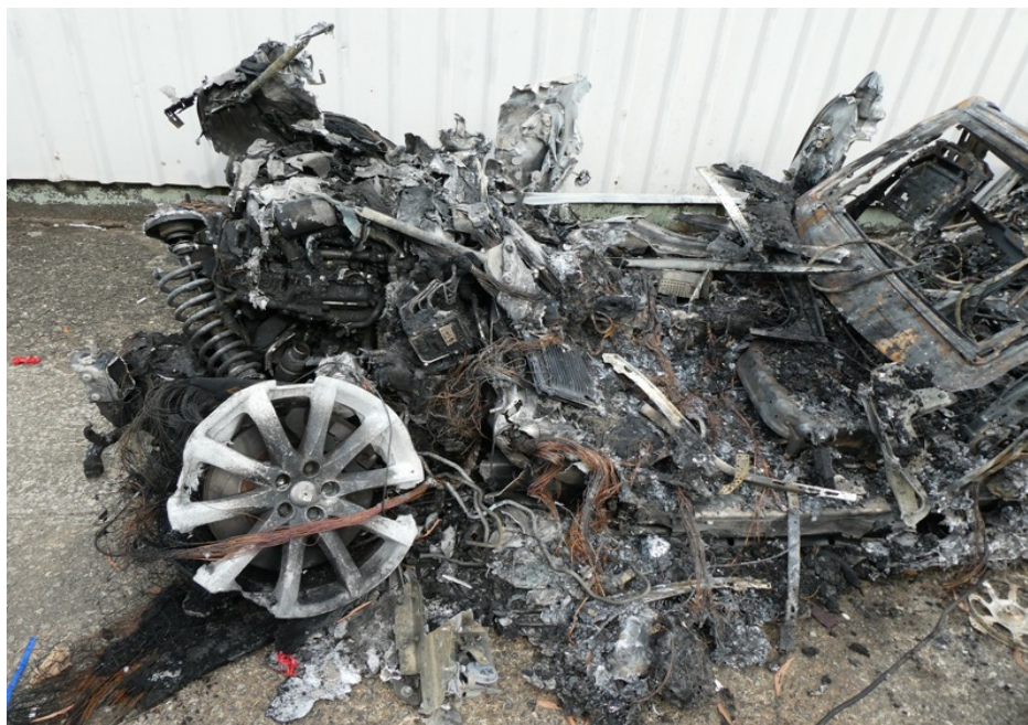
Photo 3 shows a general view of the front portion of the Insured Vehicle at the time of my inspection. Its front portion and centre portion were burned to char leaving skeletal remains.
