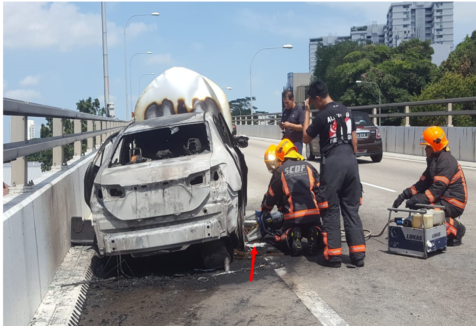
Photo 16 shows the Insured Vehicle at the incident location after the fire was extinguished by SCDF personnel. Firefighters can be seen using a hydraulic winch to remove the remnants of the burnt mattress that was stuck under the rear exhaust muffler of the Insured Vehicle (arrowed). The extent of damage and burn pattern to the Insured Vehicle was observed to be similar to what we had observed during our physical inspection of the Insured Vehicle.
