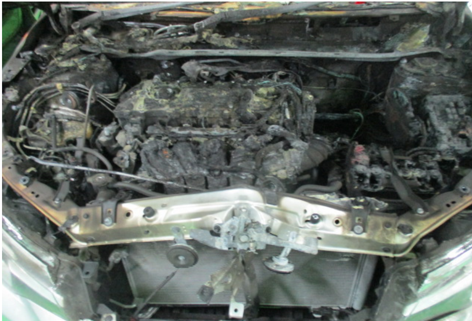
Photo 7 shows the engine compartment of the Insured Vehicle at the time of our inspection. The entire engine compartment of the Insured Vehicle was observed to be severely burnt. Most of the parts inside the engine compartment were found to be burnt and/or melted as a result of the fire.
