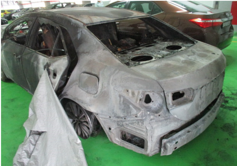
Photo 5 shows the general view of the rear left body of the Insured Vehicle at the time of our inspection. The Insured Vehicle was observed to have sustained extensive fire damage all around. Rust had accumulated all over the rear and centre portion of the Insured Vehicle as a result of exposure to environmental condition for a period of time.
