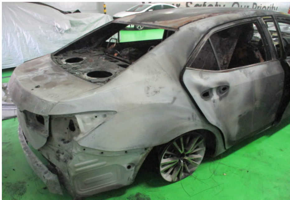
Photo 4 shows the general view of the rear right body of the Insured Vehicle at the time of our inspection. The Insured Vehicle was observed to have sustained extensive fire damage all around. Rust had accumulated all over the rear and centre portion of the Insured Vehicle as a result of exposure to environmental condition for a period of time.
