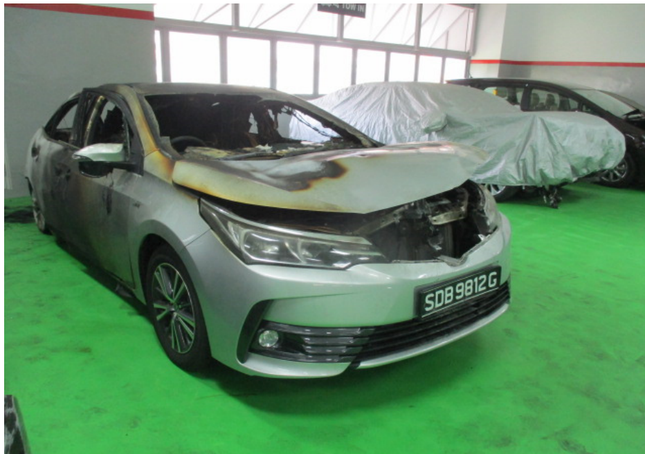
Photo 3 shows the general view of the right body of the Insured Vehicle at the time of our inspection. The Insured Vehicle was observed to have sustained extensive fire damage all around. Rust had accumulated all over the rear and centre portion of the Insured Vehicle as a result of exposure to environmental condition for a period of time.
