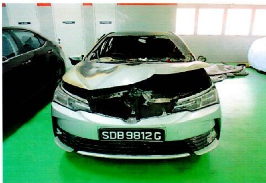
Photo 1 shows the general view of the front portion of the Insured Vehicle at the time of our inspection. The Insured Vehicle was observed to have sustained extensive fire damage all around. Its engine compartment and interior compartment were completely burnt. Rust had accumulated all over the rear and centre portion of the Insured Vehicle as a result of exposure to environmental condition for a period of time.
