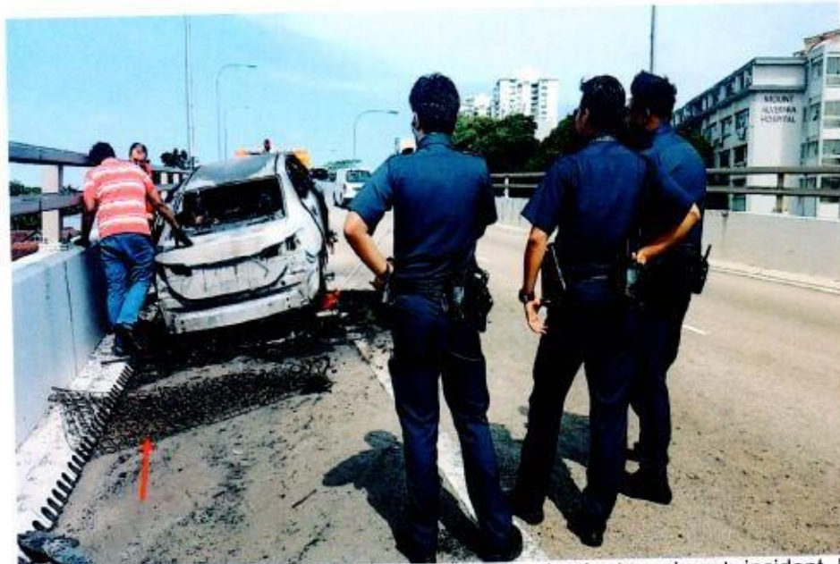
Photo 17 shows the Insured Vehicle being prepped to be towed post-incident. In general, the information that could be gathered from this photograph had corresponded to the events that were related to us by Mr Cheng, which is the fire was caused by the mattress (arrowed) that was stuck under the rear exhaust muffler of the Insured Vehicle.
