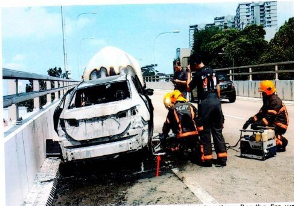
Photo 16 shows the Insured Vehicle at the incident location after the fire was extinguished by SCDF personnel. Firefighters can be seen using a hydraulic winch to remove the remnants of the burnt mattress that was stuck under the rear exhaust muffler of the Insured Vehicle (arrowed). The extent of damage and burn pattern to the Insured Vehicle was observed to be similar to what we had observed during our physical inspection of the Insured Vehicle.
