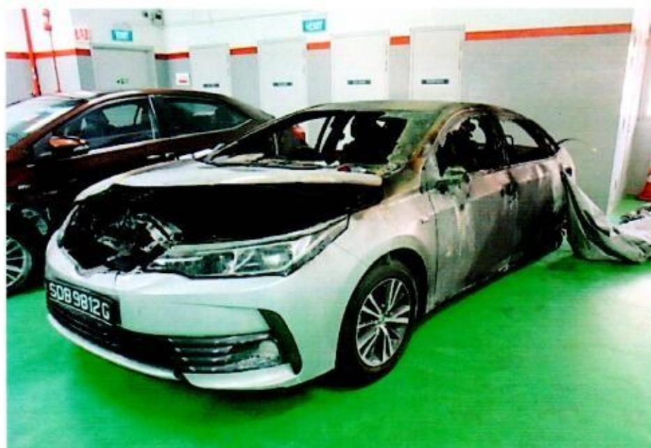
Photo 2 shows the general view of the left body of the Insured Vehicle at the time of our inspection. The Insured Vehicle was observed to have sustained extensive fire damage all around. Rust had accumulated all over the rear and centre portion of the Insured Vehicle as a result of exposure to environmental condition for a period of time.
