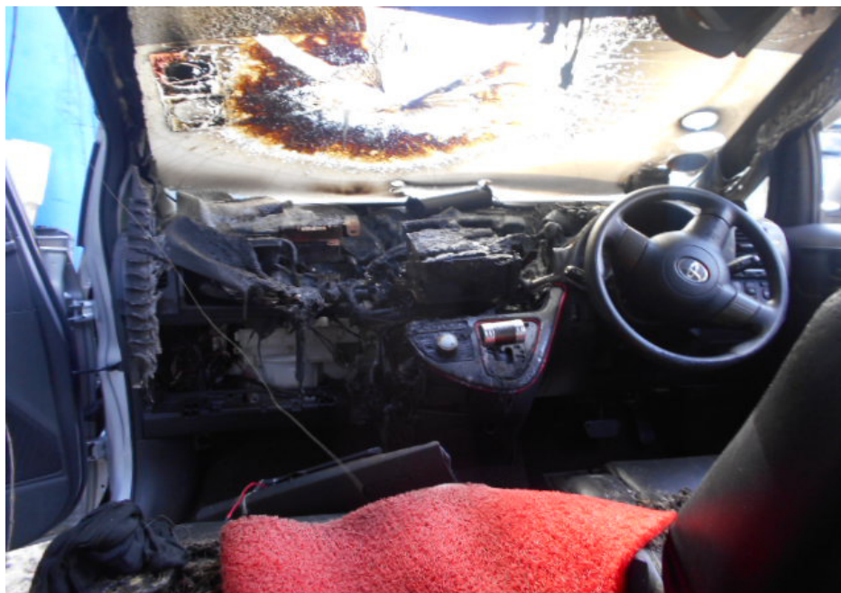
Photo 5 shows a general view of the interior compartment of the Insured Vehicle. The fire damage to the Insured Vehicle was confined to mainly the front area of its interior compartment. The front dashboard, seats, upholstery, carpets and various plastic trims amongst others were observed to have been partially melted/burnt.
