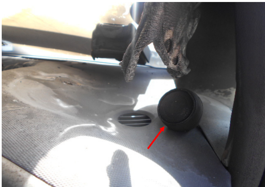
Photo 7 shows the audio speaker (arrowed) that was found to be additionally fitted near the right side "A" pillar trim of the Insured Vehicle. The same audio speaker fitted near the left side "A" pillar trim was observed to be partially melted/burnt as a result of the fire.
