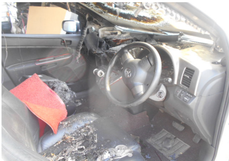
Photo 4 shows a general view of the interior compartment of the Insured Vehicle. The fire damage to the Insured Vehicle was confined to mainly the front area of its interior compartment. The front dashboard, seats, upholstery, carpets and various plastic trims amongst others were observed to have been partially melted/burnt.
