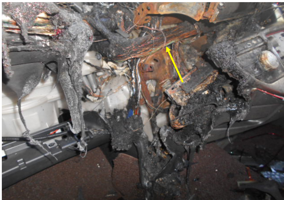
Photo 13 shows the burnt wirings that were with greenish colour residue (arrowed). This was at the area behind the centre of the front dashboard, behind and slightly below the location of the stereo. The presence of greenish residue indicates internal heating of copper wires, a sign of an electrical short circuit occurring. The greenish residue is normally left behind from oxidation as a result of chemical reaction involving the copper wires. This physical evidence would then appear to indicate that the cause of fire to the Insured Vehicle was due to electrical nature.
