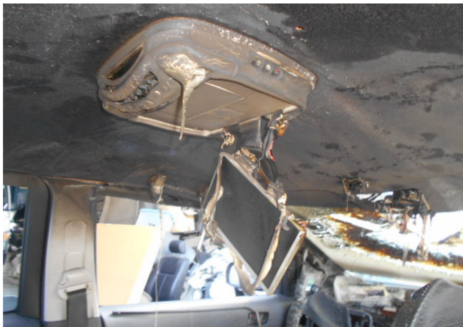
Photo 8 shows the media screen that was additionally fitted on the roof of the Insured Vehicle. The media screen was observed to be partially melted/burnt as a result of the fire.
