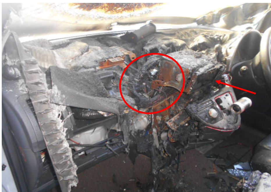
Photo 12 shows the interior compartment of the Insured Vehicle. Basing on the information gathered during the course of my investigations, and the physical damage to the Insured Vehicle, the fire had originated at the area (circled) behind the centre of the front dashboard. This was also behind and slightly below the location where the stereo (arrowed) is located.
