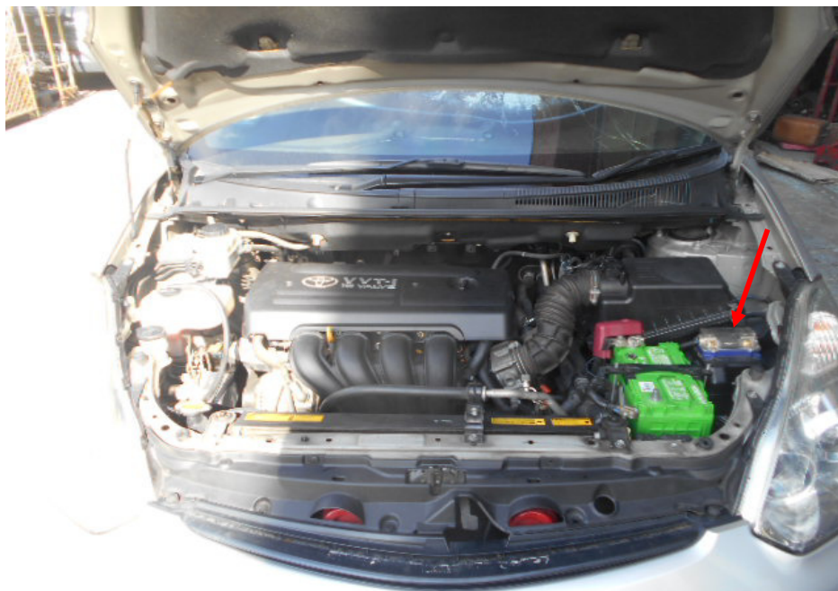
Photo 3 shows the engine compartment of the Insured Vehicle at the time of my inspection. There was no damage of burn nature observed within the engine compartment. A high ampere fuse (arrowed) was observed to be additionally fitted inside the engine compartment.
