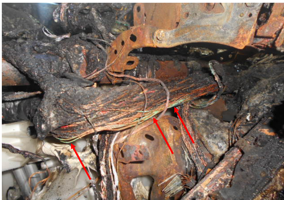
Photo 14 shows a closer view of the burnt wiring that were with greenish colour residue (arrowed). The presence of greenish residue indicates internal heating of copper wires, a sign of an electrical short circuit occurring.
