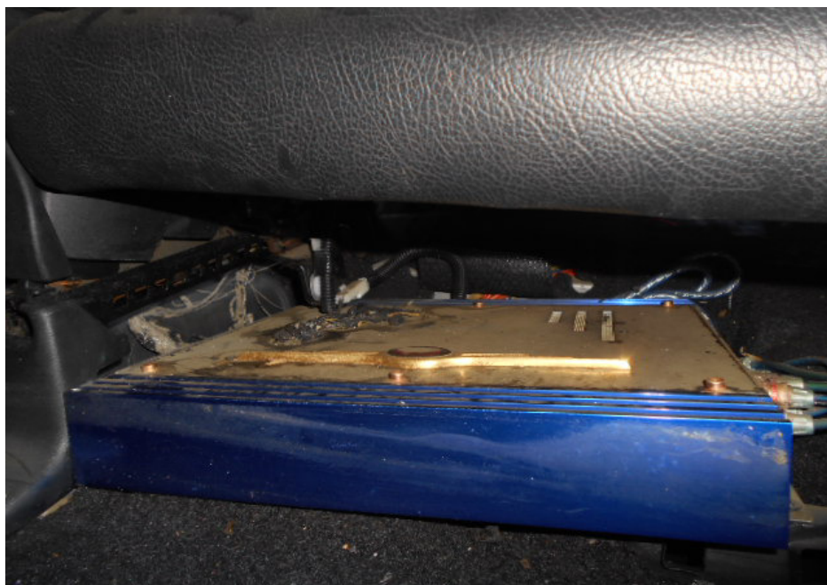
Photo 6 shows the audio amplifier that was found to be additionally fitted under the front left passenger seat of the Insured Vehicle. The audio amplifier and the connecting wire cables were found to be without any burnt marks.
