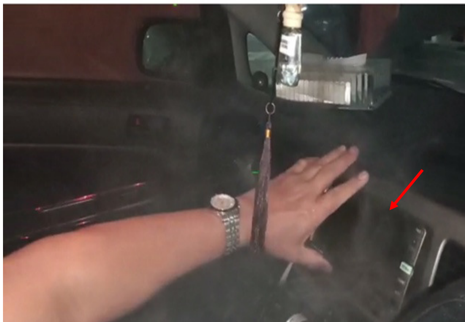
Photo 10 shows smoke in the interior compartment of the Insured Vehicle before the fire. From the video recordings, the smoke appear to be emitting from the area where the stereo (arrowed) is fitted.
