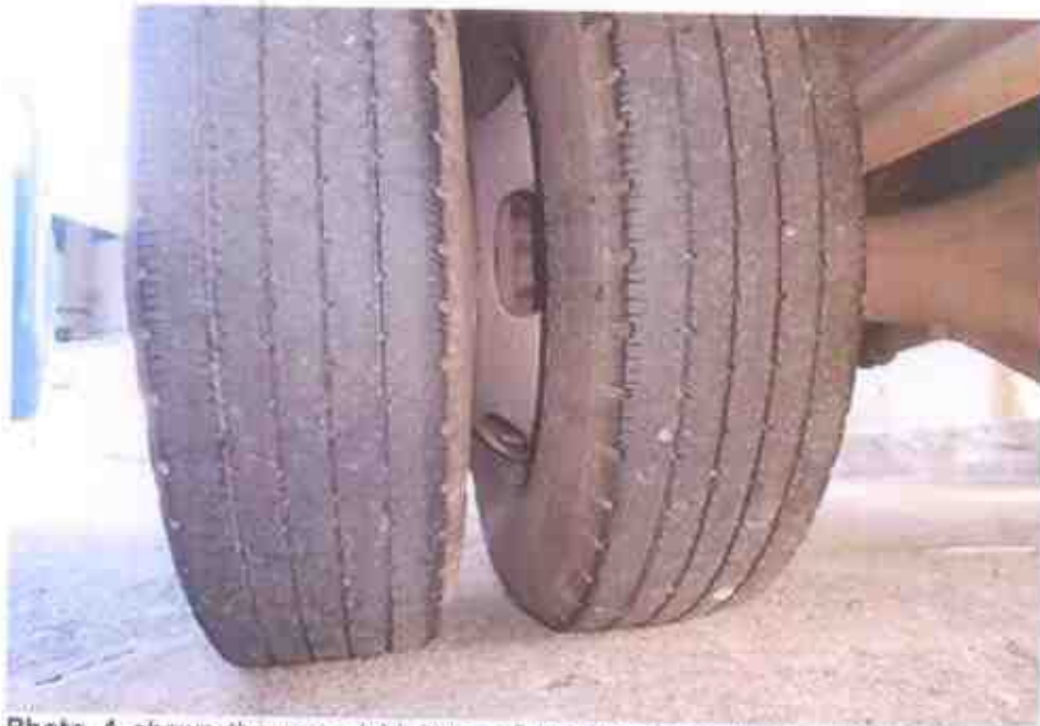
Photo 4 shows the rear right tyres of the insured vehicle at the time of my inspection. The pattern of the tread of both rear right tyres were observed to be still visible. Both these tyres were found to be sufficiently inflated for vehicular operation and without any tear, cut or burst mark(s) on the outer and the inner sidewalls as well as across the tread. The remaining tread depth of the 2 rear right tyres were measured to be approximately 2mm to 3mm each.
