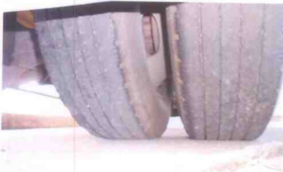
Photo 4 shows the rear right tyres of the insured vehicle at the time of my inspection. The pattern of the tread of both rear right tyres were observed to be still visible. Both these tyres were found to be sufficiently inflated for vehicular operation and without any tear, cut or burst mark(s) on the outer and the inner sidewalls as well as across the tread. The remaining tread depth of the 2 rear right tyres were measured to be approximately 2mm to 3mm each.
