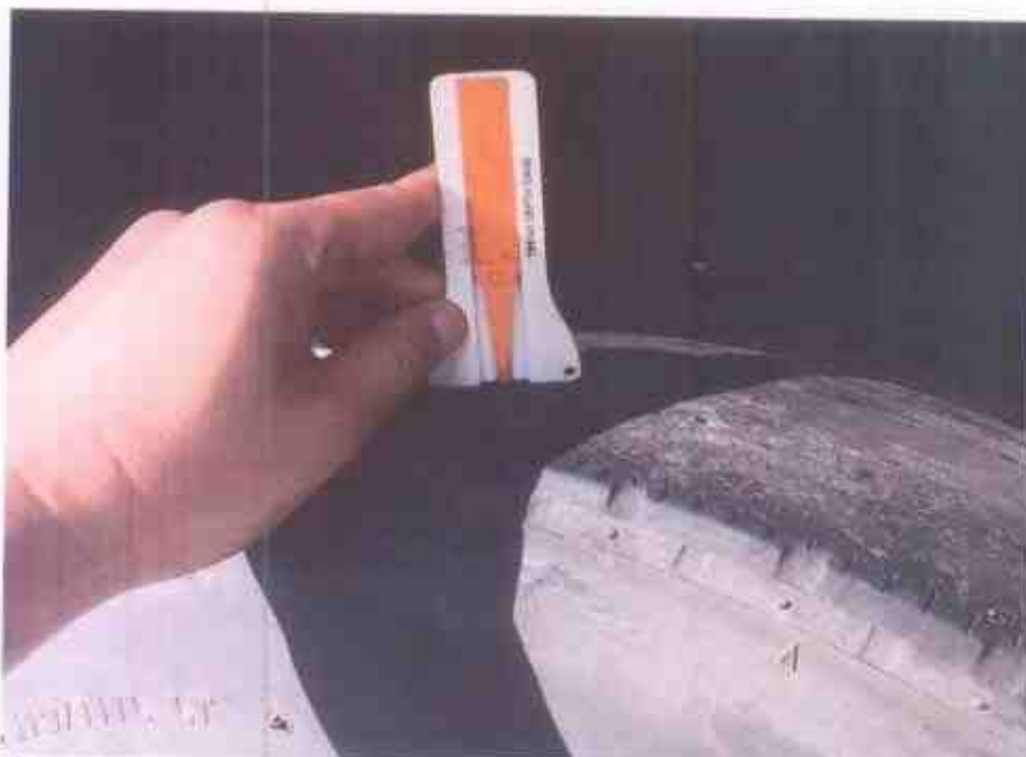
Photo 8 shows measurement being carried out to the remaining tread depth of the insured vehicle's rear left tyres.
