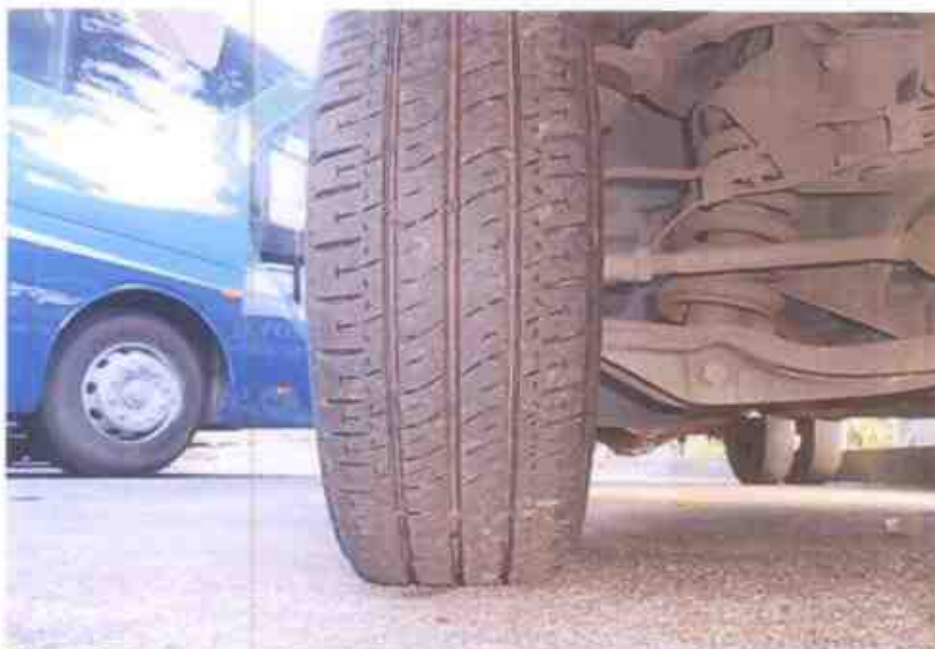
Photo 3 shows the condition of the front right tyre of the insured vehicle, which was observed to be in serviceable condition with remaining tread depth of approximately 7mm. The front right tyre was also observed to be sufficiently inflated for vehicular operation with no tear, cut or burst mark(s) on its outer and inner sidewalls, as well as across its tread.
