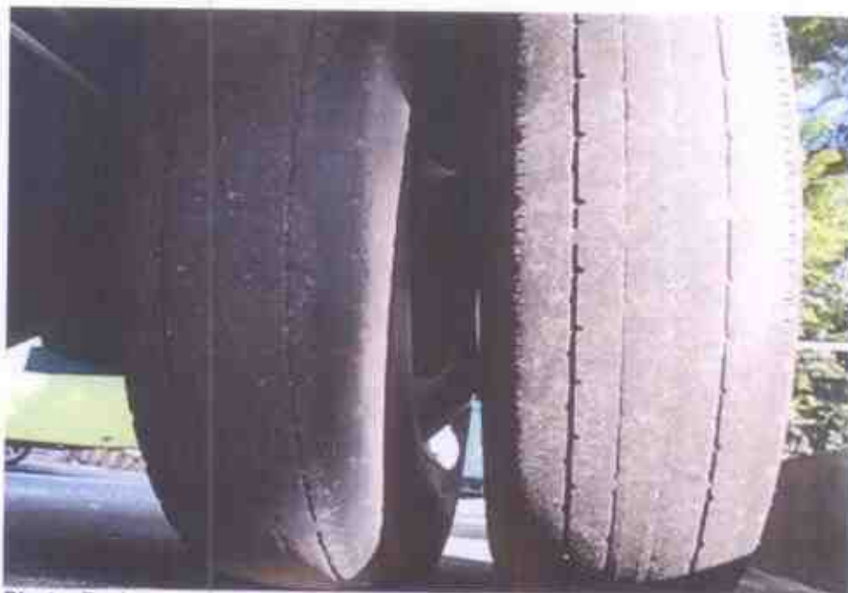
Photo 7 shows the rear left tyres of the insured vehicle at the time of my inspection. The pattern of the tread at the centre area of both rear left tyres were observed to be no longer visible while the pattern of the tread at the outer areas were barely visible. The non-visible tread pattern was due to the rubber wearing off. Both these tyres were found to be sufficiently inflated for vehicular operation and without any tear, cut or burst mark(s) on the outer and the inner sidewalls as well as across the tread.
