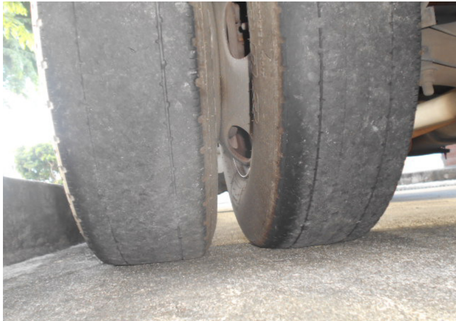
Photo 6 shows the rear left tyres of the insured vehicle at the time of my inspection. The pattern of the tread at the centre area of both rear left tyres were observed to be no longer visible while the pattern of the tread at the outer areas were barely visible. The non-visible tread pattern was due to the rubber wearing off. Both these tyres were found to be sufficiently inflated for vehicular operation and without any tear, cut or burst mark(s) on the outer and the inner sidewalls as well as across the tread.
