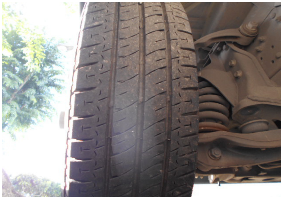
Photo 2 shows the condition of the front left tyre of the insured vehicle, which was observed to be in serviceable condition with remaining tread depth of approximately 7mm. It was also found to be sufficiently inflated for vehicular operation and without any tear, cut or burst mark(s) on the outer and the inner sidewalls as well as across the tread.
