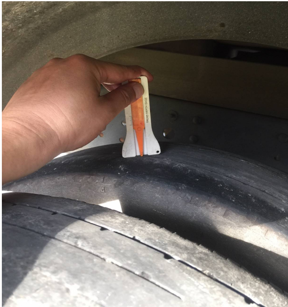
Photo 10 shows the measurement of the remaining depth of the tread pattern at the outer area of the inner rear left tyre. The measurement had indicated slightly above 0mm. In general, measurements of the outer areas of the insured vehicle's rear left tyres, where the pattern of the tread was still barely visible reveal remaining tread depth of approximately slightly above 0mm to below 1mm.
