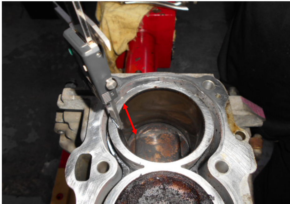
Photo 18 shows measurement being carried out to the stroke (arrowed) of cylinder 4 of the Toyota engine. The bore and stroke measurements of the Toyota engine were carried out using a digital Vernier Caliper that was calibrated prior to the start of measurements.
