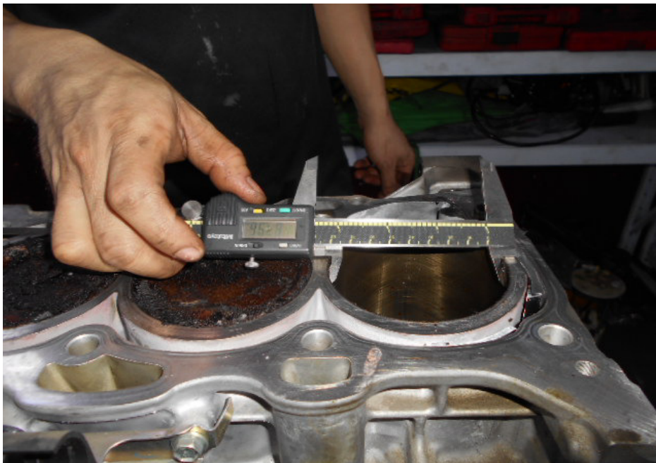
Photo 6 shows measurement being carried out to the bore of cylinder 1 of the Toyota engine. The measurements were carried out using a digital Vernier Caliper that was calibrated before the start of the measurements.
