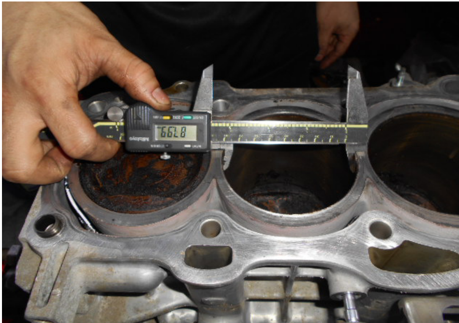
Photo 13 shows measurement being carried out to the bore of cylinder 3 of the Toyota engine. The bore and stroke measurements of the Toyota engine were carried out using a digital Vernier Caliper that was calibrated before the start of measurements. The bore measurement of cylinder 3 was recorded to be 87.99mm.
