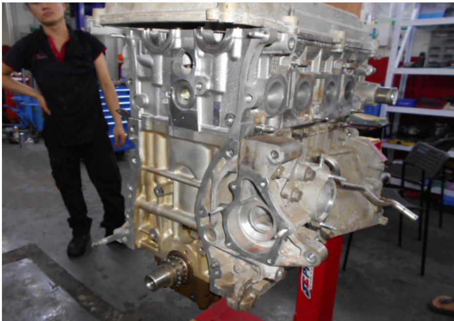
Photo 2 shows a general view of the Toyota engine that I had inspected. My visual examination of the engine housing revealed the housing to be of serviceable/satisfactory condition. There was no crack and/or hole observed on the engine housing.
