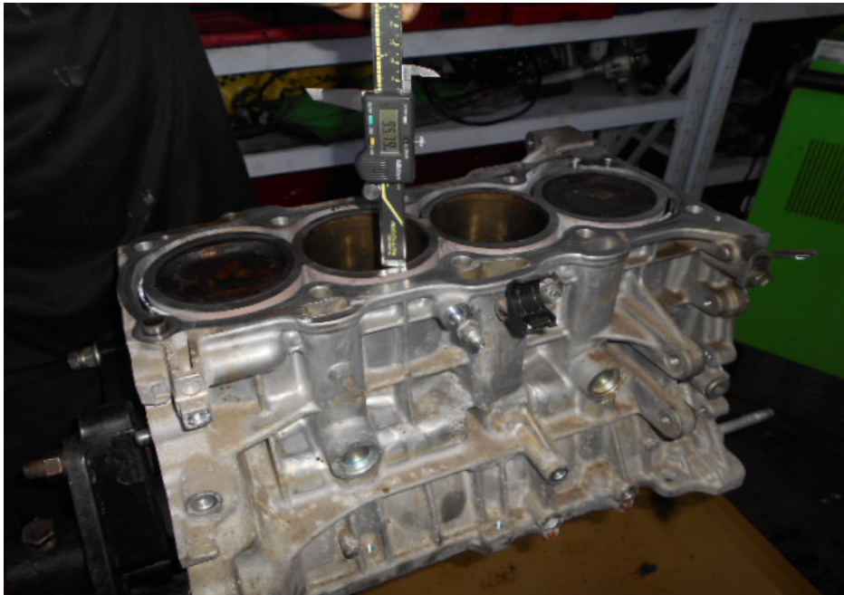
Photo 15 shows measurement of the stroke for cylinder 3 of the Toyota engine that I had inspected. The bore and stroke measurements of the Toyota engine were carried out using a digital Vernier Caliper that was calibrated before the start of measurements.
