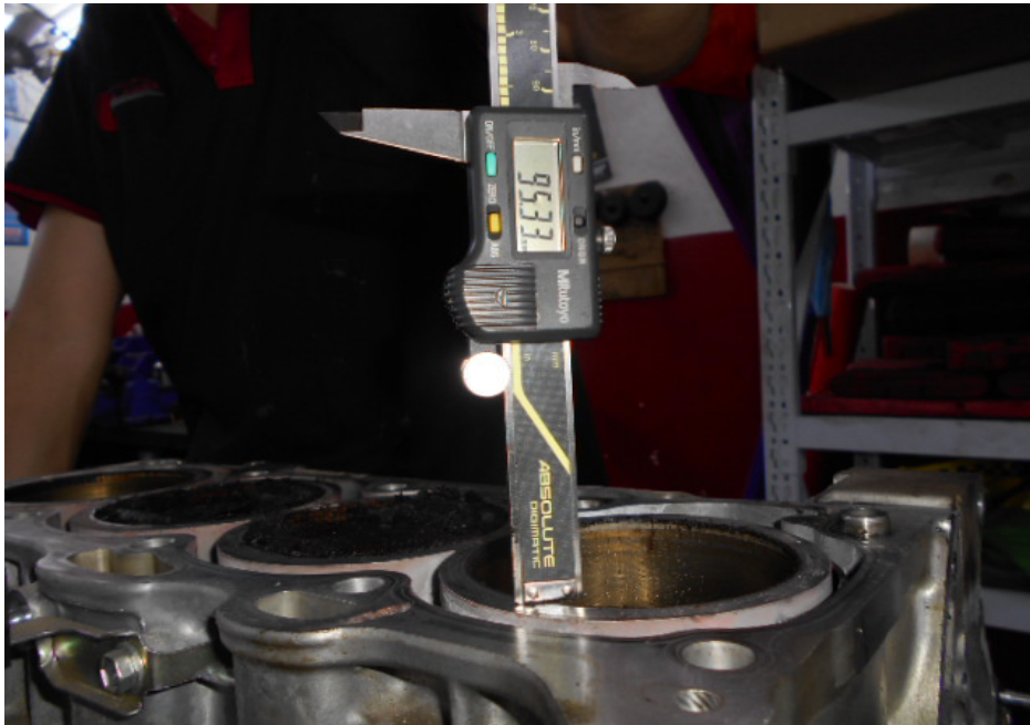
Photo 9 shows the stroke measurement of cylinder 1, which was recorded to be 95.33mm.
