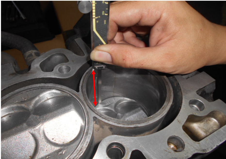
Photo 7 shows measurement being carried out to the stroke (arrowed) of cylinder 1 of the Honda engine. The bore and stroke measurements of the Honda engine were carried out using a digital Vernier Caliper that was calibrated before the start of the measurements.
