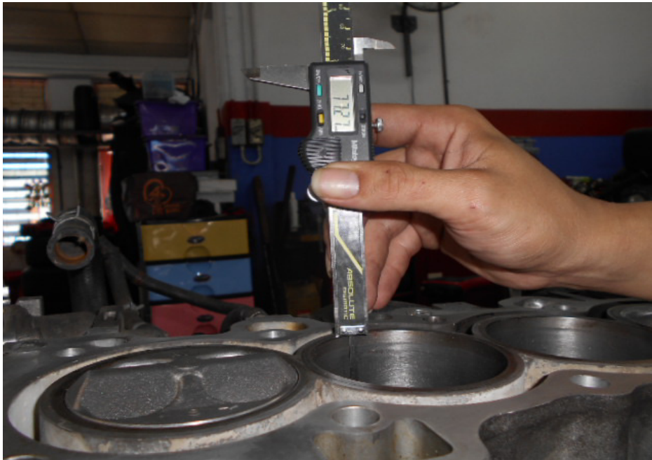
Photo 15 shows the stroke measurement of cylinder 3, which was recorded to be 77.27mm.
