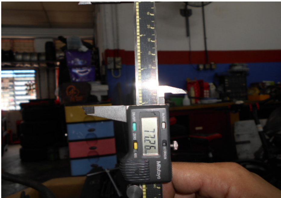
Photo 12 shows the stroke measurement of cylinder 2, which was recorded to be 77.26mm.
