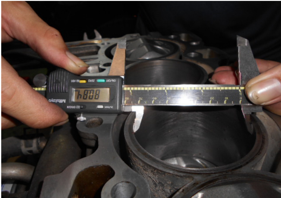
Photo 13 shows measurement being carried out to the bore of cylinder 3 of the Honda engine. The bore and stroke measurements of the Honda engine were carried out using a digital Vernier Caliper. The bore measurement of cylinder 3 was recorded to be 80.84mm.
