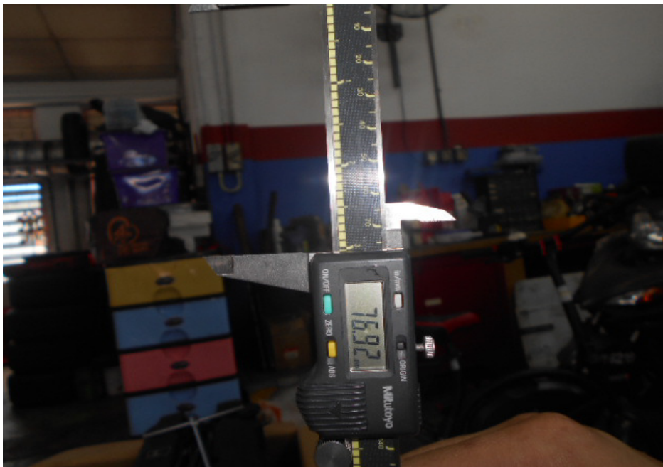
Photo 8 shows the stroke measurement of cylinder 1, which was recorded to be 76.92mm.
