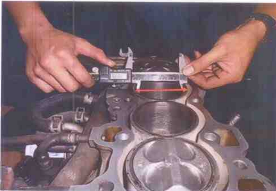
Photo 9 shows measurement being carried out to the bore (arrowed) of cylinder 2 of the Honda engine. The bore measurement of cylinder 2 was recorded to be 80.20mm.
