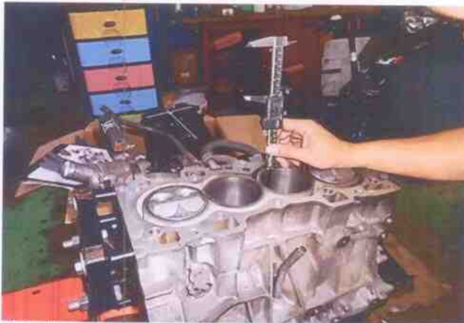
Photo 11 shows measurement of the stroke of cylinder 2 of the Honda engine that I had inspected. The bore and stroke measurements of the Honda engine were carried out using a digital Vernier Caliper that was calibrated before the start of measurements.
