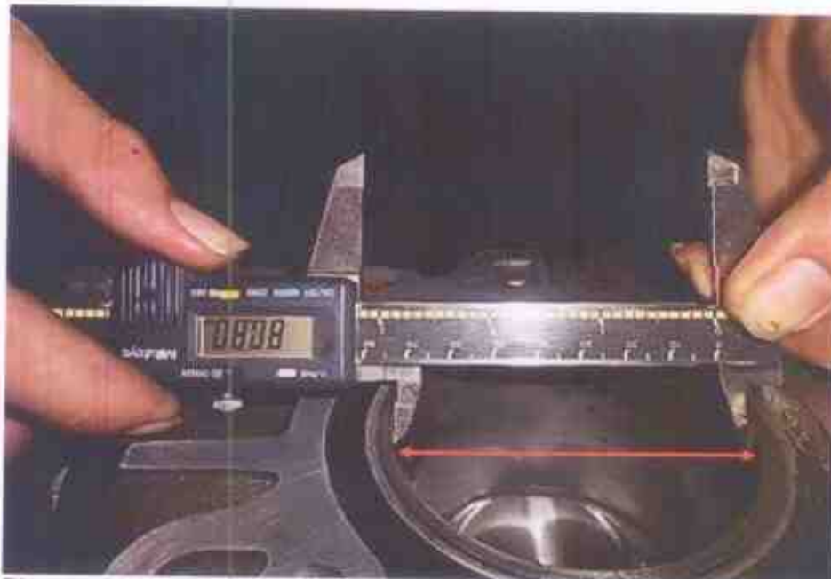
Photo 6 shows measurement being carried out to the bore (arrowed) of cylinder 1 of the Honda engine. The bore measurement of cylinder 1 was recorded to be 80.80mm.
