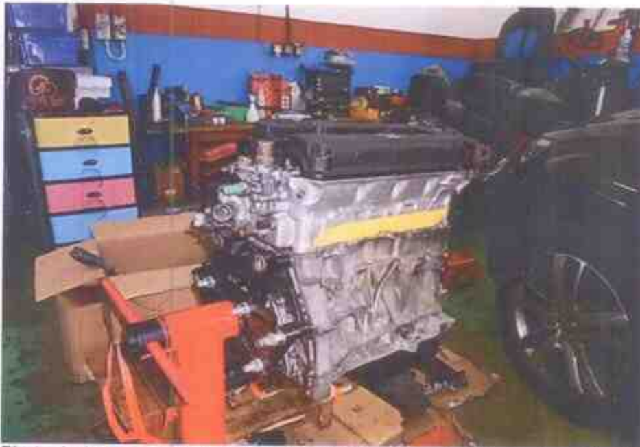
Photo 1 shows a general view of the Honda engine that I had inspected. The Honda engine was observed to be a used engine and was not fitted on any motor car. My visual examination of the engine housing revealed the housing to be of serviceable/satisfactory condition. There was no crack and/or hole observed on the engine housing.
