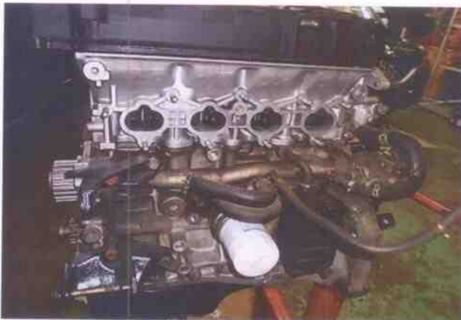
Photo 2 shows a general view of the Honda engine that I had inspected. My visual examination of the engine housing revealed the housing to be of serviceable/satisfactory condition. There was no crack and/or hole observed on the engine housing.
