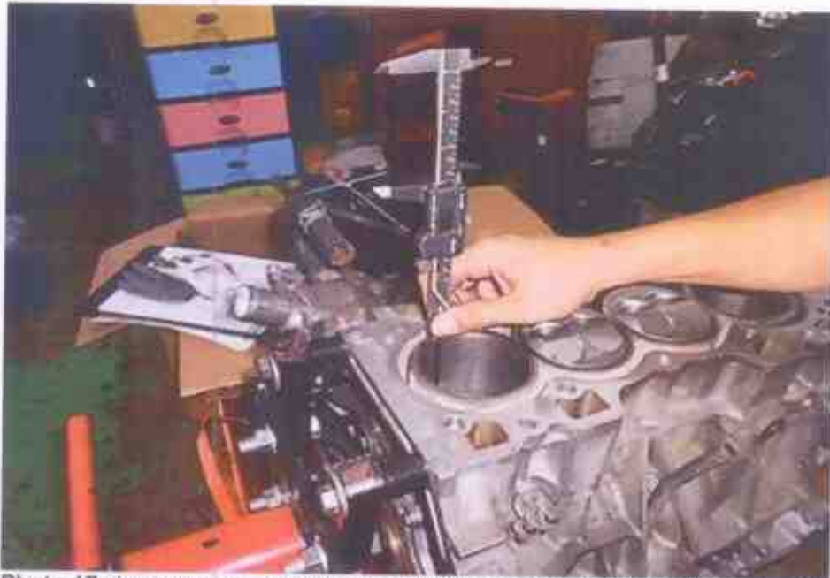
Photo 17 shows measurement being carried out to the stroke of cylinder 4 of the Honda engine. The bore and stroke measurements of the Honda engine were carried out using a digital Vernier Caliper that was calibrated before the start of measurements.
