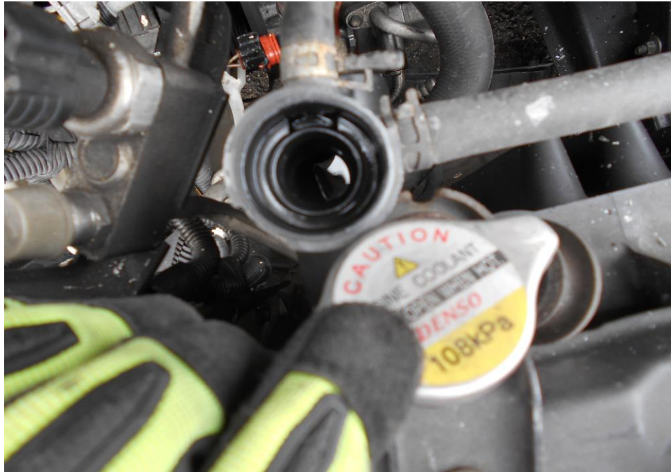
Photo 17 shows the coolant fluid tank of the Motor Car at the time of our inspection. The coolant fluid was observed to be of insufficient level as a result of the damaged radiator due to the accident.
