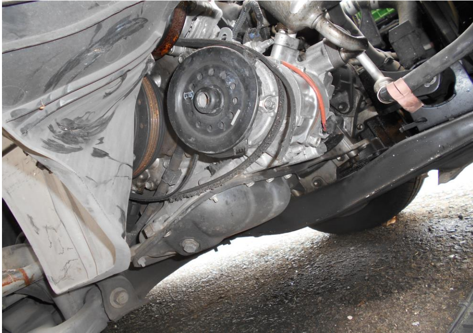
Photo 21 shows the belting of the Motor Car at the time of our inspection. It was observed to be damaged due to the accident's impact.
