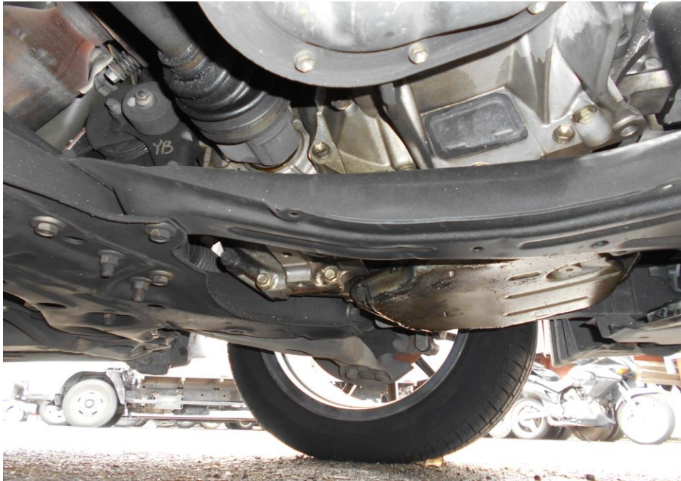
Photo 19 shows leakage of the various operating fluids such as engine fluid & brake fluid was noted. Given the extent of damages to the engine compartment, the leakages were likely due to the accident. The engine undercarriage was however observed to be covered with reddish fluid, suggesting leakage of fluid. There was no accumulation of dust and/or dirt particles on the engine housing where the fluid stains had formed. This would indicate that the fluid leakage was a fresh leak and likely to be a result of the accident.
