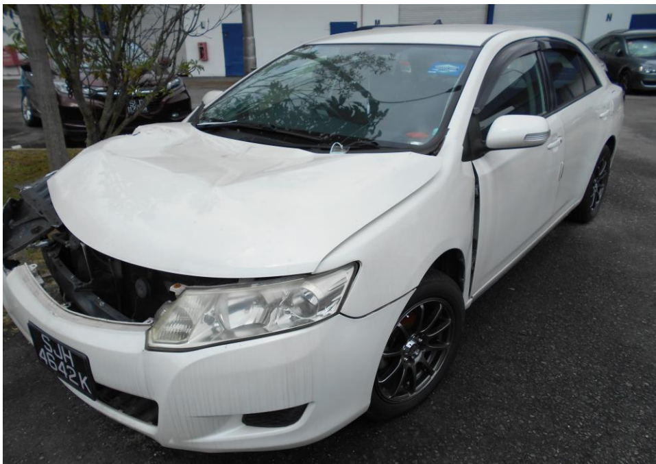
Photo 4 shows a general view of the front left body of the Motor Car at the time of our inspection. The Motor Car was observed to have sustained minor damages at the left frontal portion.
