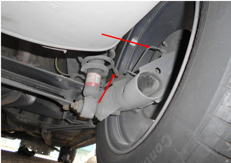
Photo 25 shows the various undercarriage components at the rear right wheel of the Motor Car. We did not observe any leakage of brake fluid at the time of our inspection of the Motor Car. Our visual inspection of the various mechanical components of the Motor Car's braking system revealed all to be intact and without visible damage, indicating that the braking system was likely to be in serviceable condition at the material time of accident.
