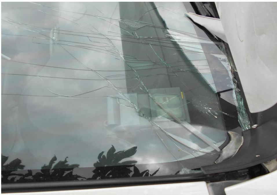
Photo 8 shows a close up view of the shattering cracked of the Motor Car's windshield at the time of our inspection.
