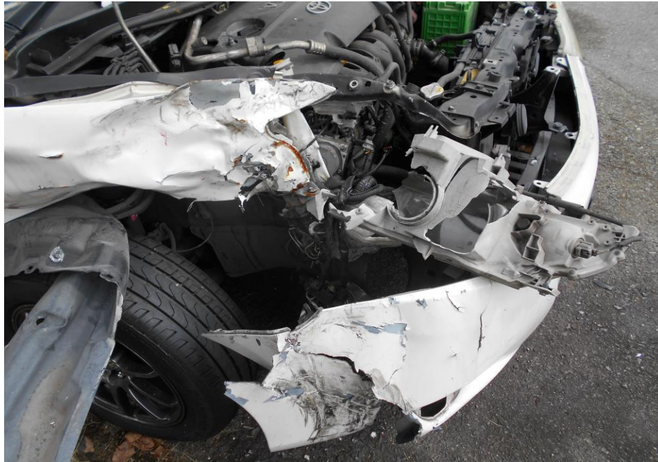
Photo 5 shows a close up view of the front right headlamp of the Motor Car at the time of our inspection. It had sustained damages likely due to the accident.
