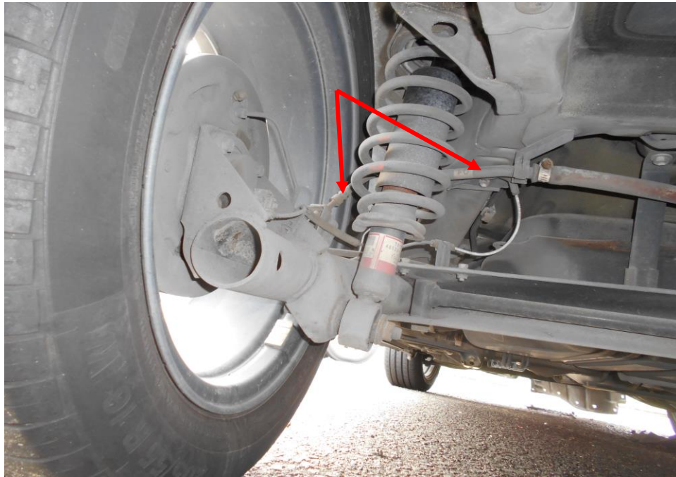
Photo 22 shows the brake hose (arrowed) at the rear left wheel of the Motor Car. Our visual inspection of the various mechanical components of the Motor Car's braking system revealed all to be intact and without visible damage, indicating that the braking system was likely to be in serviceable condition at the material time of accident.
