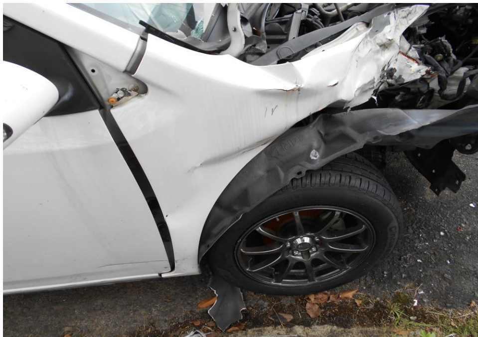
Photo 6 shows a close up view of the right side fender of the Motor Car at the time of our inspection. It had sustained damages likely due to the accident.
