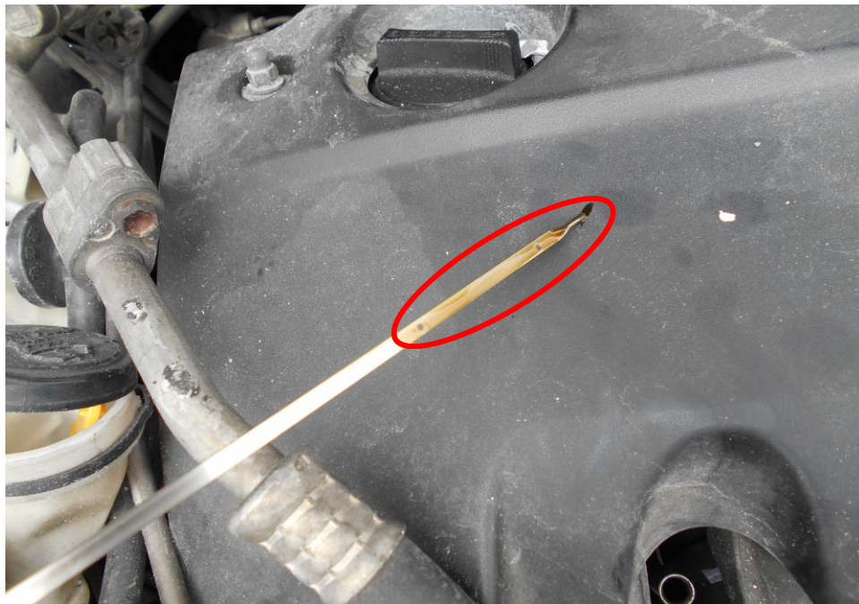
Photo 18 shows the engine oil dip stick of the Motor Car at the time of our inspection. The engine oil was observed to be of sufficient level and without any visible contamination.
