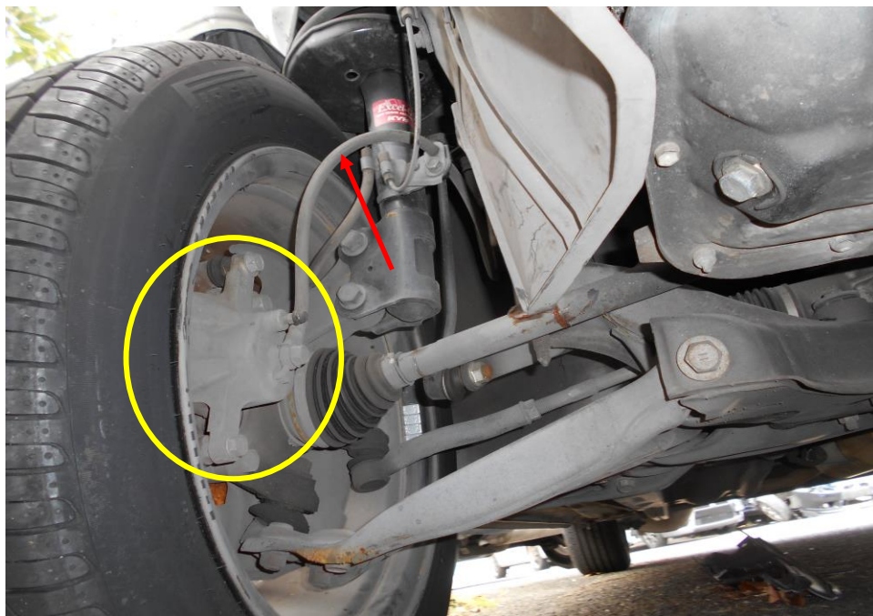
Photo 23 shows the brake hose (arrowed) at the front right wheel of the Motor Car. Our visual inspection of the various mechanical components of the Motor Car's braking system, including its brake calliper (circled), revealed all to be intact and without visible damage, indicating that the braking system was likely to be in serviceable condition at the material time of accident.
