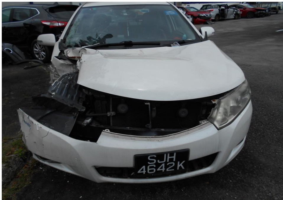
Photo 2 shows a general view of the front body of the Motor Car at the time of our inspection. The Motor Car was observed to have sustained extensive damages at the front right portion.
