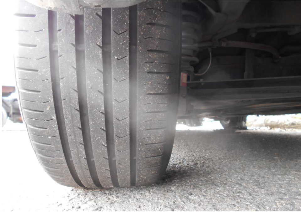
Photo 12 shows the condition of the rear left tyre of the Motor Car, which was observed to be in serviceable condition with remaining tread depth of approximately 7mm. The tyre was also observed to be sufficiently inflated for vehicular operation.
