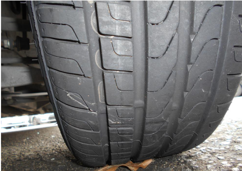
Photo 10 shows the condition of the front left tyre of the Motor Car, which was observed to be in serviceable condition with remaining tread depth of approximately 7mm. The tyre was also observed to be sufficiently inflated for vehicular operation.
