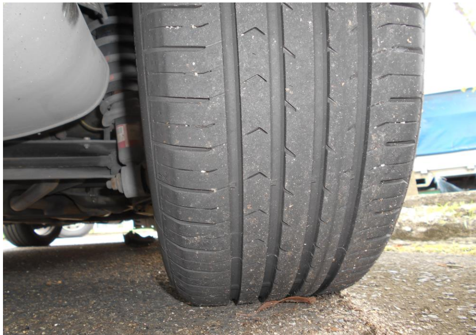
Photo 13 shows the condition of the rear right tyre of the Motor Car, which was observed to be in serviceable condition with remaining tread depth of approximately 7mm.
