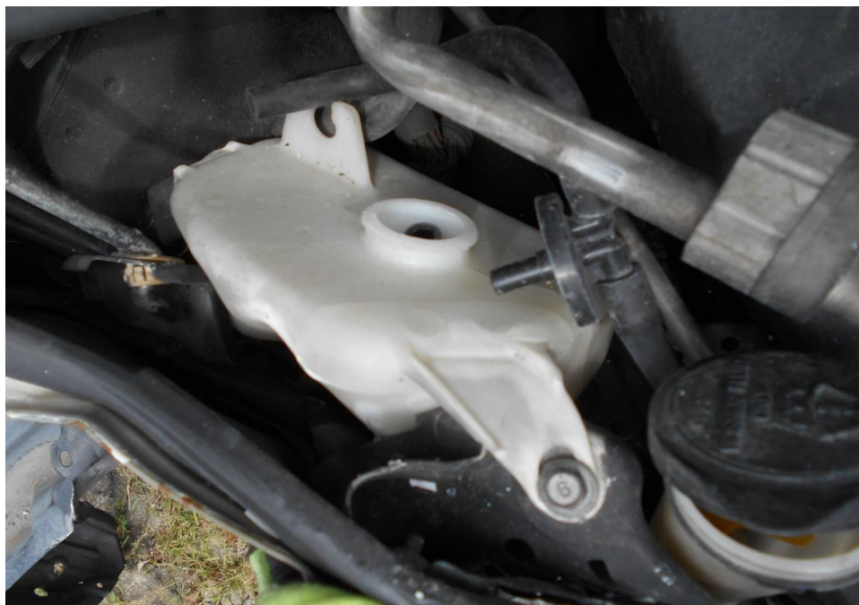
Photo 16 shows the coolant fluid reservoir of the Motor Car at the time of our inspection. The coolant fluid reservoir was observed to be damaged due to the accident's impact.
