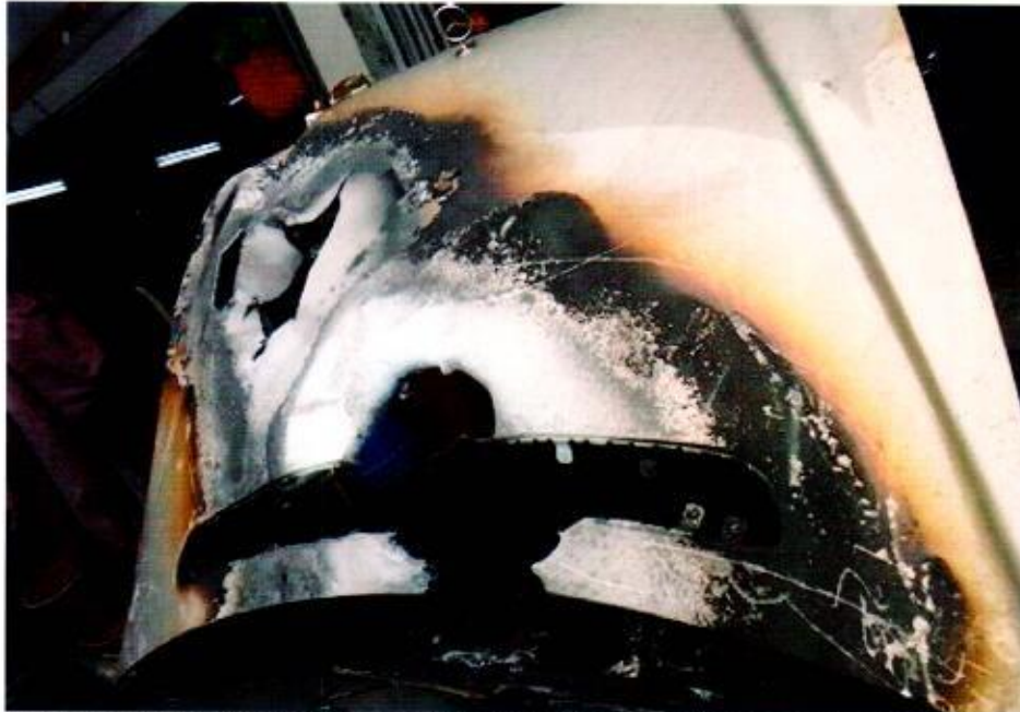
Photo 3 shows the topside bonnet of the Insured Vehicle at the time of our inspection. It was observed to sustain with burnt marks.
