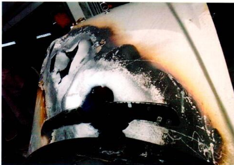
Photo 5 shows the burn pattern and whitish burn marks that were found on the topside of the front bonnet of the Insured Vehicle. Such whitish burn marks are a result of exposure to prolong heat intensity, which may indicate where the fire had started. Rust would also begin to develop on these areas soon after the fire.
