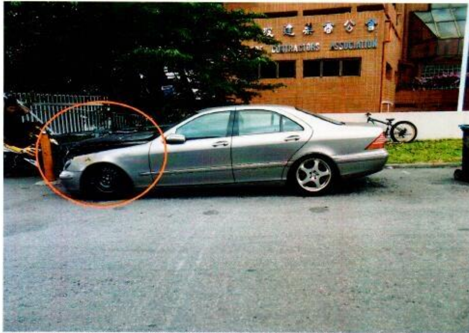
Photo 1 shows the general view of the Insured Vehicle at the time of our inspection. The fire damage to the Insured Vehicle was confined to its front bonnet and entire engine parts were amongst the body parts that were found to have been affected as a result of the fire.
