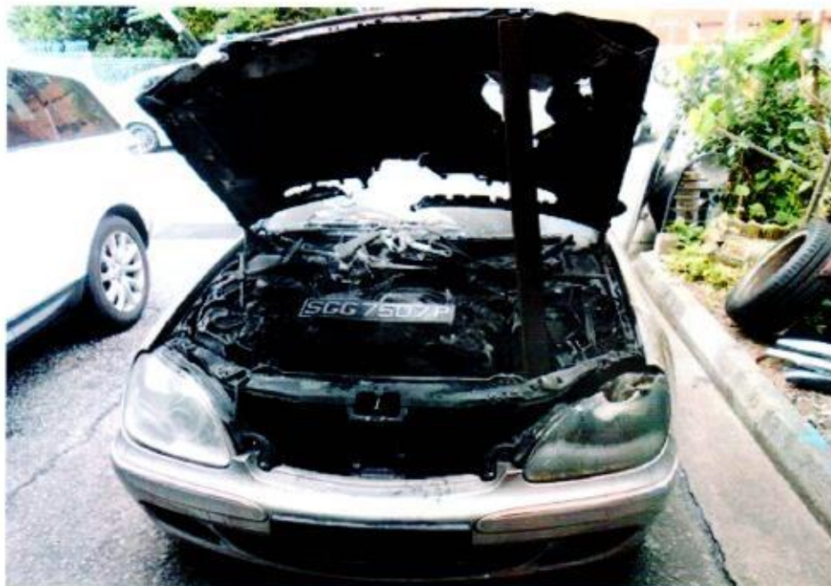
Photo 2 shows the general view of the front centre portion of the Insured Vehicle at the time of our inspection. The fire damage to the Insured Vehicle was confined to its front bonnet and entire engine parts were amongst the body parts that were found to have been affected as a result of the fire.
