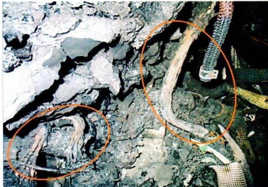
Photo 10 shows a closer view of the burnt wirings around the rear centre portion of the engine compartment, which is in the immediate vicinity where the fire to the Insured Vehicle had likely started. We noticed greenish residue on several stretches of burnt wirings (circled). The presence of greenish residue indicates internal heating of copper wires, a sign of an electrical short circuit occurring. The greenish residue is normally left behind from oxidation as a result of chemical reaction involving the copper wires.
