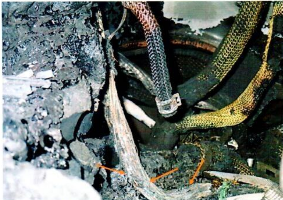
Photo 11 shows a close up view of the greenish residue found on several stretches of burnt wirings (red arrows). The presence of such greenish residue suggests occurrence of an electrical short circuit.
