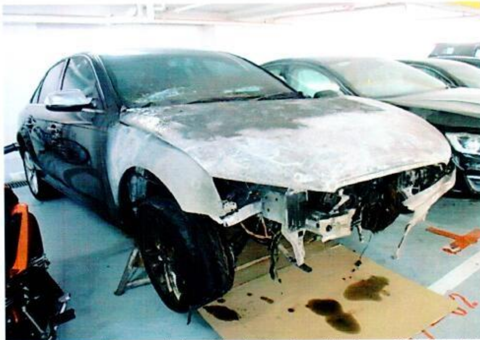
Photo 3 shows the general view of the right portion of the Insured Vehicle at the time of our inspection. The exterior body of the Insured Vehicle had sustained visible fire damage. This included its front windscreen, front bonnet, front bumper, right front panel, right headlight, right front rim and right front tyre.
