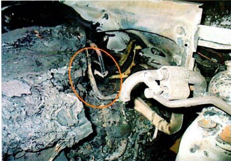
Photo 9 shows the burnt wirings around the rear centre portion of the engine compartment (circled), which is in the immediate vicinity where the fire to the Insured Vehicle had likely started.
