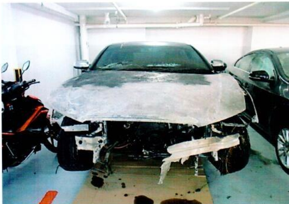
Photo 2 shows the general view of the front portion of the Insured Vehicle at the time of our inspection. The exterior body of the Insured Vehicle had sustained visible fire damage. This included its front windscreen, front bonnet, headlights, front bumper, side panels, front rims and front tyres.
