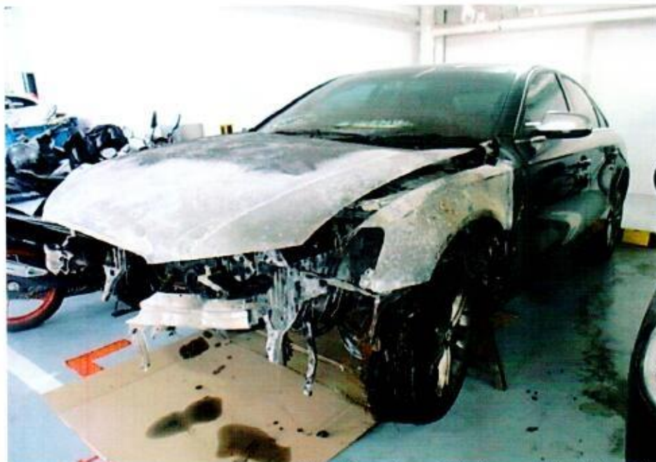
Photo 4 shows the general view of the left portion of the Insured Vehicle at the time of our inspection. The exterior body of the Insured Vehicle had sustained visible fire damage. This included its front windscreen, front bonnet, left headlight, front bumper, left front panel, left front rim and left front tyre.
