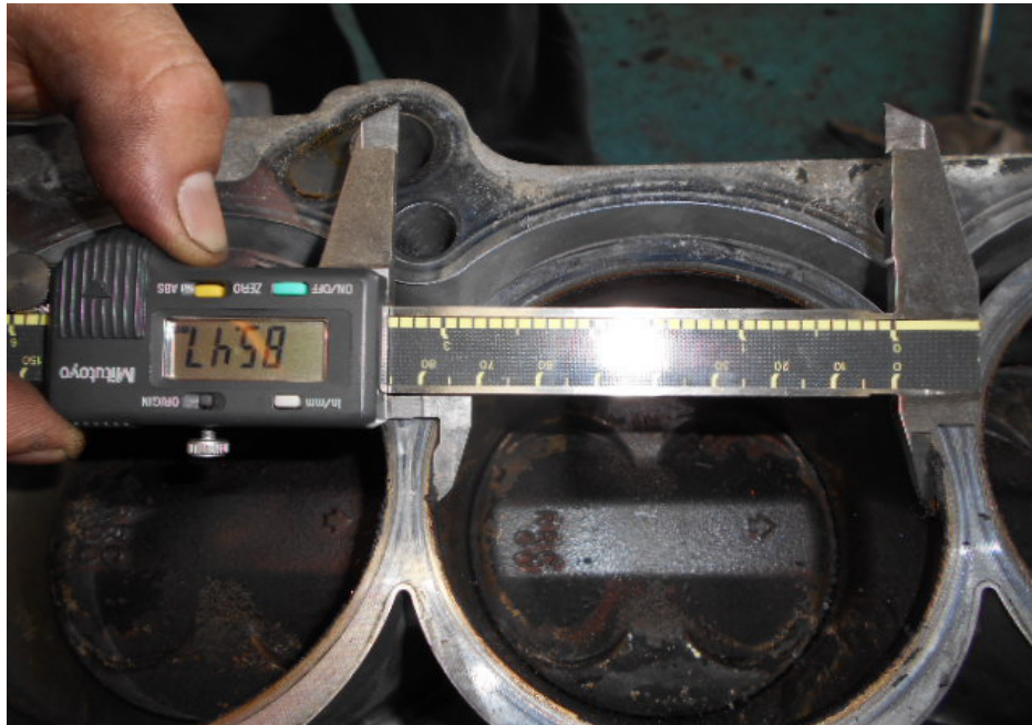
Photo 17 shows measurement being carried out to the bore (arrowed) of cylinder 3 of the Honda engine. The bore measurement of cylinder 3 was recorded to be 85.47mm.
