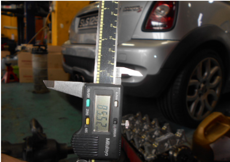
Photo 19 shows the stroke measurement of cylinder 3, which was recorded to be 85.52mm.
