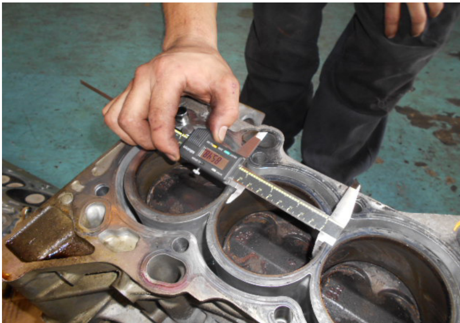
Photo 16 shows measurement being carried out to the bore of cylinder 3 of the Honda engine. The bore and stroke measurements of the Honda engine were carried out using a digital Vernier Caliper.
