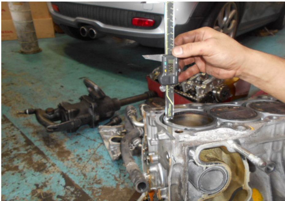
Photo 10 shows measurement being carried out to the stroke of cylinder 1 of the Honda engine. The bore and stroke measurements of the Honda engine were carried out using a digital Vernier Caliper.
