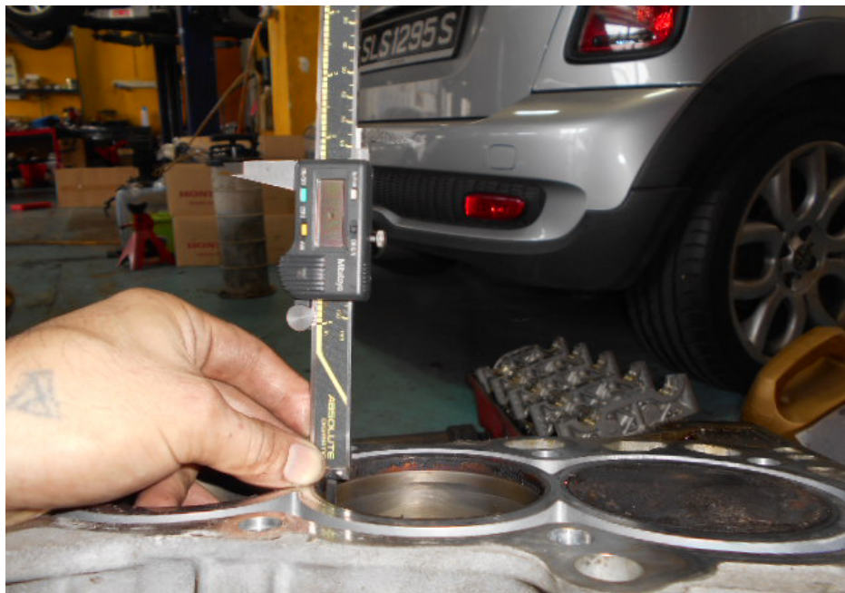
Photo 18 shows measurement of the stroke for cylinder 3 of the Honda engine that I had inspected. The bore and stroke measurements of the Honda engine were carried out using a digital Vernier Caliper that was calibrated before the start of measurements.
