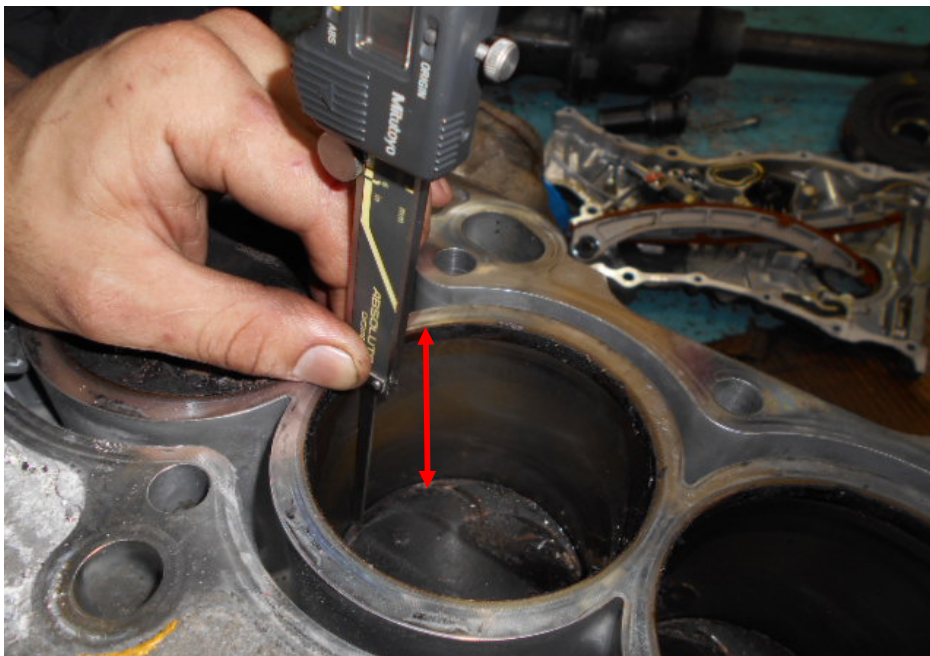
Photo 14 shows measurement of the stroke (arrowed) for cylinder 2 of the Honda engine that I had inspected.
