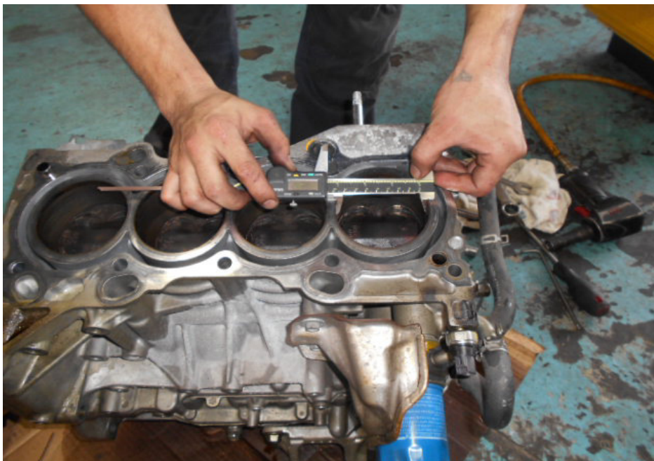
Photo 8 shows measurement being carried out to the bore of cylinder 1 of the Honda engine. The measurements were carried out using a digital Vernier Caliper that was calibrated before the start of the measurements.
