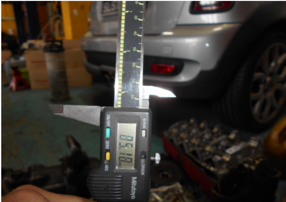
Photo 15 shows the stroke measurement of cylinder 2, which was recorded to be 85.18mm.
