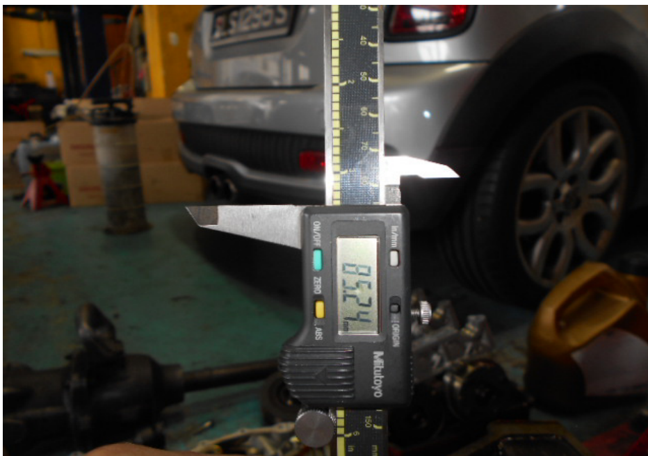
Photo 22 shows the stroke measurement of cylinder 4, which was recorded to be 85.24mm.
