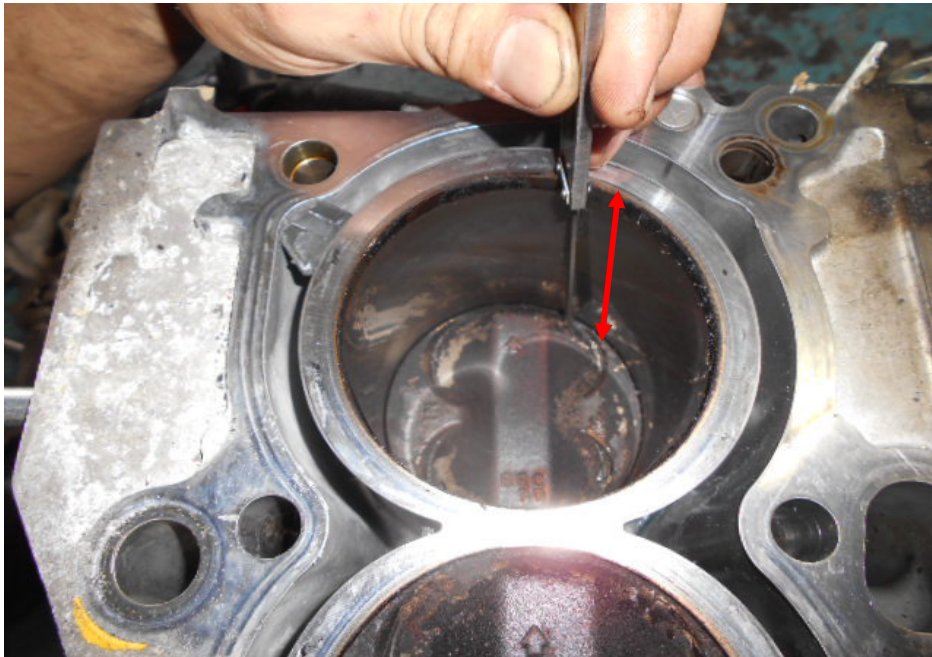
Photo 11 shows measurement being carried out to the stroke (arrowed) of cylinder 1 of the Honda engine. The bore and stroke measurements of the Honda engine were carried out using a digital Vernier Caliper that was calibrated before the start of the measurements,
