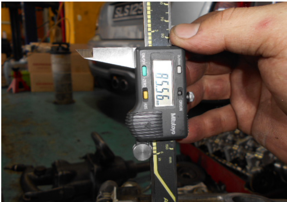
Photo 12 shows the stroke measurement of cylinder 1, which was recorded to be 85.56mm.
