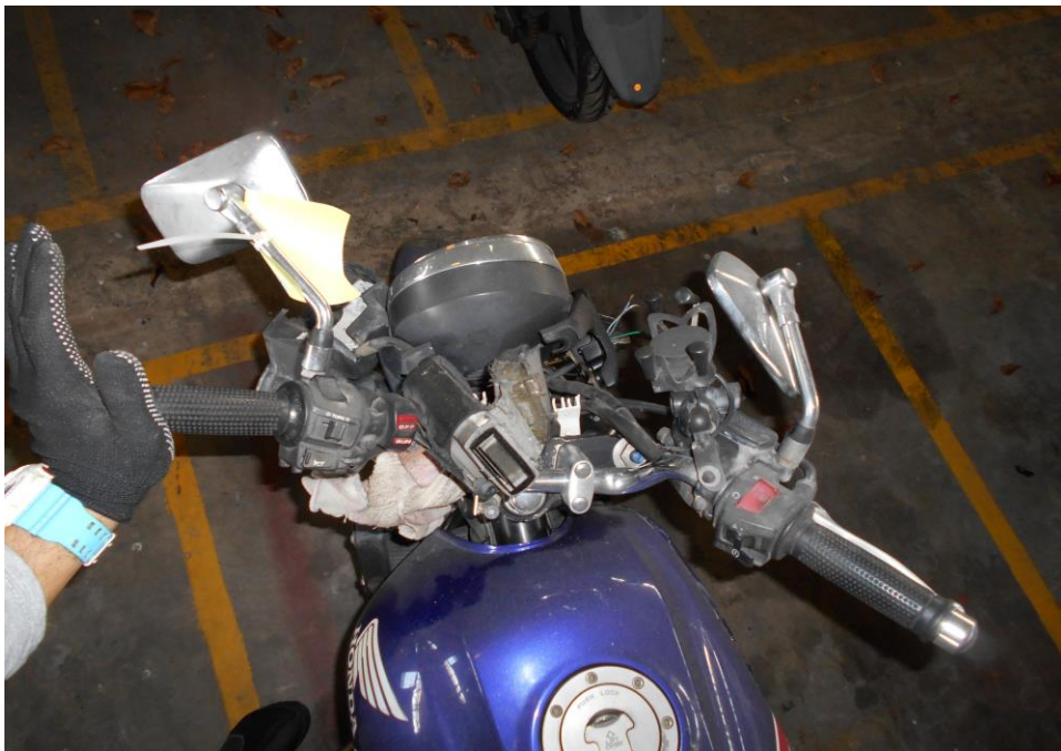
Photo 14 shows the steering system was observed to be damaged likely due to the accident's impact.
