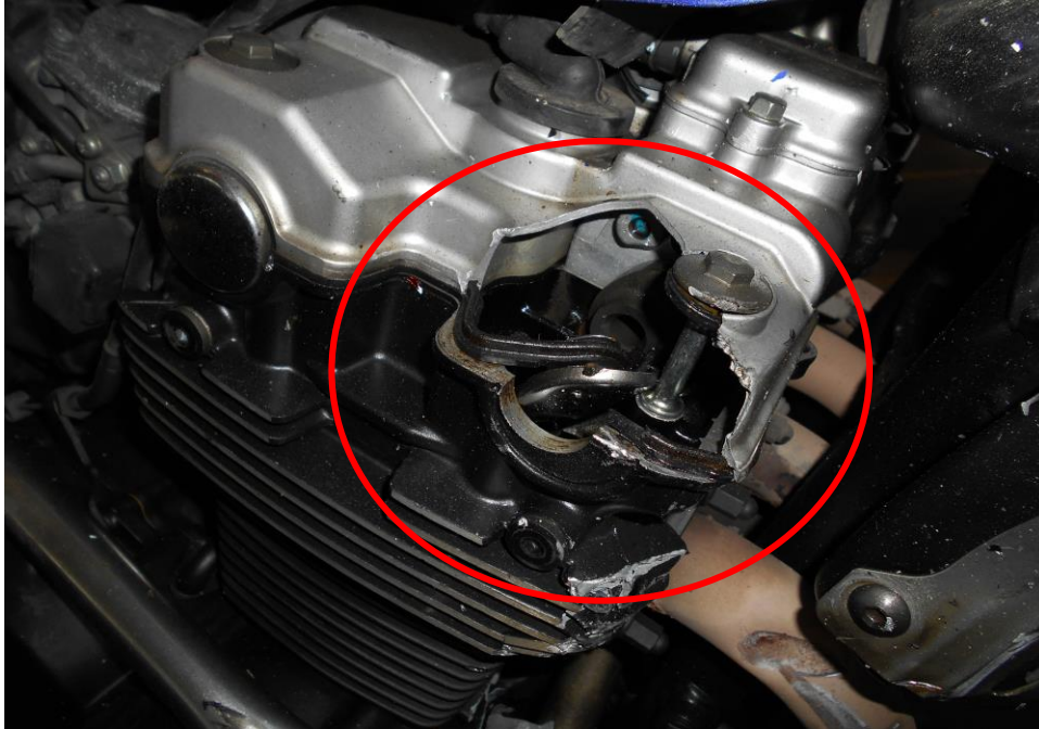
Photo 9 shows extensive damages on the engine block. It was observed to be damaged as a result of the accident.
