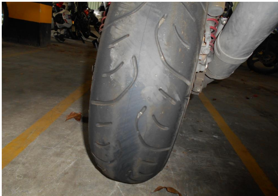
Photo 7 shows the rear tyre of the Motorcycle. The rear tyre was observed to be in serviceable condition with remaining tread depth of approximately 4mm. However, it was observed to be deflated likely due to the accident's impact.
