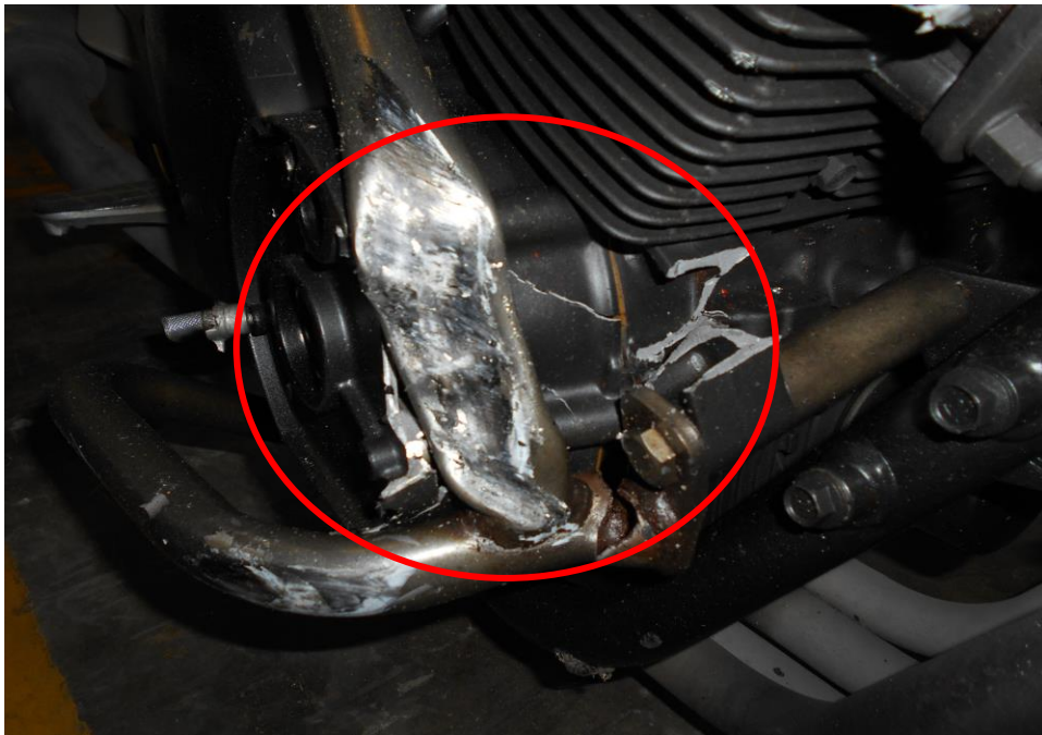
Photo 10 shows the damaged crash bar as a result of the accident.
