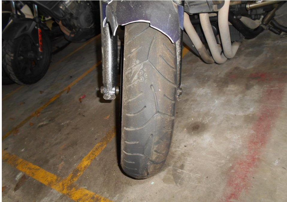
Photo 8 shows the front tyre of the Motorcycle. The pattern of the tread was clearly visible. There was no tear, burst mark(s) and/or punctured hole(s) on the sidewalls as well as across the tread of the front tyre with thread depth of 4mm.
