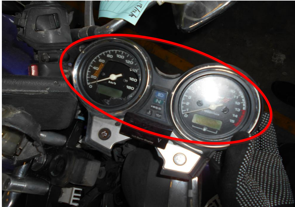
Photo 1 shows the speedo-meter of the Motorcycle where it was found dislodged from the original installation.
