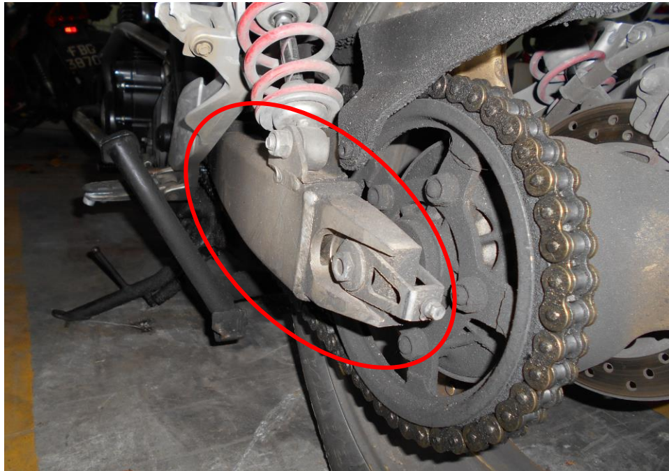
Photo 11 shows the gear chain of the motorcycle was found to sustained slight misalignment due to the accident's impact. However, it was observed to be adequately lubricated for operating purposes.
