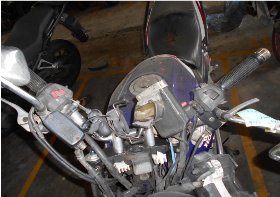
Photo 13 shows the handle bar was observed to be damaged by the accident's impact. It was observed to be misaligned likely due to the accident's impact.
