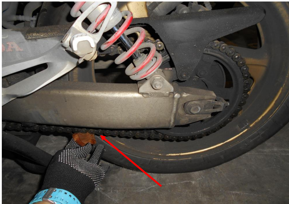
Photo 12 shows the general view of the gear train (arrowed) of the Motorcycle, which was observed to be tight due to the misalignment. Free play tension was unable to be established. Conclusively, it was unacceptable for operating purposes.
