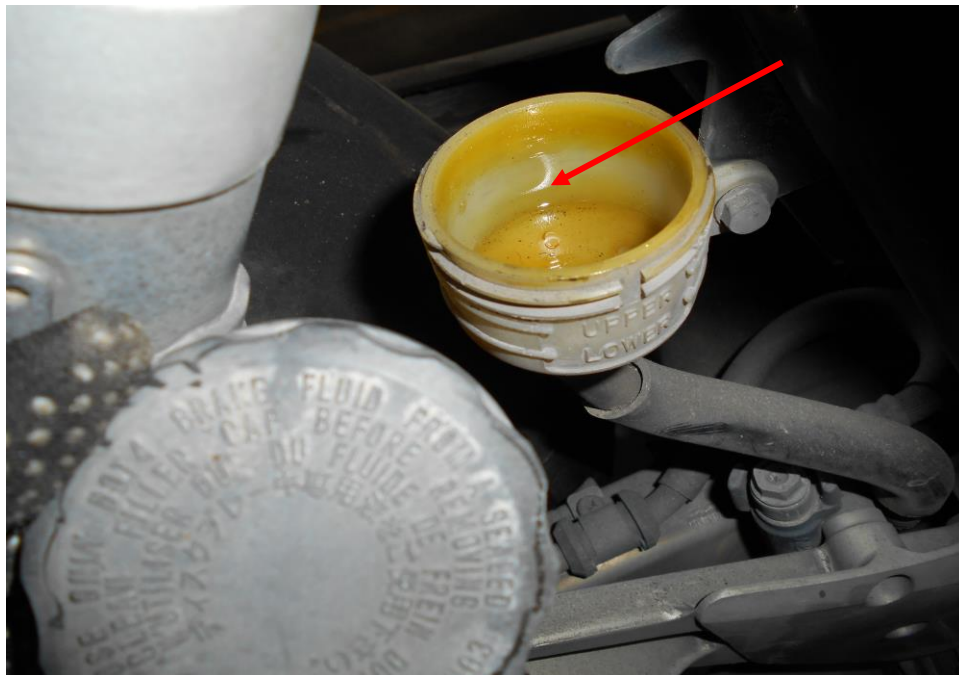
Photo 16 shows the brake fluid reservoir for the rear brake. It was observed to be at sufficient level not affected by the accident.
