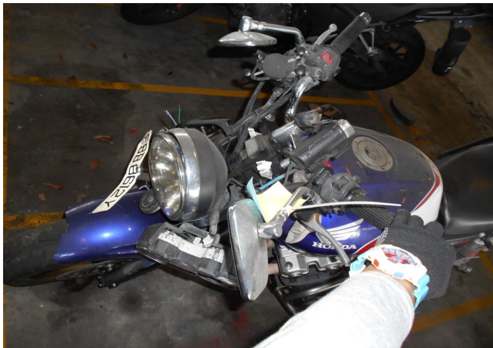
Photo 2 shows a general view of the front portion of the Motorcycle at the time of our inspection. The Motorcycle was observed to be sustained with damages due to the accident collision.
