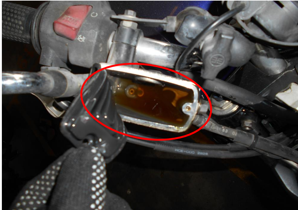
Photo 15 shows the fluid brake reservoir for the front brake that was observed to be unaffected by the accident. It was observed to be with sufficient level of brake fluid without any contamination.
