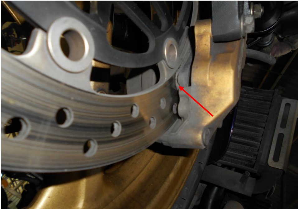
Photo 17 shows the brake pad for the front brake, observed to be in serviceable condition at time of our inspection. The frictional material found to be sufficient for operational purposes.
