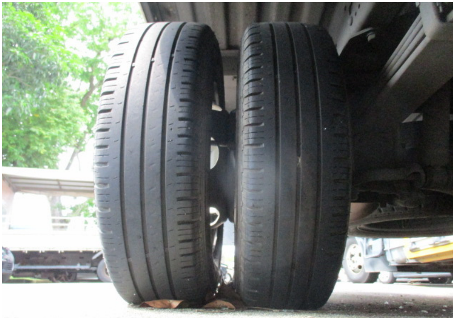
Photo 7 shows the condition of the rear right tyres of the Motor Lorry, which were observed to be in serviceable condition with remaining tread depth of approximately 3mm. There was also no tear, cut or burst mark(s) on the outer and the inner sidewalls as well as across the tread of the 6 tyres that were fitted on the Motor Lorry.
