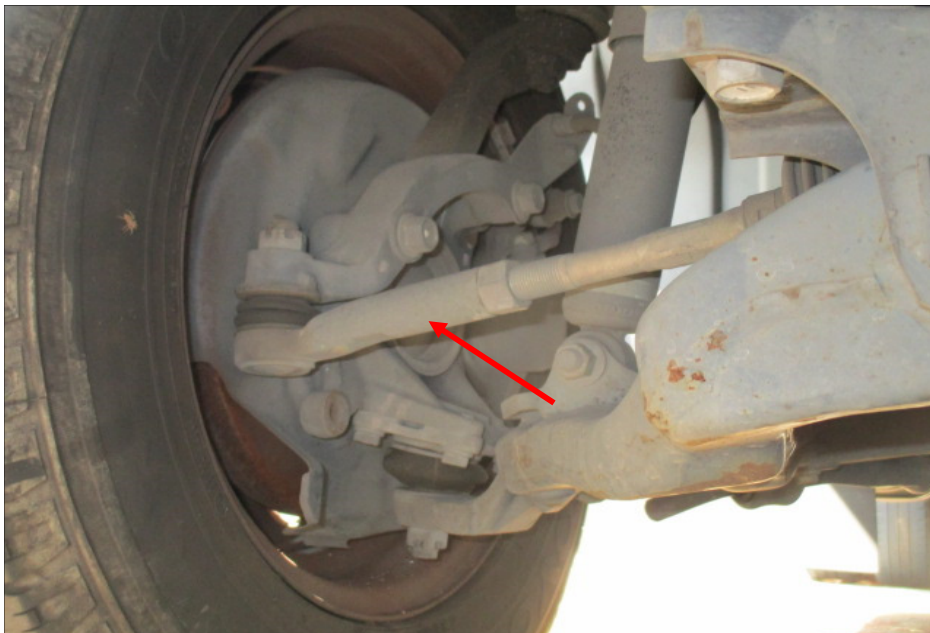
Photo 15 shows the various undercarriage components at the front right wheel of the Motor Lorry, in particular the steering tie rod end (arrowed). The various steering components were all found to be intact, suggesting that the steering system of the Motor Lorry was likely to be in serviceable condition at the material time of accident. There was also no sign of fluid stain(s) observed on the various undercarriage components.
