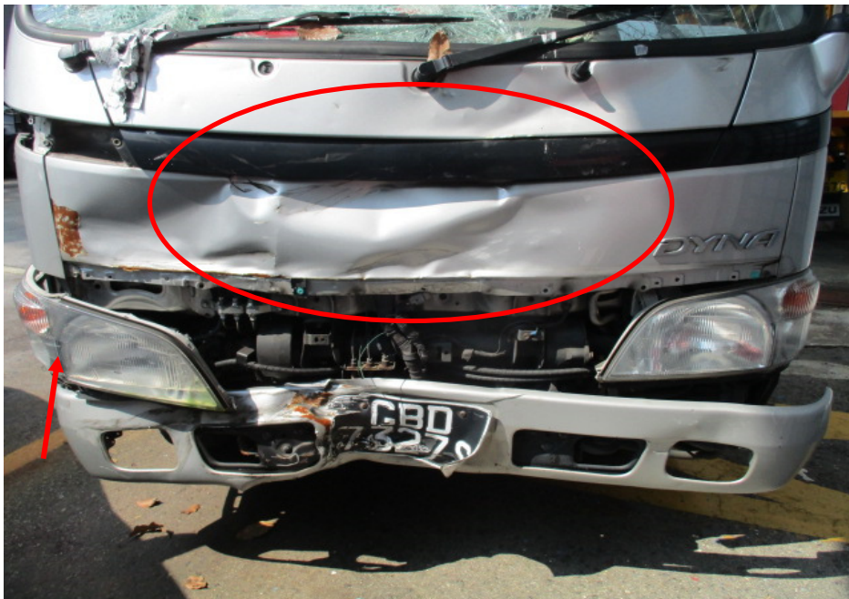
Photo 3 shows a closer view of the dislodged front bumper, dented front bonnet, dented front panel (circled) and cracked right headlight (arrowed) of the Motor Lorry at the time of our inspection.
