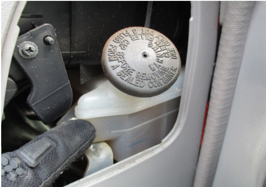
Photo 9 shows the brake fluid reservoir of the Motor Lorry at the time of our inspection. The brake fluid was observed to be of sufficient level and without any visible contamination.
