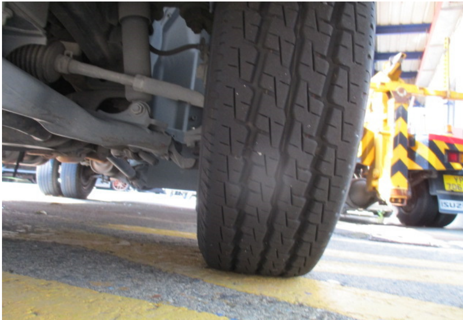
Photo 4 shows the condition of the front left tyre of the Motor Lorry, which was observed to be in serviceable condition with remaining tread depth of approximately 11mm. The tyre, which was wrapped around standard alloy wheel rim, was also observed to be sufficiently inflated for vehicular operation. There was no tear, cut or burst mark(s) on the outer and the inner sidewalls as well as across the tread of the 6 tyres that were fitted on the Motor Lorry.
