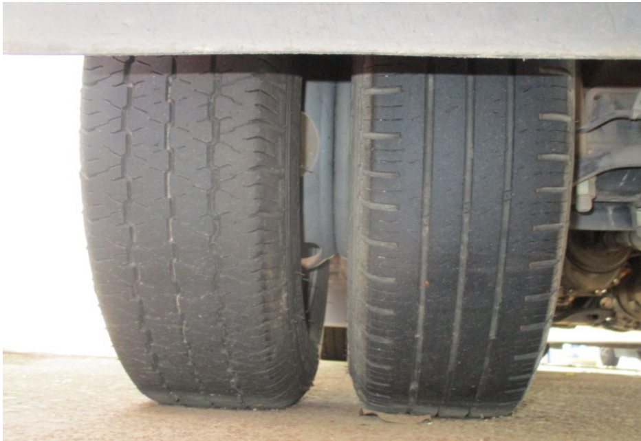
Photo 6 shows the condition of the rear left tyres of the Motor Lorry, which was observed to be in serviceable condition with remaining tread depth of approximately 3mm. The tyres, which were wrapped around standard alloy wheel rim, were also observed to be sufficiently inflated for vehicular operation. There was also no damage found on all 6 alloy wheel rims of the Motor Lorry.
