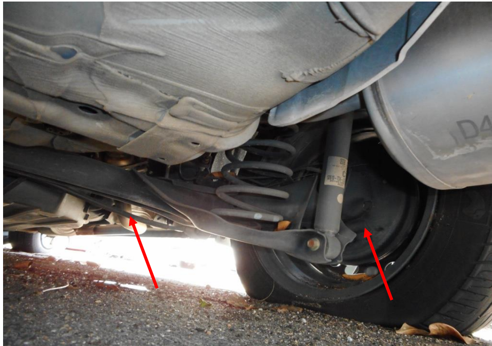
Photo 18 shows the various undercarriage components at the rear right wheel of the Motor Car, the brake hoses (arrowed). I did not observe any leakage of brake fluid & my visual inspection of the various mechanical components of the braking system revealed all to be intact and without visible damage, indicating that the braking system was likely to be in serviceable condition at the material time of accident.
