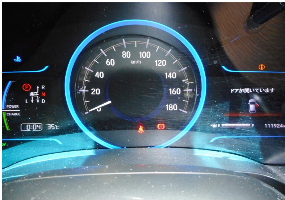
Photo 20 shows no warning lights illuminated on the instrument panel of the Motor Car after the engine was cranked. This would suggest that there was no abnormality to the various electronic operating systems of the Motor Car, like the ABS, EPS, TC and SRS etc.
