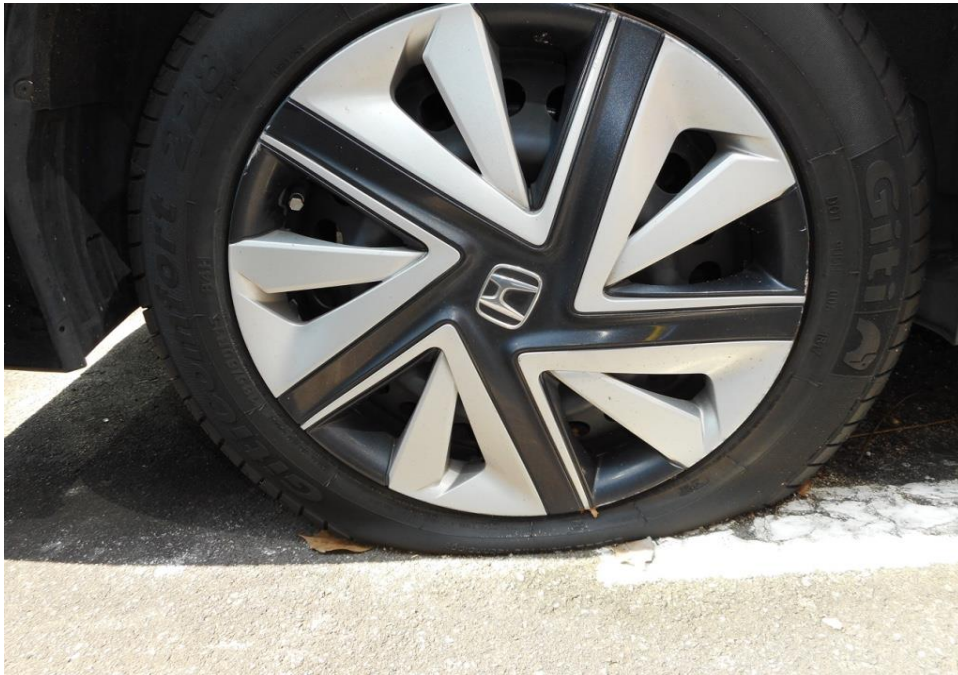
Photo 8 shows a general view of the rear right wheel rim and tyre of the Motor Car. The front right tyre was observed to be deflated. Which was observed to be in serviceable condition with remaining tread depth of approximately 4.6mm. There was no tear, cut or burst mark(s) on the outer and the inner sidewalls as well as across the tread of this tyre.
