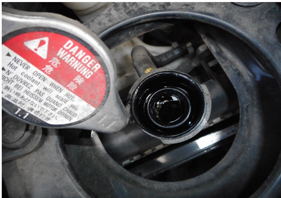
Photo 12 shows checks being carried out to the engine coolant of the Motor Car at the time of my inspection. The engine coolant was observed to be of sufficient level and without any visible contamination.
