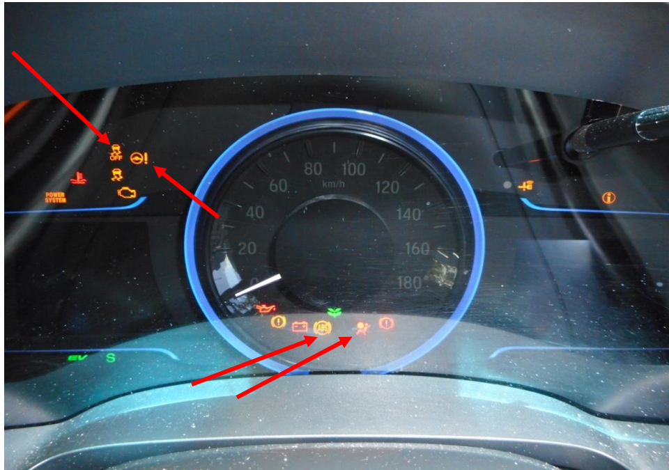
Photo 19 shows the warning light for Anti-Lock Brake System (ABS), Electric Power Steering System (EPS), Traction Control (TC) and Supplemental Restraint System (SRS) appearing on the instrument panel of the Motor Car during the self-test of its various electronic operating systems when its engine was cranked.
