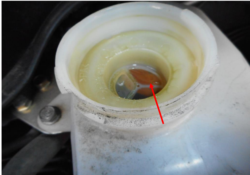
Photo 11 shows the brake fluid reservoir of the Motor Car at the time of my inspection. The brake fluid was observed to be of sufficient level (as indicated by the red arrows) and without any visible contamination.
