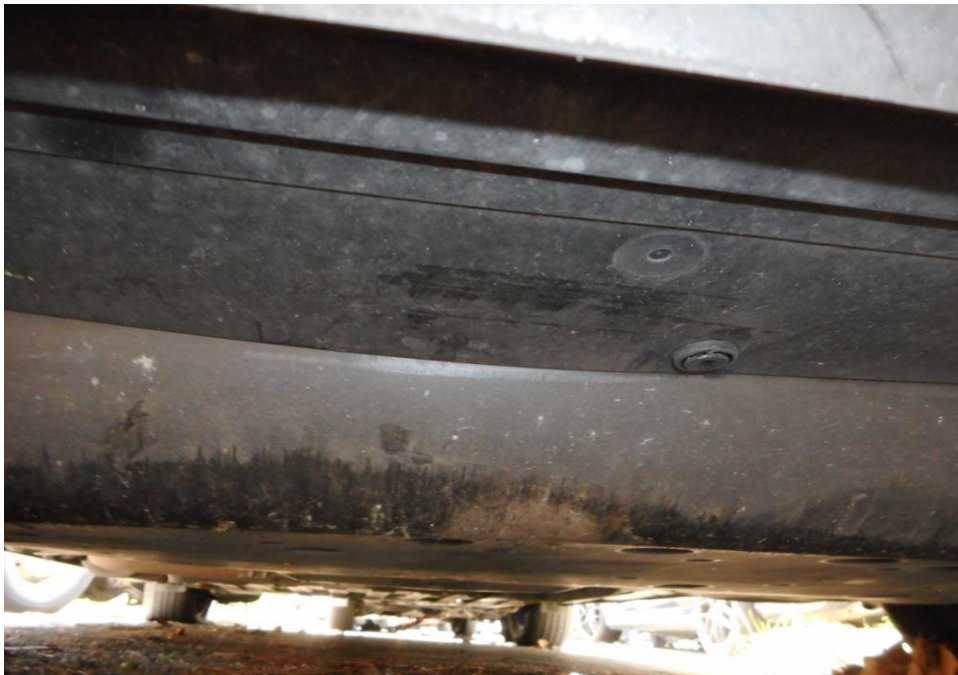
Photo 14 shows the front underside of the Motor Car. I did not find any sign(s) or indication(s) of fluid leak and/or fluid stain(s) on the underside.
