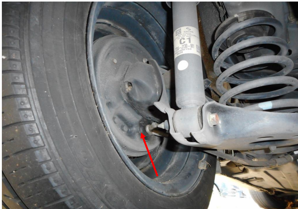
Photo 17 shows the various undercarriage components at the rear left wheel of the Motor Car, the brake hoses (arrowed). I did not observe any leakage of brake fluid & my visual inspection of the various mechanical components of the braking system revealed all to be intact and without visible damage, indicating that the braking system was likely to be in serviceable condition at the material time of accident.
