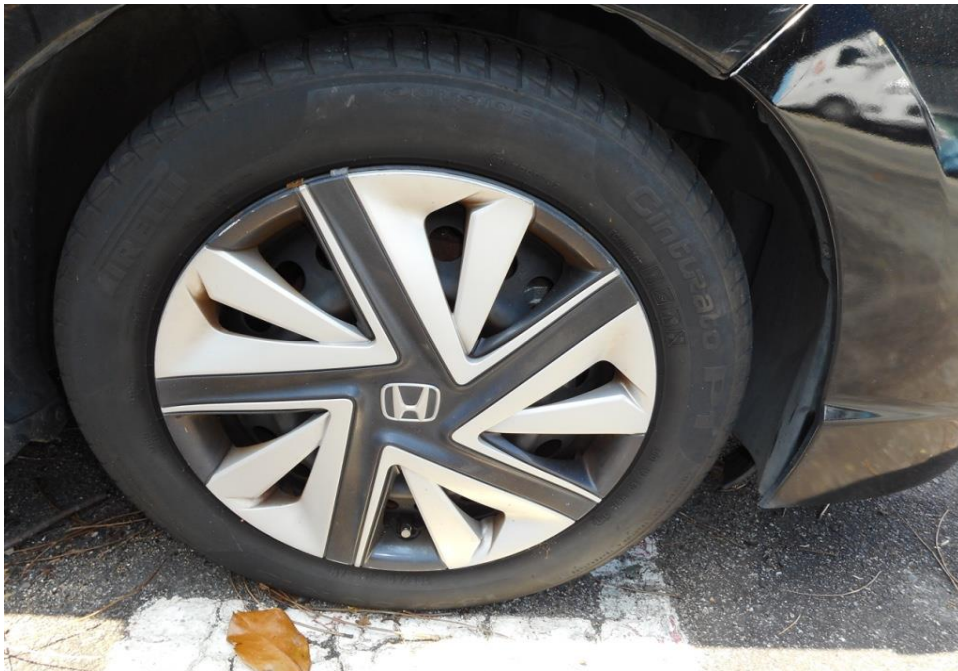
Photo 9 shows the condition of the front left tyre of the Motor Car, which was observed to be in serviceable condition with remaining tread depth of approximately 4.5mm. There was no tear, cut or burst mark(s) on the outer and the inner sidewalls as well as across the tread of this tyre. The tyre, which was wrapped around alloy wheel rim, was also observed to be sufficiently inflated for vehicular operation.
