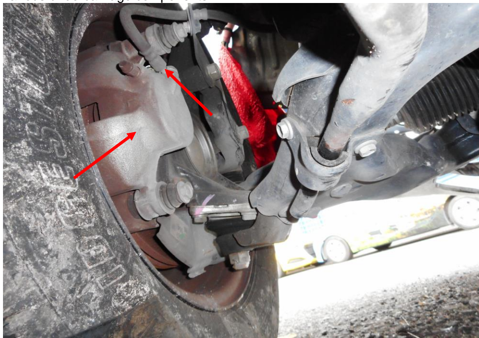
Photo 22 shows the various undercarriage components at the front right wheel of the Motor Lorry, in particular the brake hose and callipers (arrowed). The various undercarriage components of the Motor Lorry were all found to be intact without any visible damage. There was also no sign of fluid stain(s) observed on the various undercarriage components.
