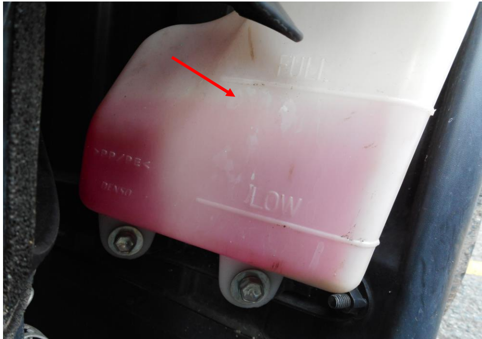
Photo 16 shows the engine coolant reservoir of the Motor Lorry at the time of our inspection. The engine coolant was observed to be of sufficient level and without any visible contamination (arrowed).
