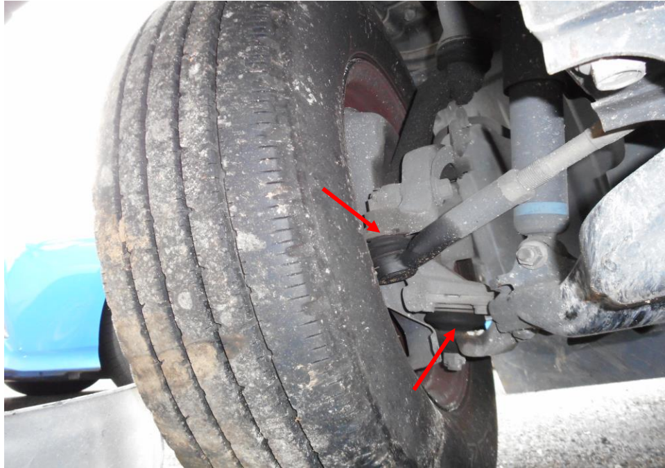
Photo 19 shows the various undercarriage components at the front left wheel of the Motor Lorry, in particular the steering tie rod end and ball joints (arrowed). The various undercarriage components of the Motor Lorry were all found to be intact without any visible damage. There was also no sign of fluid stain(s) observed on the various undercarriage components.
