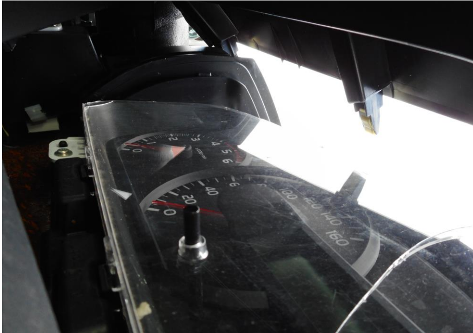
Photo 1 shows no mileage readings were recorded due to the damaged odometer in the instrument cluster of the Motor Lorry at the time of our inspection.
