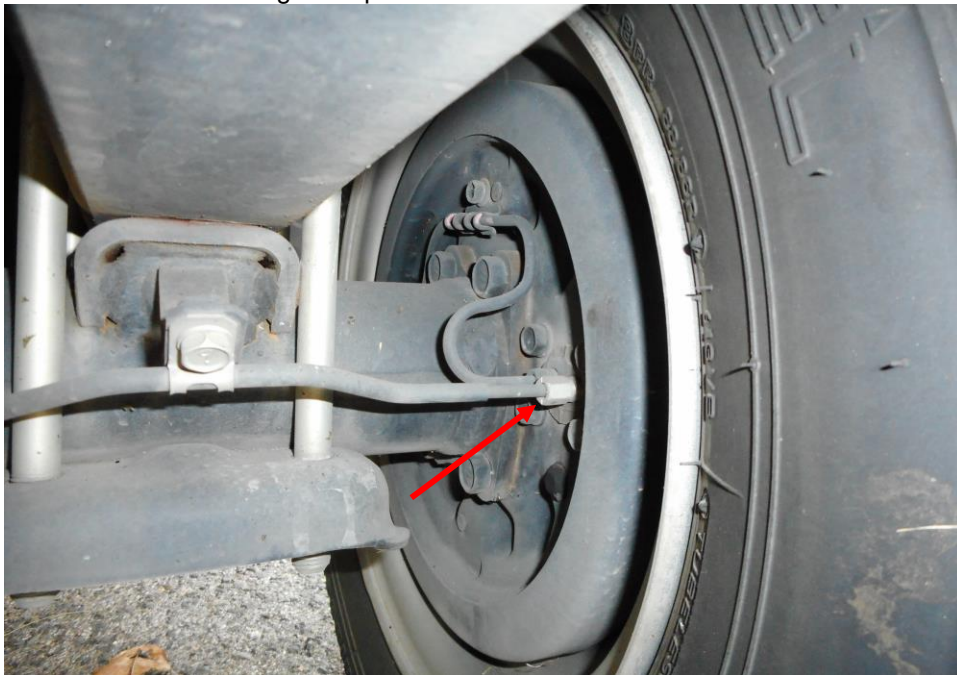
Photo 24 shows the various undercarriage components at the rear right wheel of the Motor Lorry, in particular the brake hose and drum brake (arrowed). The various undercarriage components of the Motor Lorry were all found to be intact without any visible damage. There was also no sign of fluid stain(s) observed on the various undercarriage components.
