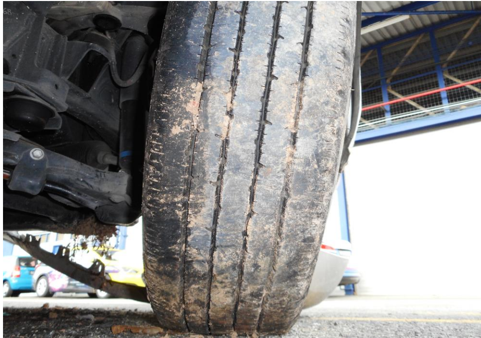
Photo 11 shows the condition of the front right tyre of the Motor Lorry, which was observed to be in serviceable condition with remaining tread depth of approximately 5.5mm. The tyre, which was wrapped around standard alloy wheel rim, was also observed to be sufficiently inflated for vehicular operation.
