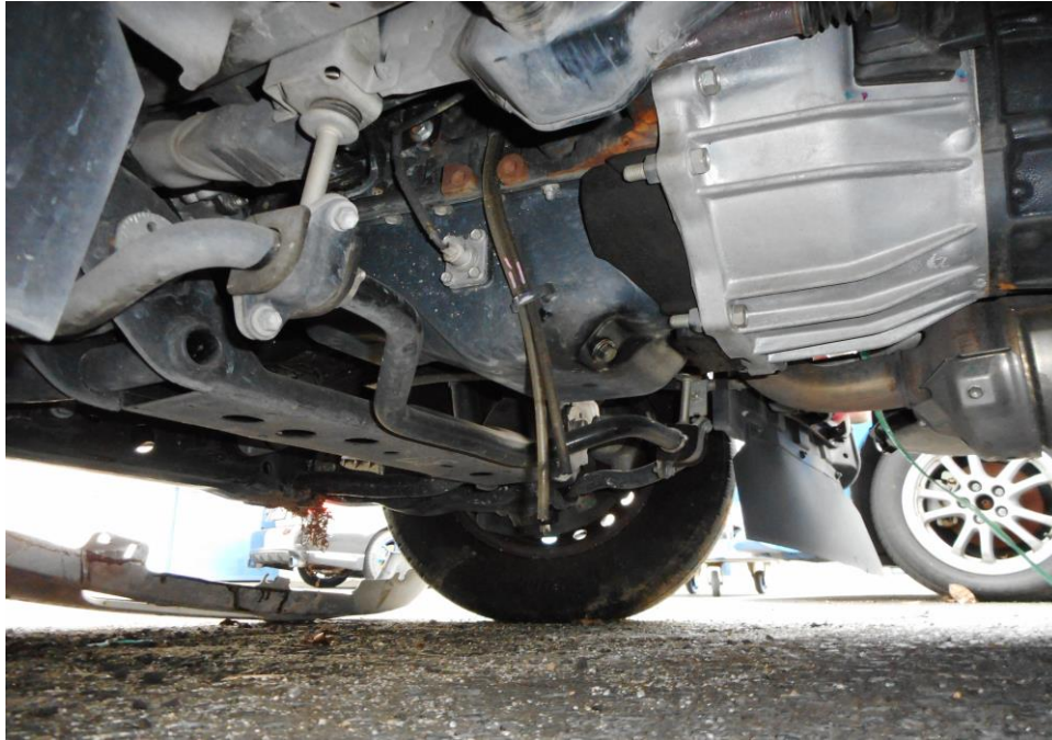
Photo 18 shows the undercarriage of the engine of the Motor Lorry at the time of our inspection. There was also no sign(s) or indication(s) of fresh fluid leakage and/or fluid stain within the engine area.
