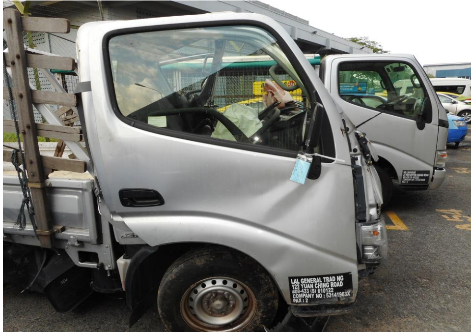
Photo 7 shows the close up view of the right door of the Motor Lorry at the time of our inspection. The Motor Lorry was observed to have sustained major damages to its doors that was crushed and dislodged due to the accident's impact.
