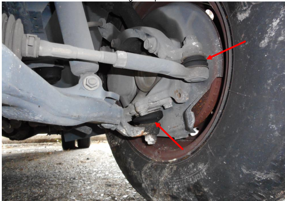
Photo 20 shows the various undercarriage components at the front right wheel of the Motor Lorry, in particular the steering tie rod end and ball joints (arrowed). The various undercarriage components of the Motor Lorry were all found to be intact without any visible damage. There was also no sign of fluid stain(s) observed on the various undercarriage components.
