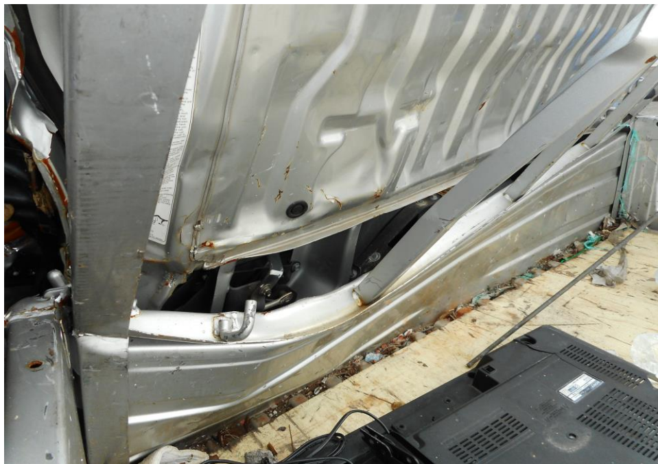
Photo 15 shows the induced damage to the cabin of the Motor Lorry's which immobilised the opening and viewing of the various parts and components inside the engine compartment, a result of the accident.
