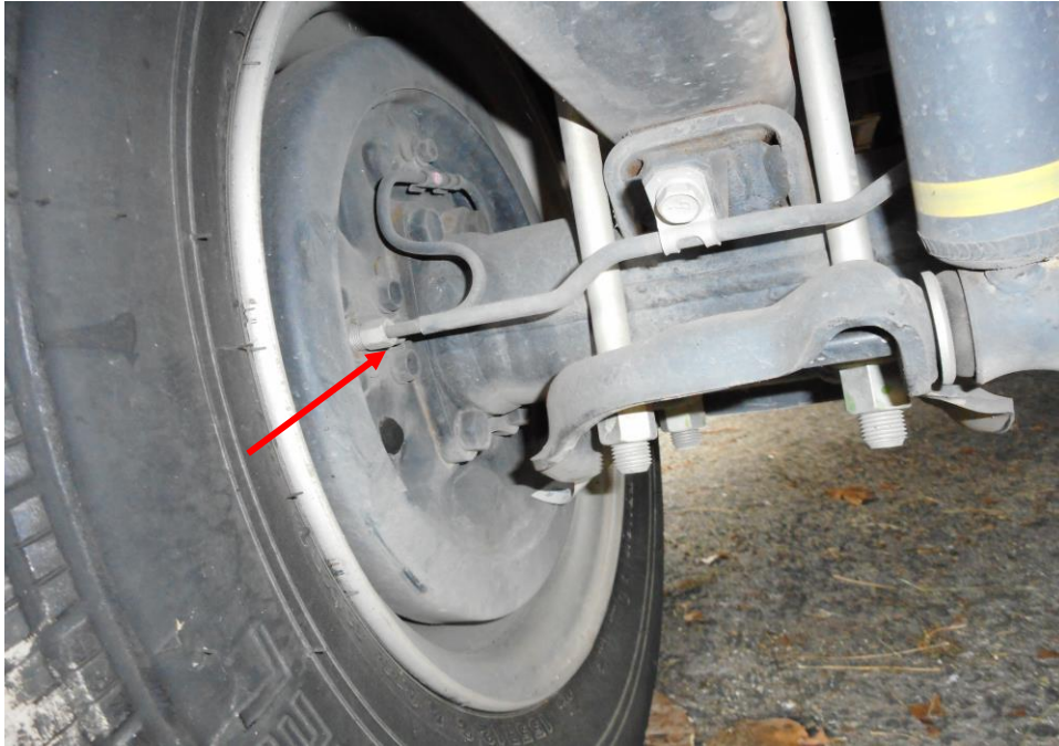
Photo 23 shows the various undercarriage components at the rear left wheel of the Motor Lorry, in particular the brake hose and drum brake (arrowed). The various undercarriage components of the Motor Lorry were all found to be intact without any visible damage. There was also no sign of fluid stain(s) observed on the various undercarriage components.
