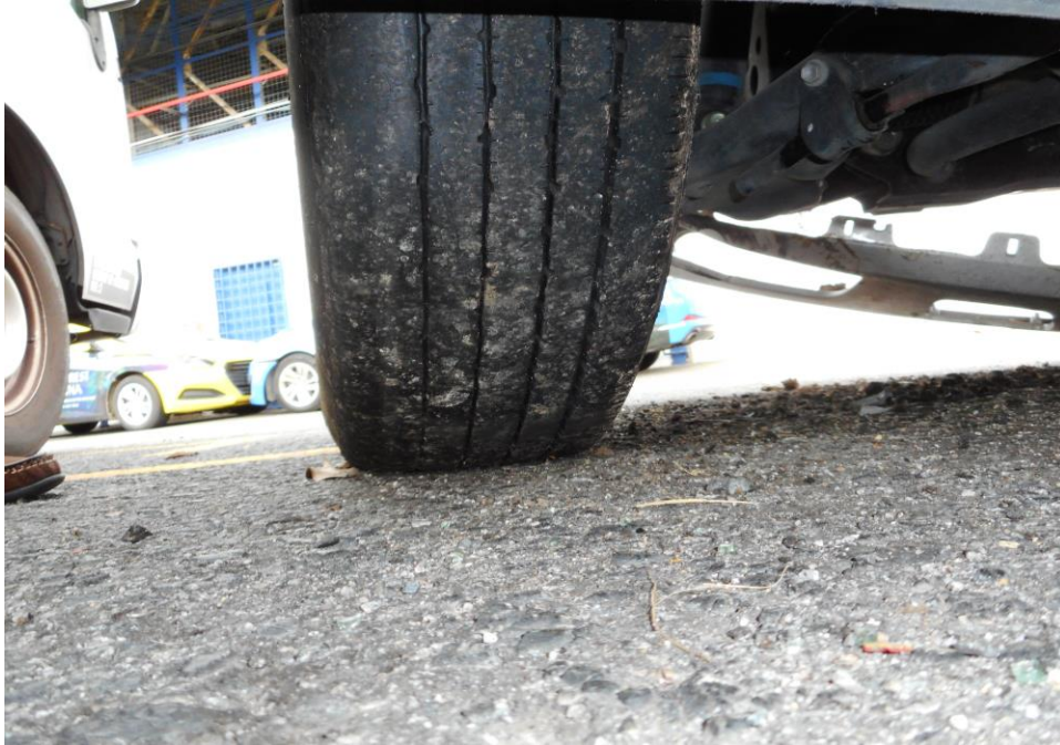
Photo 10 shows the condition of the front left tyre of the Motor Lorry, which observed to be in serviceable condition with remaining tread depth of approximately 3.7mm. The tyre, which was wrapped around standard alloy wheel rim, was also observed to be sufficiently inflated for vehicular operation.
