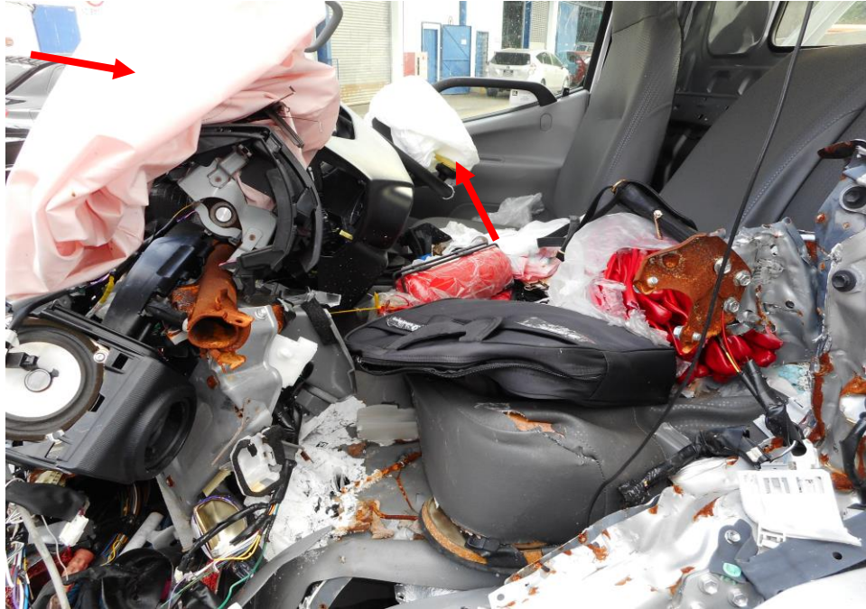
Photo 9 shows the close up view of the interior cabin of the Motor Lorry. It was observed to have sustained extensive induced damages to the dashboard, foot well and triggering both the driver and passenger's (SRS) airbags to be deployed as a result of the accident.
