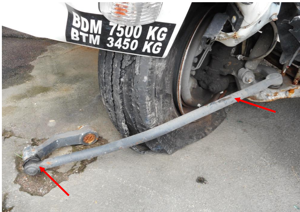
Photo 20 shows the various undercarriage components at the front right wheel of the Motor Lorry, in particular the steering tie rod end and ball joints (arrowed). were all found to be damage and dislodged from the steering box.
