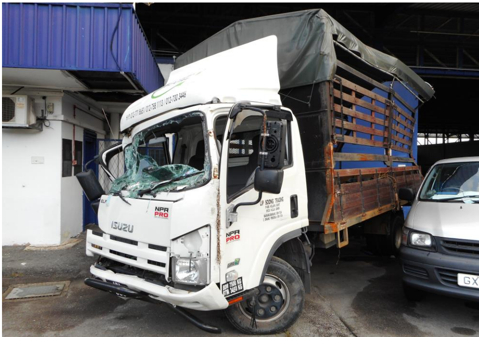
Photo 4 shows a general view of the left body of the Motor Lorry at the time of our inspection. The Motor Lorry was observed to have sustained major damages to its front windscreen, doors that was crushed and dislodged due to the accident's impact.
