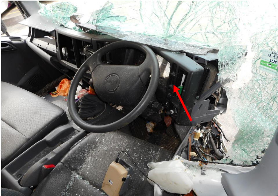
Photo 26 shows the damages on the Motor Lorry's instrument cluster induce impact from the accident rendering it not serviceable at the time of inspection. (Unable to operate)
