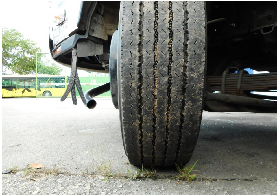
Photo 10 shows the condition of the front left tyre of the Motor Lorry, which observed to be in serviceable condition with remaining tread depth of approximately 10.7mm. The tyre, which was wrapped around standard alloy wheel rim, was also observed to be sufficiently inflated for vehicular operation.
