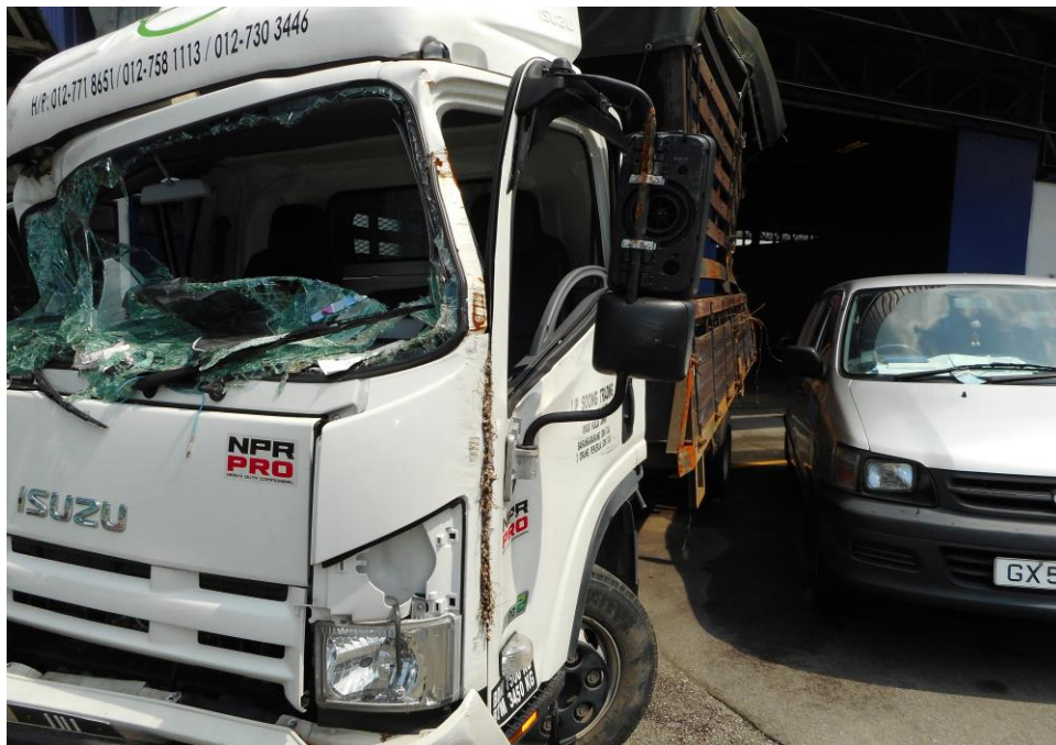
Photo 6 shows the close up view of the left door of the Motor Lorry at the time of our inspection. The Motor Lorry was observed to have sustained major damages to its front windscreen, doors that was crushed and dislodged due to the accident's impact.
