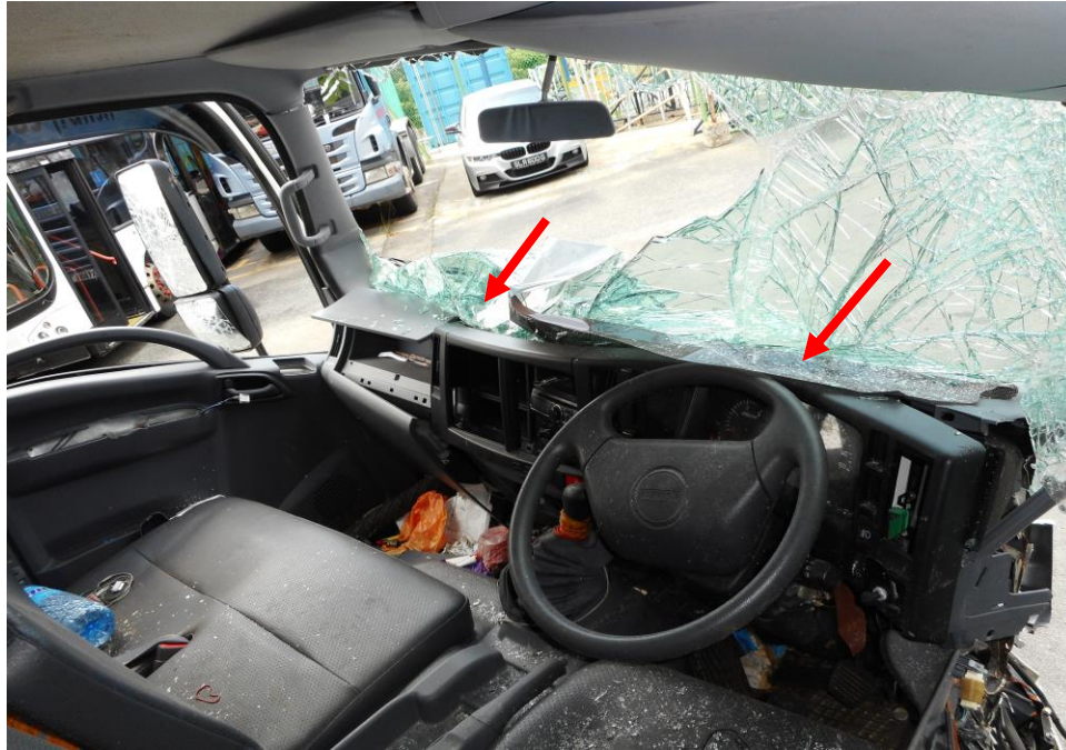
Photo 9 shows the close up view of the interior cabin of the Motor Lorry. It was observed to have sustained extensive induced damages to the dashboard and foot well which caused the whole to shift inwards the cabin.
