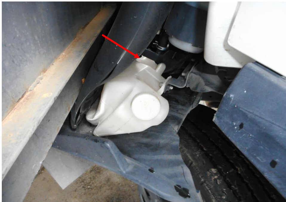
Photo 17 shows the engine coolant reservoir (arrowed) of the Motor Lorry crushed and emptied at the time of our inspection due to the induced damage from the accident.
