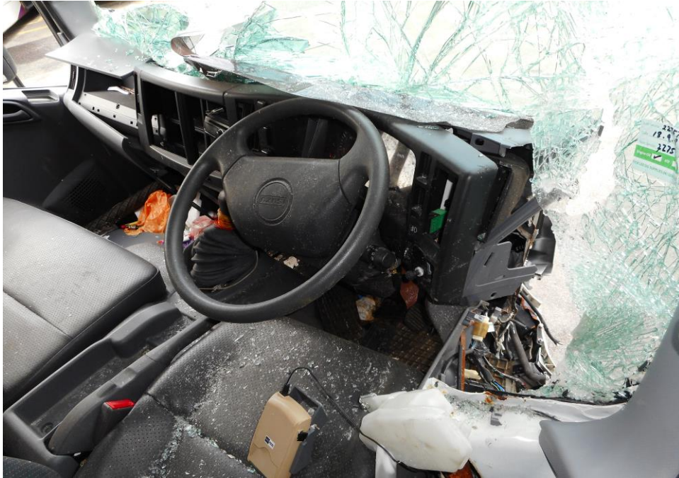
Photo 1 shows no mileage readings were recorded due to the damaged to the instrument cluster which holds the odometer of the Motor Lorry at the time of our inspection.
