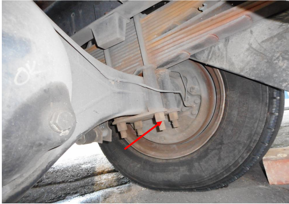
Photo 25 shows the various undercarriage components at the rear left wheel of the Motor Lorry, in particular the brake hose and drum brake (arrowed). The various undercarriage components of the Motor Lorry were all found to be intact without any visible damage. There was also no sign of fluid stain(s) observed on the various undercarriage components.
