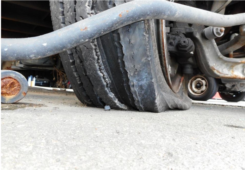
Photo 11 shows the condition of the front right tyre of the Motor Lorry, which was observed to have been cut and delated likely caused by the accident with remaining tread depth of approximately 9.1mm. The tyre was wrapped around standard alloy wheel rim.
