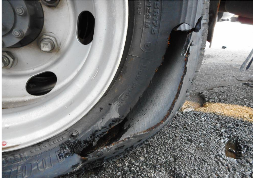
Photo 13 shows the condition of the rear right tyre of the Motor Lorry, which was observed to have been cut and delated likely caused by the accident with remaining tread depth of approximately 8.7mm. The tyre was wrapped around standard alloy wheel rim.
