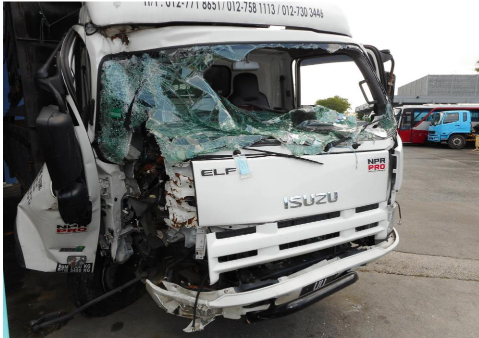
Photo 7 shows the close up view of the right door of the Motor Lorry at the time of our inspection. The Motor Lorry was observed to have sustained major damages to its front windscreen, doors that was crushed and dislodged due to the accident's impact.
