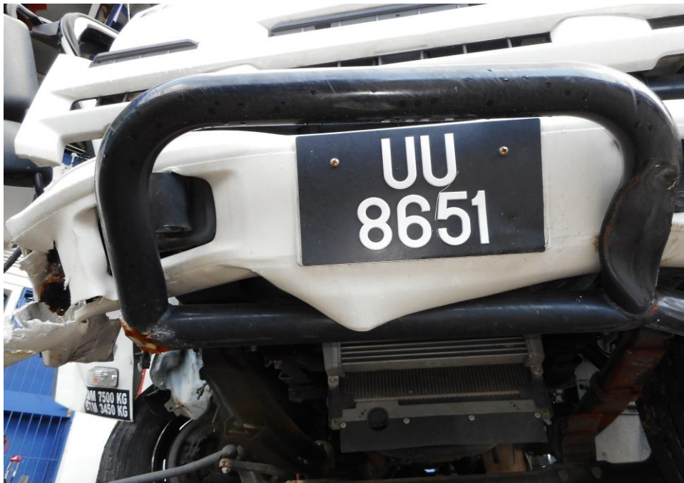
Photo 3 shows the number plate and the general view of the rear portion of the Motor Lorry at the time of our inspection. The Motor Lorry was observed sustained major damages to its rear which the tailgate was shifted out of place, likely due to the accident's impact.
