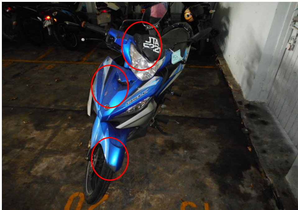
Photo 2 shows a general view of the front body of the Motorcycle at the time of our inspection. The Motorcycle was observed to have sustained relatively minor damages at time of inspection. The damages were observed to be confined to its front & right side of the Motorcycle.
