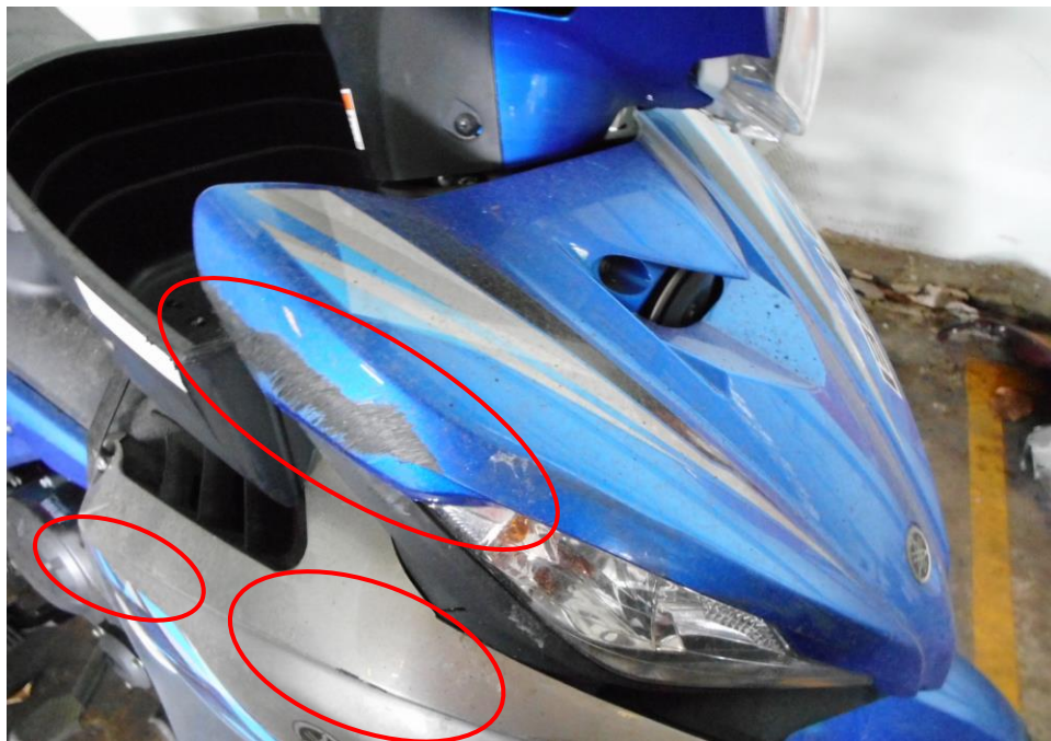
Photo 6 shows a close up view of the front right body of the Motorcycle at the time of our inspection. The Motorcycle was observed to have sustained relatively minor damages at time of inspection. The damages were observed to be at its front & right side fairing of the Motorcycle.
