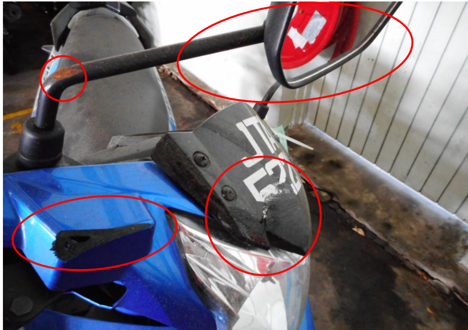
Photo 3 shows a close up view of the front right body of the Motorcycle at the time of our inspection. The Motorcycle was observed to have sustained relatively minor damages at time of inspection. The damages were observed to be confined to its front, right side of the Motorcycle.
