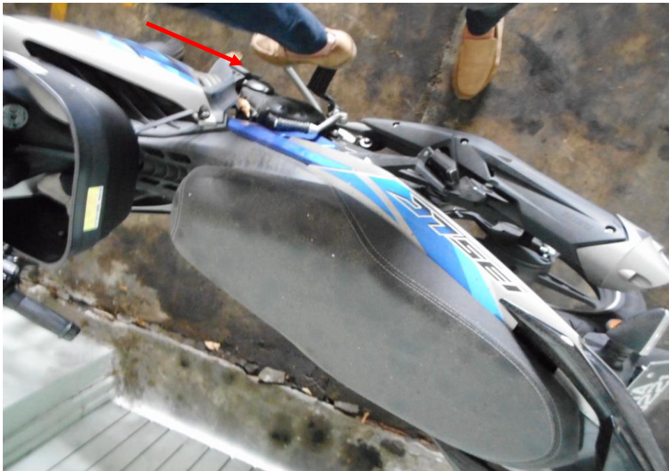
Photo 20 shows testing of the braking of the rear brake in progress. The braking force was felt upon pressing the brake lever. The brakes are in serviceable condition.
