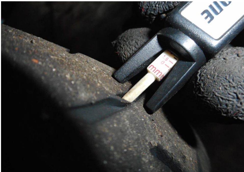
Photo 10 shows the rear tyre of the Motorcycle. The rear tyre was observed with remaining tread depth of approximately 2mm. The tyre was also observed to be sufficiently inflated for vehicular operation.
