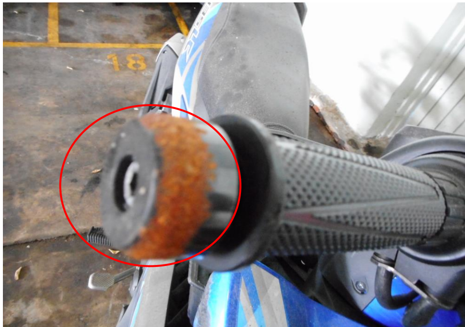
Photo 4 shows a close up view of the front right body of the Motorcycle at the time of our inspection. The Motorcycle was observed to have sustained relatively minor damages at time of inspection. The damages were observed to be confined to its front, right side handle bar of the Motorcycle.
