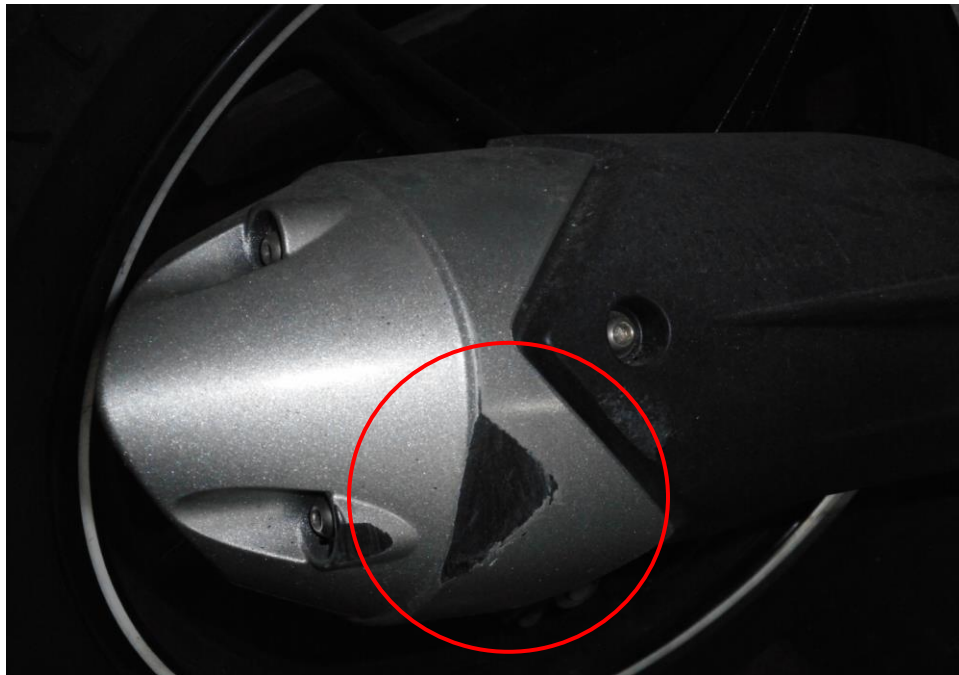
Photo 8 shows a close up view of the exhaust area of the Motorcycle at the time of our inspection. The Motorcycle was observed to have sustained relatively minor damages at time of inspection. The damages were observed to be at the exhaust muffer of the Motorcycle.
