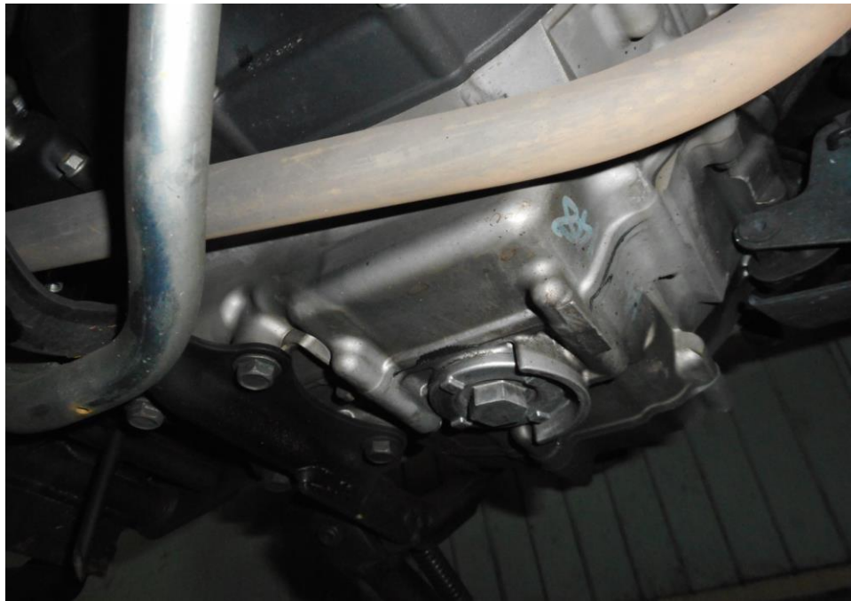
Photo 13 shows no sign(s) or indication(s) of fluid leak observed around the underside of the engine area of the Motorcycle
