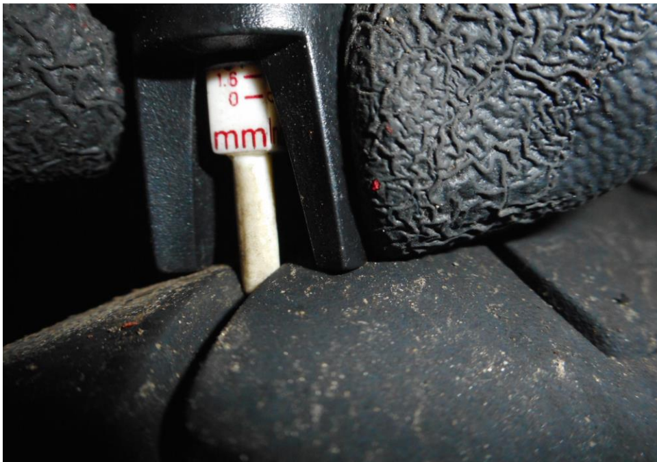
Photo 12 shows the front tyre of the Motorcycle. The front tyre was observed with remaining tread depth of approximately 2mm. The tyre was also observed to be sufficiently inflated for vehicular operation.
