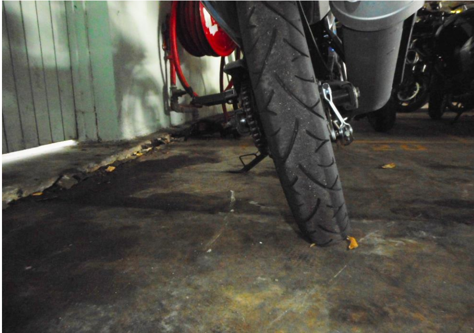
Photo 9 shows the rear tyre of the Motorcycle. The rear tyre was observed to be in serviceable condition & the tyre was also observed to be sufficiently inflated for vehicular operation.
