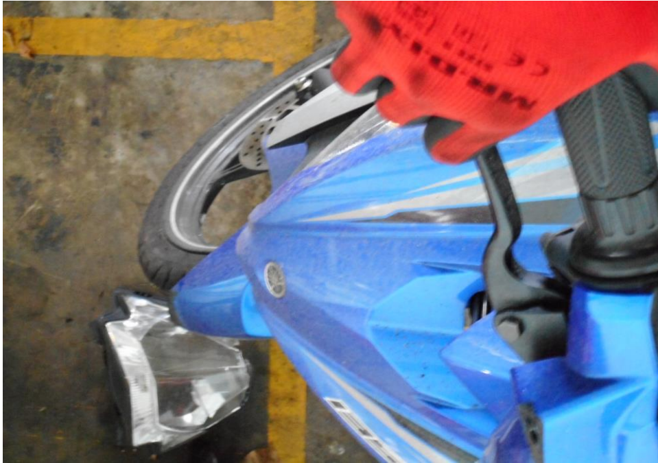
Photo 19 shows testing of the braking of the front brake in progress. The braking force was felt upon pressing the brake lever. The brakes are in serviceable condition.
