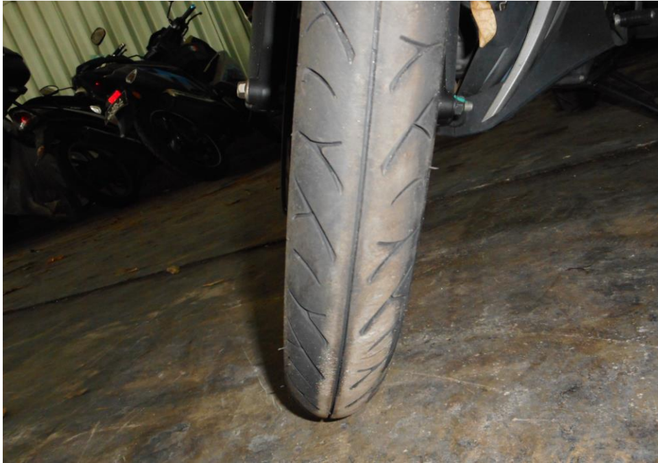
Photo 11 shows the front tyre of the Motorcycle. The front tyre was observed to be in serviceable condition & the tyre was also observed to be sufficiently inflated for vehicular operation.
