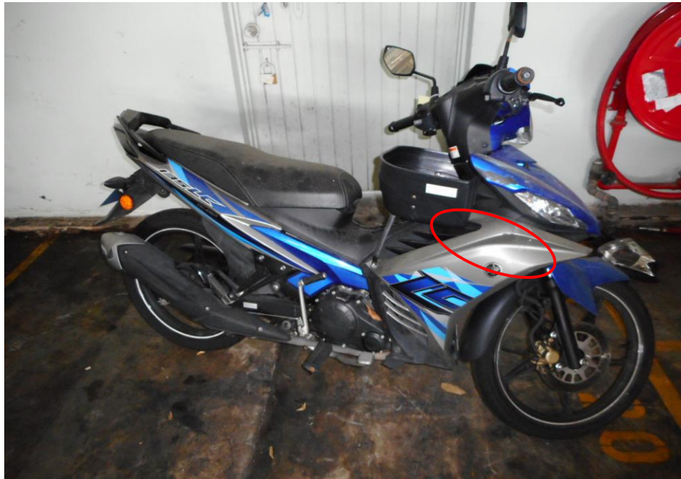
Photo 5 shows a general view of the front right body of the Motorcycle at the time of our inspection. The Motorcycle was observed to have sustained relatively minor damages at time of inspection. The damages were observed to be at its front & right side fairing of the Motorcycle.
