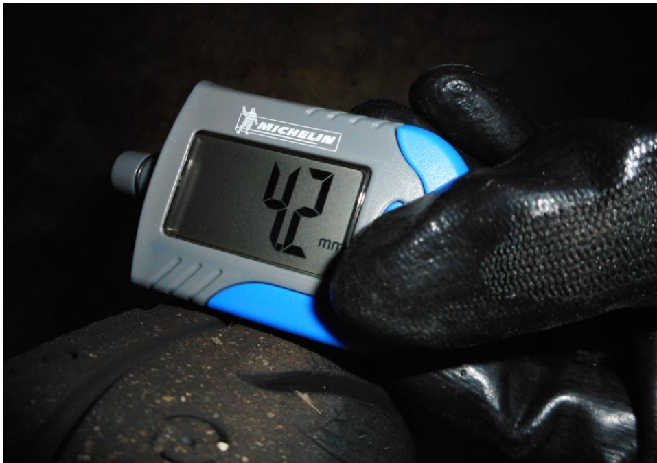
Photo 10 shows the rear tyre of the Motorcycle. The rear tyre was observed remaining tread depth of 4.2mm. The tyre was also observed to be sufficiently inflated for vehicular operation.
