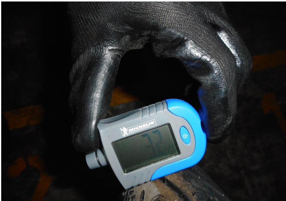
Photo 12 shows the front tyre of the Motorcycle. The front tyre was observed remaining tread depth of 3.2mm & was also observed to be sufficiently inflated for vehicular operation.
