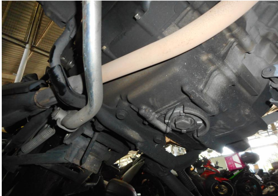
Photo 13 shows no sign(s) or indication(s) of fluid leak observed around the undercarriage of the engine area of the Motorcycle.
