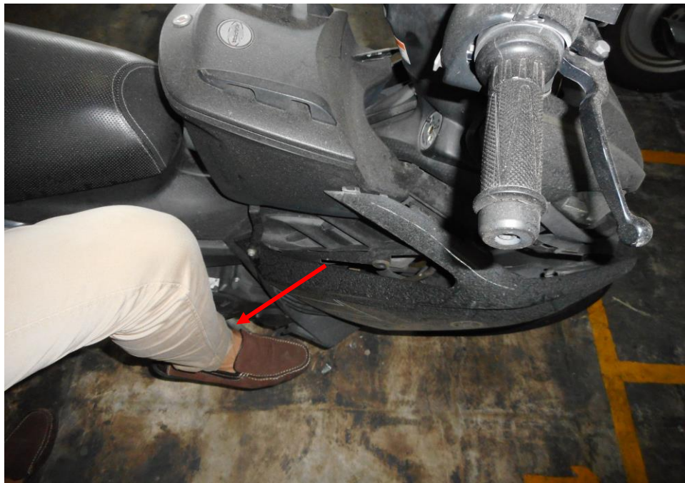
Photo 22 shows testing of the braking of the rear brake in progress. The braking force was felt upon pressing the brake lever. The brakes are in serviceable condition.
