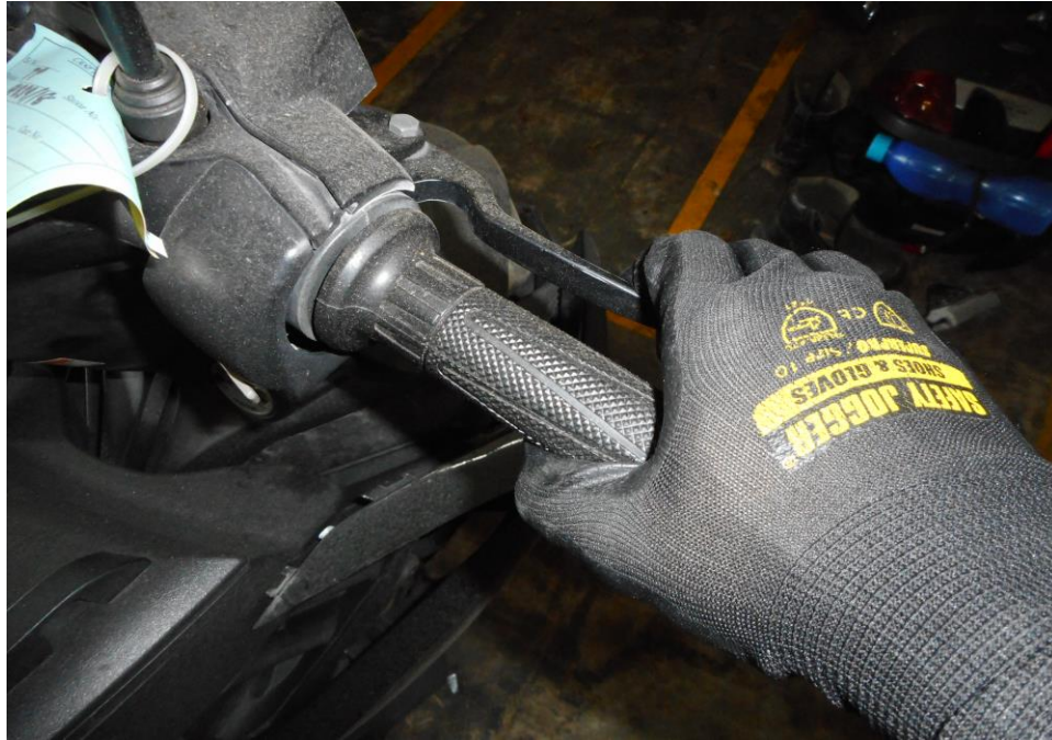
Photo 21 shows testing of the braking of the front brake in progress. The braking force was felt upon pressing the brake lever. The brakes is in serviceable condition
