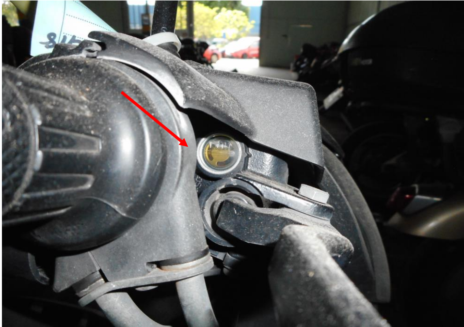
Photo 17 shows our checks on the brake fluid (front) reservoir had also indicated that the brake fluid was of sufficient level for operational purposes, and without contamination.
