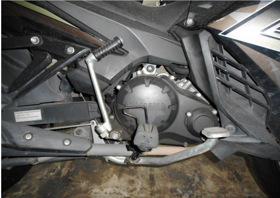
Photo 14 shows no sign(s) or indication(s) of fluid leakage stain observed around the right side engine area of the Motorcycle.
