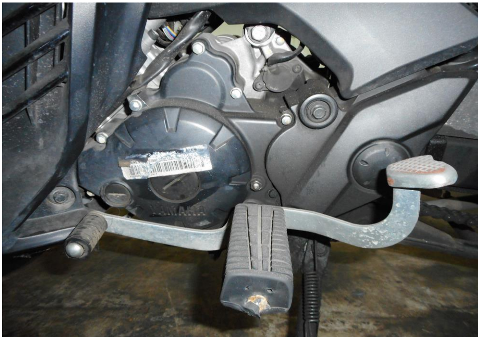
Photo 15 shows no sign(s) or indication(s) of fluid leakage stain observed around the left engine area of the Motorcycle.
