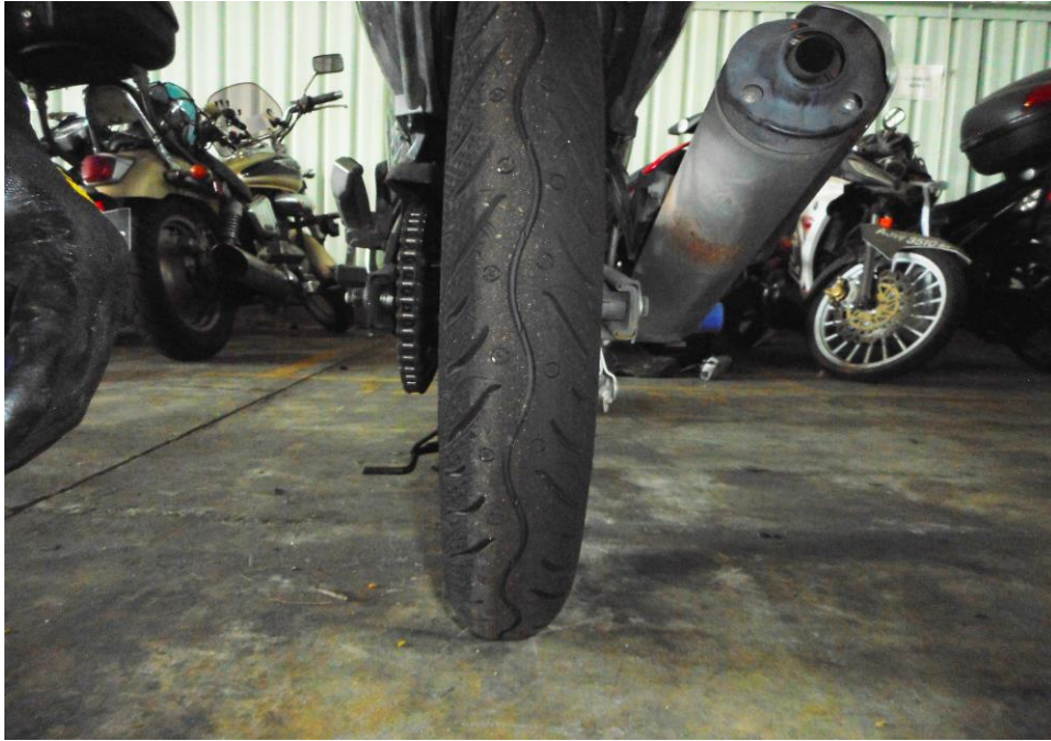
Photo 9 shows the rear tyre of the Motorcycle. The rear tyre was observed to be in serviceable condition & was also observed to be sufficiently inflated for vehicular operation.
