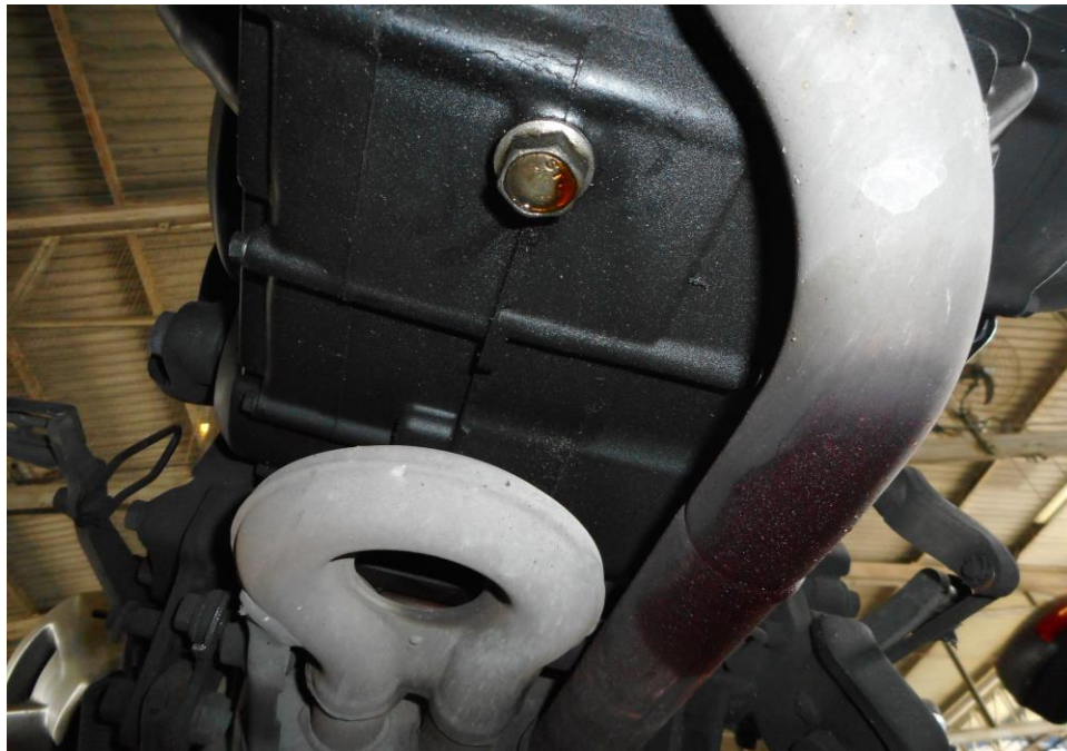
Photo 13 shows minimal flesh fluid leakage observed around the drain plug and the exhaust area underneath the engine area of the Motorcycle.
