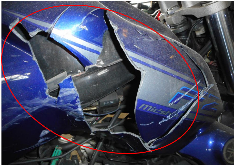
Photo 4 shows a close up view of the damages to the fuel tank cover and the battery panel at time of inspection likely due to the cause of the accident. See above
