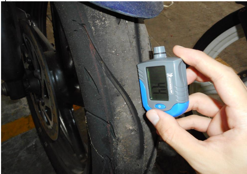
Photo 10 shows the front tyre of the Motorcycle. The rear tyre was observed with remaining tread depth of approximately 4.4mm. The tyre was also observed to be sufficiently inflated for vehicular operation.
