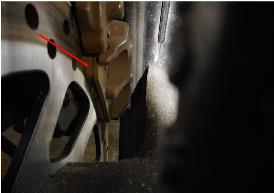
Photo 21 shows a close-up view our checks on the brake pad (front). The frictional material was observed to be in a sufficient level for operational purposes.
