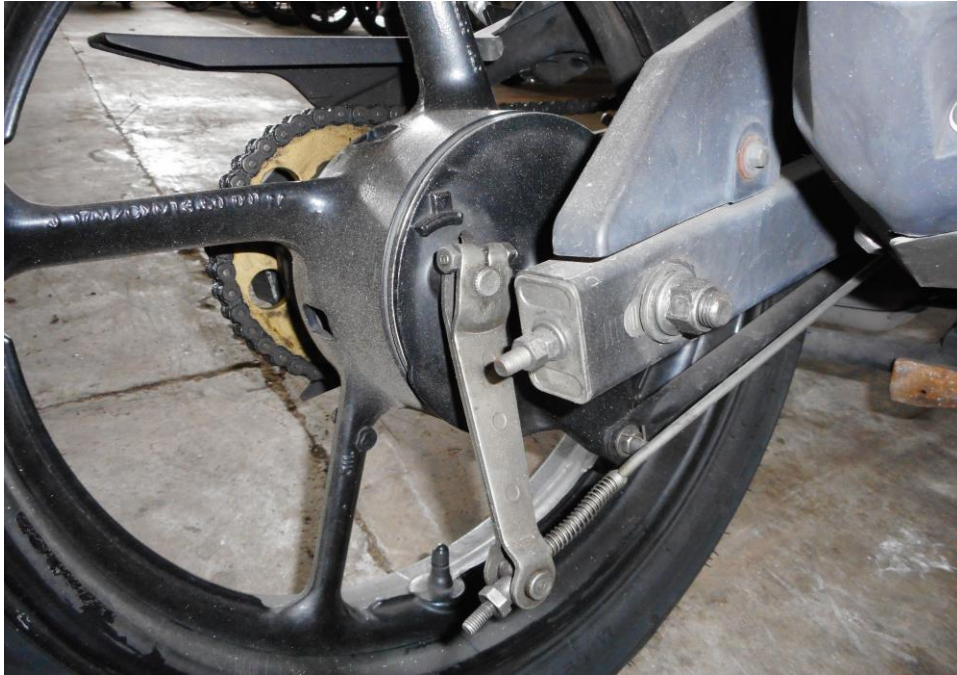
Photo 20 shows our checks on the drum brake housing (rear) no leakage or fluids is found present around it
