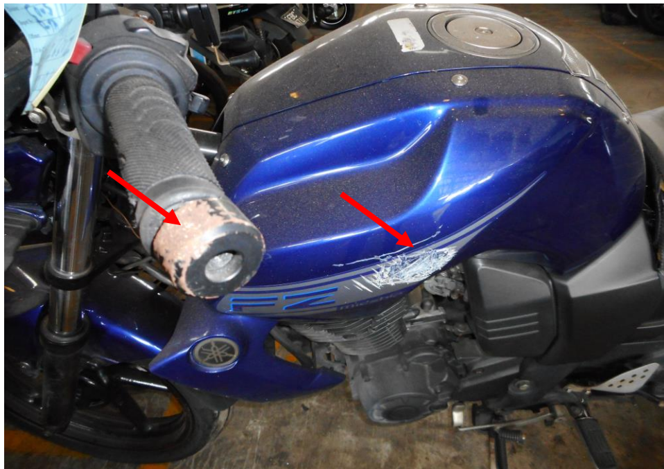
Photo 8 shows a close up view of the damages to the fuel tank cover and the rear panel at time of inspection likely due to the cause of the accident.
