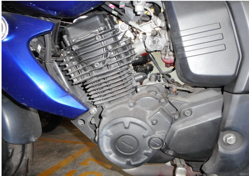
Photo 14 shows no sign(s) or indication(s) of fluid leakage stain observed around the left engine area of the Motorcycle.
