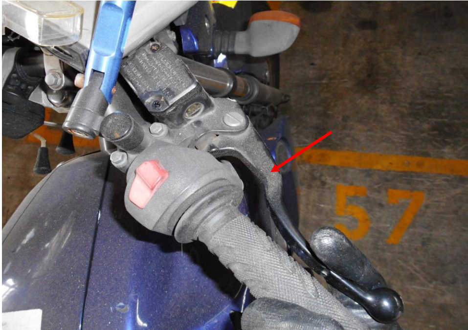
Photo 22 shows testing of the braking of the front brake in progress. The braking force was not felt upon pressing the brake lever as the damage likely due to the accident.
