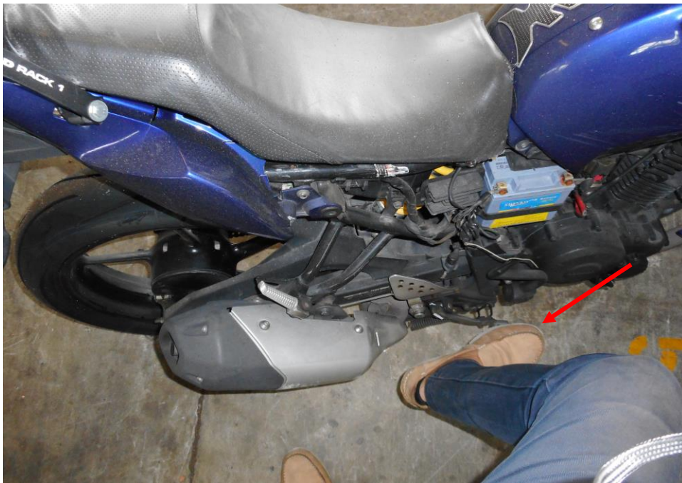
Photo 23 shows testing of the braking of the rear brake in progress. The braking force was felt upon stepping on the brake lever. The brakes are in serviceable condition.
