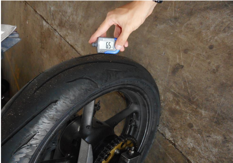
Photo 12 shows the rear tyre of the Motorcycle. The front tyre was observed with remaining tread depth of approximately 6.5mm. The tyre was also observed to be sufficiently inflated for vehicular operation.
