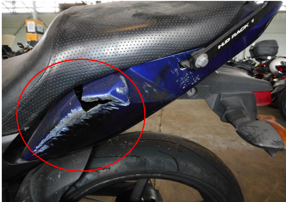
Photo 9 shows a close up view of the damages to the rear panel at time of inspection likely due to the cause of the accident.
