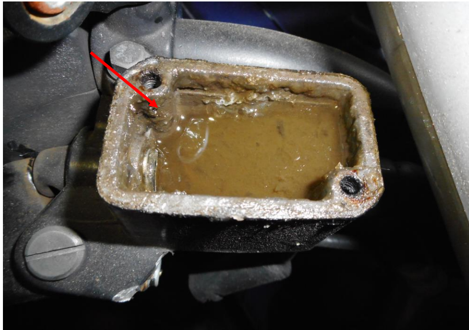
Photo 18 shows our checks on the brake fluid (front) reservoir had also indicated that the brake fluid is sufficient level and in serviceable operational purposes.
