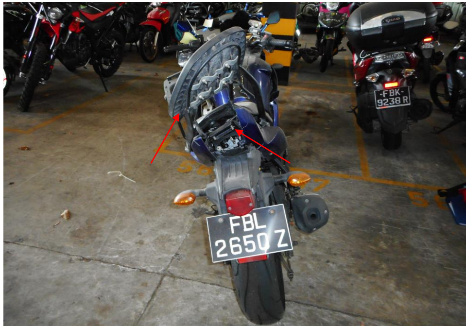
Photo 6 shows a general view of the rear body of the Motorcycle at the time of our inspection. The Motorcycle was observed to have sustained damages at the rear box carrier likely due to the cause of the accident.
