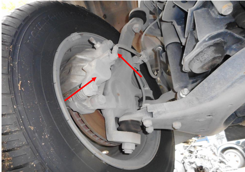
Photo 20 shows the various undercarriage components at the front and right wheel of the Motor Lorry, in particular the brake hose and callipers (arrowed). The various undercarriage components of the Motor Lorry were all found to be intact without any visible damage. There was also no sign of fluid stain(s) observed on the various undercarriage components.
