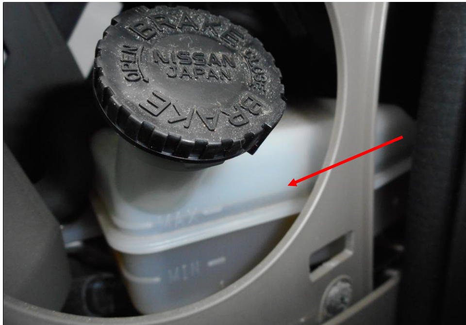
Photo 12 shows the brake fluid reservoir of the Motor Lorry at the time of our inspection. The brake fluid was observed to be of sufficient level and without any visible contamination (arrowed).
