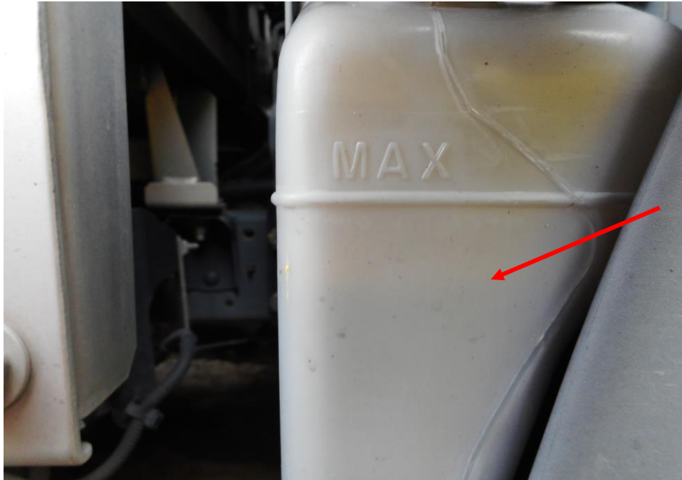
Photo 13 shows the engine coolant reservoir of the Motor Lorry at the time of our inspection. The engine coolant was observed to be of sufficient level and without any visible contamination (arrowed).
