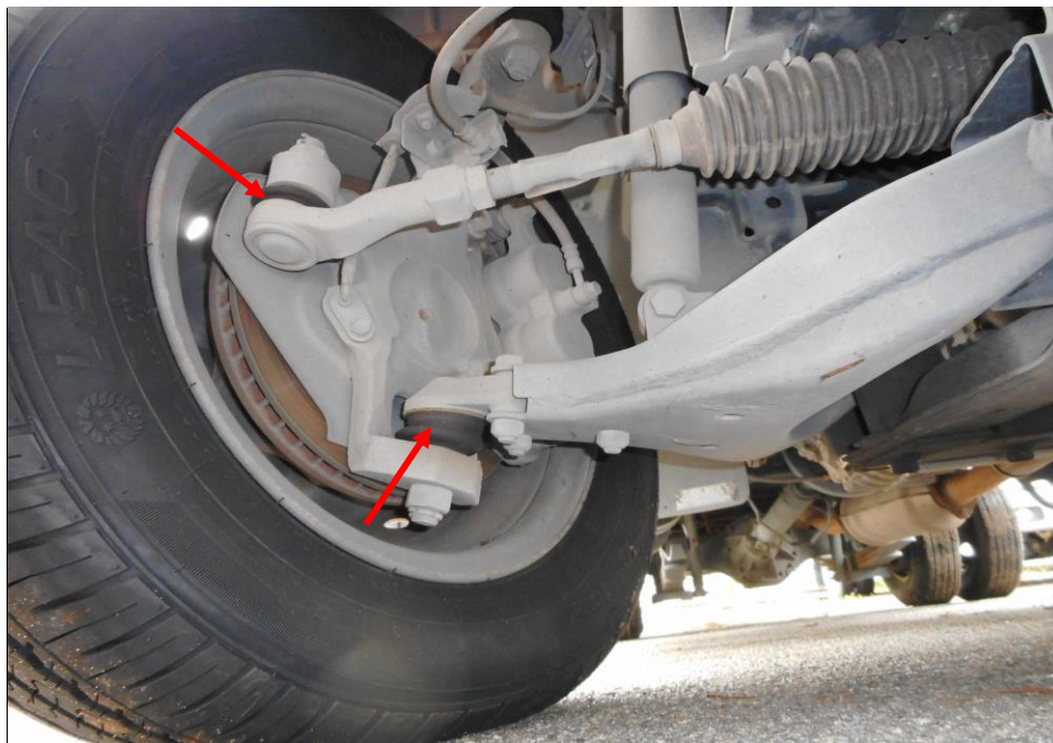
Photo 17 shows the various undercarriage components at the front left wheel of the Motor Lorry, in particular the steering tie rod end and ball joints (arrowed). The various undercarriage components of the Motor Lorry were all found to be intact without any visible damage. There was also no sign of fluid stain(s) observed on the various undercarriage components.
