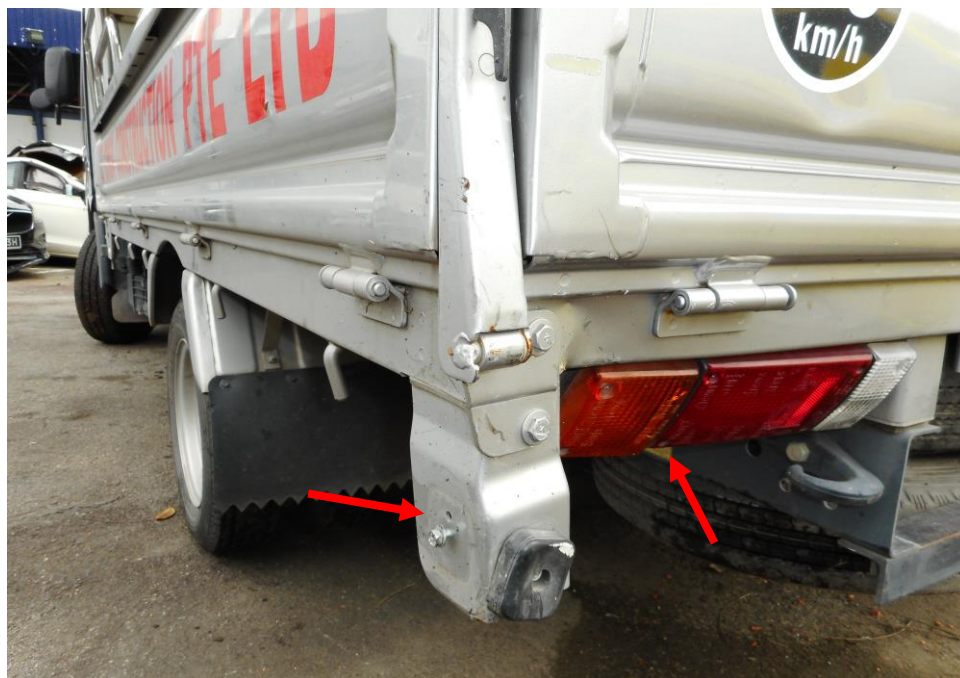
Photo 6 shows the close up view of the rear tailgate of the Motor Lorry. It was observed to have sustained damages around the rear left brake lamps and body panel (Arrowed) as a result of the accident.
