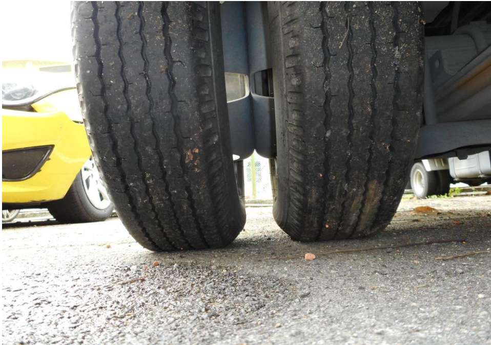
Photo 10 shows the condition of the rear right tyres of the Motor Lorry, which were observed to be in serviceable condition with remaining, tread depth of approximately 3.4mm.
