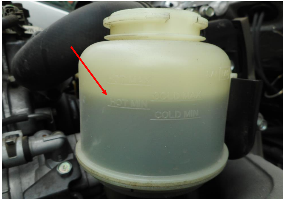
Photo 15 shows the power steering reservoir of the Motor Lorry at the time of our inspection. The power steering fluid was observed to be of sufficient level and without any visible contamination (circled).
