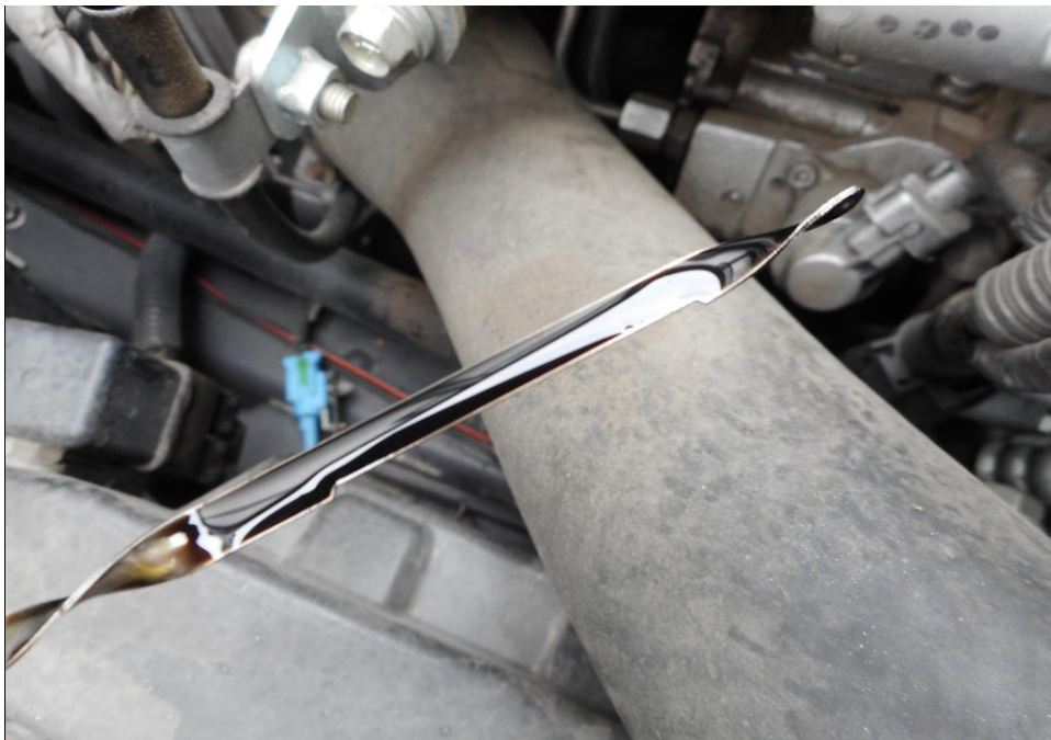
Photo 14 shows the engine dip stick of the Motor Lorry at the time of our inspection. The engine oil was observed to be of sufficient level and without any visible contamination.
