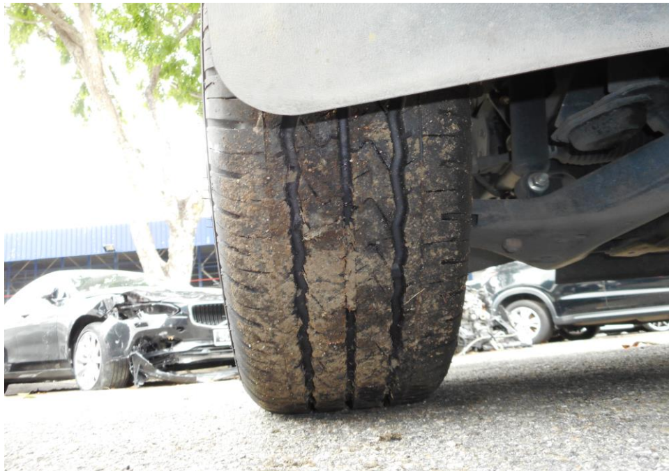
Photo 7 shows the condition of the front left tyre of the Motor Lorry, which observed to be in serviceable condition with remaining tread depth of approximately 8.1mm. The tyre, which was wrapped around standard alloy wheel rim, was also observed to be sufficiently inflated for vehicular operation.
