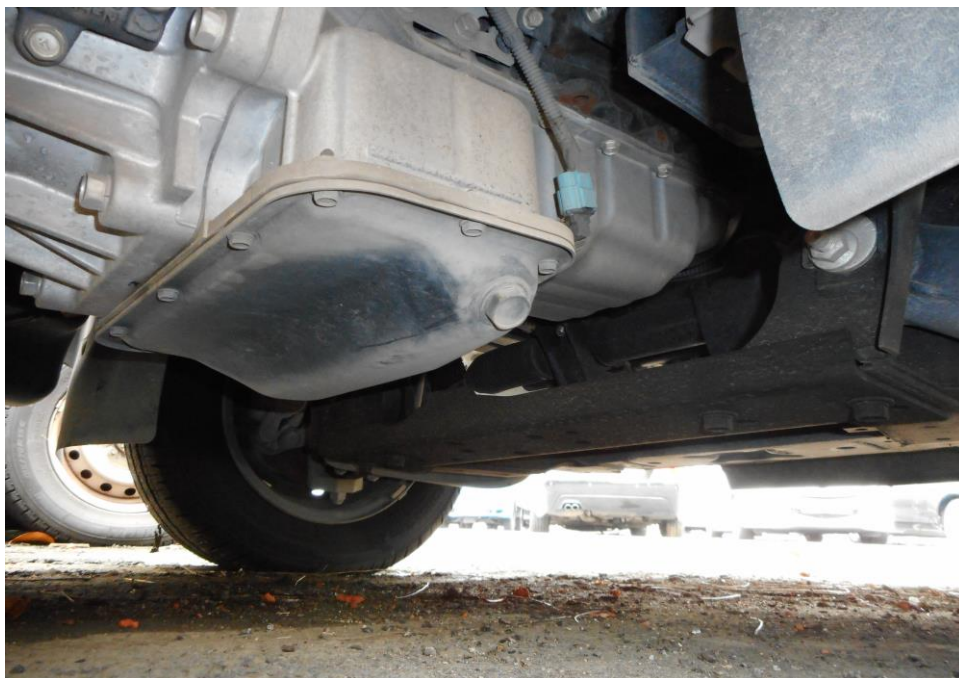
Photo 16 shows the undercarriage of the engine of the Motor Lorry at the time of our inspection. There was also no sign(s) or indication(s) of fresh fluid leakage and/or fluid stain within the engine.
