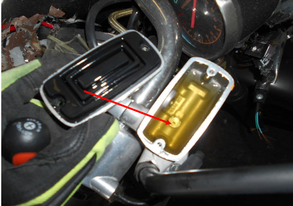
Photo 19 shows the front brake fluid reservoir of the Motorcycle. It was observed to be of sufficient level without any contamination at time of our inspection.
