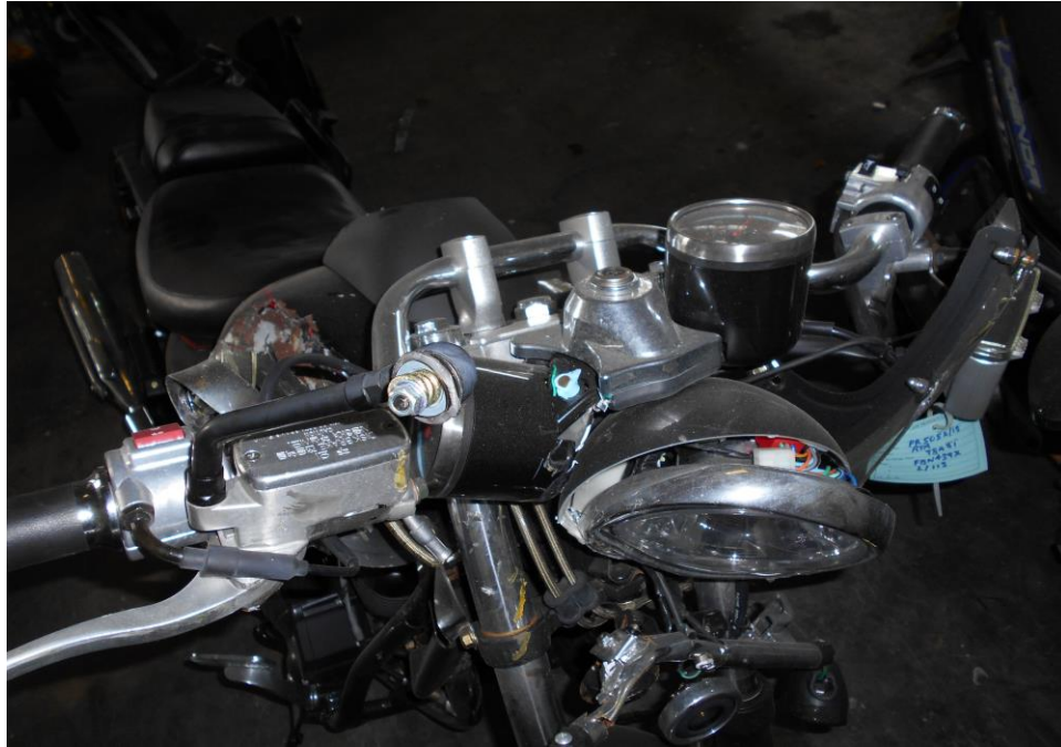
Photo 15 shows the handle bar and front fork was observed to be bent inwards as a result of the accident. Hence, we are not able to conduct any tests on the steering system of the Motorcycle.
