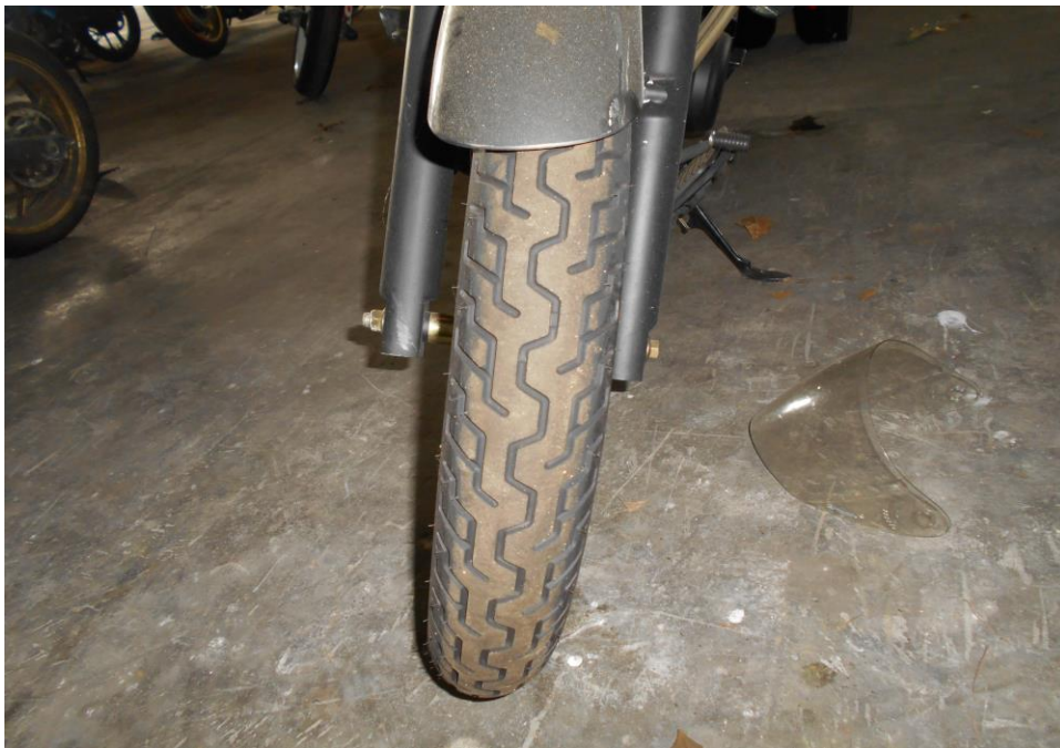
Photo 11 shows the front tyre of the Motorcycle. The pattern of the tread was clearly visible with remaining tread depth of approximately 5mm. There was no tear, burst mark(s) and/or punctured hole(s) on the sidewalls as well as across the tread of the front tyre.
