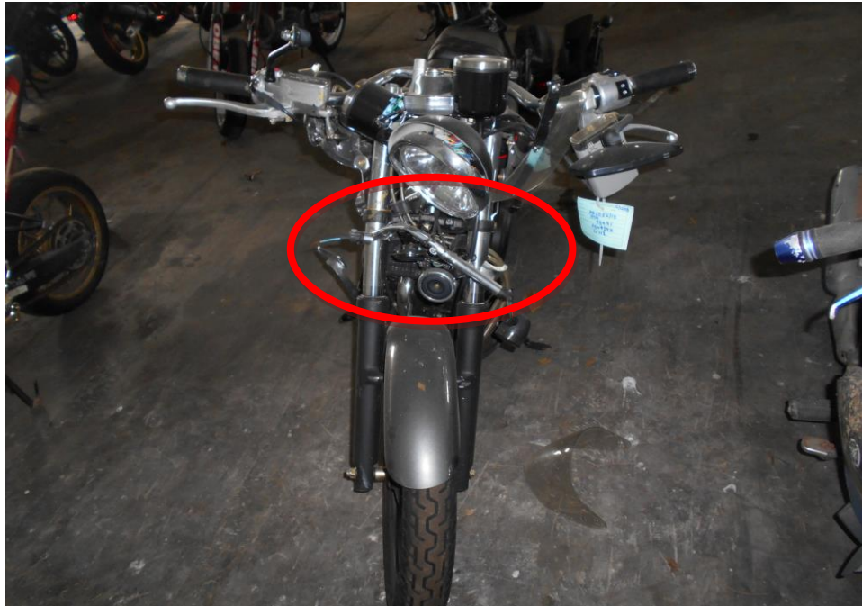
Photo 2 shows a general view of the front body of the Motorcycle at the time of our inspection. The Motorcycle was observed to be sustained with relatively extensive impact due to the accident collision. Amongst the body parts damaged was its steering system (circled), which was observed to be bent inwards.
