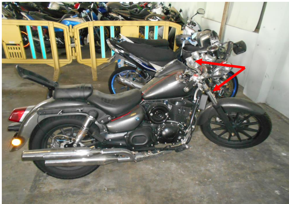
Photo 3 shows a general view of the front right body of the Motorcycle at the time of our inspection. The Motorcycle was observed to be sustained with relatively extensive impact due to the accident collision. Amongst the body parts damaged was its handle bar & front fork-steering system (arrowed), which was observed to be bent inwards.
