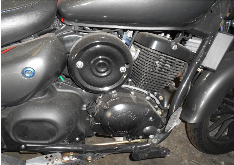
Photo 13 shows the semi-close view of the engine compartment. It was observed to be intact & undamaged unaffected by the accident's impact.
