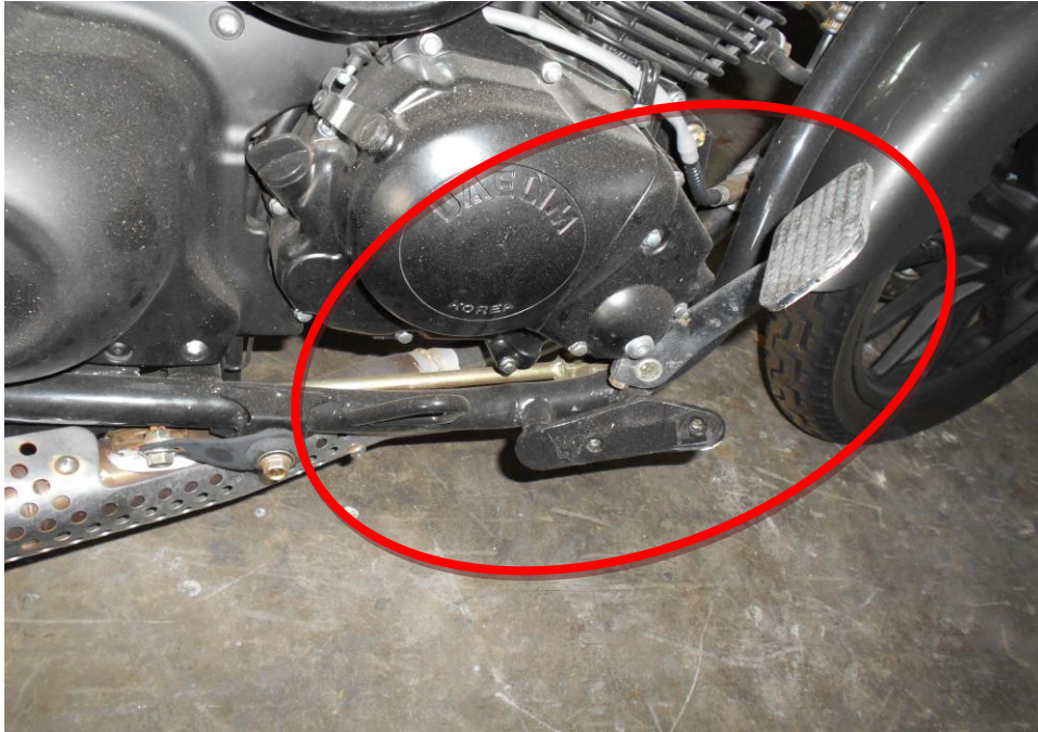
Photo 8 shows a close-up view of the missing right side foot rest of the Motorcycle at the time of our inspection. It was observed to be missing due to the accident collision.
