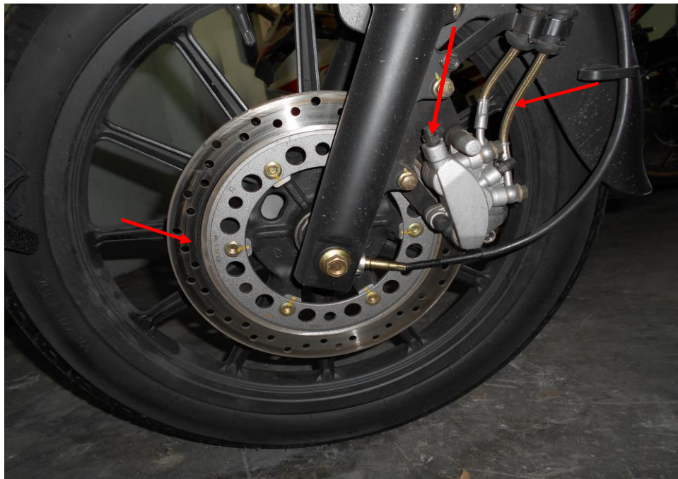
Photo 16 shows the front brake calliper, front brake disc and front brake hose of the Motorcycle (arrowed), which are all part of the components in the front brake system of the Motorcycle. Our visual checks of these various components had revealed all to be intact with no visible damage. No leakage of brake fluid was also observed.
