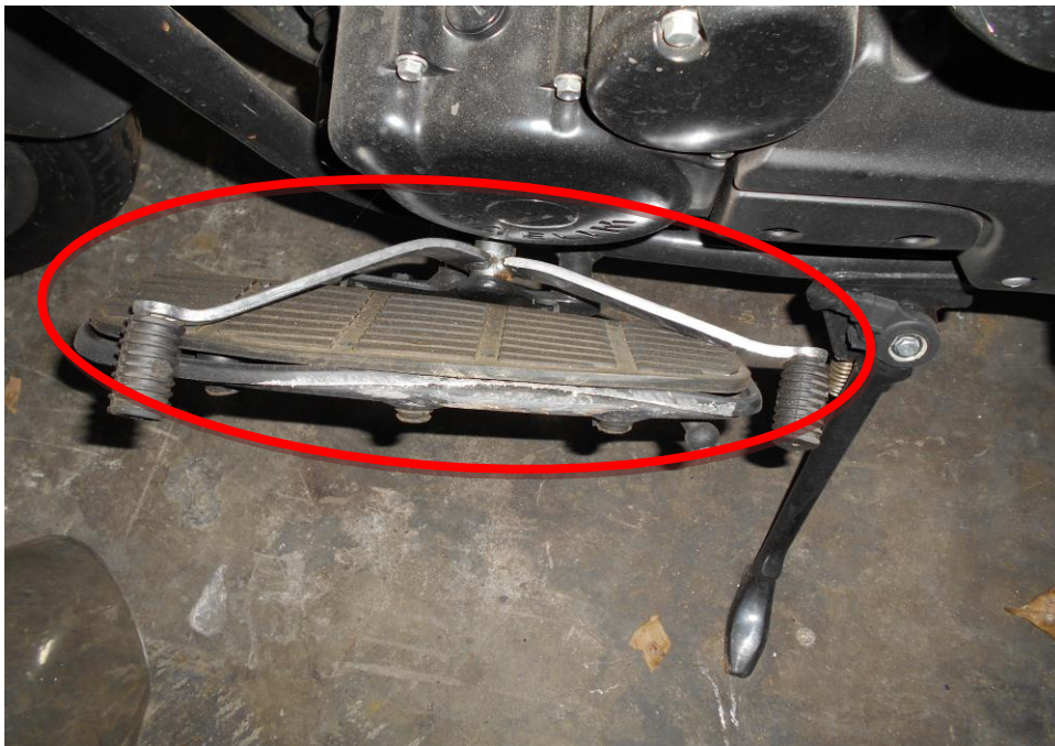
Photo 9 shows a close-up view of the stuck left side foot rest and gear shifter of the Motorcycle at the time of our inspection. It was observed to have sustained with damages due to the accident collision.
