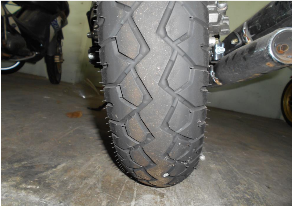
Photo 10 shows the rear tyre of the Motorcycle at the time of our inspection. The rear tyre was observed to be in serviceable condition with remaining tread depth of approximately 6mm. The tyre was also observed to be sufficiently inflated for vehicular operation. There was no significant damage observed on the rear wheel rim & tyre.
