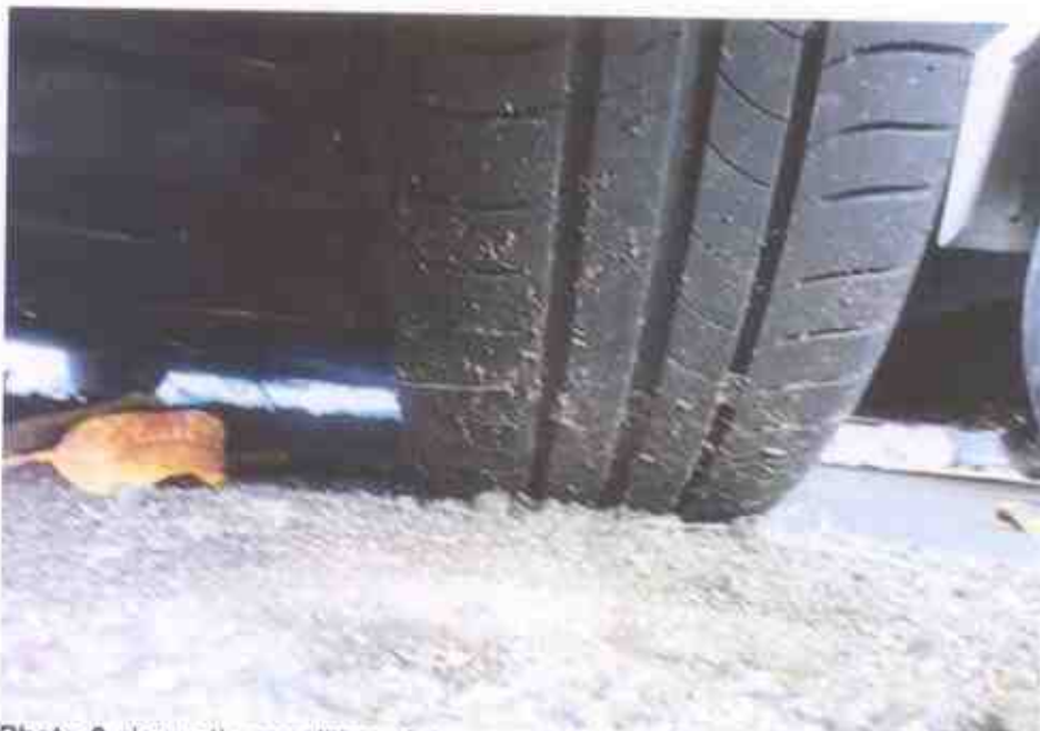
Photo 9 shows the condition of the rear right tyre of the Motor Taxi, which was observed to be in serviceable condition with remaining tread depth of approximately 4mm. There was also no tear, cut or burst mark(s) on the outer and the inner sidewalls as well as across the tread of the 4 tyres.
