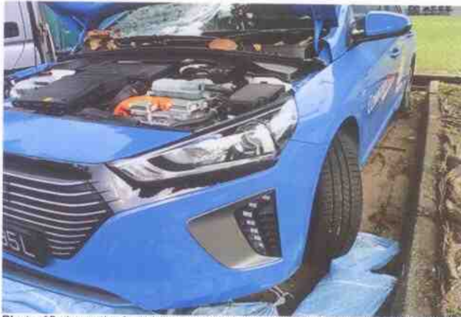
Photo 18 shows the front left wheel of the Motor Taxi turned to its full left. During our steering system test, we did not experience any abnormal free play and/or resistance when we had turned the steering wheel towards the left and right. This would suggest that the steering system of the Motor Taxi was likely to be in serviceable condition at the material time of accident.
