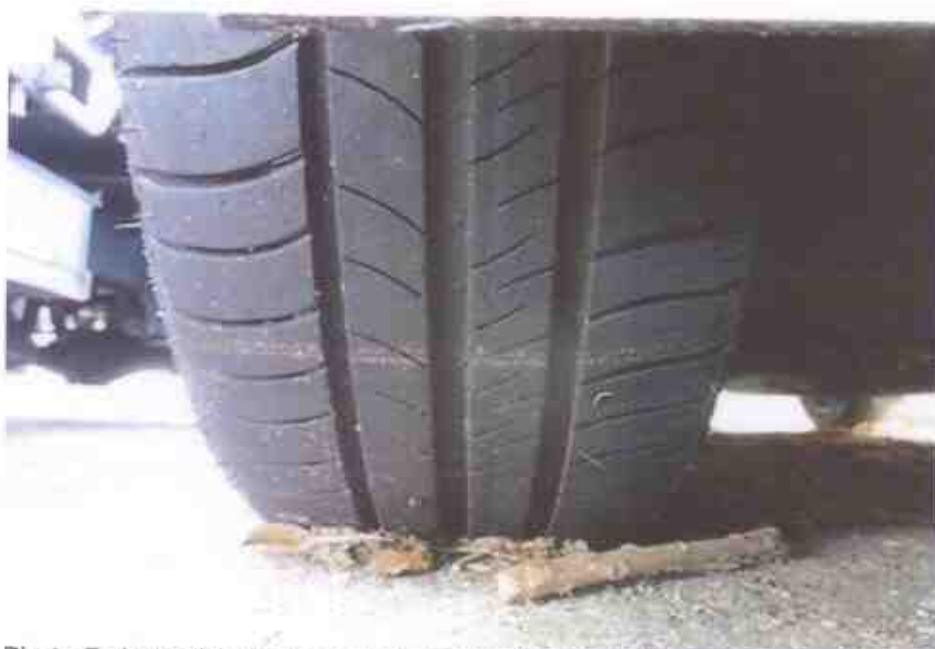
Photo 7 shows the condition of the front right tyre of the Motor Taxi, which was observed to be in serviceable condition with remaining tread depth of approximately 5mm. The tyre, which was wrapped around alloy wheel rim, was also observed to be sufficiently inflated for vehicular operation.
