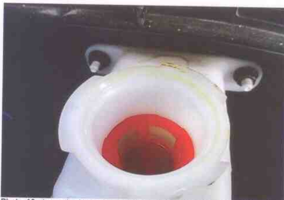
Photo 10 shows the brake fluid reservoir of the Motor Taxi at the time of our inspection. The brake fluid was observed to be of sufficient level and without any visible contamination.
