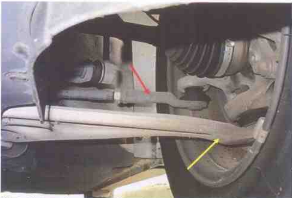
Photo 17 shows the various undercarriage components at the front left wheel of the Motor Taxi, which had included the steering tie rod (red arrow) and left drive shaft (yellow arrow). The various undercarriage components of the Motor Taxi were all found to be intact without any visible damage.
