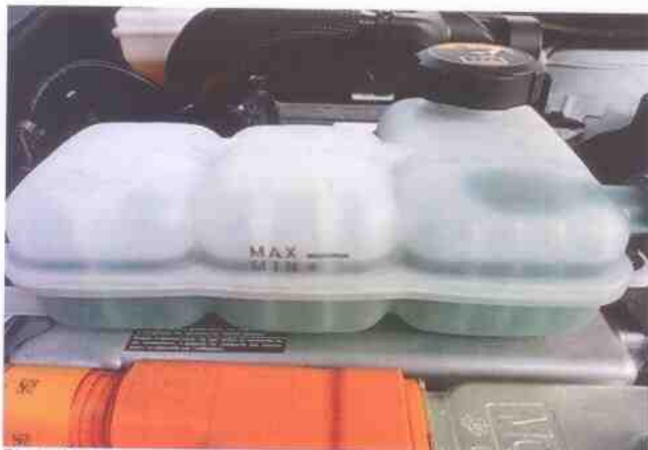
Photo 12 shows the coolant reservoir for the hybrid system of the Motor Taxi at the time of our inspection. The hybrid system coolant was observed to be of sufficient level and without any visible contamination.
