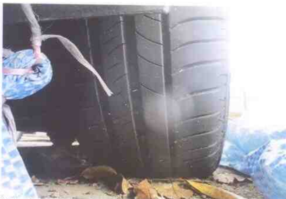
Photo 6 shows the condition of the front left tyre of the Motor Taxi, which was observed to be in serviceable condition with remaining tread depth of approximately 6mm. The tyre, which was wrapped around alloy wheel rim, was also observed to be sufficiently inflated for vehicular operation. There was no tear, cut or burst mark(s) on the outer and the inner sidewalls as well as across the tread of the 4 tyres.
