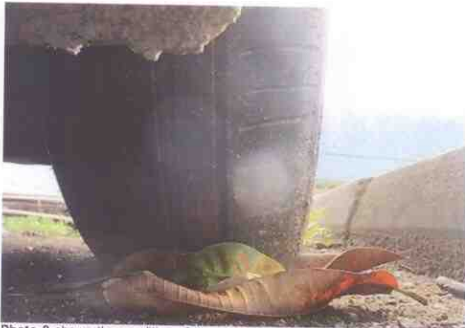
Photo 8 shows the condition of the rear left tyre of the Motor Taxi, which was observed to be in serviceable condition with remaining tread depth of approximately 5mm. The tyre, which was wrapped around alloy wheel rim, was also observed to be sufficiently inflated for vehicular operation. There was also no damage found on the 4 wheel rims of the Motor Taxi.
