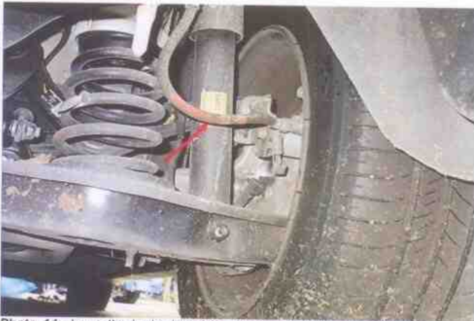
Photo 14 shows the brake hose/pipe (arrowed) at the rear right wheel of the Motor Taxi. We did not observe any leakage of brake fluid at the time of our inspection of the Motor Taxi. Static tests of the Motor Taxi's braking system had indicated that there was no internal leakage of pressure/vacuum. Hence the braking system was likely to be in serviceable condition at the material time of accident. The undercarriage components of the Motor Taxi were also all found to be intact and without any visible damage.
