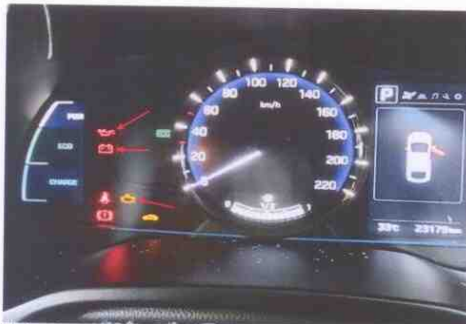
Photo 20 shows the warning lights for the various engine and electrical components of the Motor Taxi appearing on its instrument panel during the self-test when the engine is cranked, in particular the engine light, battery light and oil light (arrowed).
