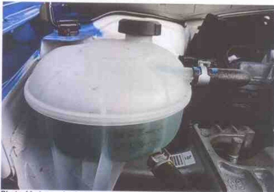
Photo 11 shows checks being carried out to the engine coolant of the Motor Taxi at the time of our inspection. The engine coolant was observed to be of sufficient level and without any visible contamination.
