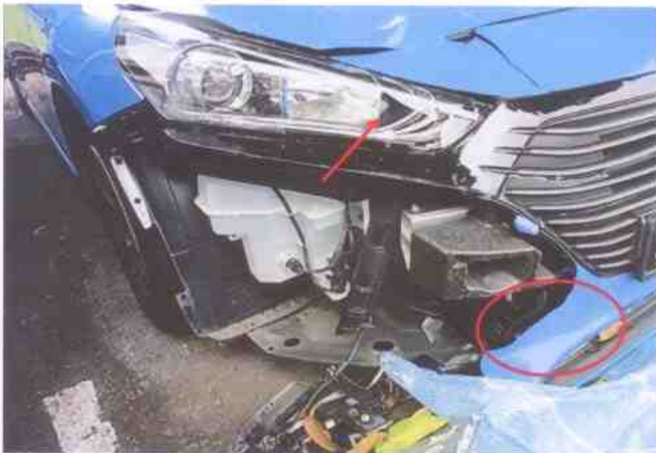
Photo 5 shows a closer view of the cracked right headlight (arrowed) as well as the dislodged front bumper (circled) of the Motor Taxi at the time of our inspection.
