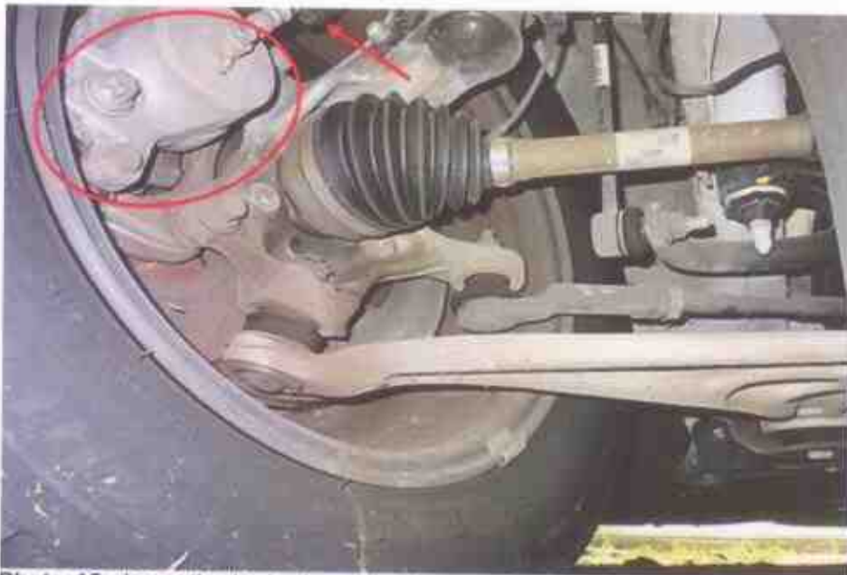
Photo 15 shows the brake hose/pipe (arrowed) at the front right wheel of the Motor Taxi. No leakage of brake fluid was observed. Visual examination of the various components of the braking system like the brake caliper (circled), brake pedal etc. had revealed all to be intact and without visible damage.
