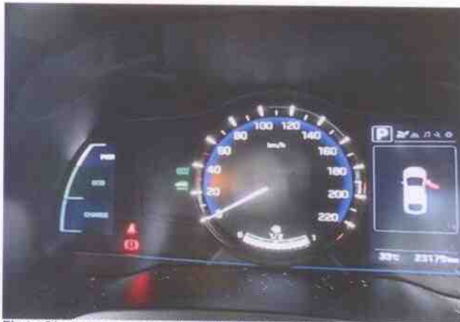
Photo 21 shows no warning lights illuminated on the instrument panel of the Motor Taxi after the engine was cranked. This would suggest that there was no abnormality to the various engine and electrical components of the Motor Taxi.
