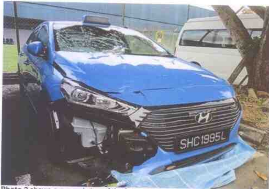
Photo 2 shows a general view of the front right body of the Motor Taxi at the time of our inspection. The Motor Taxi was observed to be in good general condition. However we had observed relatively minor impact damage that was confined to its right frontal portion. Its front bonnet was observed to have been dented; its front bumper was observed to have been dislodged and its front windscreen as well as right headlight was observed to have cracked.
