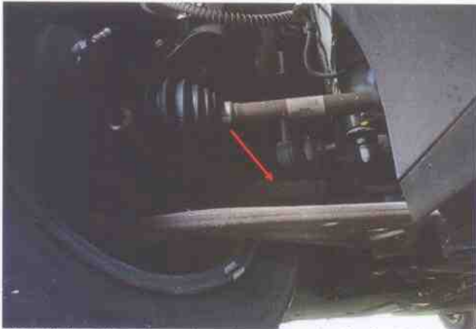
Photo 16 shows the various undercarriage components at the front right wheel of the Motor Taxi, in particular the steering tie rod (arrowed). The various steering components were all found to be intact, suggesting that the steering system of the Motor Taxi was likely to be in serviceable condition at the material time of accident. There was also no sign of fluid stain observed on the various undercarriage components at the front right wheel of the Motor Taxi.
